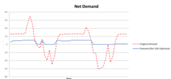
Net demand before and after optimisation – peaks have been shaved to reduce demand charges and solar export
