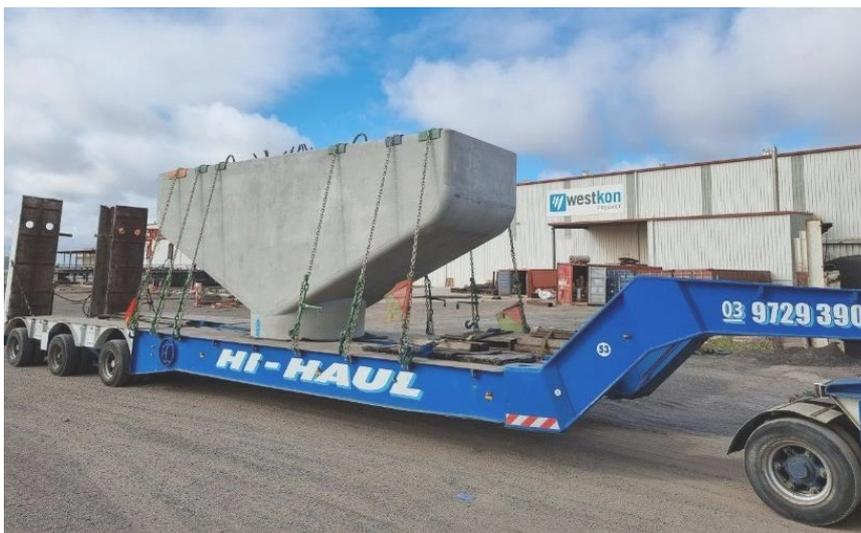
**Complete precast bridge crosshead delivery to site** [Credit Westkon Precast]
