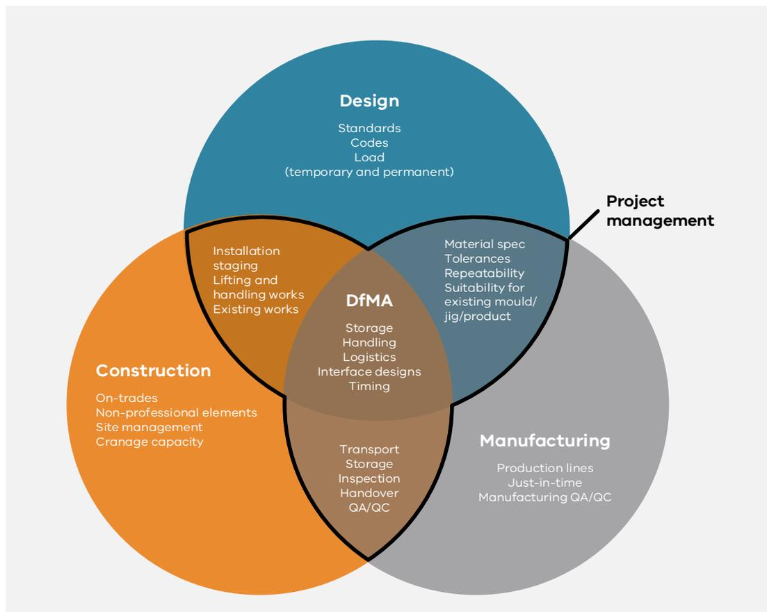
**DfMA - relating design, manufacturing and construction management of OSC**
