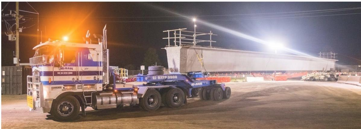
**Large precast beam delivery with rear dolly requiring clear swept path** [Credit Westkon]
