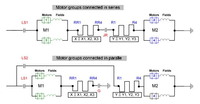
Figure 9 – Motor groups connected in series and parallel
