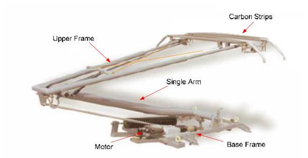
Figure 4 – Type of Pantograph on Tram 946
