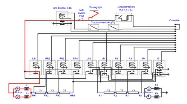
Figure 14 – Traction system circuit diagram with short circuit
