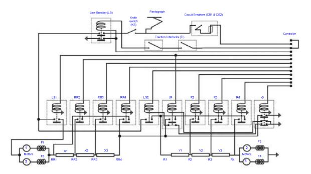
Figure 8 – Traction system circuit diagram
