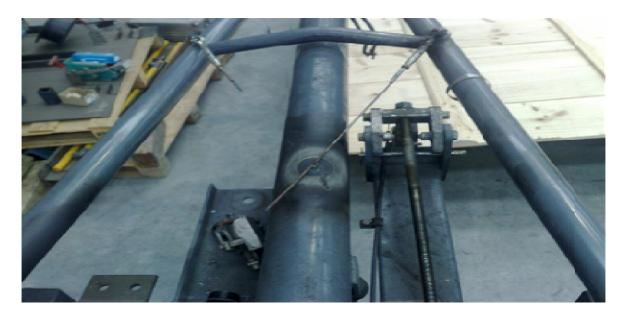
Figure 5 – Damage to pantograph caused by arcing
