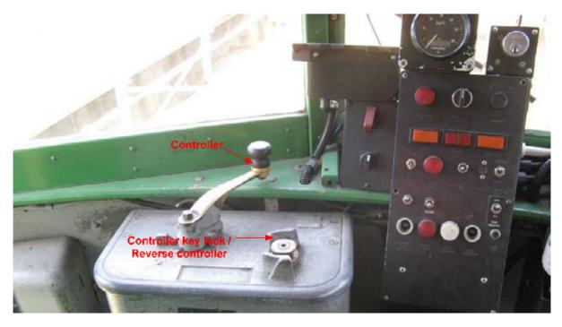
Figure 10 – Traction system controller
