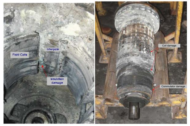
Figure 11 – Traction motor damage
