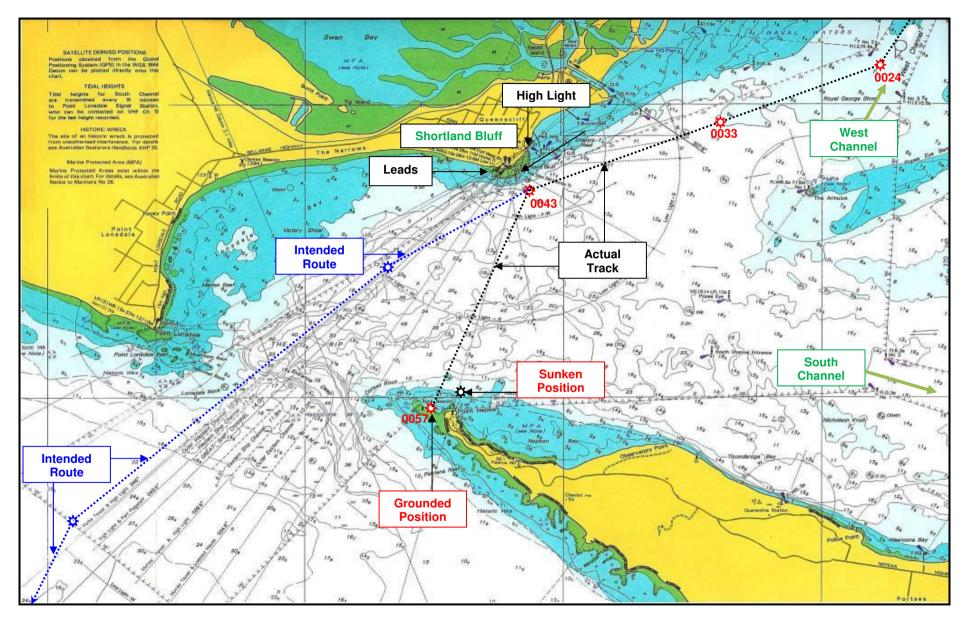
Figure 1: Lady Cheryl's track approaching Port Phillip Heads. Times shown are for the changes in vessel course, as recorded by VTS radar
