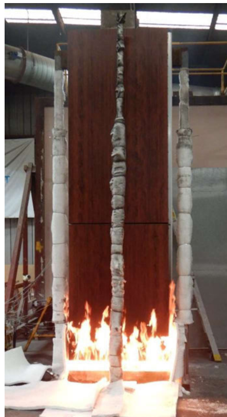
Figure 13 The specimen 2 minutes 44 seconds into the test (burner output at 100 kW)
