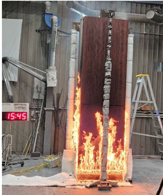
Figure 16 The specimen 15 minutes 45 seconds into the test (45 seconds after burner output was changed to 300 kW)
