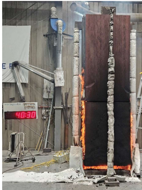
Figure 22 The specimen 40 minutes 30 seconds into the test (25 minutes 30 seconds after burner output was changed to 300 kW)
