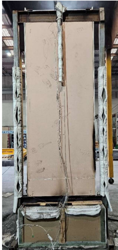
Figure 24 The specimen after the test – unexposed side.
