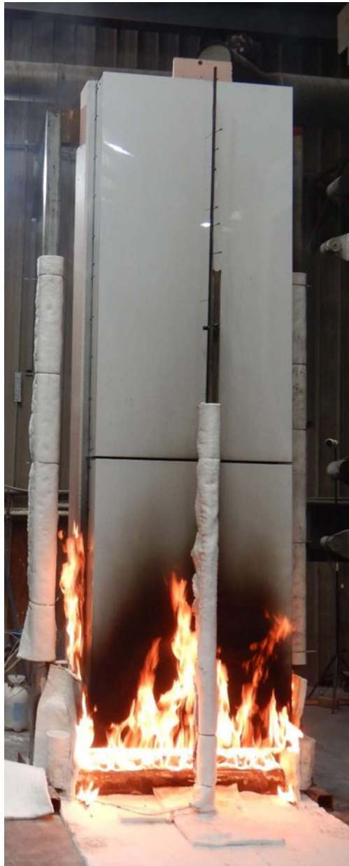
Figure 14 The specimen 4 minutes 53 seconds into the test (burner output at 100 kW)
