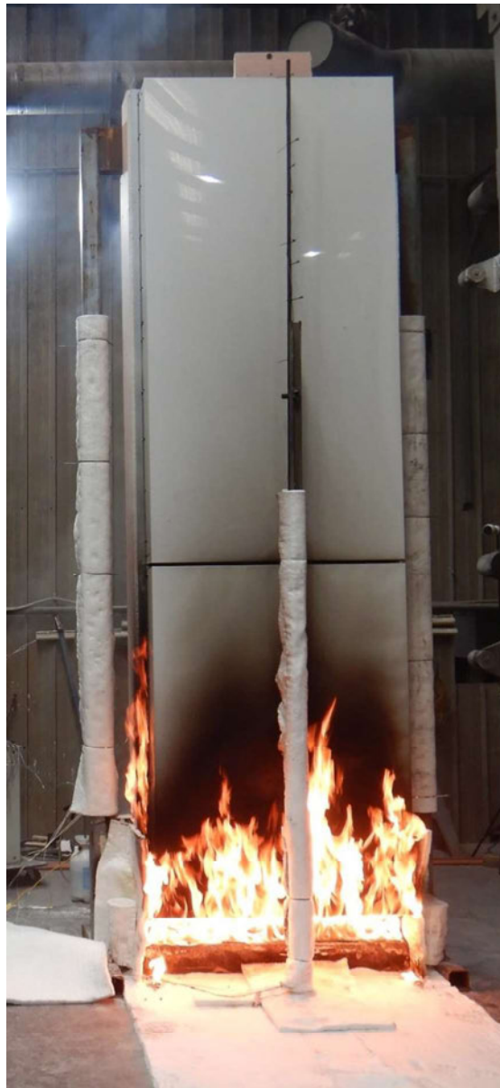
Figure 15 The specimen 9 minutes 53 seconds into the test (burner output at 100 kW)
