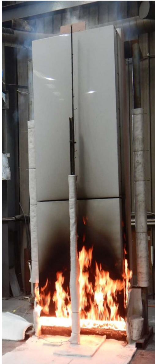
Figure 16 The specimen 13 minutes 14 seconds into the test (burner output at 100 kW)
