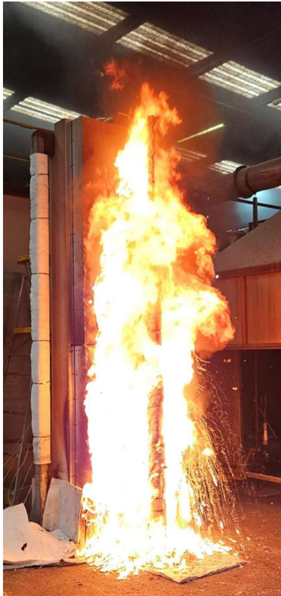
Figure 20 The specimen 6 minutes 37 seconds into the test (burner output at 200 kW)
