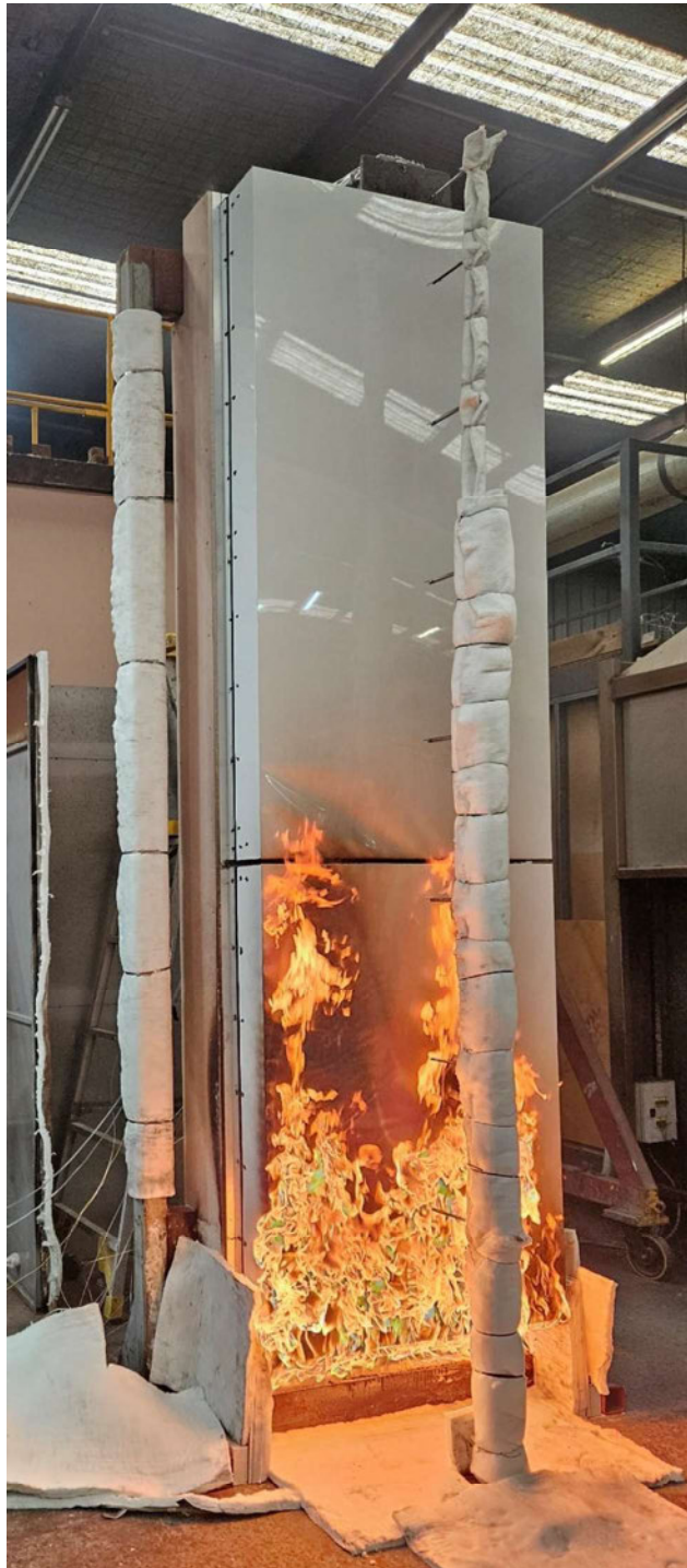
Figure 16 The specimen 5 minutes into the test (burner output at 200 kW)
