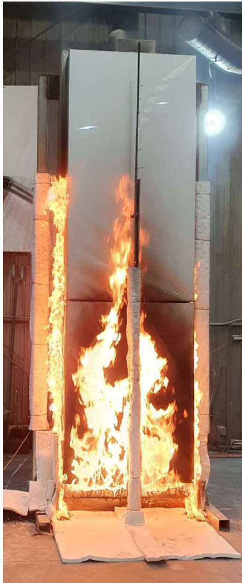
Figure 14 The specimen 9 minutes 20 seconds into the test (burner output at 200 kW)
