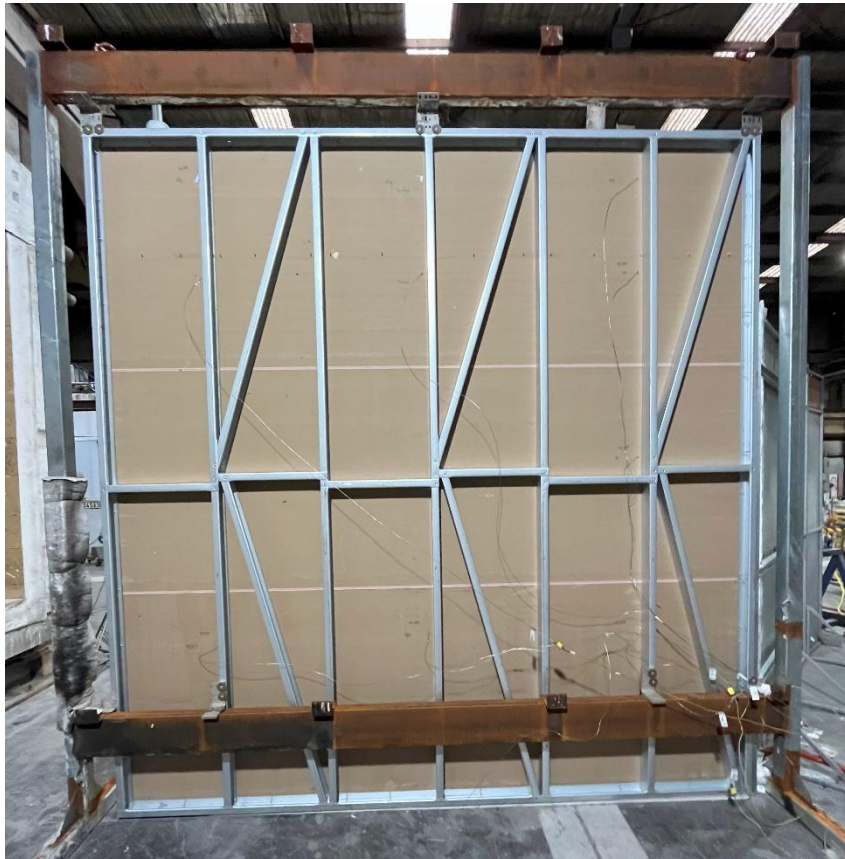
Figure 20 The specimen before the reaction to fire test - unexposed side
