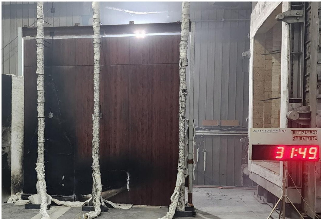
Figure 28 The specimen 31 minutes 49 seconds into the test (1 minutes 49 seconds after burner off)
