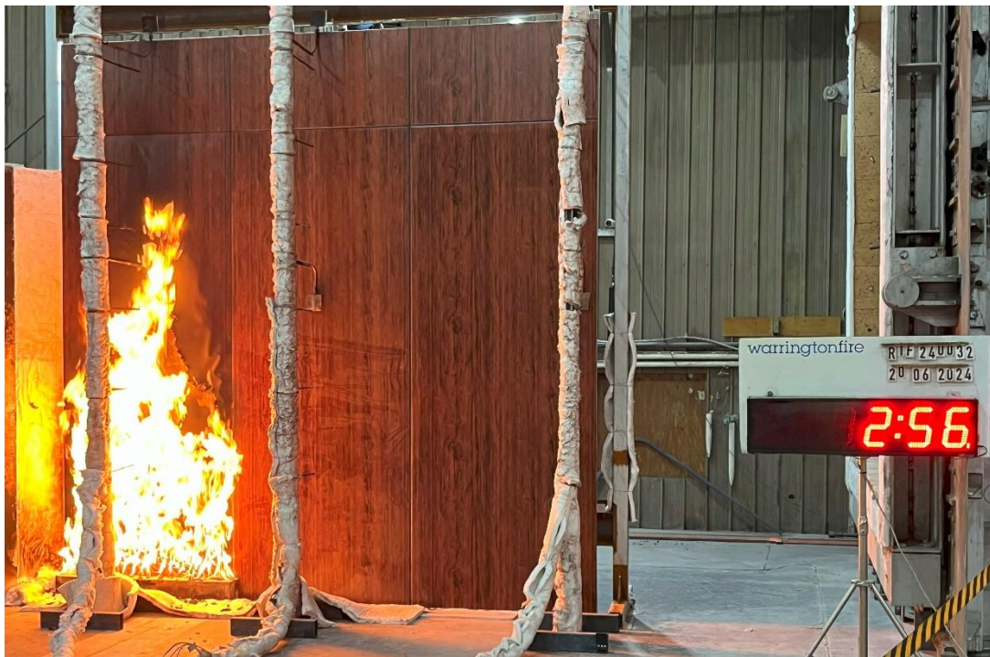
Figure 21 The specimen 2 minutes 56 seconds into the test (burner output at 300 kW)
