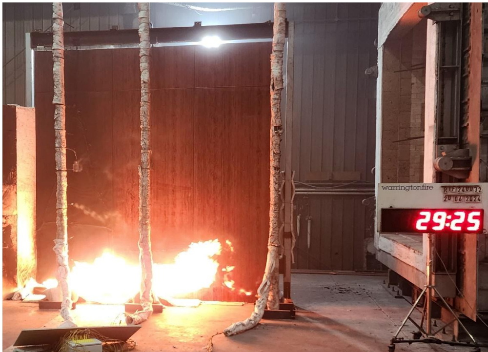
Figure 26 The specimen 29 minutes 25 seconds into the test (burner output at 300 kW)
