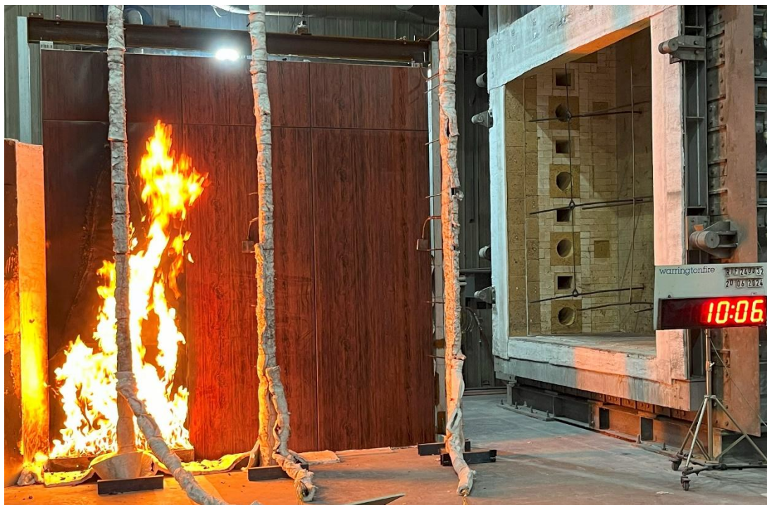
Figure 23 The specimen 10 minutes 6 seconds in the test (burner output at 300 kW)
