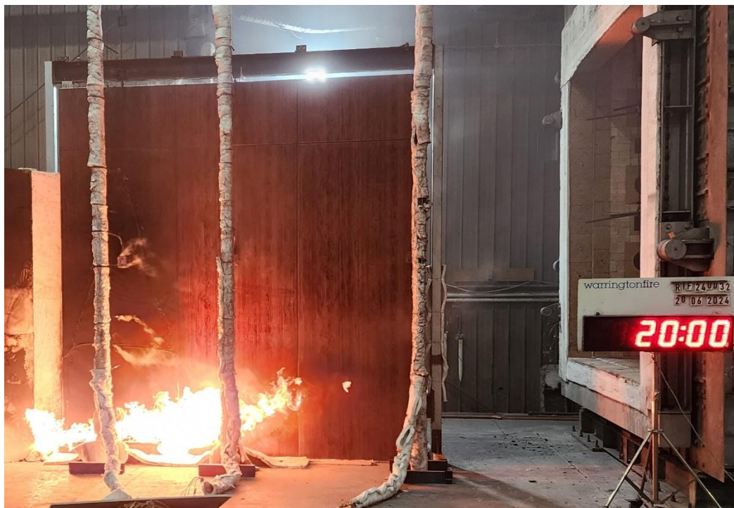
Figure 25 The specimen 20 minutes into the test (burner output at 300 kW)
