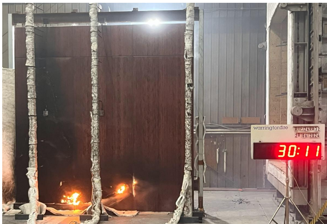
Figure 27 The specimen 30 minutes 11 seconds into the test (11 seconds after burner off)
