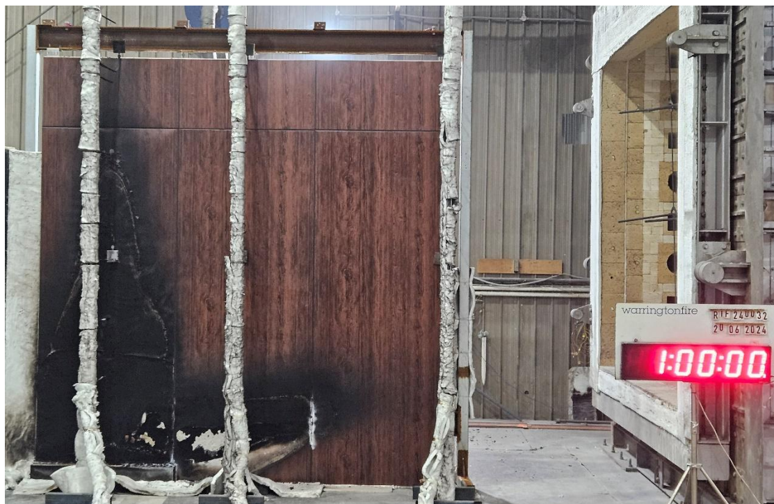
Figure 29 The specimen 60 minutes into the test (30 minutes after burner off)
