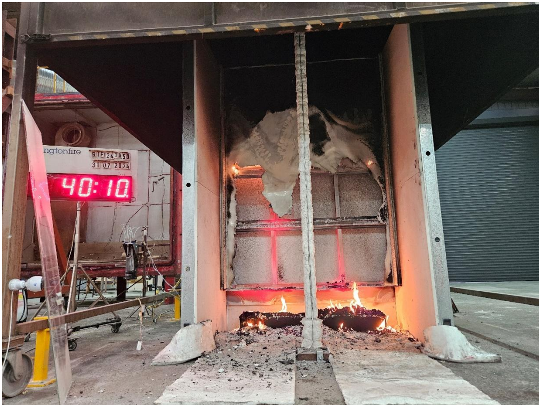
Figure 26 The specimen 40 minutes 10 seconds into the test (burner off)
