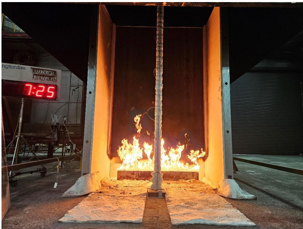
Figure 18 The specimen 7 minutes 25 seconds into the test (burner output at 100 kW)
