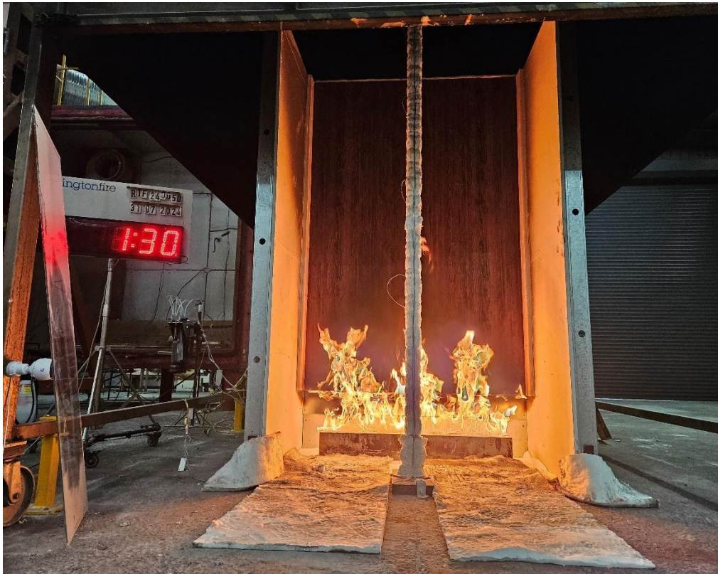
Figure 17 The specimen 1 minutes 30 seconds into the test (burner output at 100 kW)
