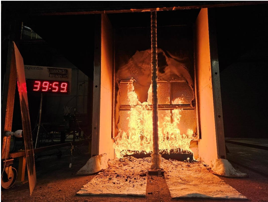
Figure 25 The specimen 39 minutes 59 seconds into the test (burner output at 300 kW)
