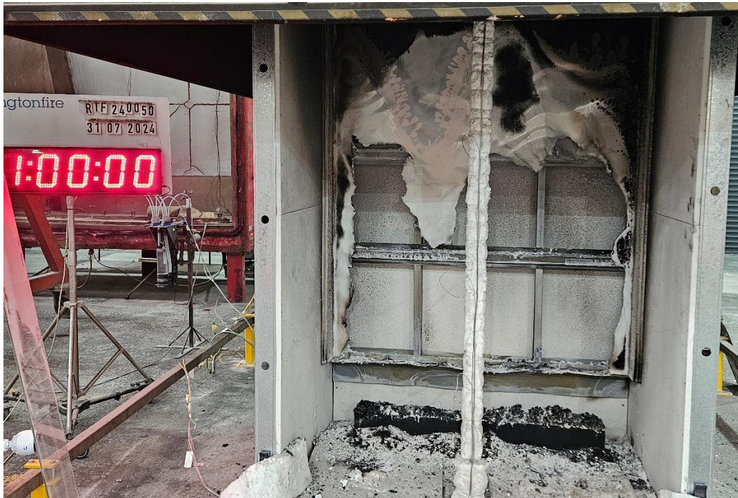
Figure 27 The specimen at end of test – exposed side
