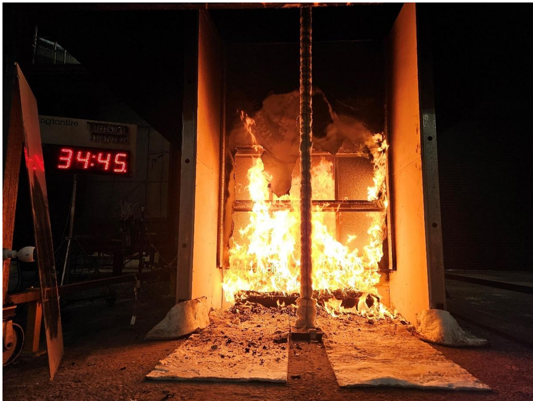
Figure 24 The specimen 34 minutes 45 seconds into the test (burner output at 300 kW)
