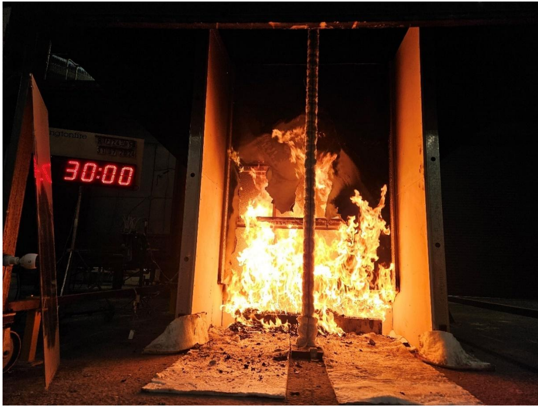
Figure 23 The specimen 30 minutes into the test (burner output at 300 kW)
