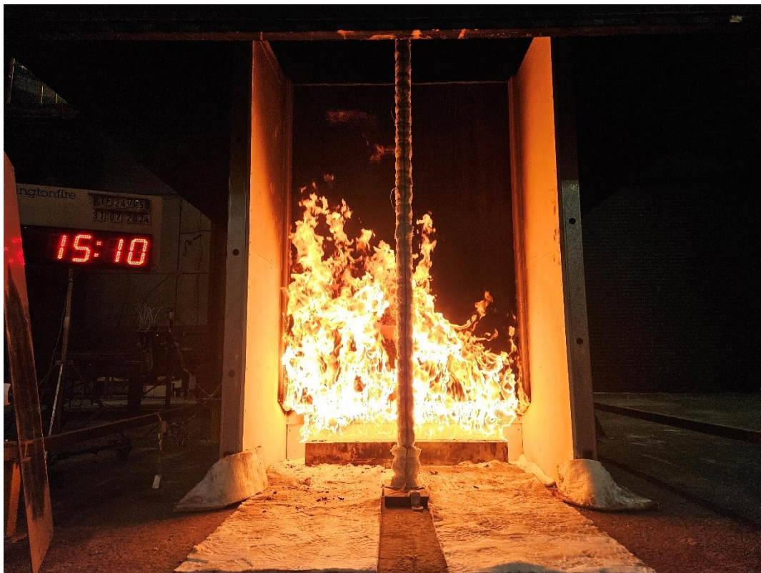
Figure 20 The specimen 15 minutes 10 seconds into the test (burner output at 300 kW)
