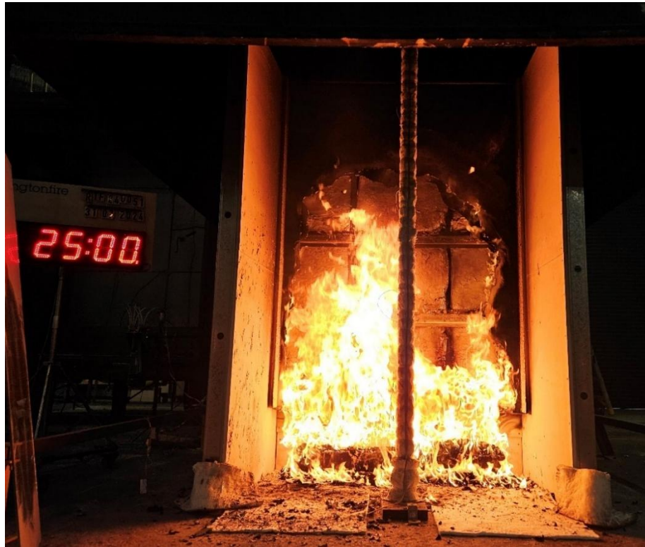
Figure 24 The specimen 25 minutes into the test (burner output at 300 kW)
