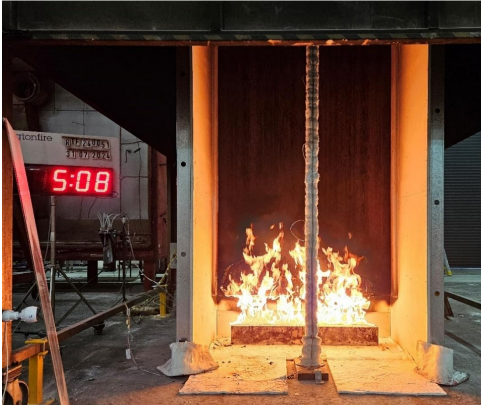
Figure 19 The specimen 5 minutes 08 seconds into the test (burner output at 100 kW)
