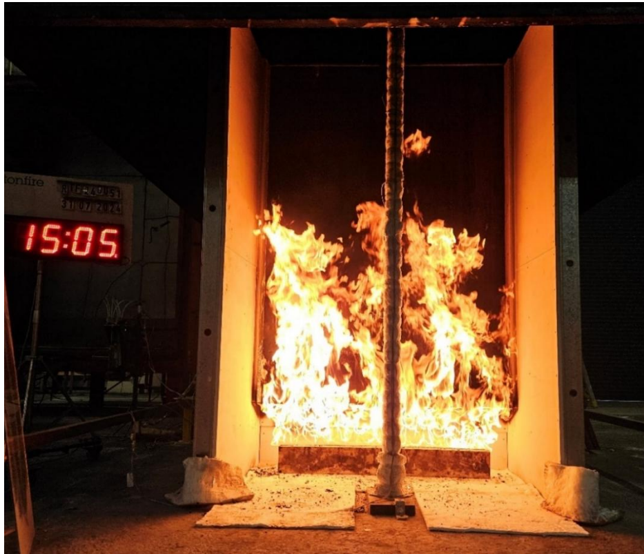
Figure 22 The specimen 15 minutes 05 seconds into the test (burner output at 300 kW)
