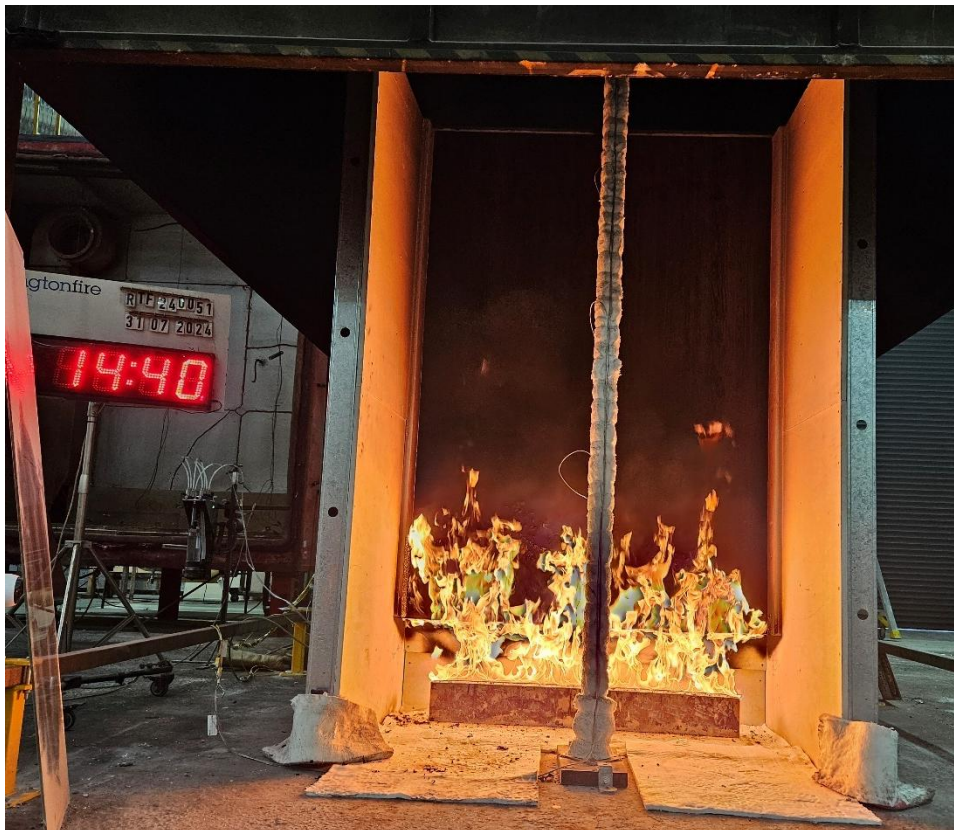
Figure 21 The specimen 14 minutes 40 seconds into the test (burner output at 100 kW)
