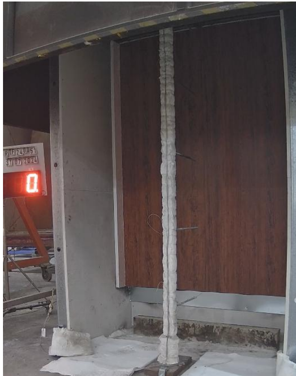
Figure 16 The specimen before the reaction to fire test – exposed side
