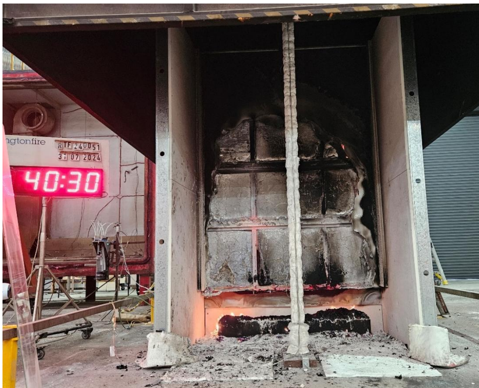
Figure 27 The specimen 40 minutes 30 seconds into the test (burner off)
