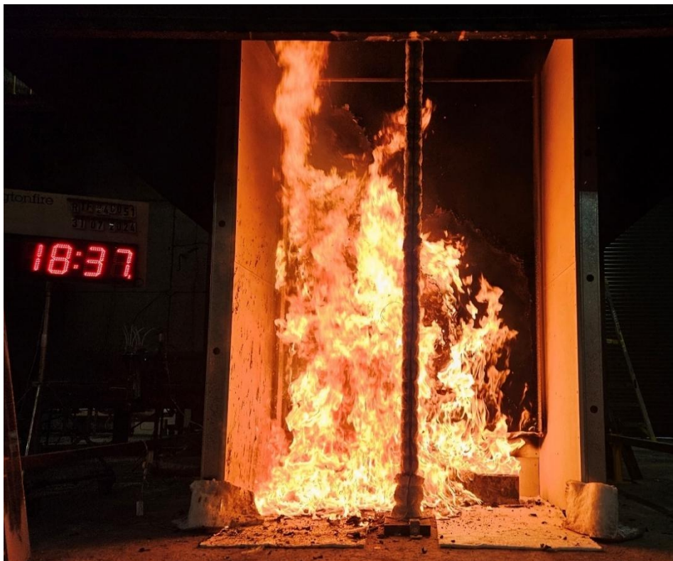
Figure 23 The specimen 18 minutes 37 seconds into the test (burner output at 300 kW)
