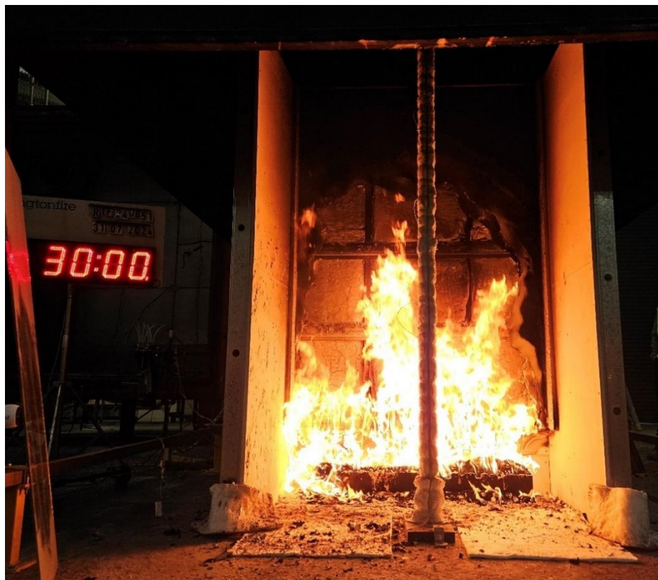
Figure 25 The specimen 30 minutes into the test (burner output at 300 kW)
