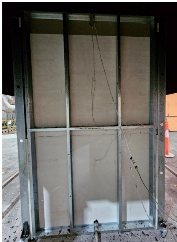
Figure 29 The specimen at end of test – unexposed side
