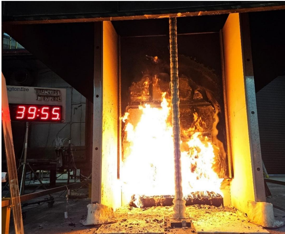
Figure 26 The specimen 39 minutes 55 seconds into the test (burner output at 300 kW)
