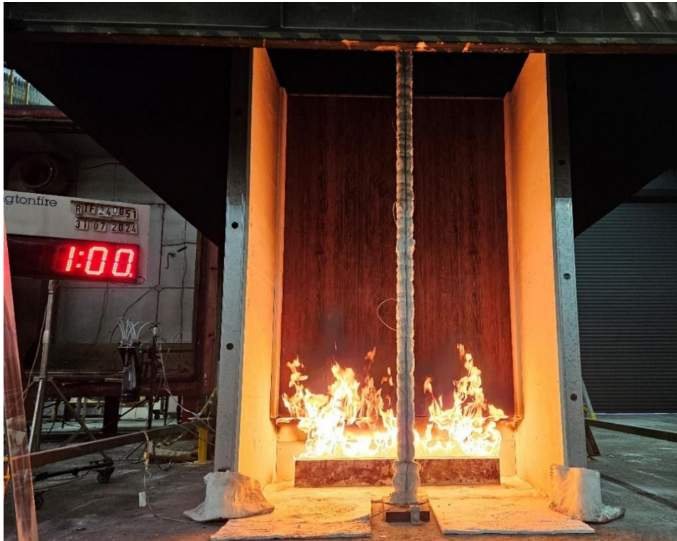
Figure 18 The specimen 1 minute into the test (burner output at 100 kW)
