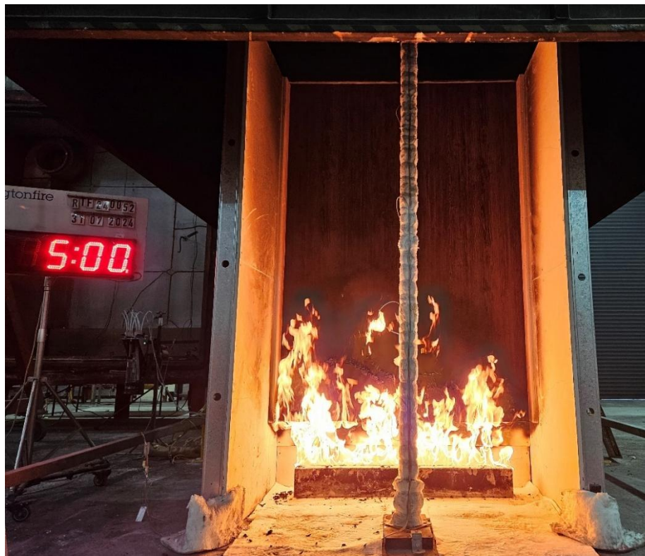
Figure 19 The specimen 5 minutes into the test (burner output at 100 kW)
