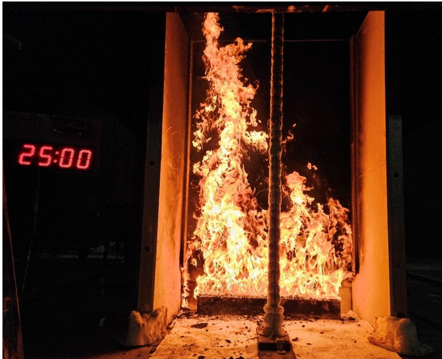
Figure 24 The specimen 25 minutes into the test (burner output at 300 kW)
