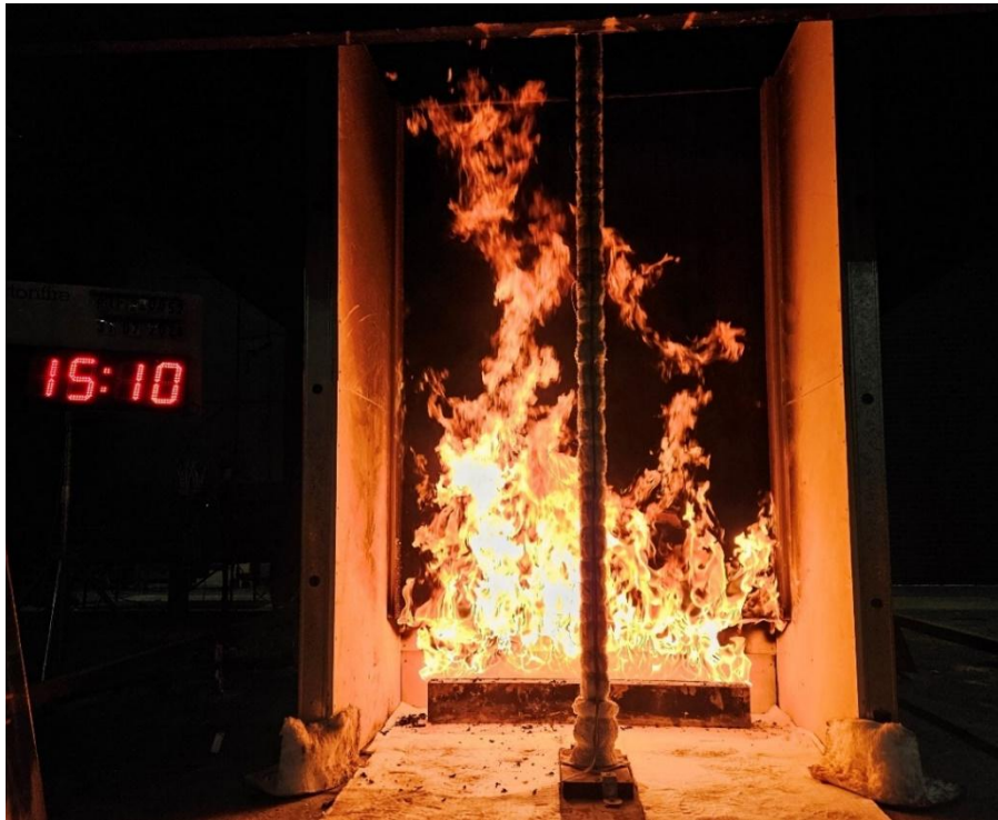
Figure 22 The specimen 15 minutes 10 seconds into the test (burner output at 300 kW)
