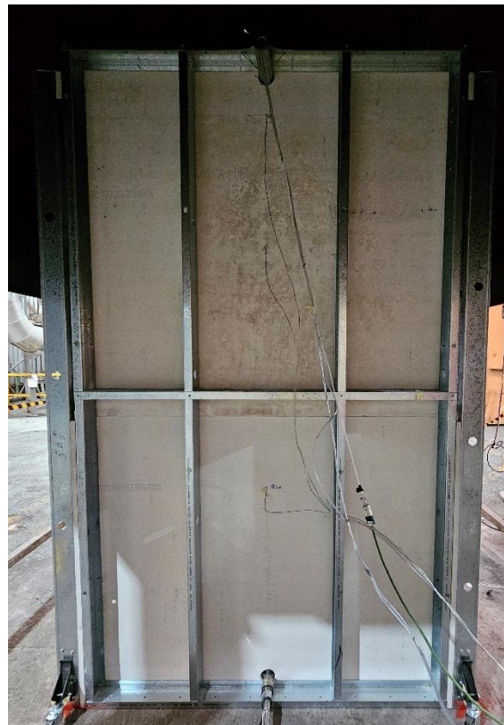
Figure 29 The specimen at end of test – unexposed side
