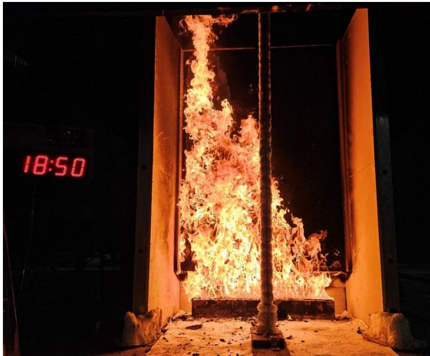
Figure 23 The specimen 18 minutes 50 seconds into the test (burner output at 300 kW)
