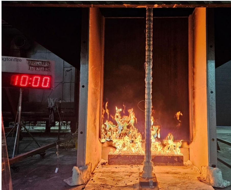
Figure 20 The specimen 10 minutes into the test (burner output at 100 kW)
