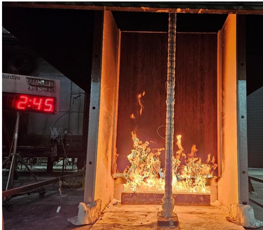
Figure 18 The specimen 2 minutes 45 seconds into the test (burner output at 100 kW)
