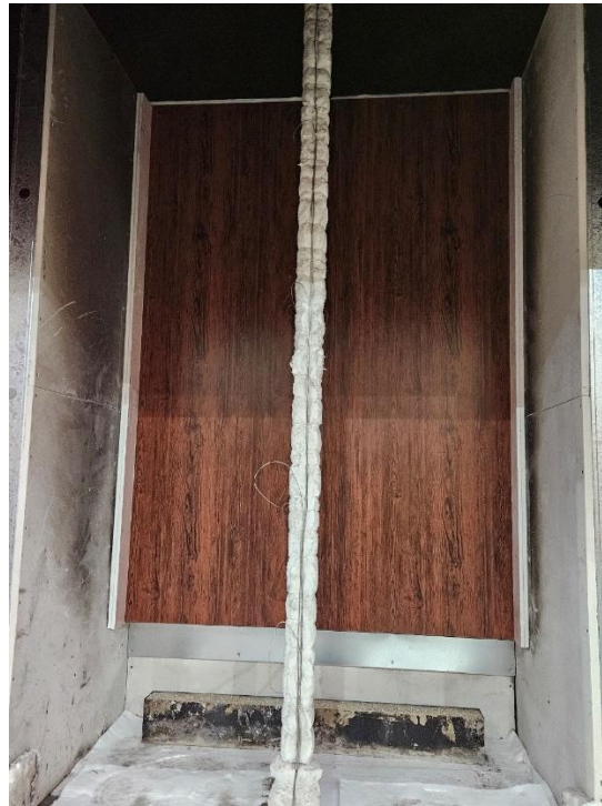
Figure 16 The specimen before the reaction to fire test – exposed side
