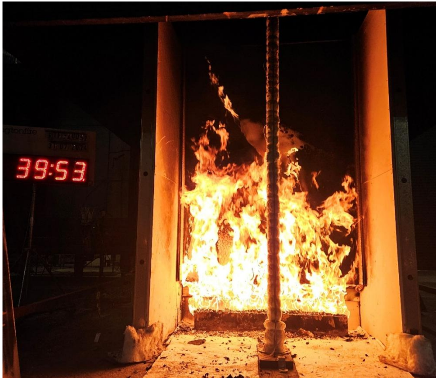
Figure 26 The specimen 39 minutes 53 seconds into the test (burner output at 300 kW)
