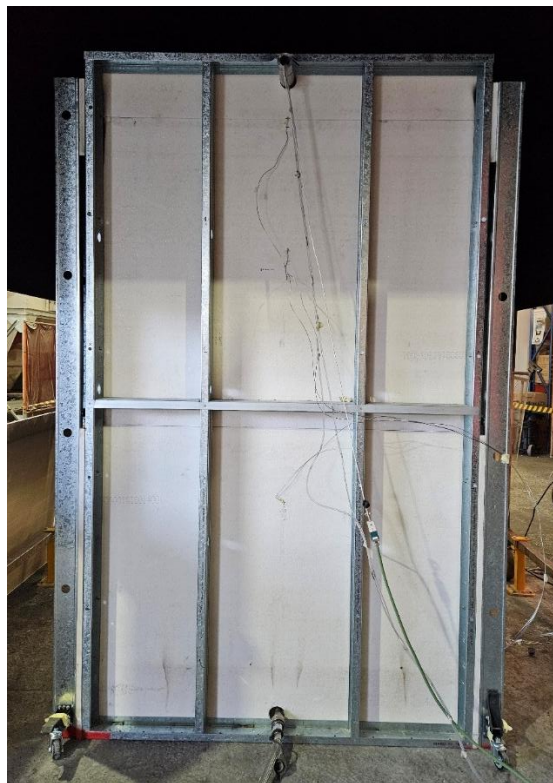
Figure 17 The specimen (unexposed side) before the reaction to fire test
