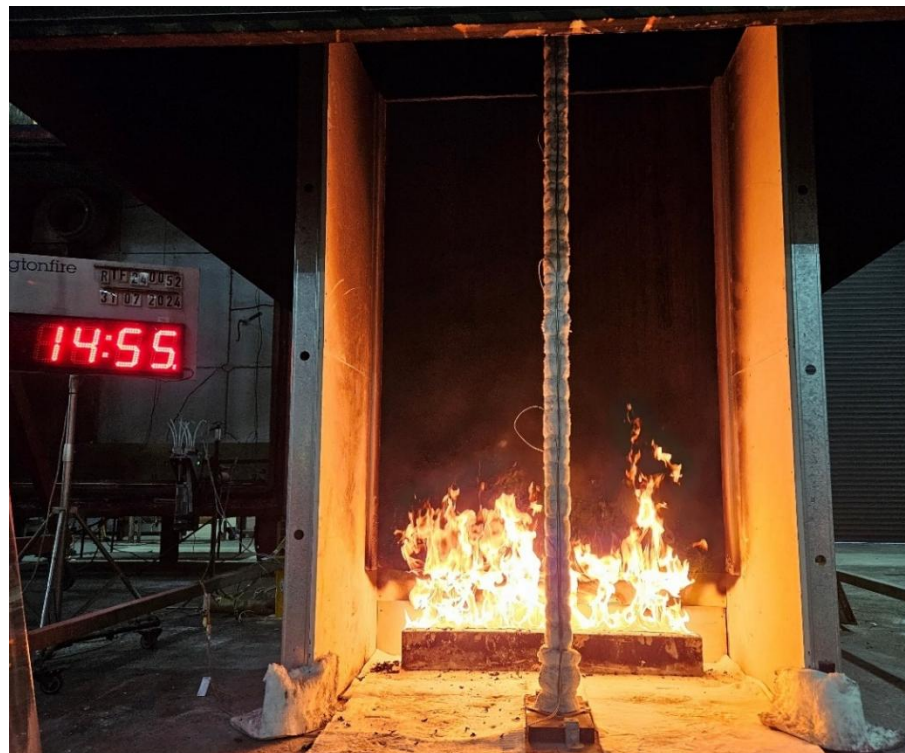
Figure 21 The specimen 14 minutes 55 seconds into the test (burner output at 100 kW)
