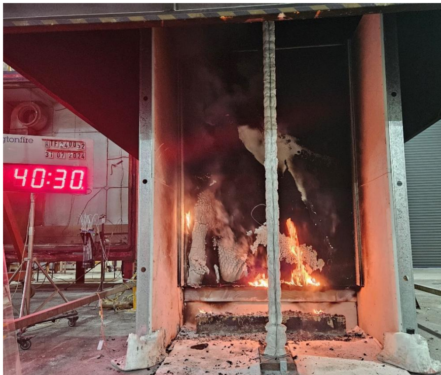
Figure 27 The specimen 40 minutes 30 seconds into the test (burner off)
