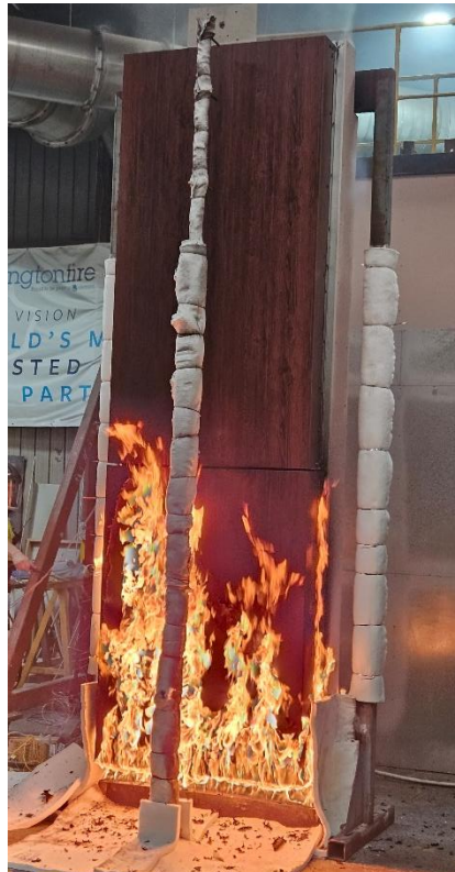
Figure 17 The specimen 18 minutes 44 seconds into the test (3 minutes 44 seconds after burner output was changed to 300 kW)
