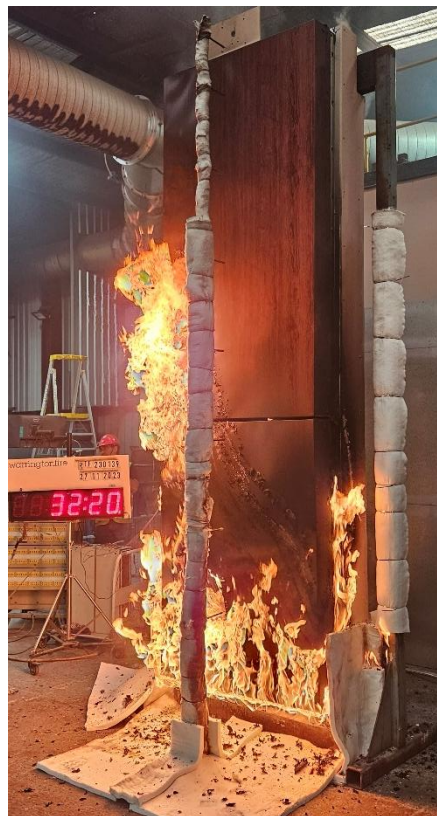
Figure 19 The specimen 32 minutes 20 seconds into the test (17 minutes 20 seconds after burner output was changed to 300 kW)
