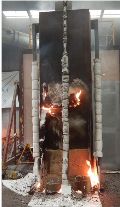
Figure 24 The specimen 47 minutes 58 seconds into the test (3 minutes 58 seconds after burner was switched off)
