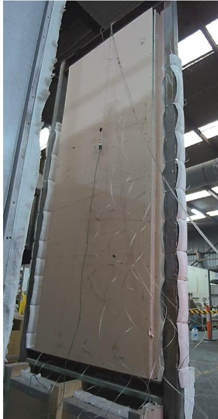
Figure 12 The specimen before the reaction to fire test – unexposed side
