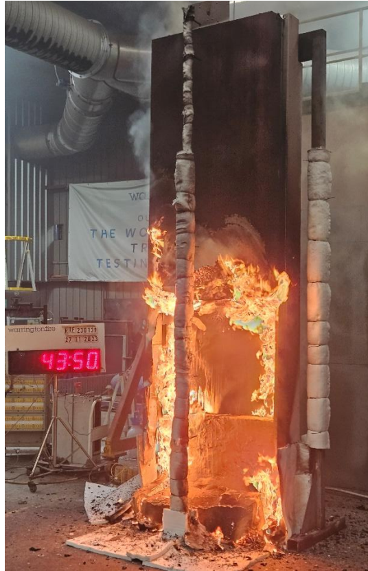
Figure 22 The specimen 43 minutes 50 seconds into the test (28 minutes 50 seconds after burner output was changed to 300 kW)
