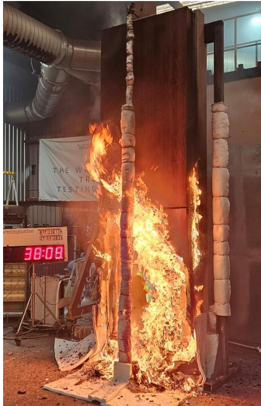
Figure 21 The specimen 38 minutes 9 seconds into the test (23 minutes 9 seconds after burner output was changed to 300 kW)
