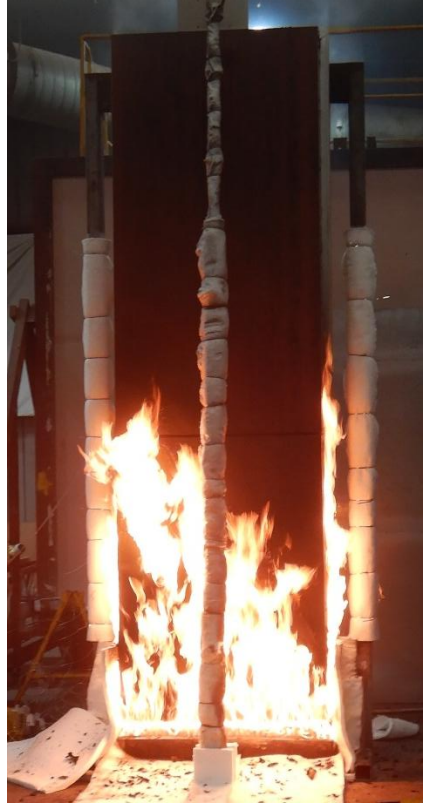
Figure 18 The specimen 21 minutes 40 seconds into the test (6 minutes 40 seconds after burner output was changed to 300 kW)
