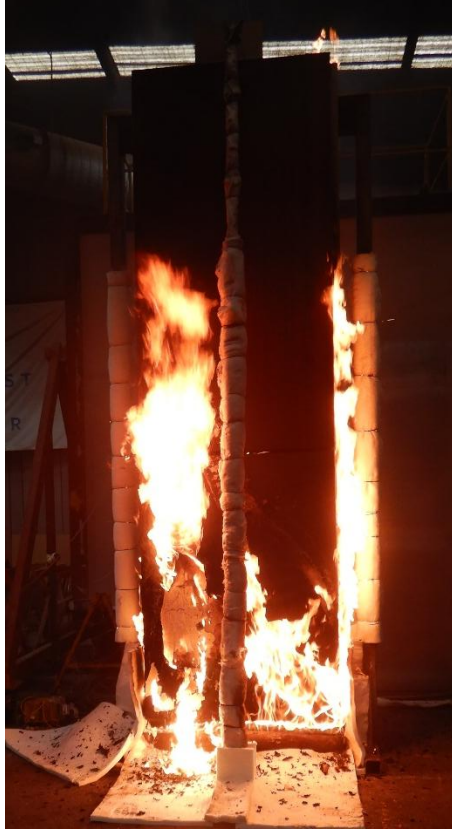
Figure 20 The specimen 36 minutes 37 seconds into the test (21 minutes 37 seconds after burner output was changed to 300 kW)
