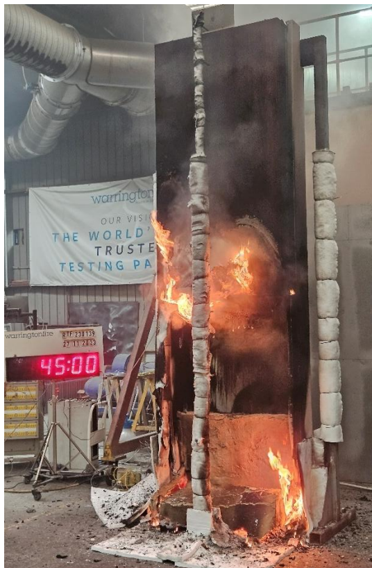
Figure 23 The specimen 45 minutes into the test (1 minute after burner was switched off)
