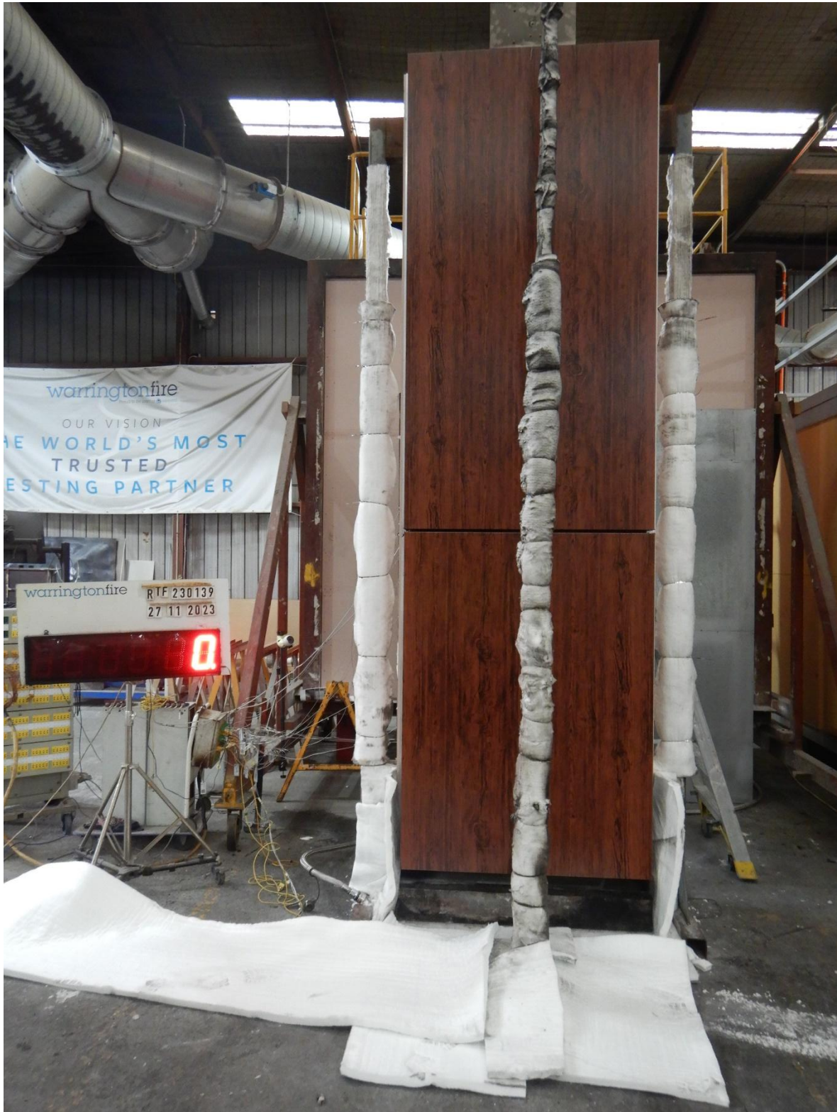
Figure 11 The specimen before the reaction to fire test
