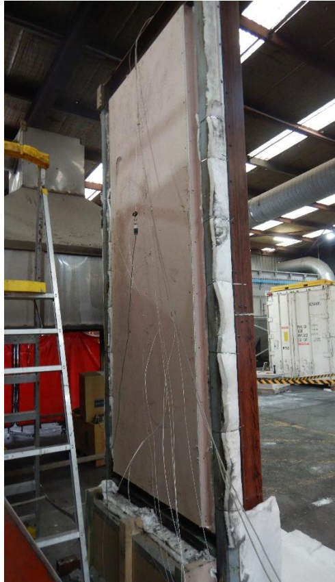
Figure 12 The specimen before the reaction to fire test – unexposed side
