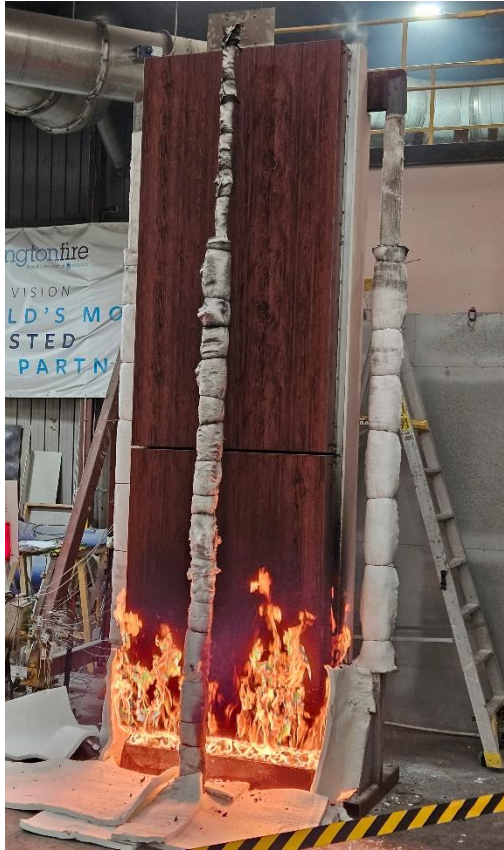
Figure 14 The specimen 8 minutes 35 seconds into the test (burner output at 100 kW)
