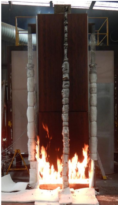
Figure 15 The specimen 14 minutes 55 seconds into the test (burner output at 100 kW)
