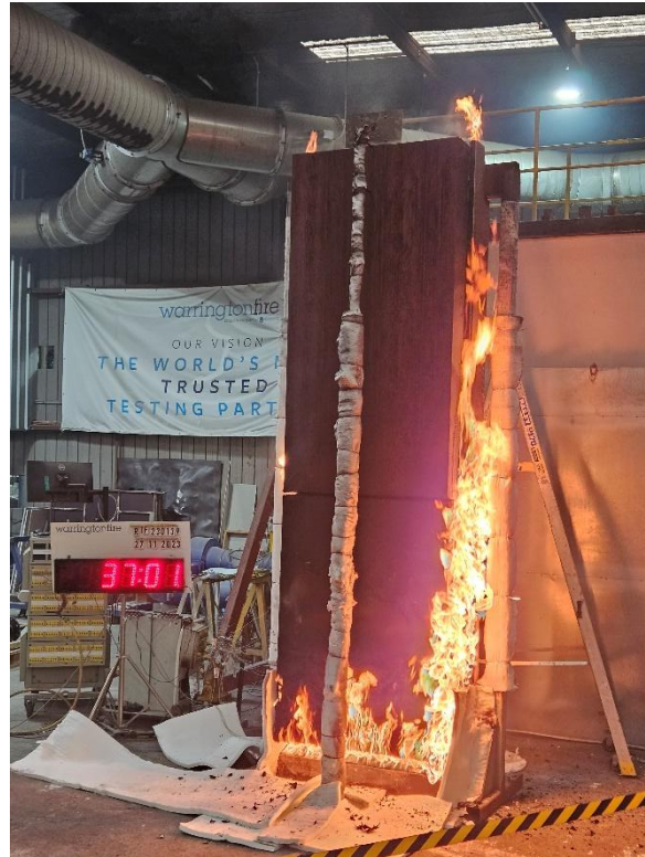
Figure 20 The specimen 37 minutes 1 second into the test (22 minutes 1 second after burner output was changed to 300 kW)
