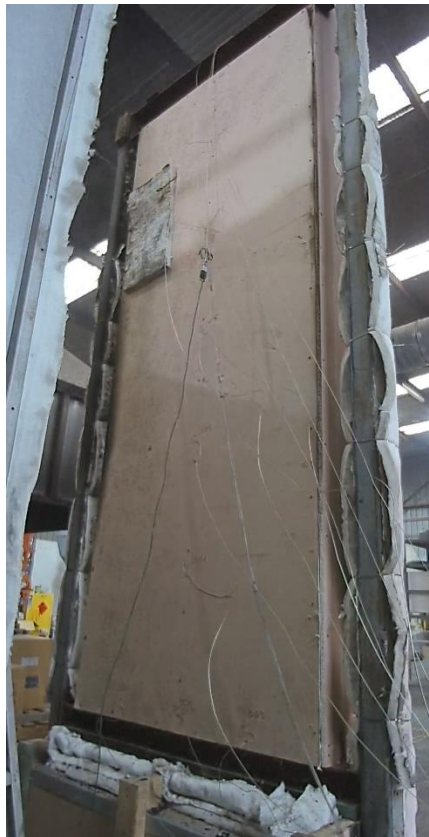
Figure 25 The specimen after the test – unexposed side
