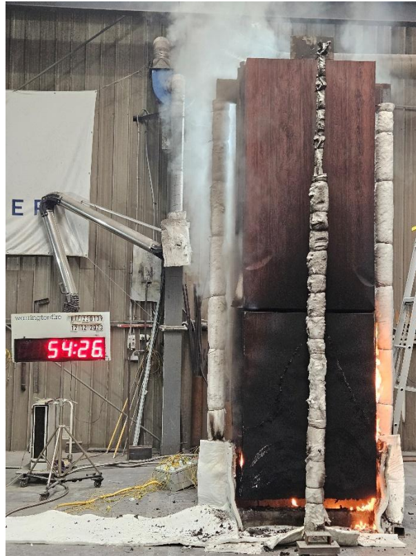
Figure 24 The specimen 54 minutes 26 seconds into the test (14 minutes 26 seconds after burner was switched off)
