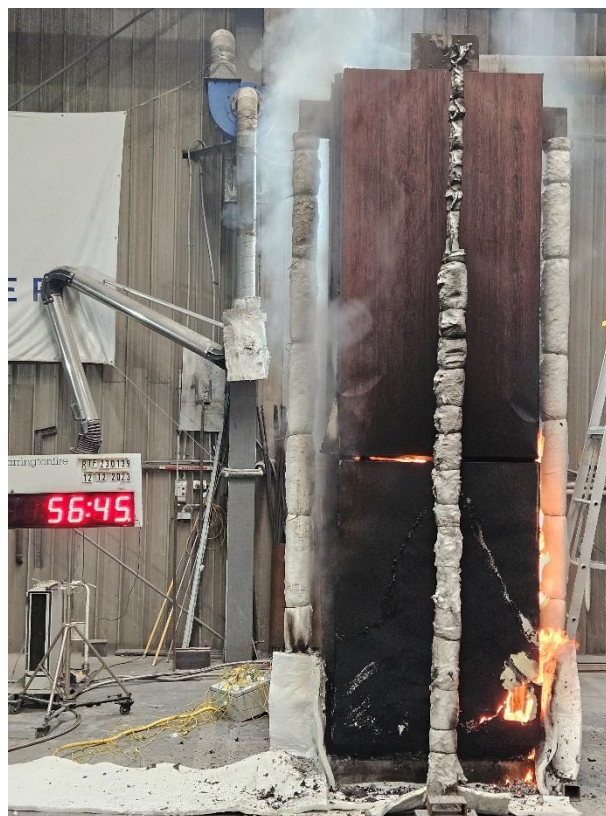
Figure 25 The specimen 56 minutes 45 seconds into the test (16 minutes 45 seconds after burner was switched off)
