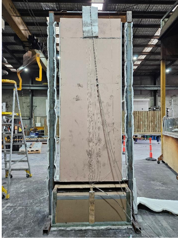
Figure 12 The specimen before the reaction to fire test – unexposed side
