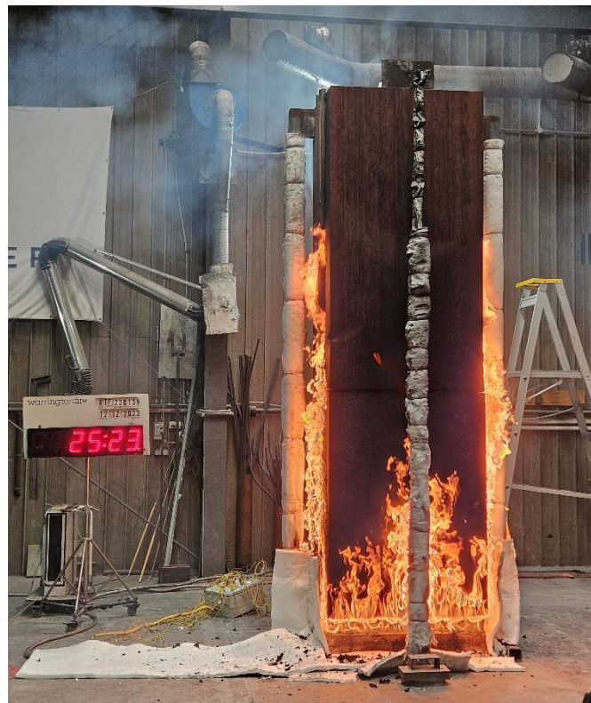
Figure 19 The specimen 25 minutes 23 seconds into the test (10 minutes 23 seconds after burner output was changed to 300 kW)
