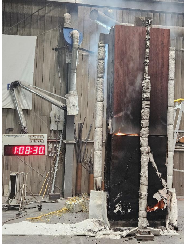
Figure 26 The specimen 68 minutes 30 seconds into the test (28 minutes 30 seconds after burner was switched off)
