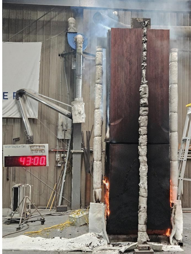
Figure 23 The specimen 43 minutes into the test (3 minute after burner was switched off)
