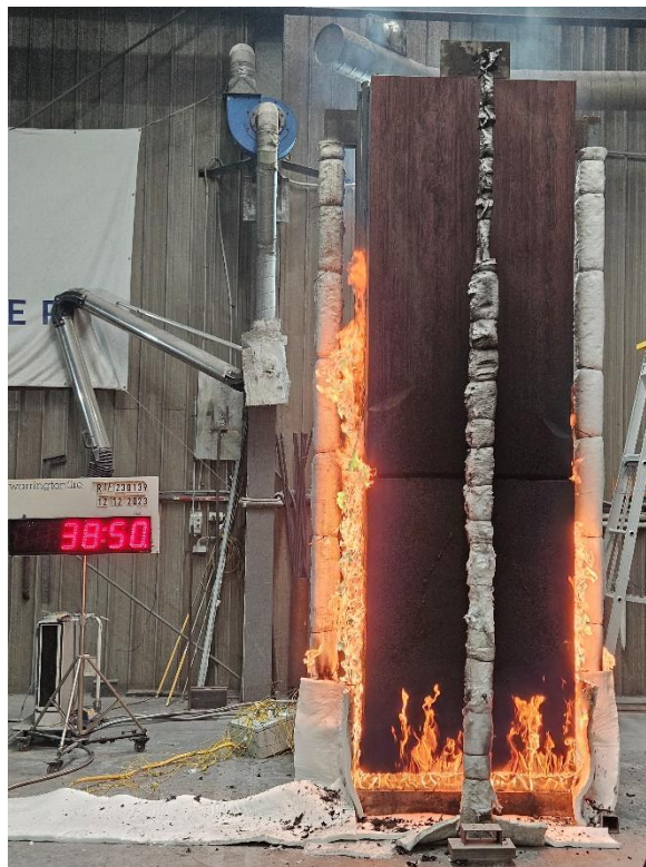
Figure 21 The specimen 38 minutes 50 seconds into the test (23 minutes 50 seconds after burner output was changed to 300 kW)
