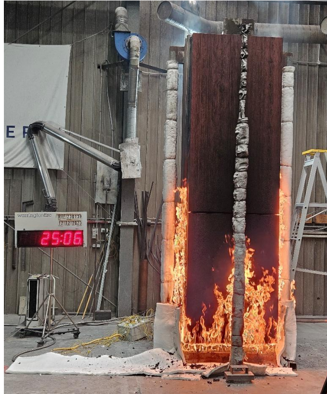
Figure 18 The specimen 25 minutes 6 seconds into the test (10 minutes 6 seconds after burner output was changed to 300 kW)
