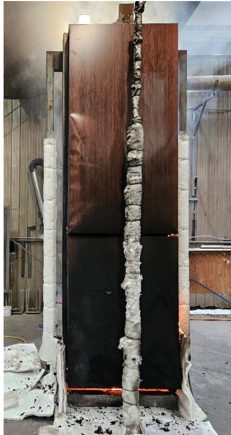
Figure 21 The specimen 41 minutes 50 seconds into the test (1 minute 50 seconds after burner was switched off)
