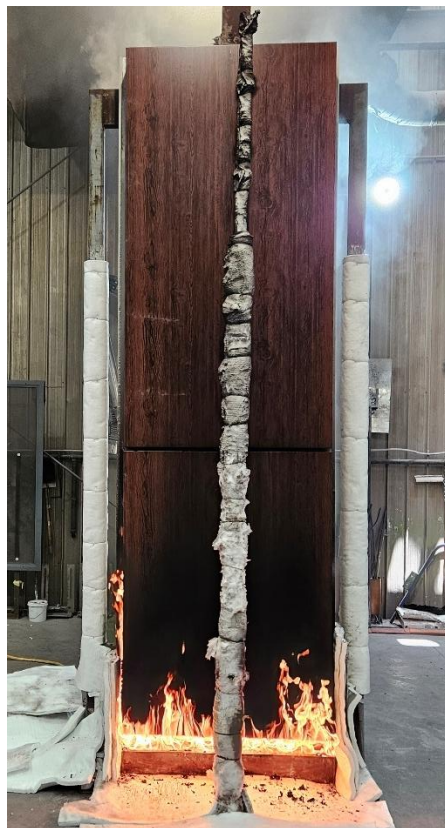
Figure 16 The specimen 14 minutes 59 seconds into the test (burner output at 100 kW)
