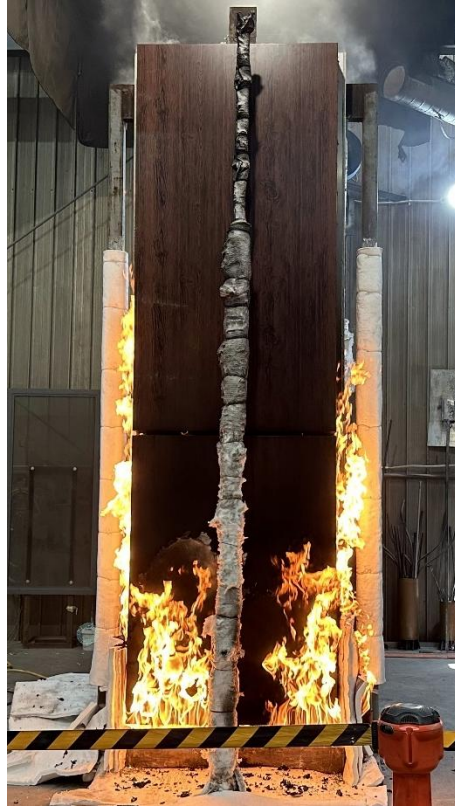
Figure 18 The specimen 20 minutes into the test (5 minutes after burner output was changed to 300 kW)
