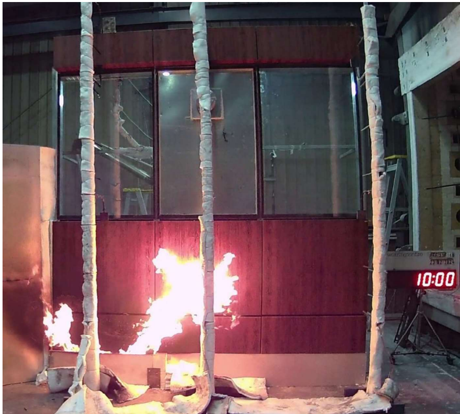
Figure 28 The specimen 10 minutes into the test (burner output at 300 kW and wind on)
