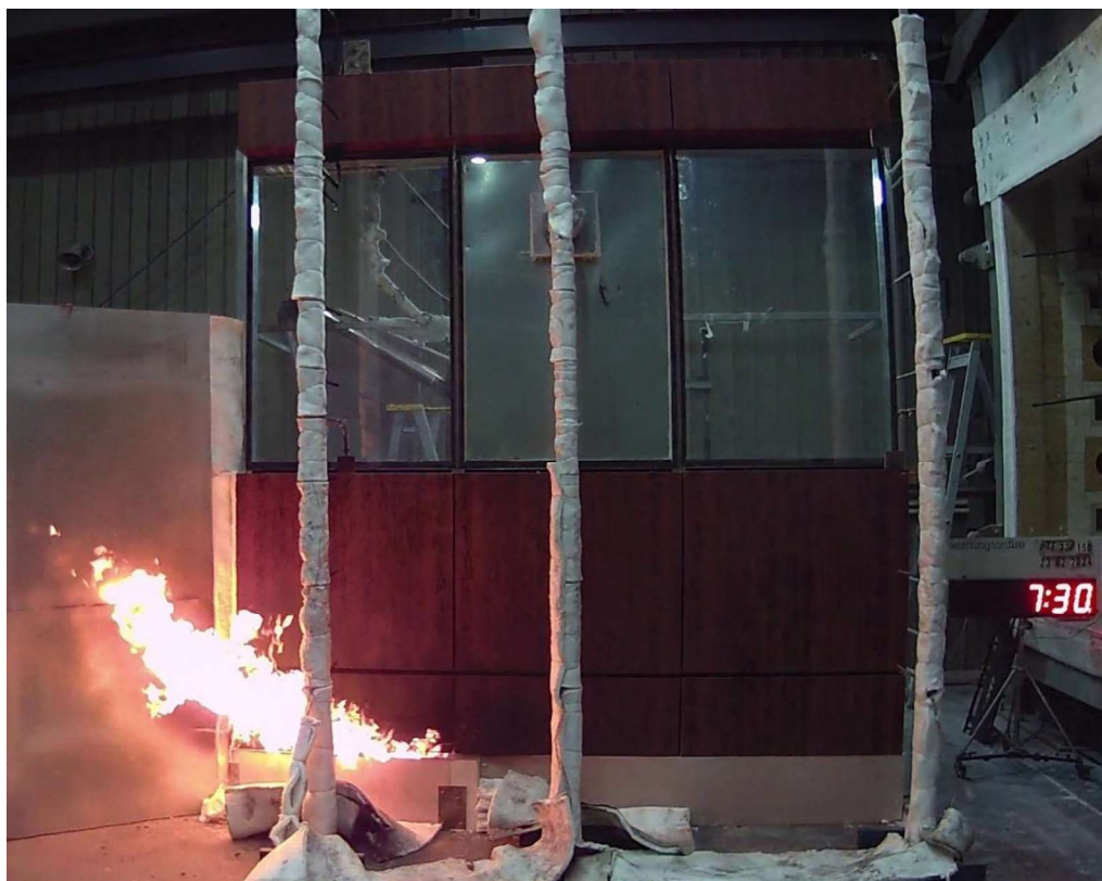
Figure 27 The specimen 7 minutes 30 seconds into the test (burner output at 300 kW and wind on)
