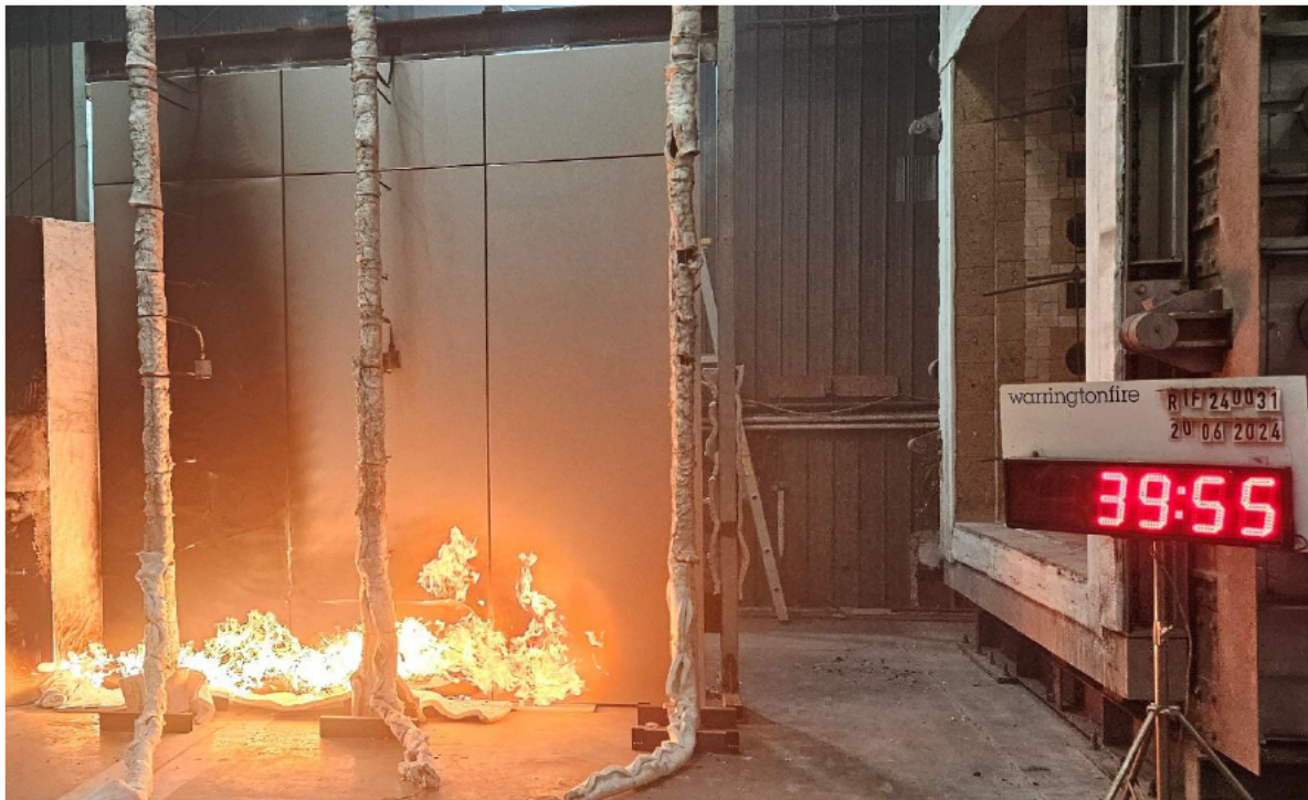
Figure 25 The specimen 39 minutes 55 seconds into the test (burner output at 300 kW)
