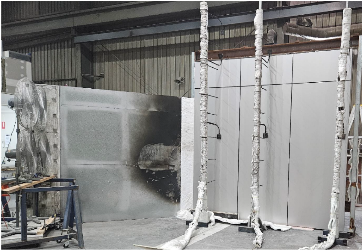
Figure 16 The specimen and test setup (angled – exposed side) before the reaction to fire test
