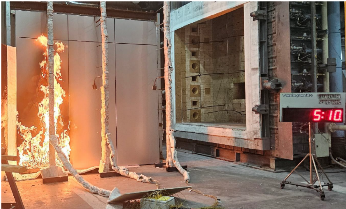
Figure 19 The specimen 5 minutes 10 seconds into the test (burner output at 300 kW)
