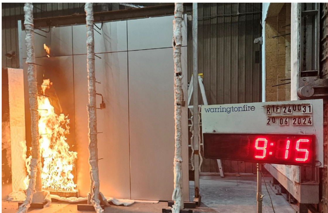
Figure 20 The specimen 9 minutes 15 seconds into the test (burner output at 300 kW)
