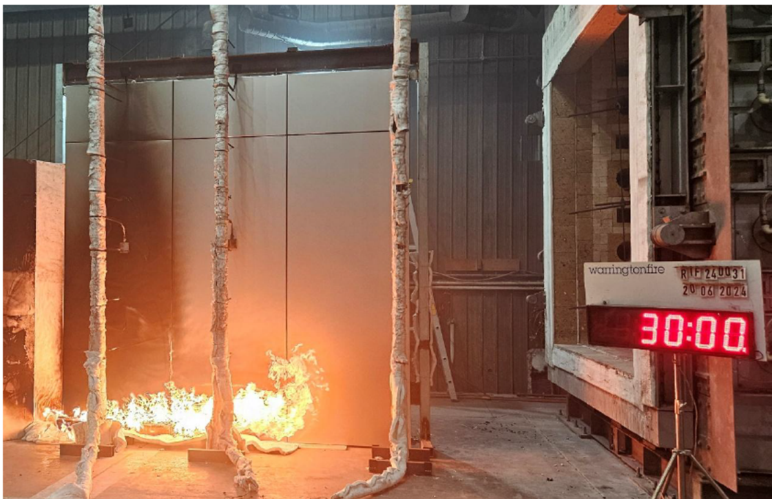
Figure 24 The specimen 30 minutes into the test (burner output at 300 kW)
