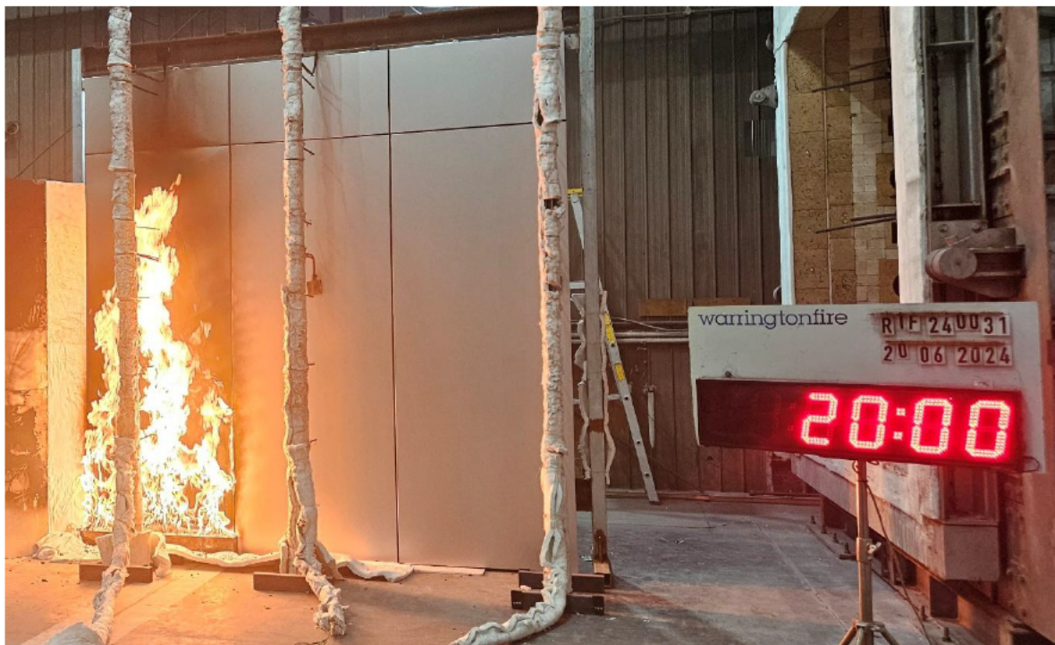
Figure 22 The specimen 20 minutes into the test (burner output at 300 kW)
