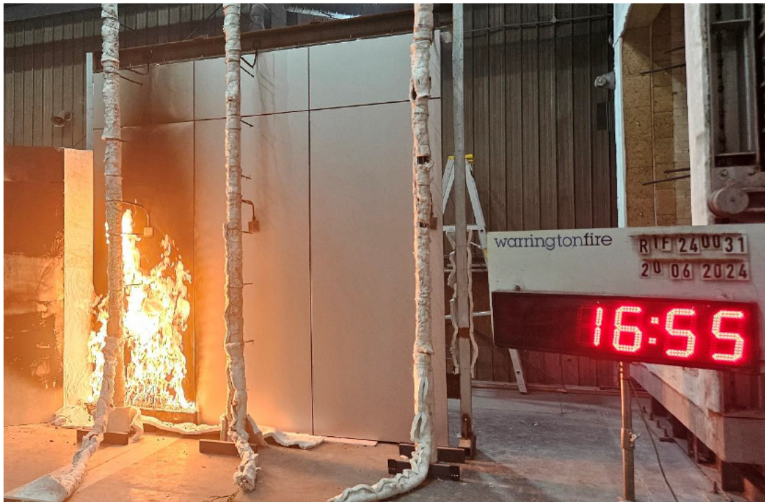
Figure 21 The specimen 16 minutes 55 seconds into the test (burner output at 300 kW)
