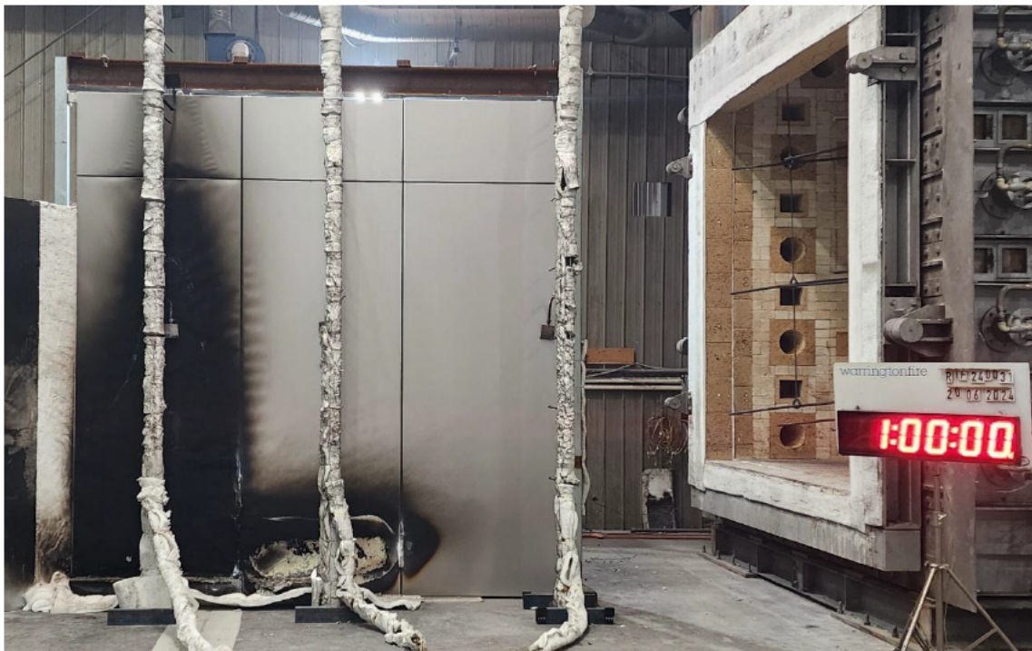
Figure 28 The specimen 60 minutes into the test (20 minutes after burner off)
