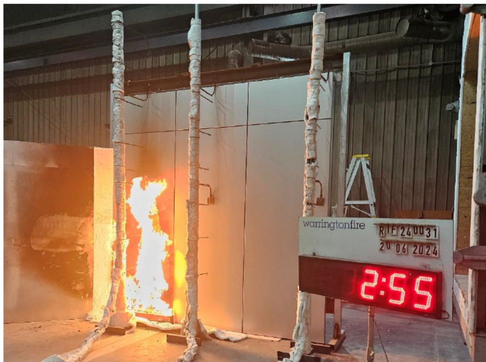
Figure 18 The specimen 2 minutes 55 seconds into the test (burner output at 300 kW)
