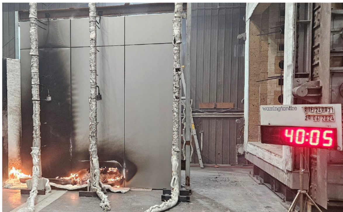
Figure 26 The specimen 40 minutes 5 seconds into the test (5 seconds after burner off)
