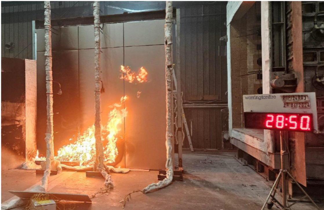
Figure 23 The specimen 28 minutes 50 seconds into the test (burner output at 300 kW)
