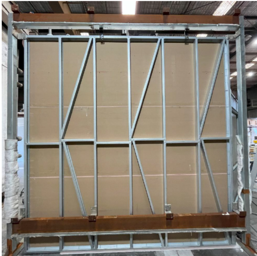
Figure 17 The specimen before the reaction to fire test - unexposed side
