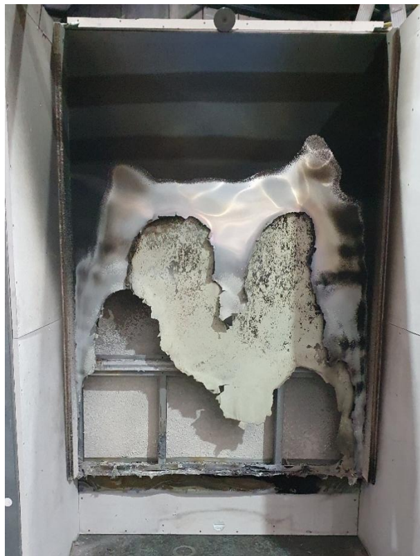
Figure 27 The specimen after the reaction to fire test – exposed side
