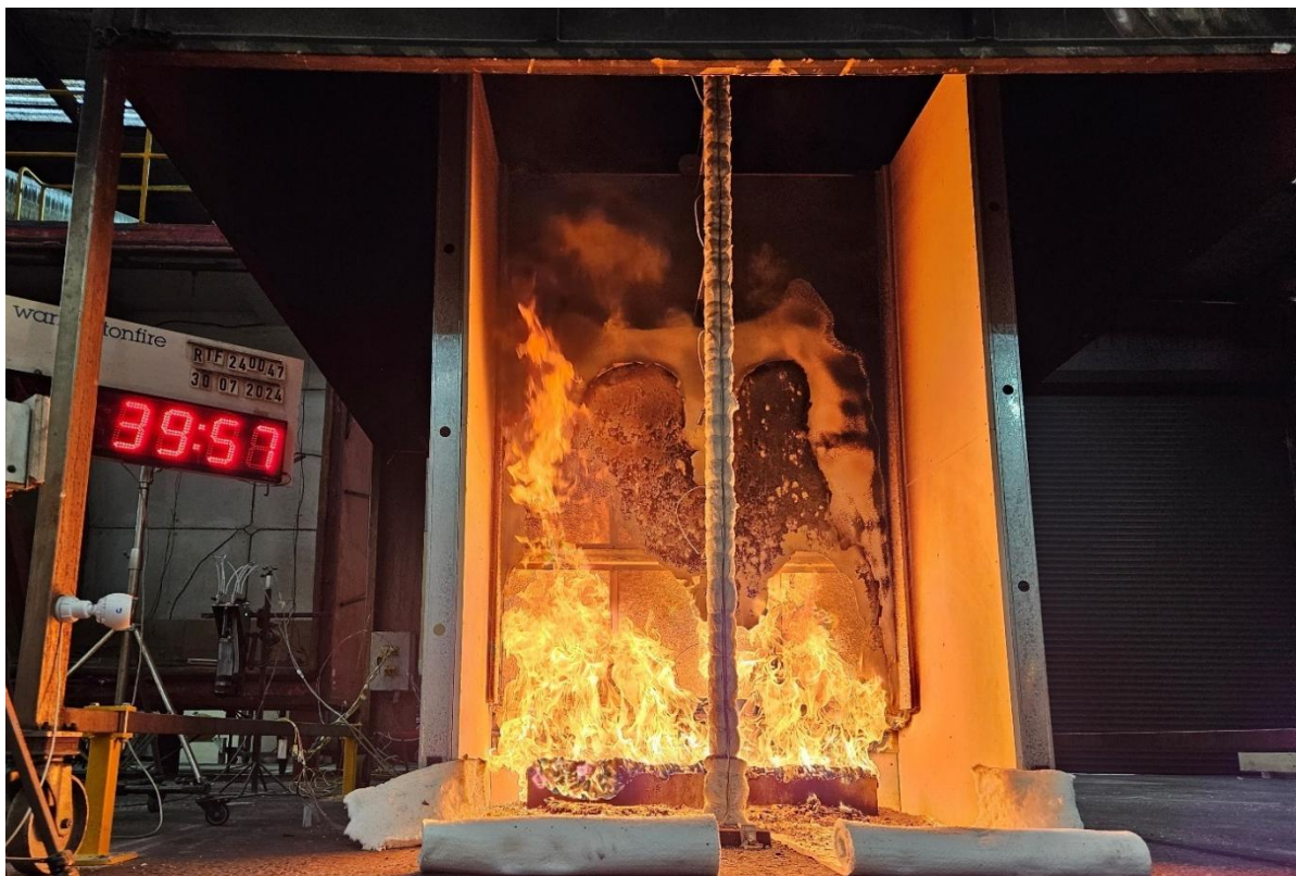
Figure 25 The specimen 39 minutes 57 seconds into the test (burner output at 300 kW)
