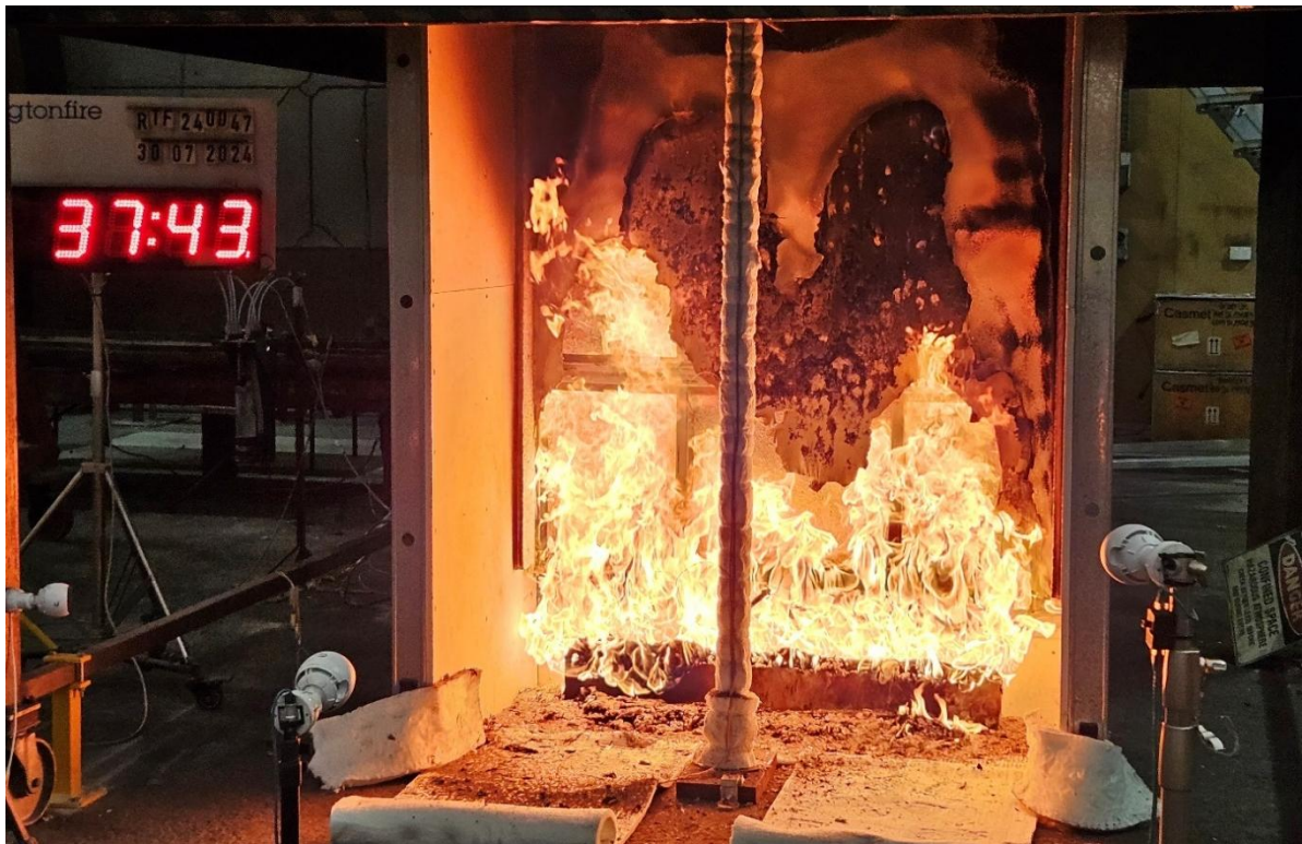
Figure 24 The specimen 37 minutes 43 seconds into the test (burner output at 300 kW)
