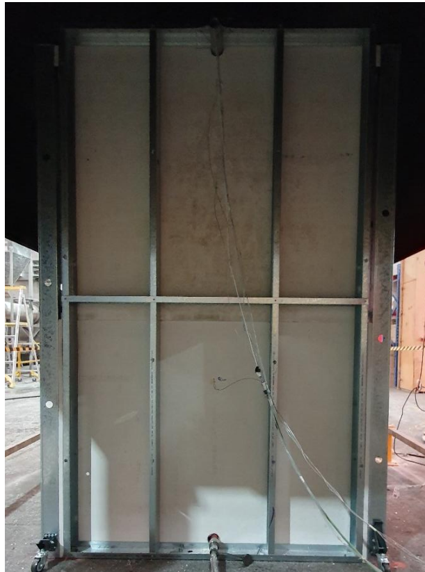
Figure 28 The specimen after the reaction to fire test – unexposed side
