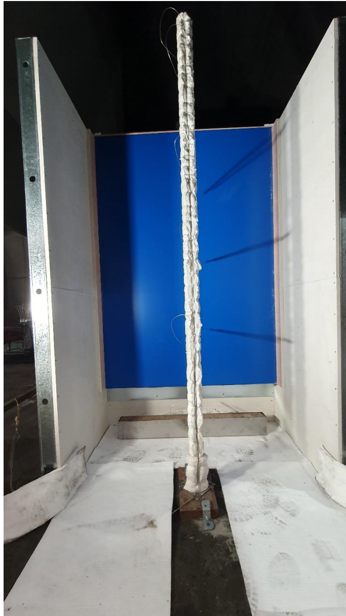
Figure 15 The specimen before the reaction to fire test – exposed side
