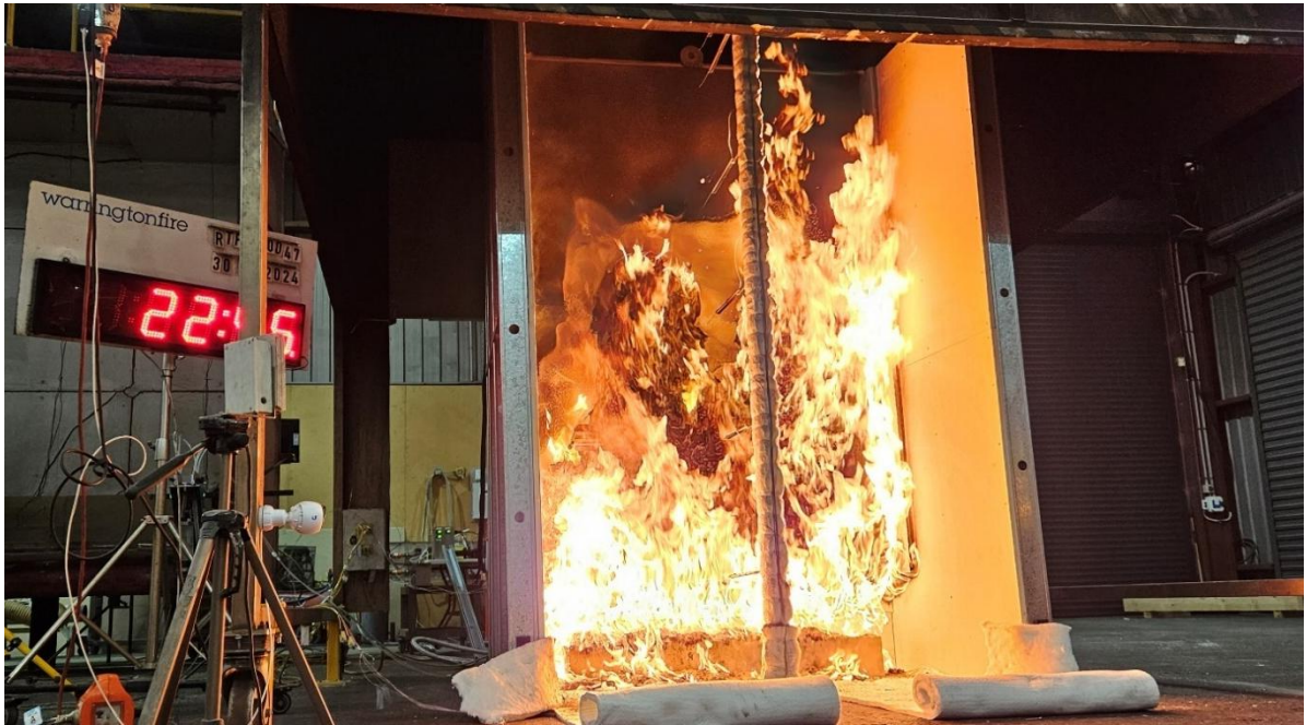
Figure 22 The specimen 22 minutes 55 seconds into the test (burner output at 300 kW)
