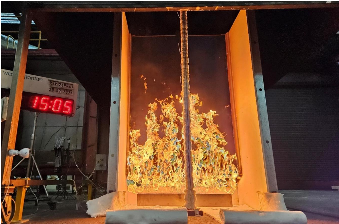
Figure 20 The specimen 15 minutes 5 seconds into the test (burner output at 300 kW)
