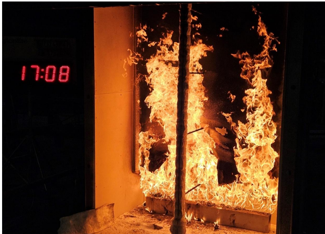
Figure 21 The specimen 17 minutes 8 seconds into the test (burner output at 300 kW)
