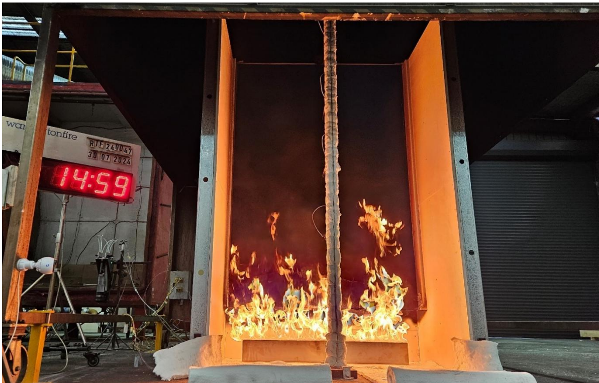
Figure 19 The specimen 14 minutes 59 seconds into the test (burner output at 100 kW)
