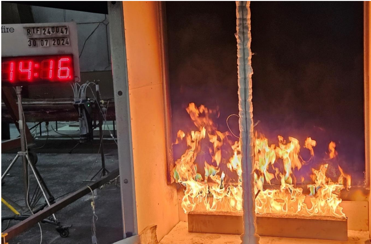
Figure 18 The specimen 14 minutes 16 seconds into the test (burner output at 100 kW)
