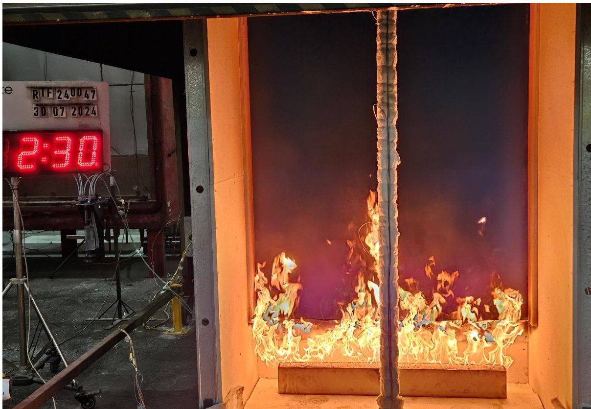
Figure 17 The specimen 2 minutes 30 seconds into the test (burner output at 100 kW)
