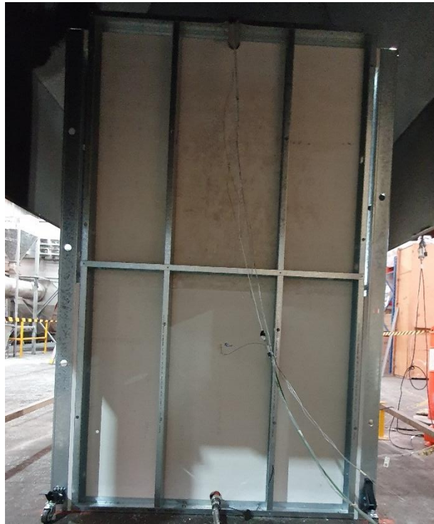
Figure 16 The specimen before the reaction to fire test – unexposed side
