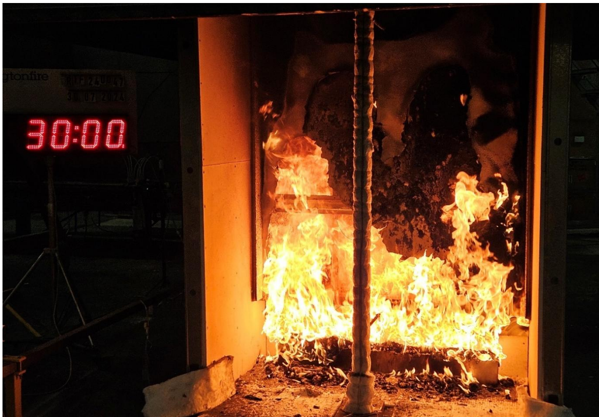
Figure 23 The specimen 30 minutes into the test (burner output at 300 kW)
