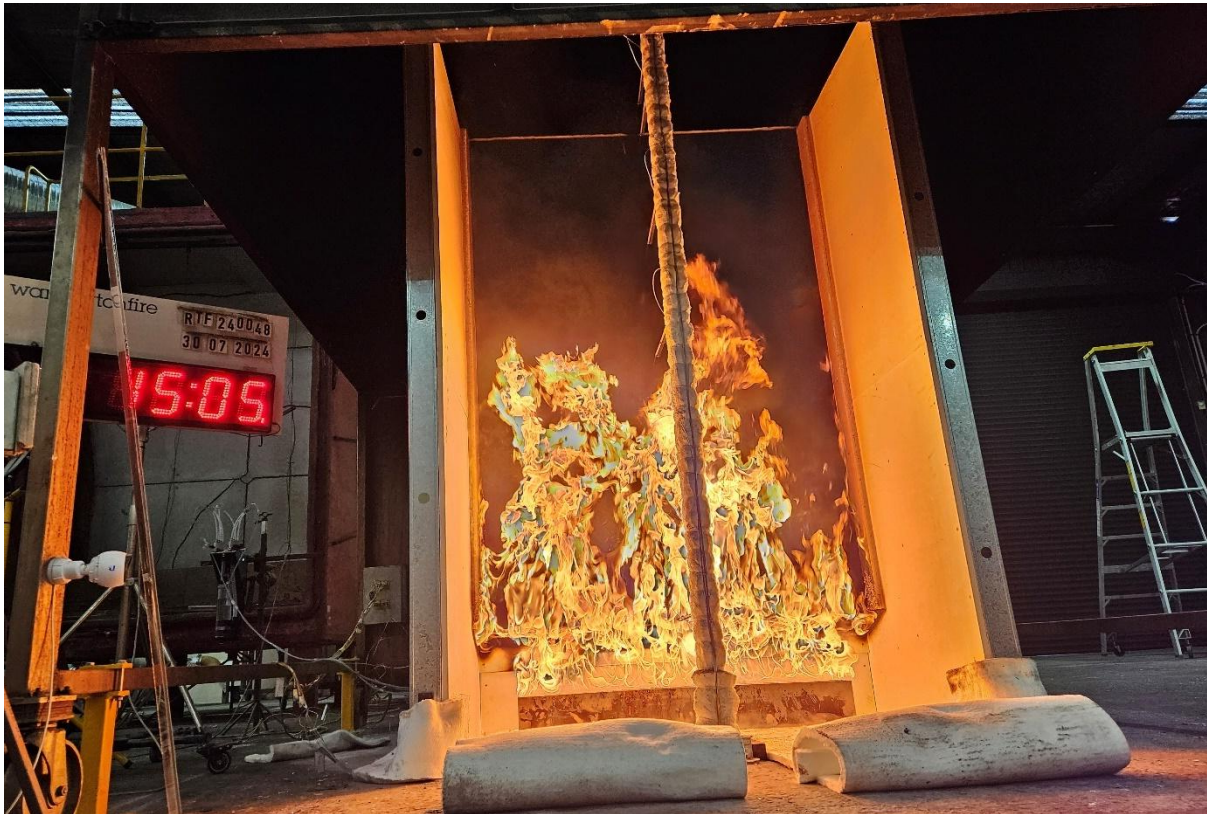
Figure 19 The specimen 15 minutes 5 seconds into the test (burner output at 300 kW)
