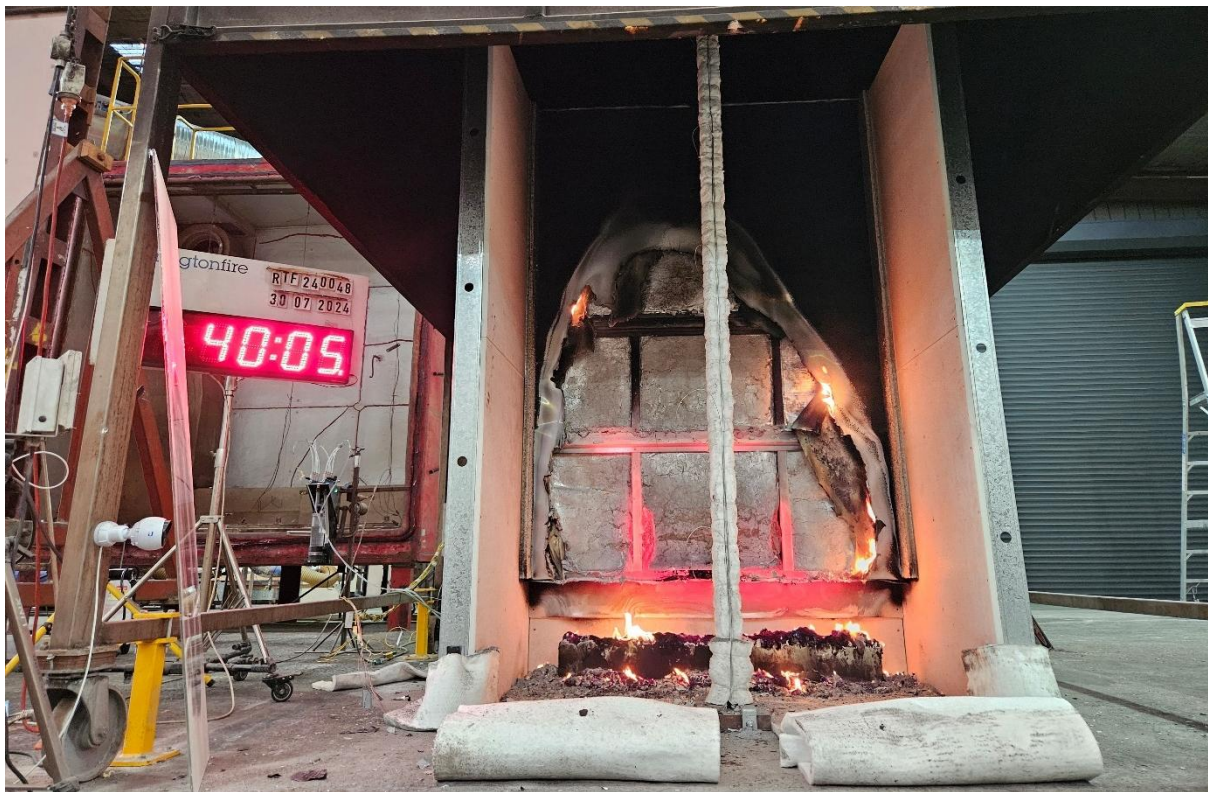
Figure 24 The specimen 40 minutes 5 seconds into the test (burner off)
