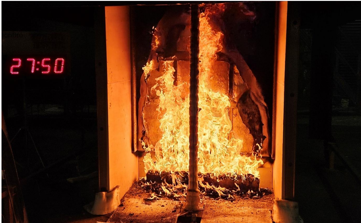
Figure 23 The specimen 27 minutes 50 seconds into the test (burner output at 300 kW)
