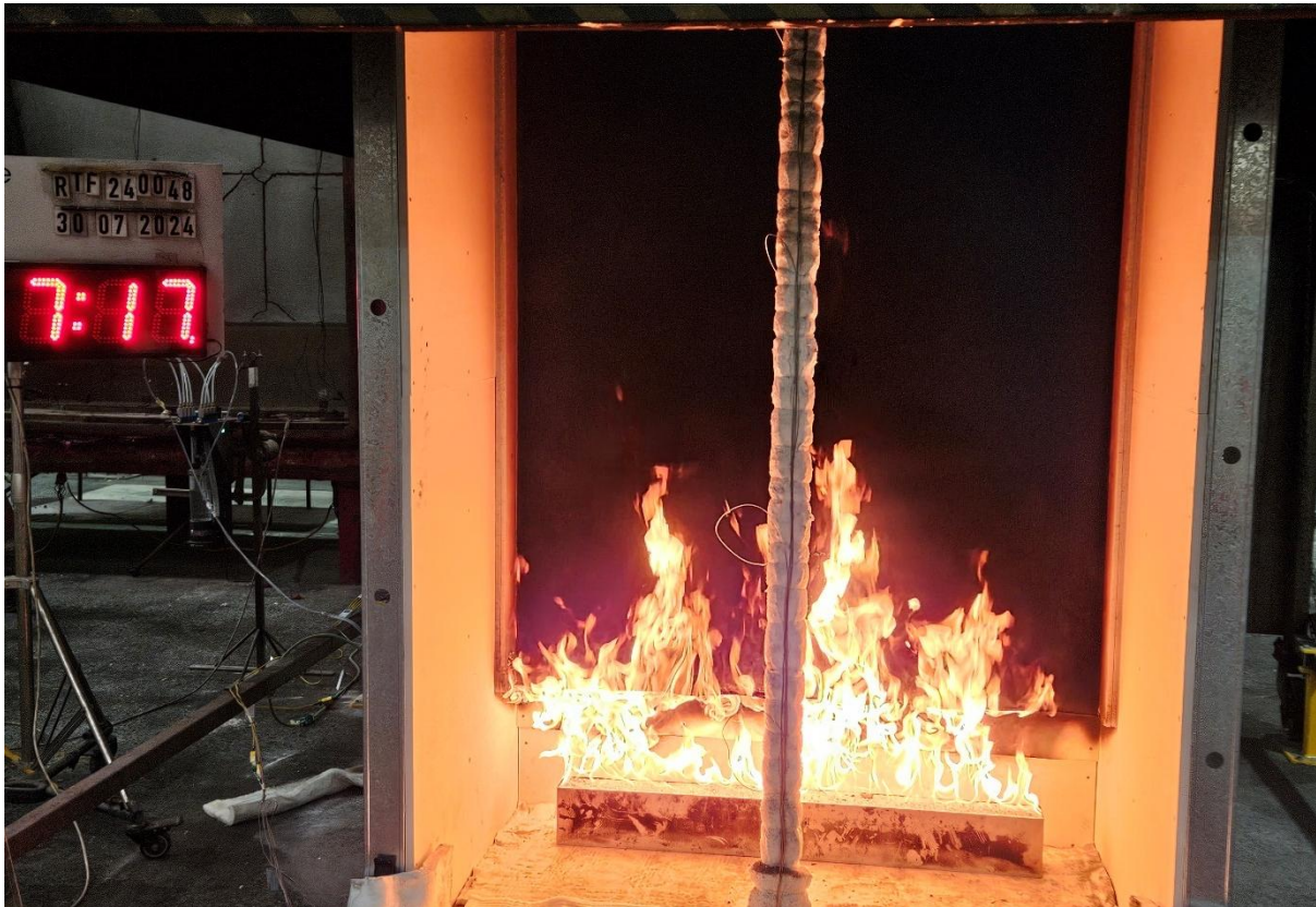
Figure 17 The specimen 7 minutes 17 seconds into the test (burner output at 100 kW)
