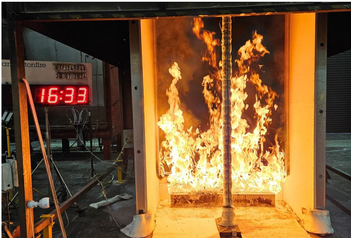
Figure 20 The specimen 16 minutes 33 seconds into the test (burner output at 300 kW)
