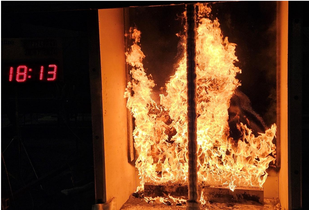
Figure 21 The specimen 18 minutes 13 seconds into the test (burner output at 300 kW)
