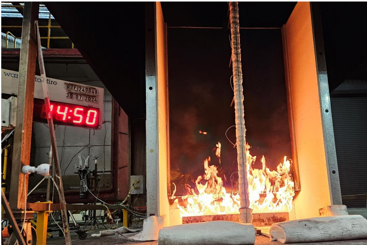
Figure 18 The specimen 14 minutes 50 seconds into the test (burner output at 100 kW)
