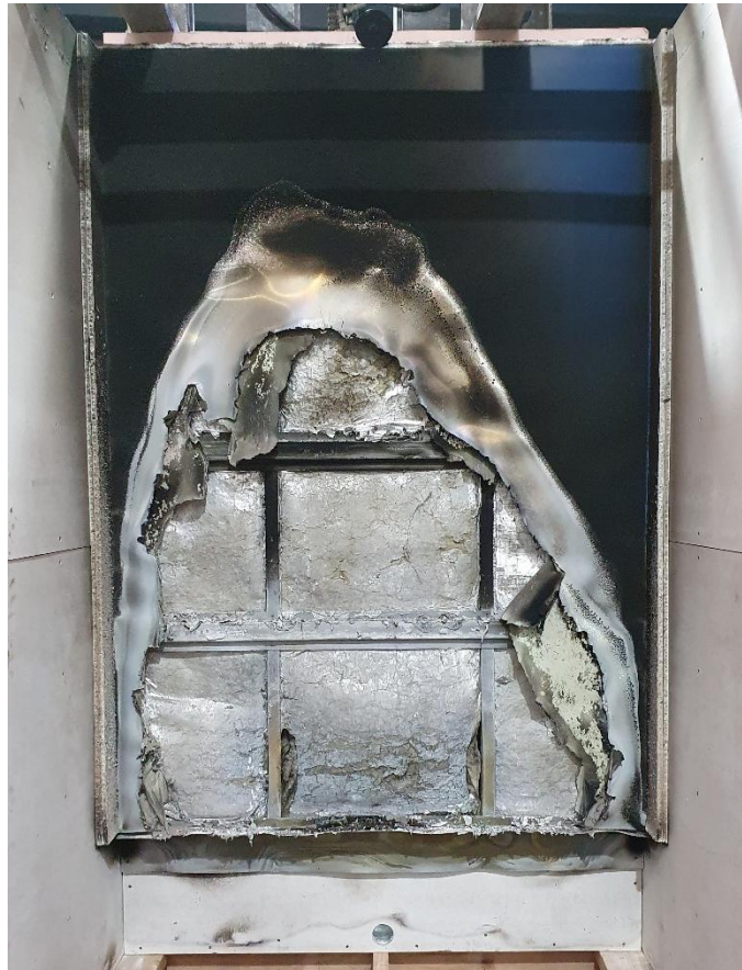
Figure 25 The specimen after the reaction to fire test – exposed side
