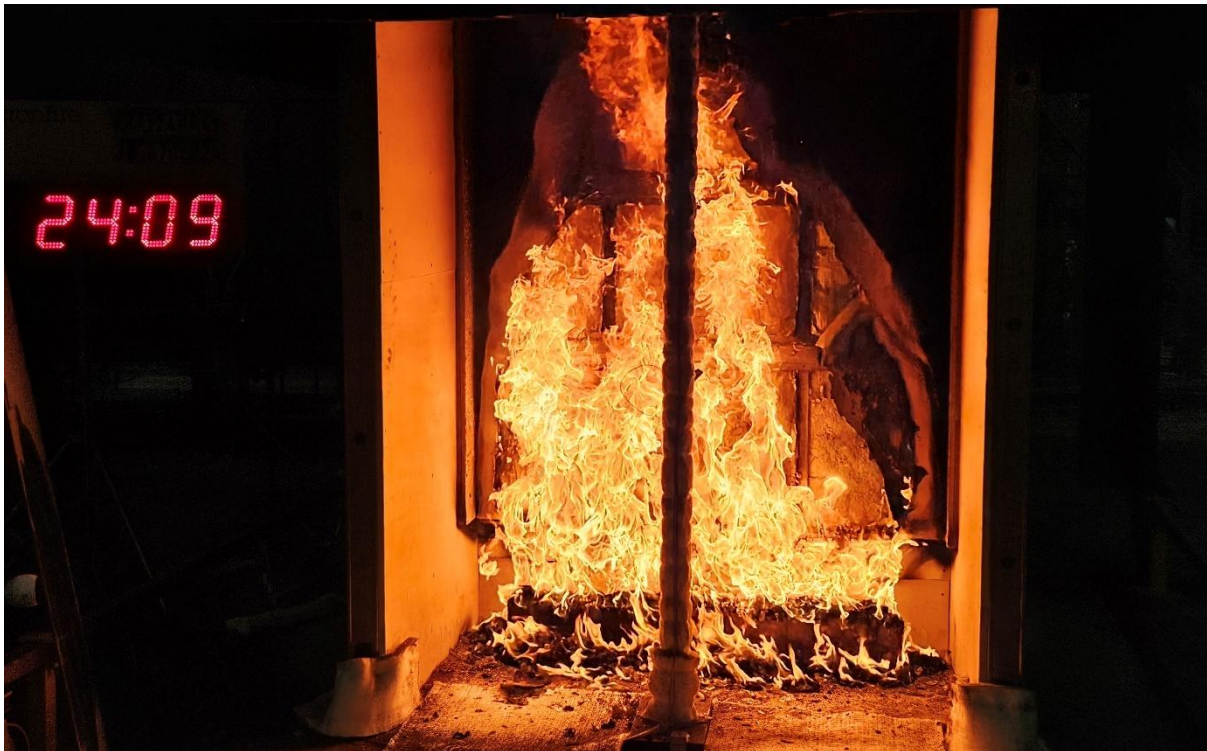
Figure 22 The specimen 24 minutes 9 seconds into the test (burner output at 300 kW)
