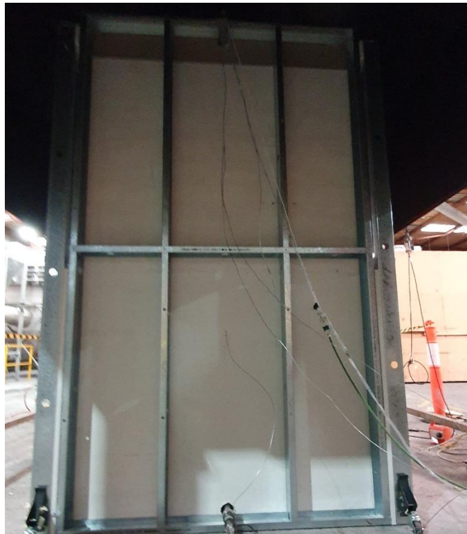
Figure 16 The specimen before the reaction to fire test – unexposed side
