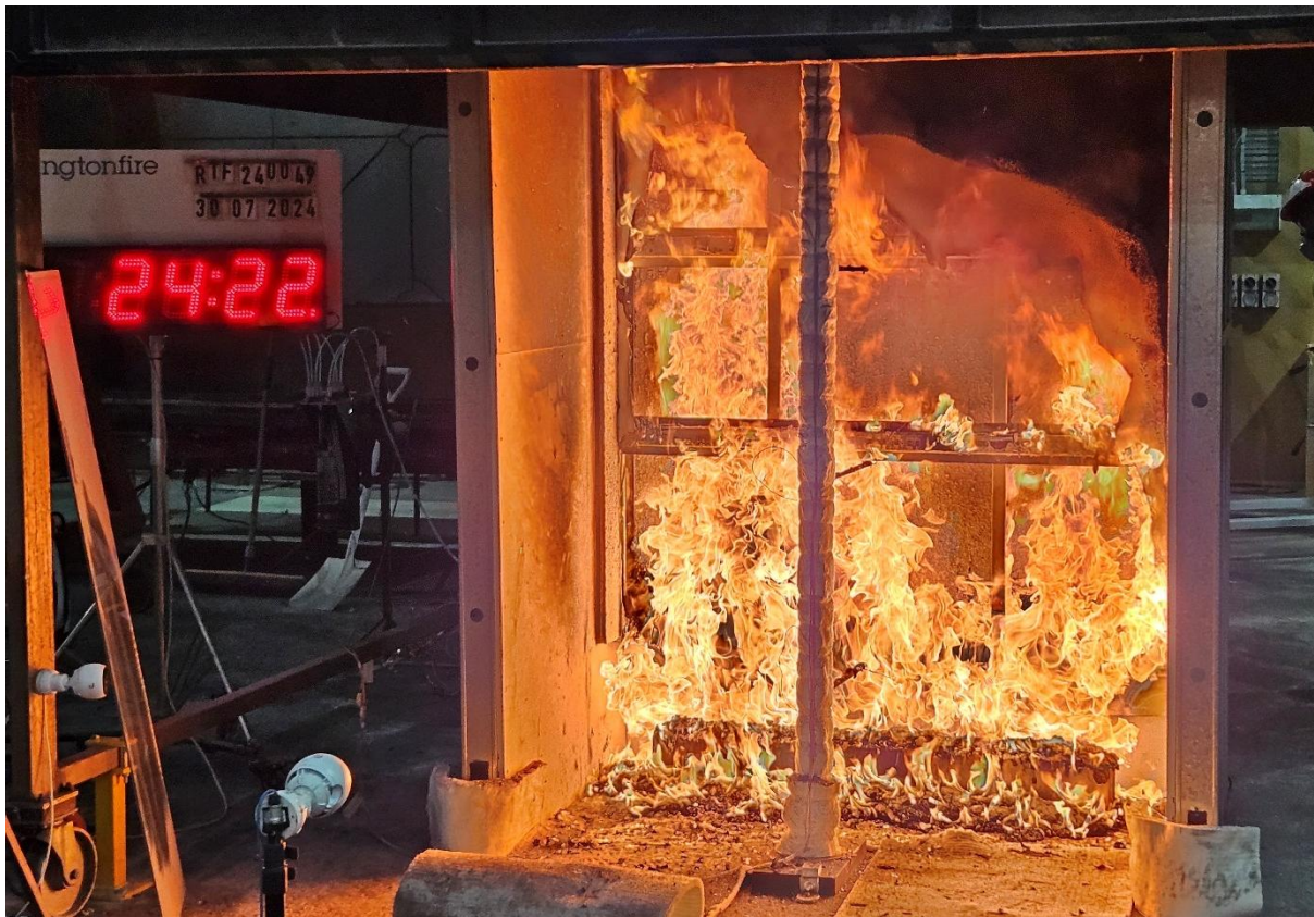
Figure 23 The specimen 24 minutes 22 seconds into the test (burner output at 300 kW)
