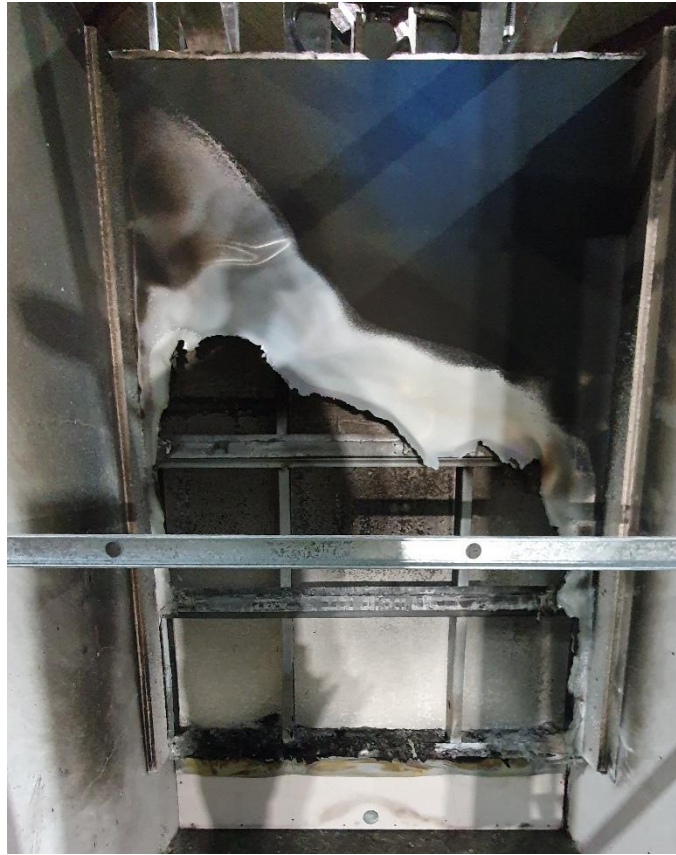
Figure 27 The specimen after the reaction to fire test – exposed side
