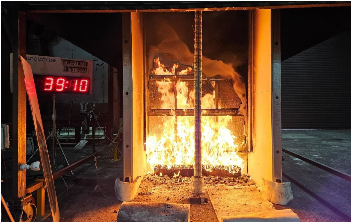
Figure 25 The specimen 39 minutes 10 seconds into the test (burner output at 300 kW)
