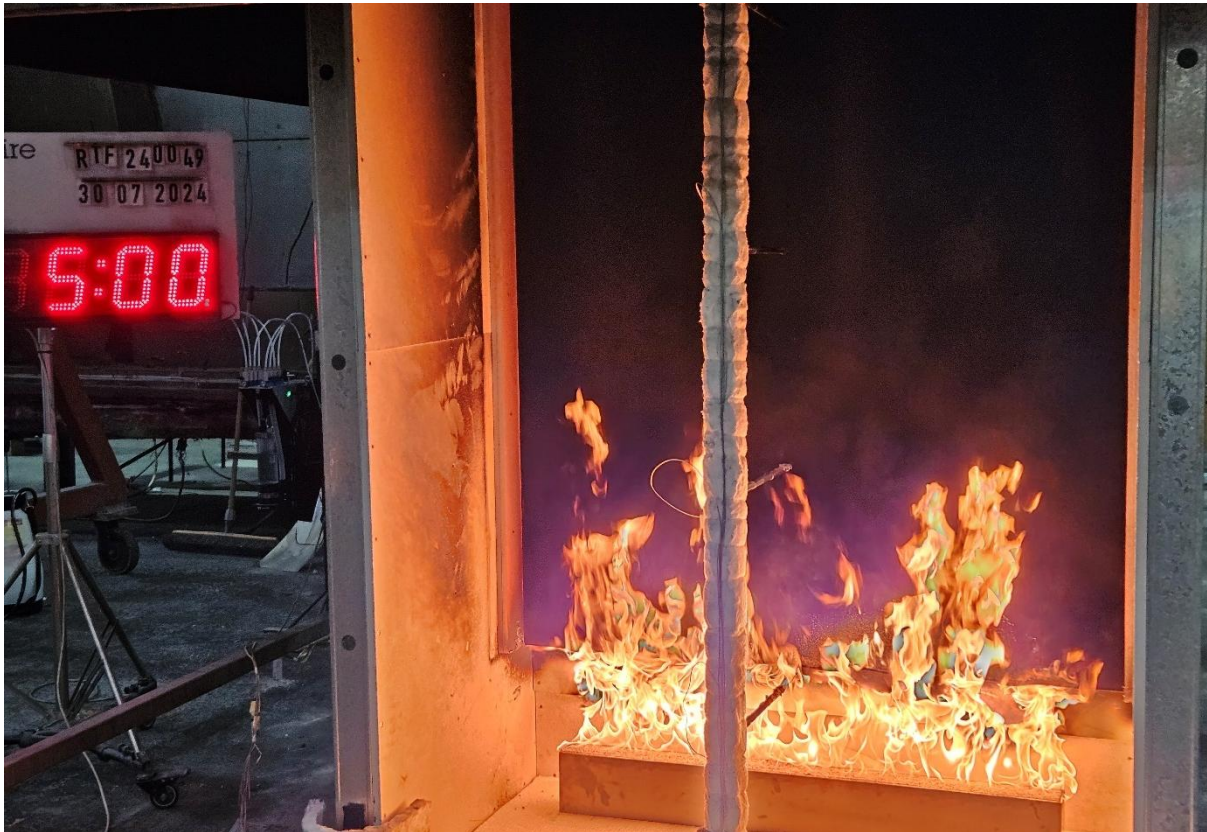
Figure 17 The specimen 5 minutes into the test (burner output at 100 kW)
