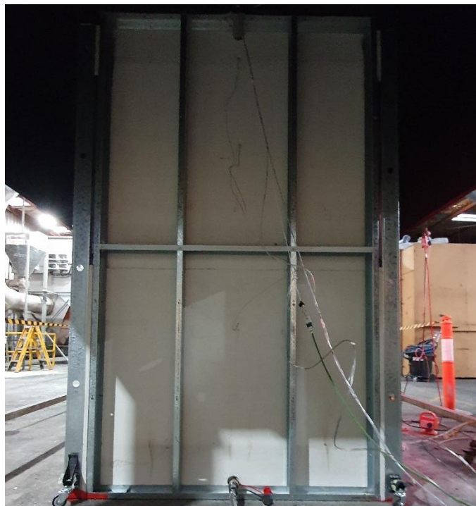
Figure 28 The specimen after the reaction to fire test – unexposed side
