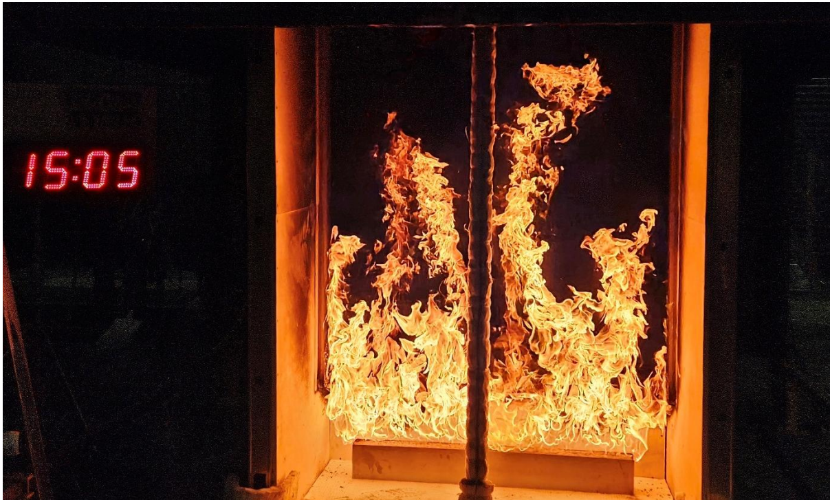
Figure 19 The specimen 15 minutes 5 seconds into the test (burner output at 300 kW)
