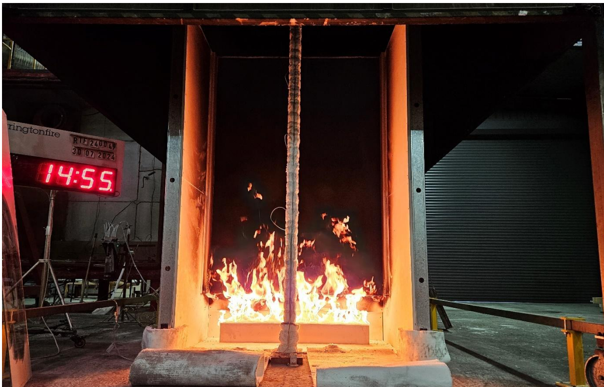
Figure 18 The specimen 14 minutes 55 seconds into the test (burner output at 100 kW)
