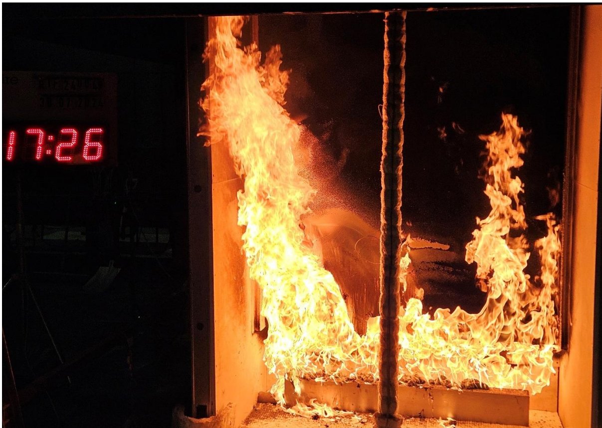
Figure 20 The specimen 17 minutes 26 seconds into the test (burner output at 300 kW)
