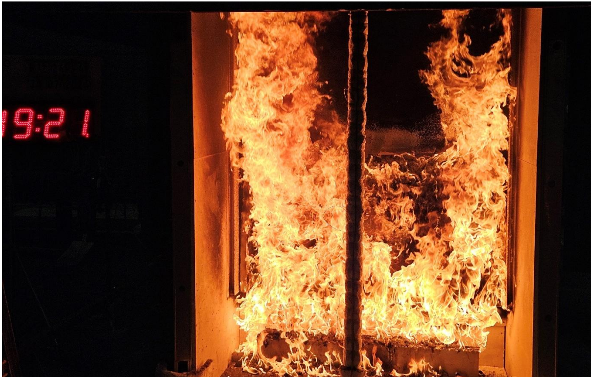
Figure 21 The specimen 19 minutes 21 seconds into the test (burner output at 300 kW)
