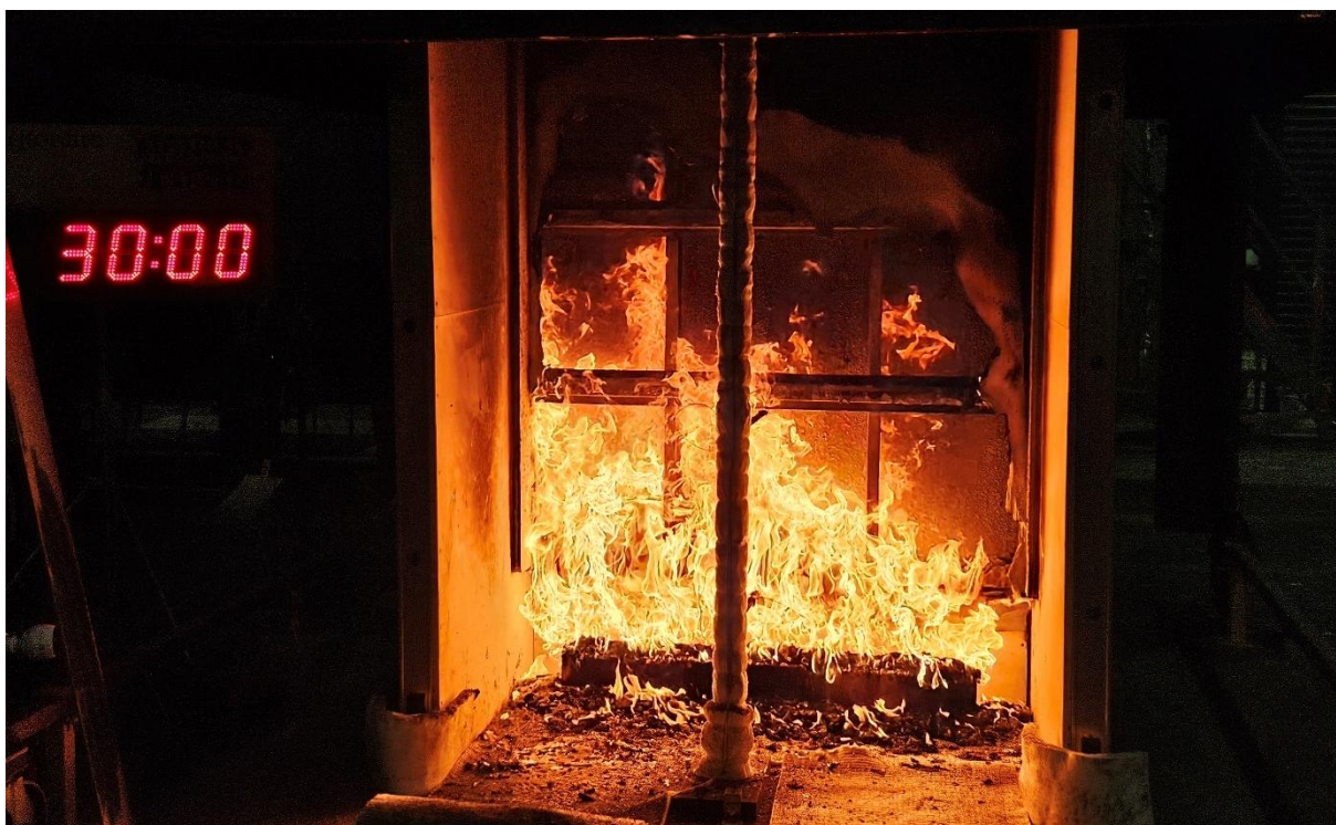
Figure 24 The specimen 30 minutes into the test (burner output at 300 kW)
