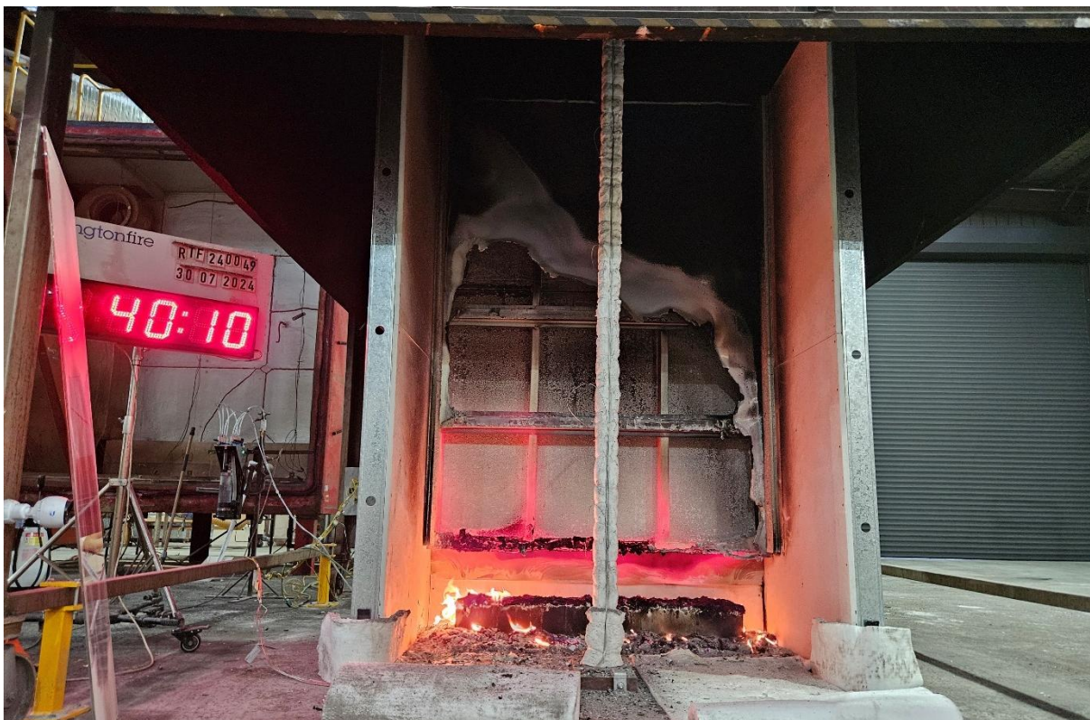
Figure 26 The specimen 40 minutes 10 seconds into the test (burner off)
