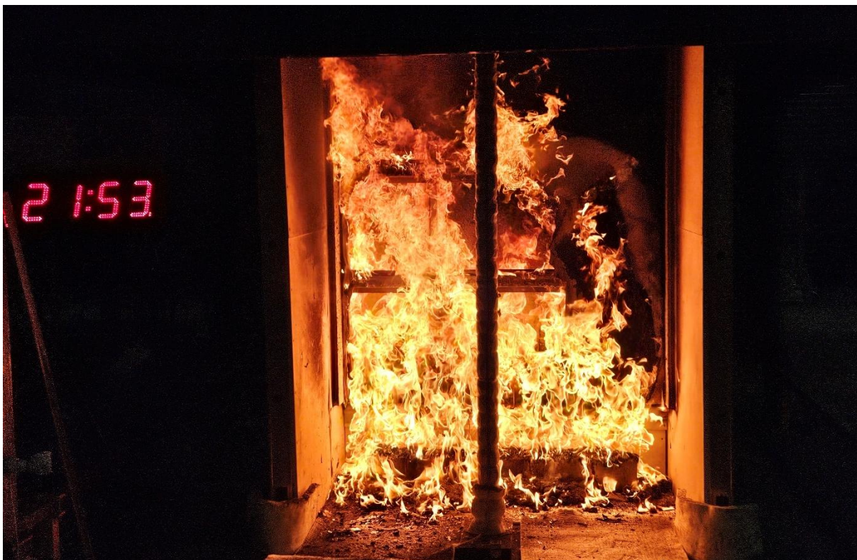
Figure 22 The specimen 21 minutes 53 seconds into the test (burner output at 300 kW)
