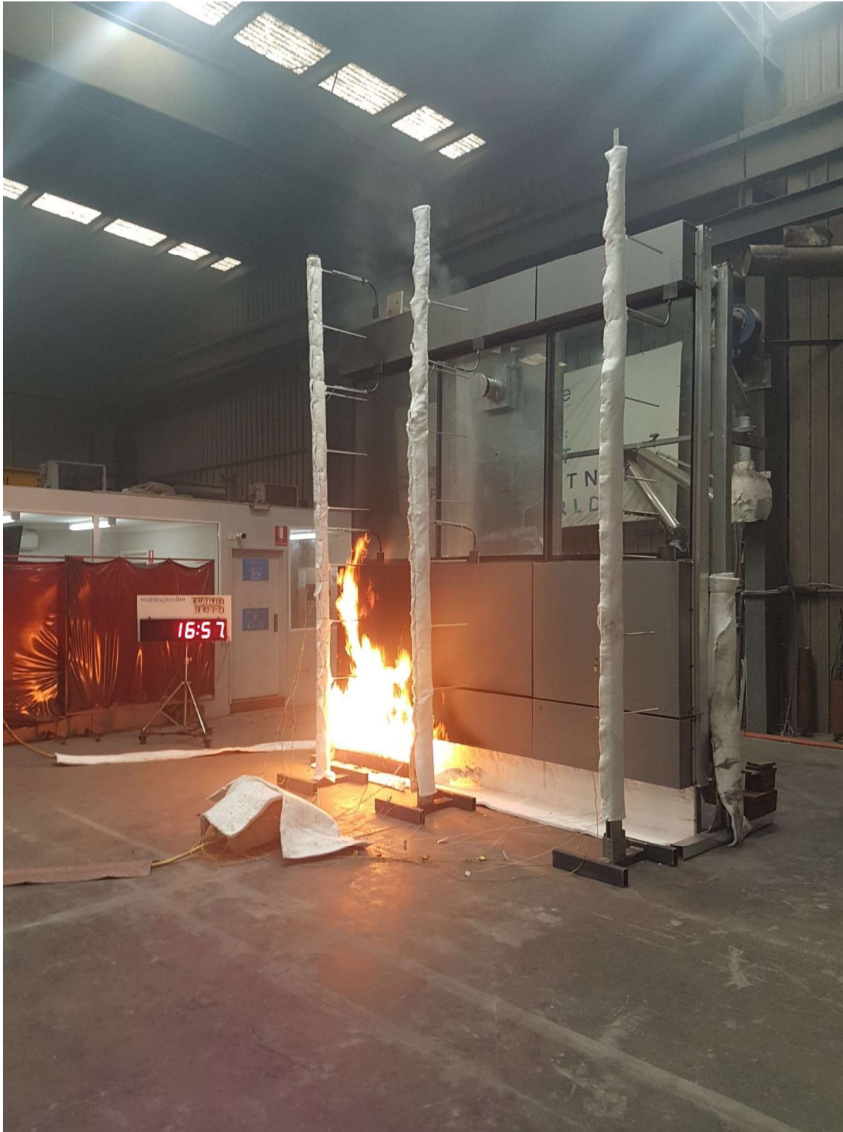
Figure 35 The specimen 16 minutes 57 seconds into the test (burner output at 300 kW)
