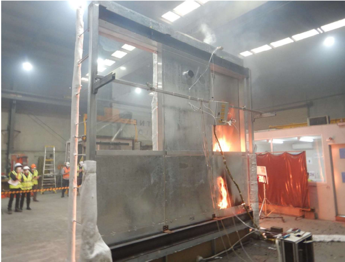
Figure 48 The specimen 28 minutes 1 second into the test (burner output at 300 kW) – unexposed side.
