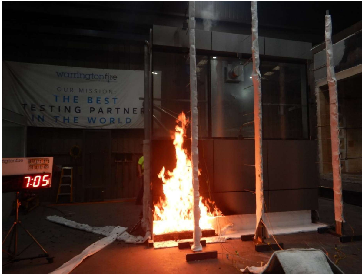
Figure 27 The specimen 7 minutes 5 seconds into the test (burner output at 300 kW)
