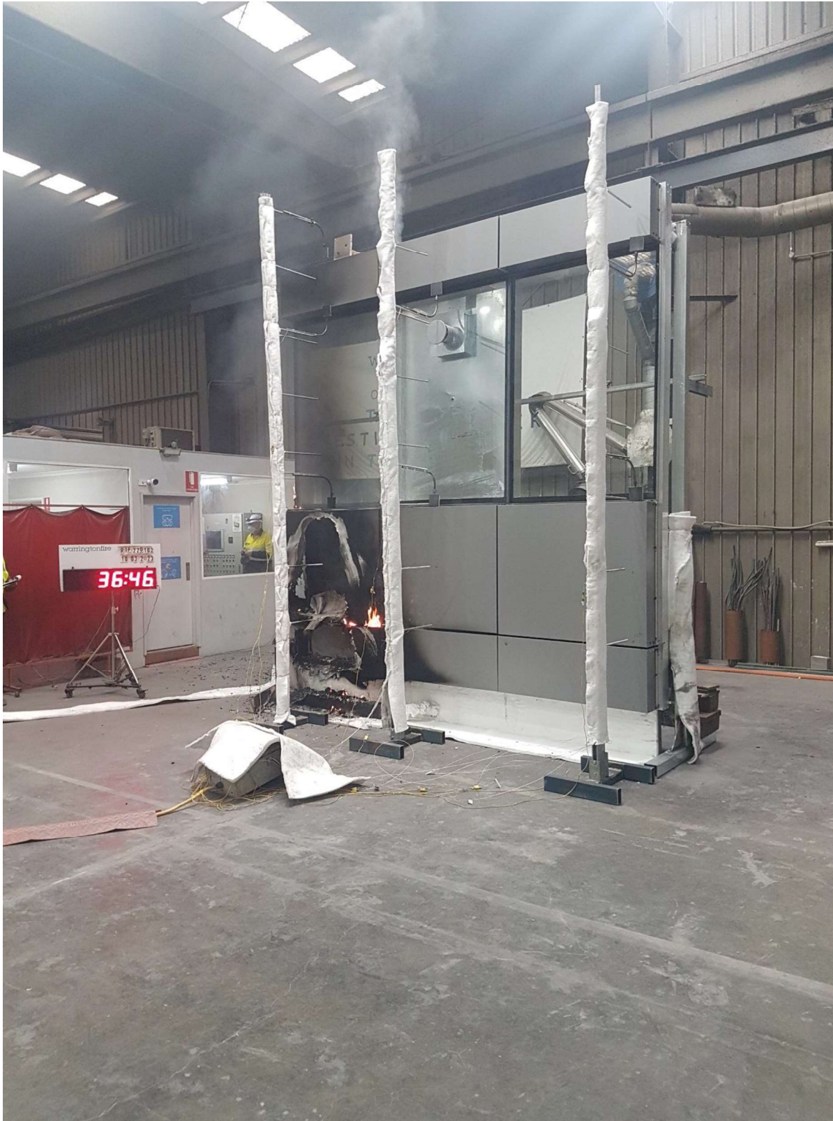
Figure 57 The specimen 36 minutes 46 seconds into the test (burner off).
