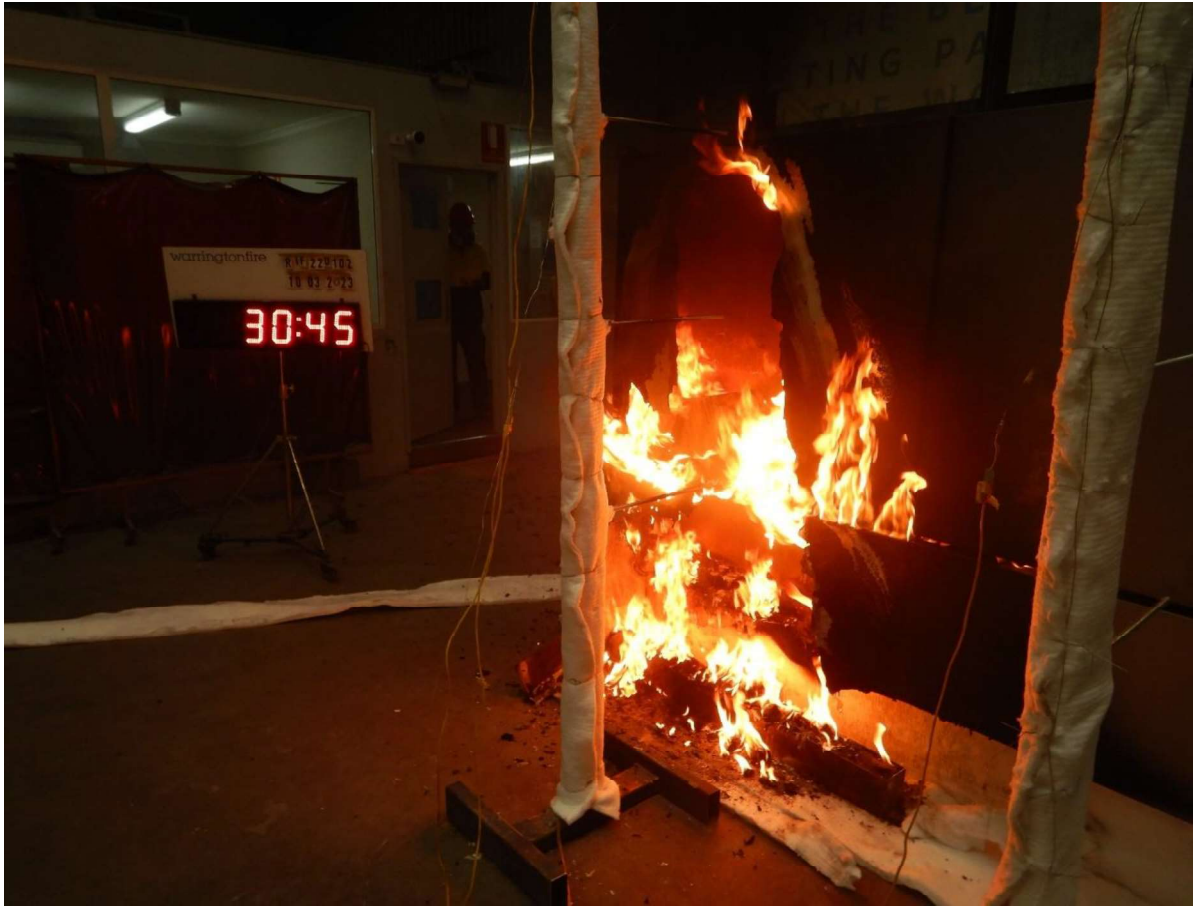
Figure 53 The specimen 30 minutes 45 seconds into the test (burner off).
