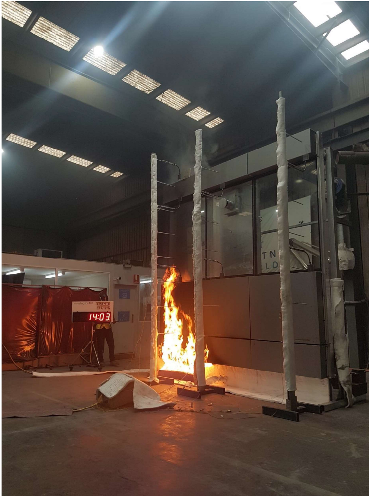
Figure 33 The specimen 14 minutes 3 seconds into the test (burner output at 300 kW)
