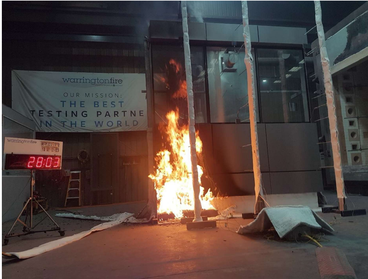
Figure 47 The specimen 28 minutes 3 seconds into the test (burner output at 300 kW)
