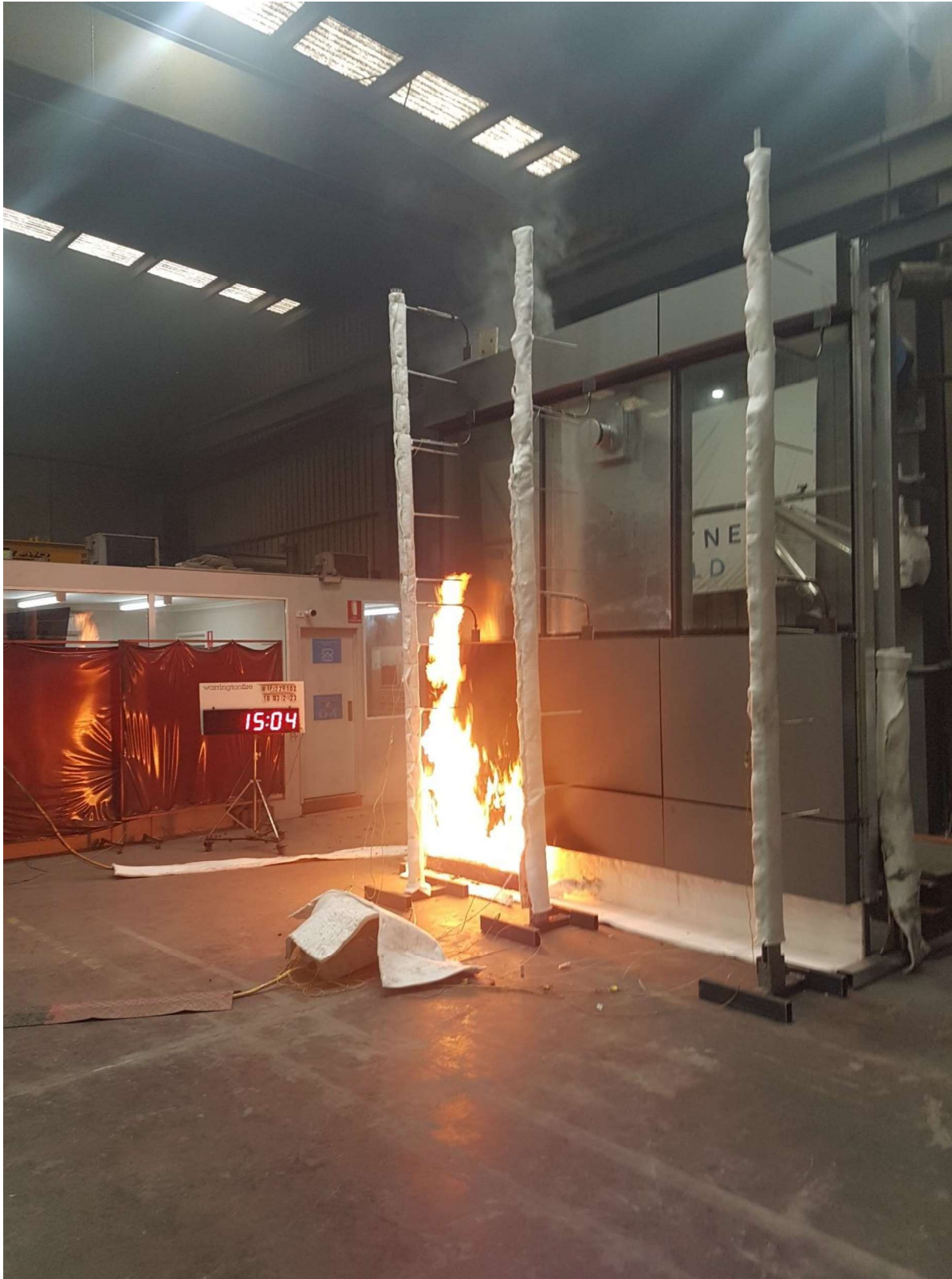
Figure 34 The specimen 15 minutes 4 seconds into the test (burner output at 300 kW)
