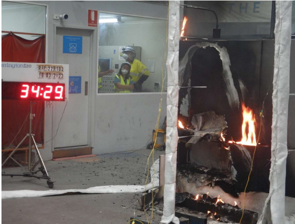
Figure 55 The specimen 34 minutes 29 seconds into the test (burner off).
