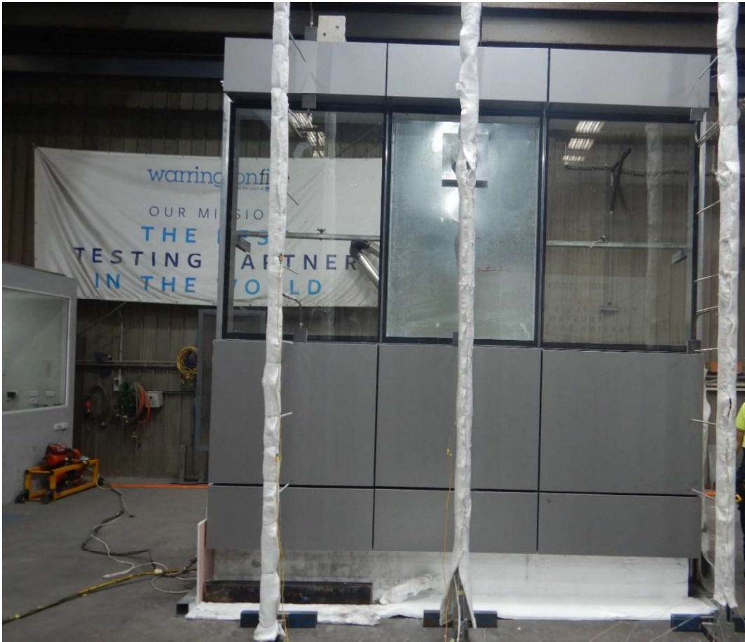
Figure 20 The specimen (exposed side) before the reaction to fire test
