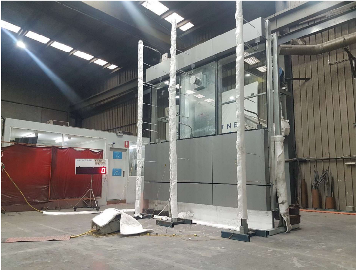
Figure 22 The specimen (angled - exposed side) before the reaction to fire test
