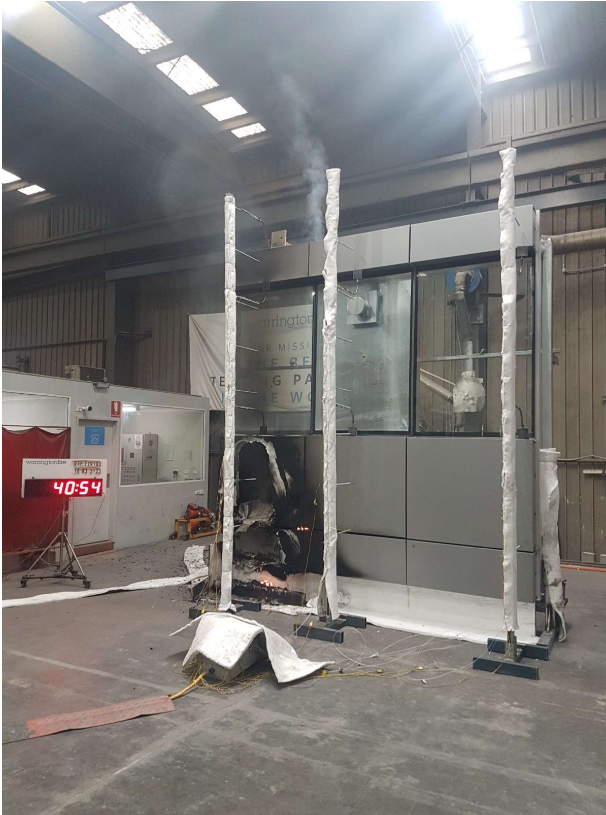
Figure 58 The specimen 40 minutes 54 seconds into the test (burner off).
