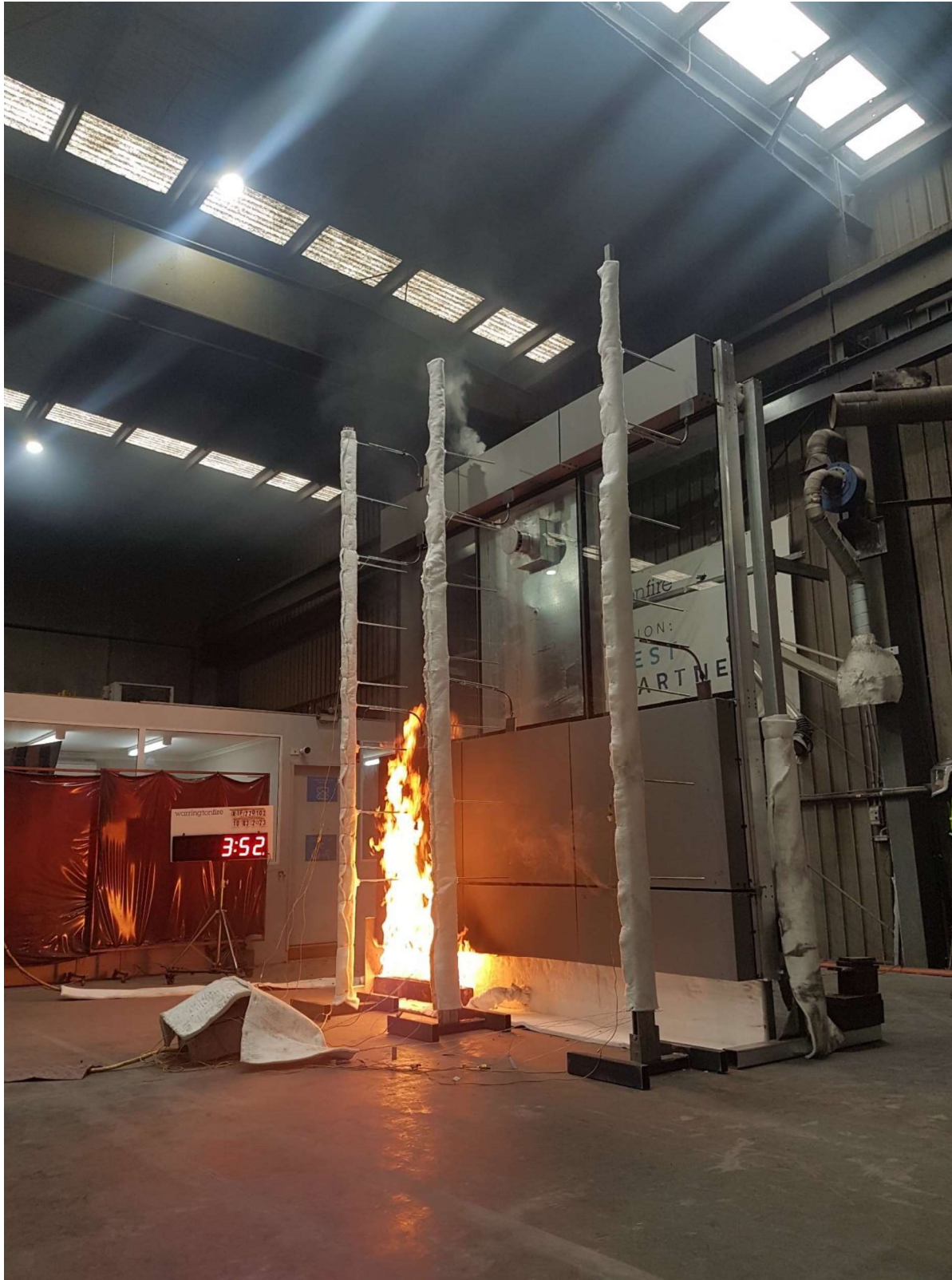
Figure 26 The specimen 3 minutes 52 seconds into the test (burner output at 300 kW)
