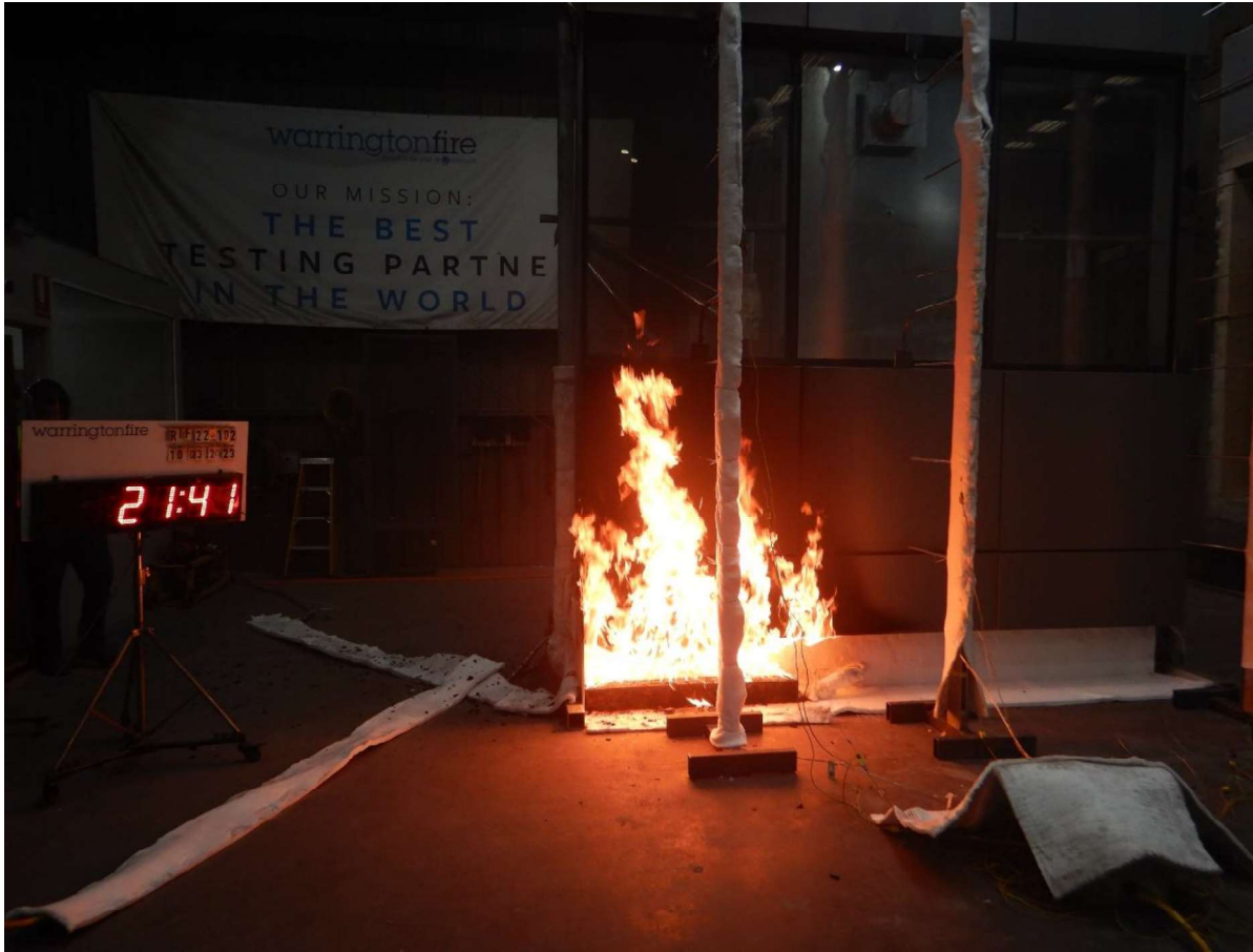
Figure 40 The specimen 21 minutes 41 seconds into the test (burner output at 300 kW)
