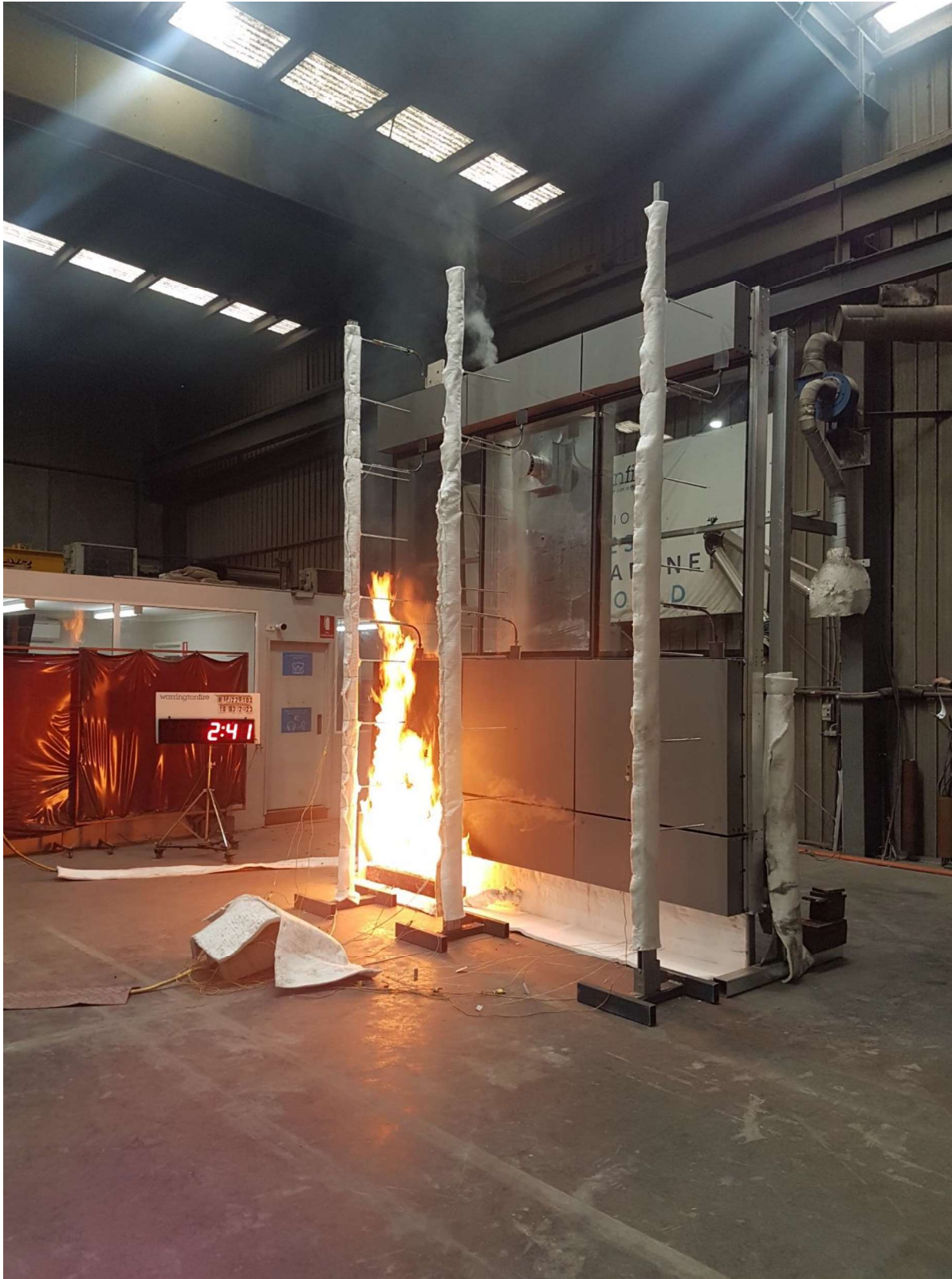
Figure 25 The specimen 2 minutes 41 seconds into the test (burner output at 300 kW)
