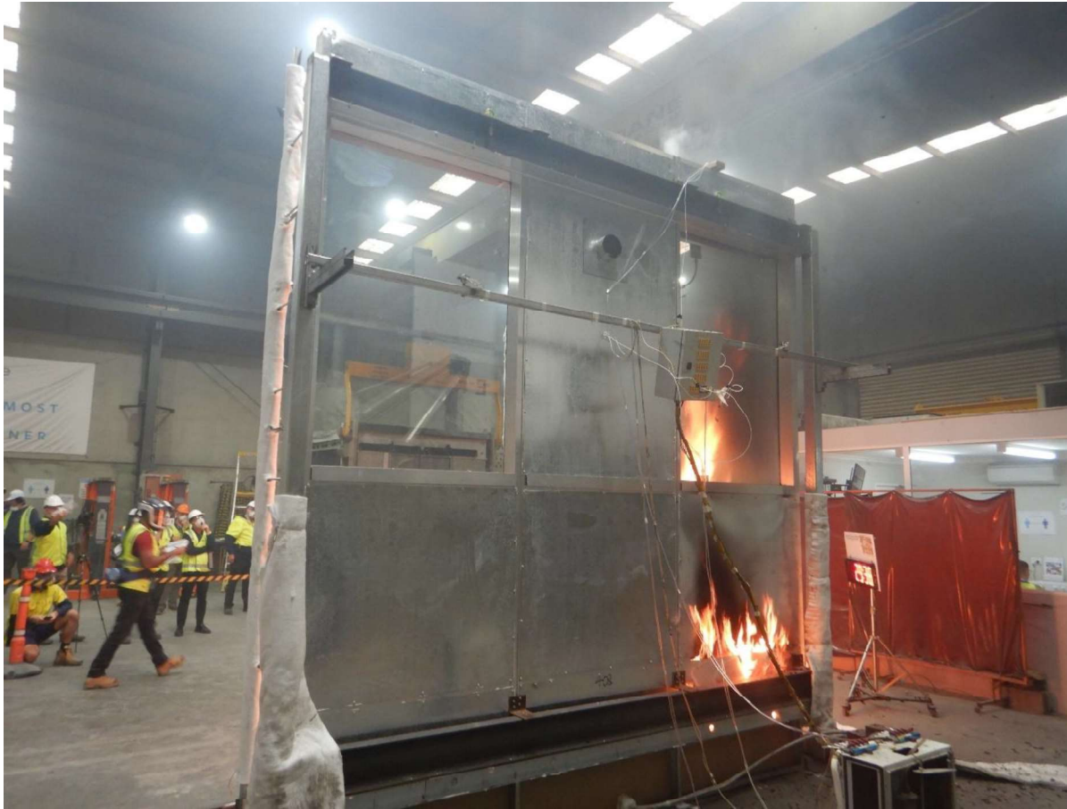
Figure 51 The specimen 29 minutes 38 seconds into the test (burner output at 300 kW) – unexposed side.
