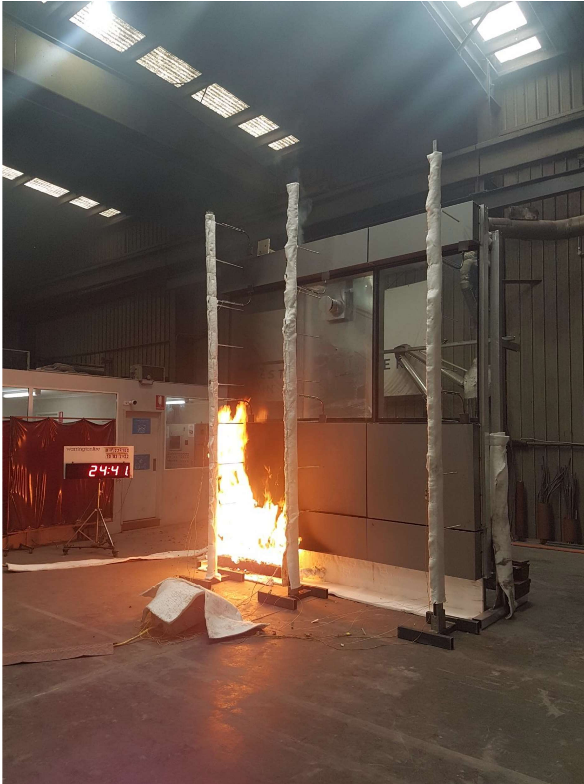
Figure 43 The specimen 24 minutes 41 seconds into the test (burner output at 300 kW)
