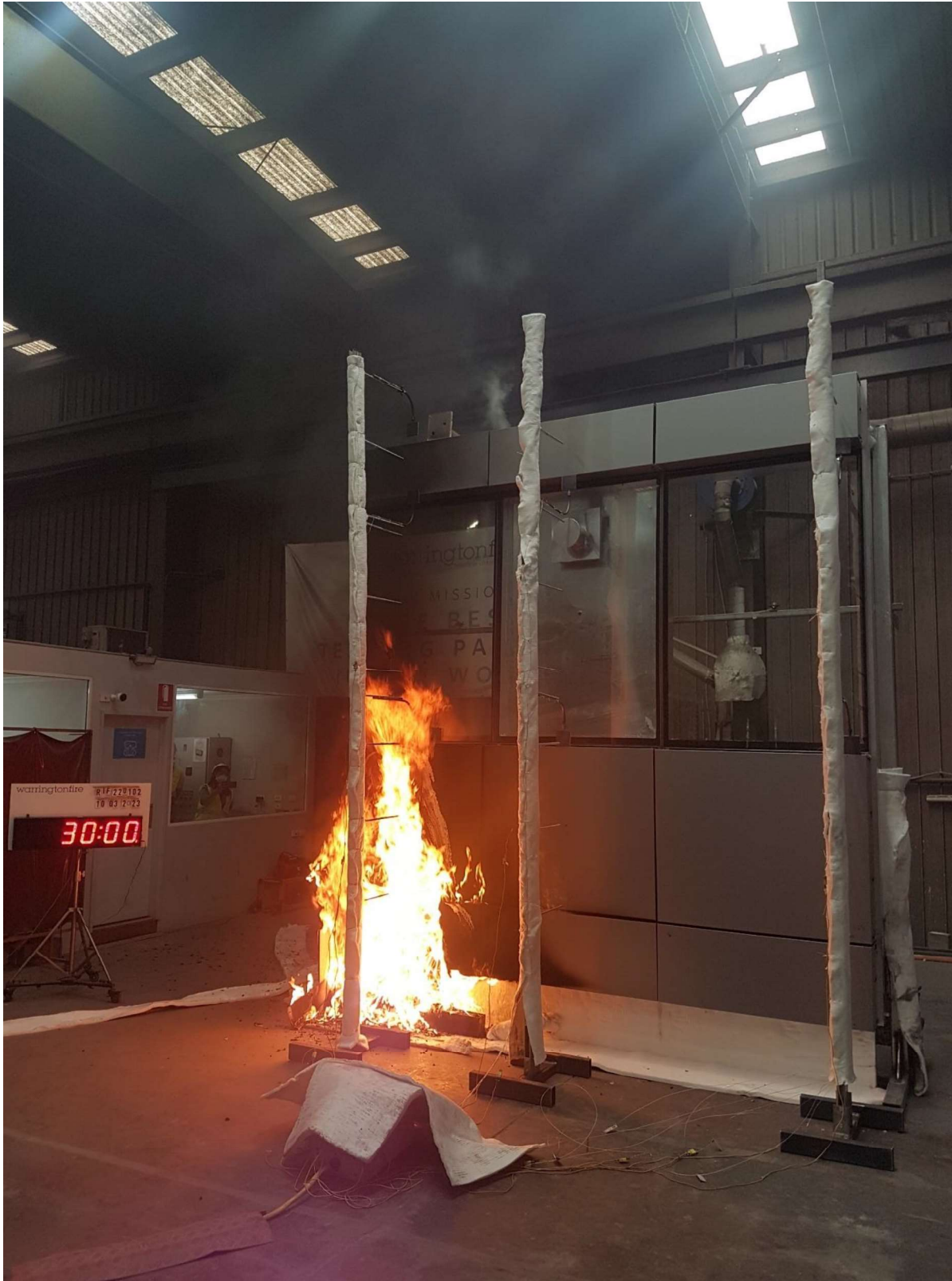
Figure 52 The specimen 30 minutes into the test - burner turned off.
