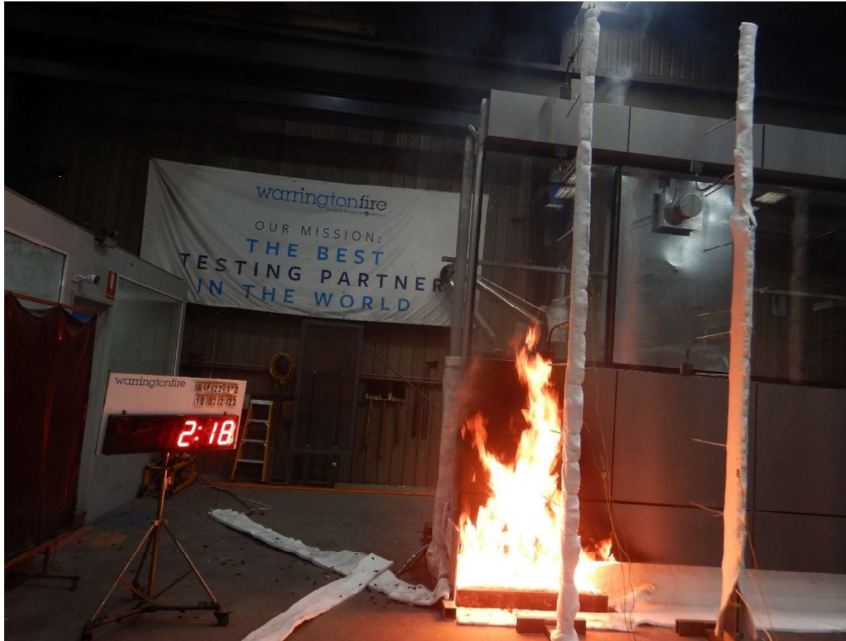
Figure 24 The specimen 2 minutes 18 seconds into the test (burner output at 300 kW)
