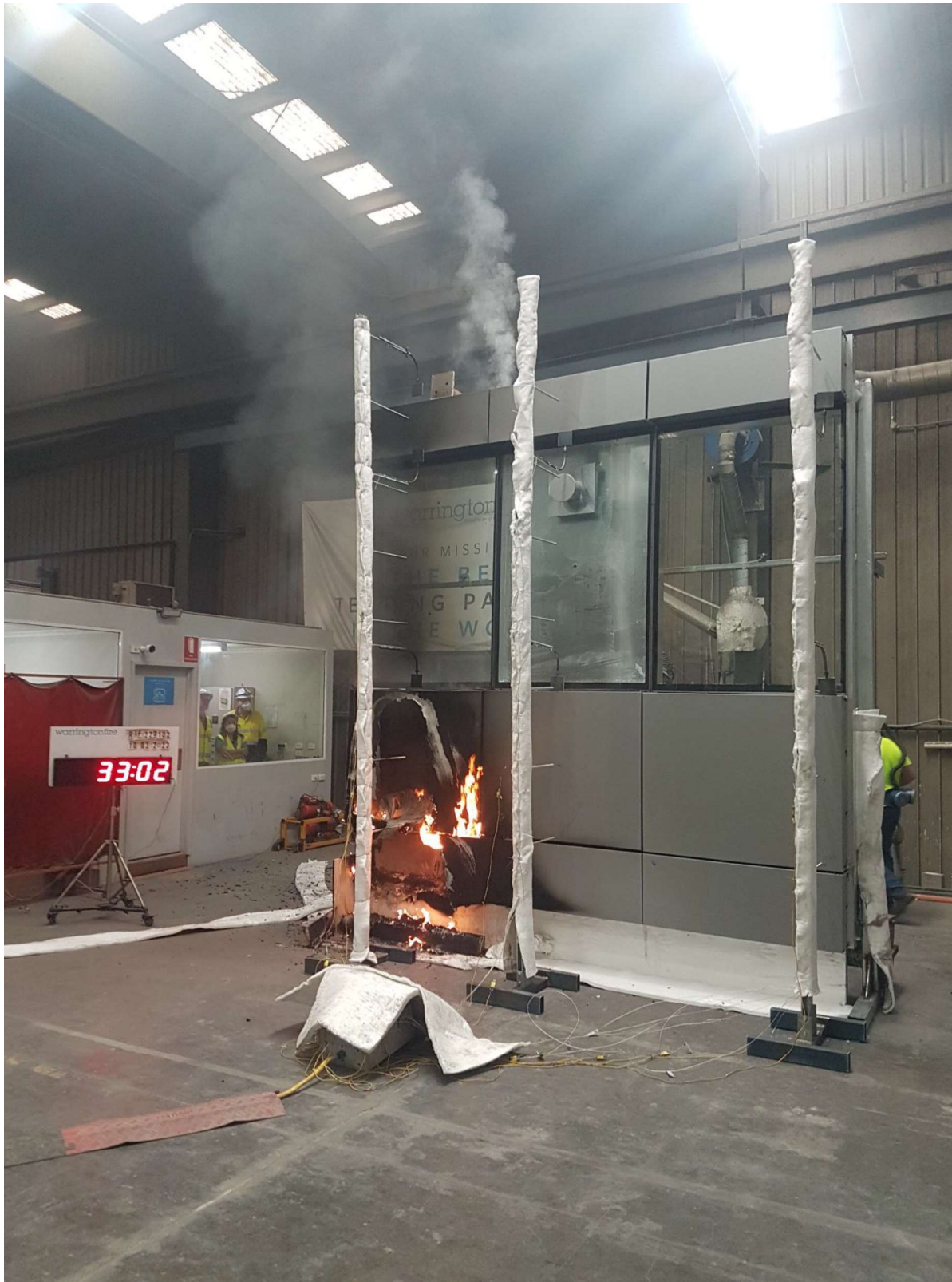
Figure 54 The specimen 33 minutes 2 seconds into the test (burner off).
