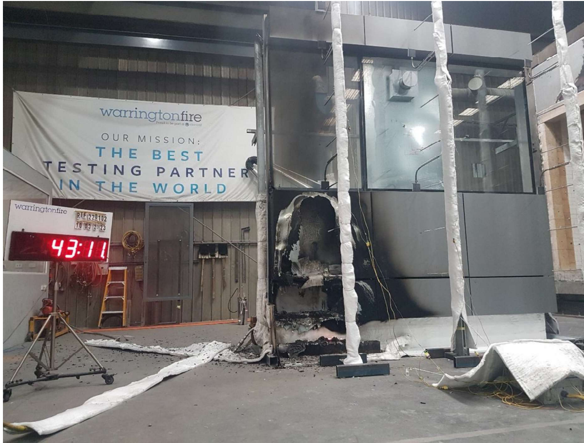
Figure 59 The specimen 43 minutes 11 seconds into the test (burner off).
