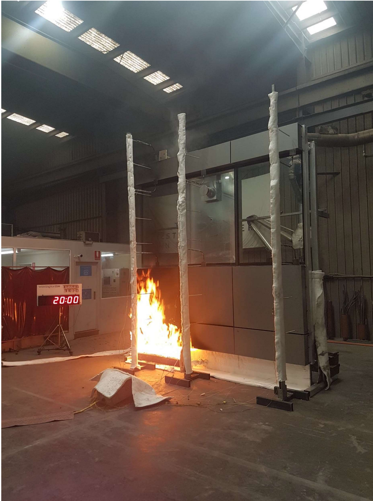
Figure 37 The specimen 20 minutes into the test (burner output at 300 kW)
