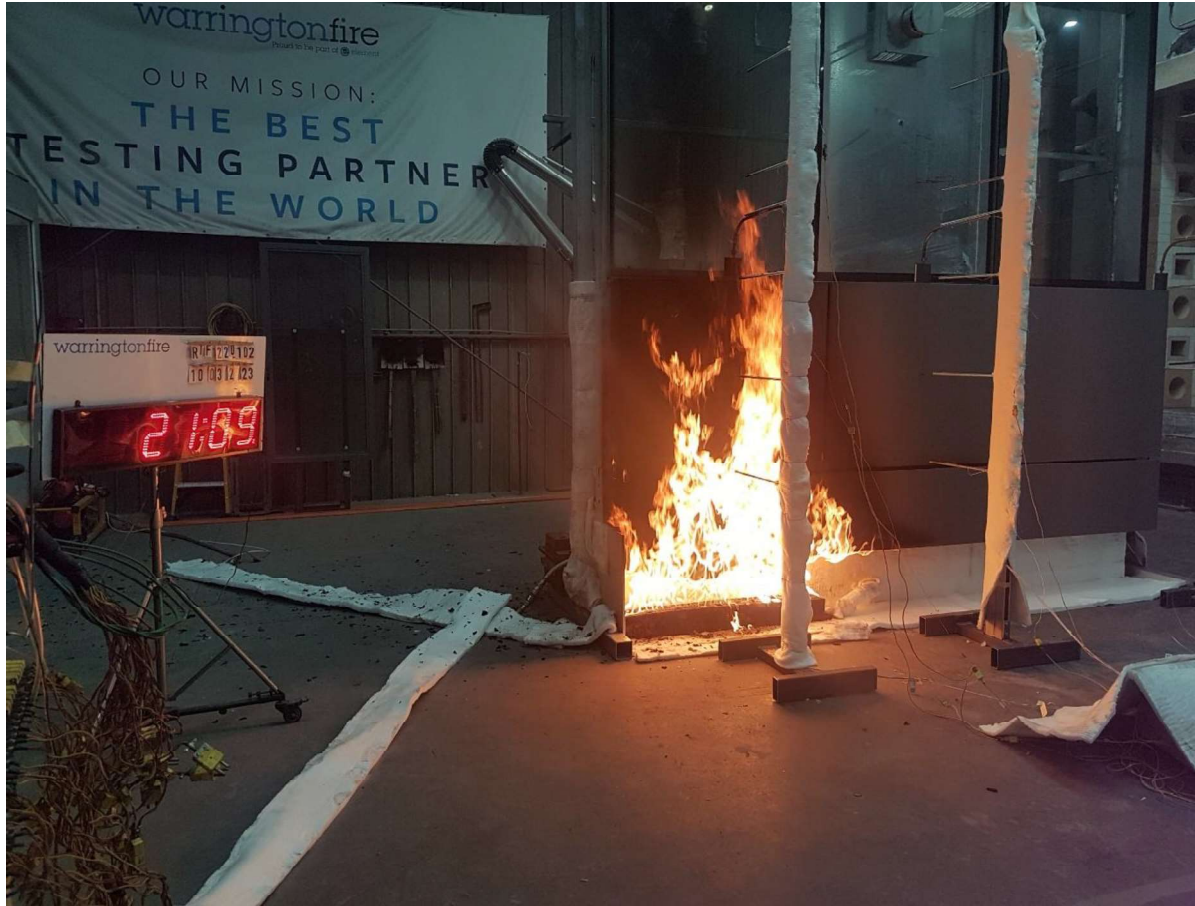
Figure 39 The specimen 21 minutes 9 seconds into the test (burner output at 300 kW)
