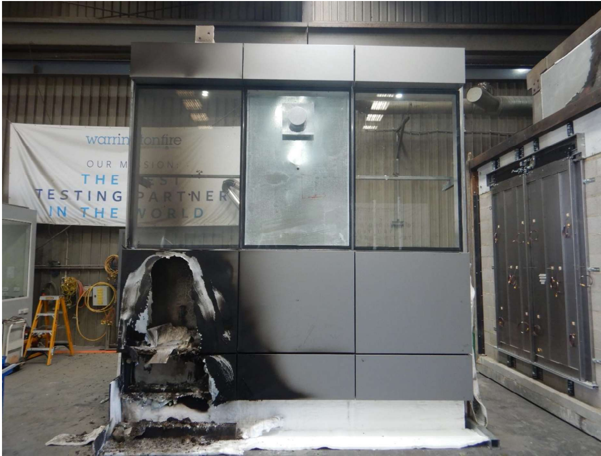
Figure 60 The specimen at end of test – exposed side.
