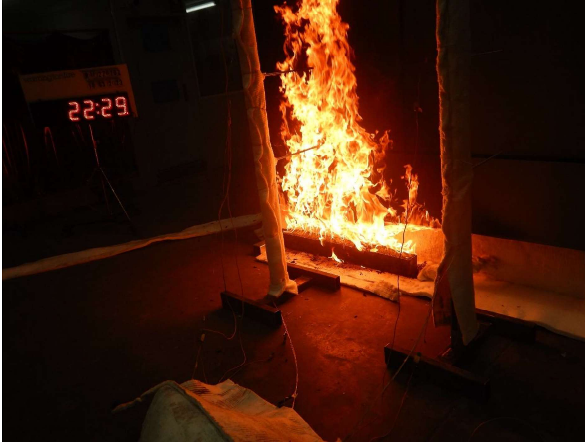
Figure 41 The specimen 22 minutes 29 seconds into the test (burner output at 300 kW)
