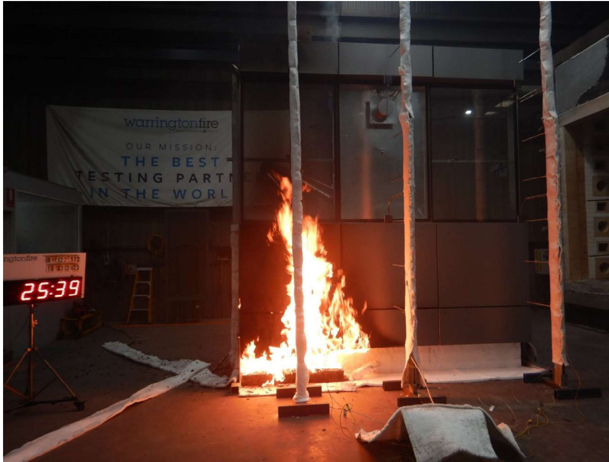
Figure 45 The specimen 25 minutes 39 seconds into the test (burner output at 300 kW)
