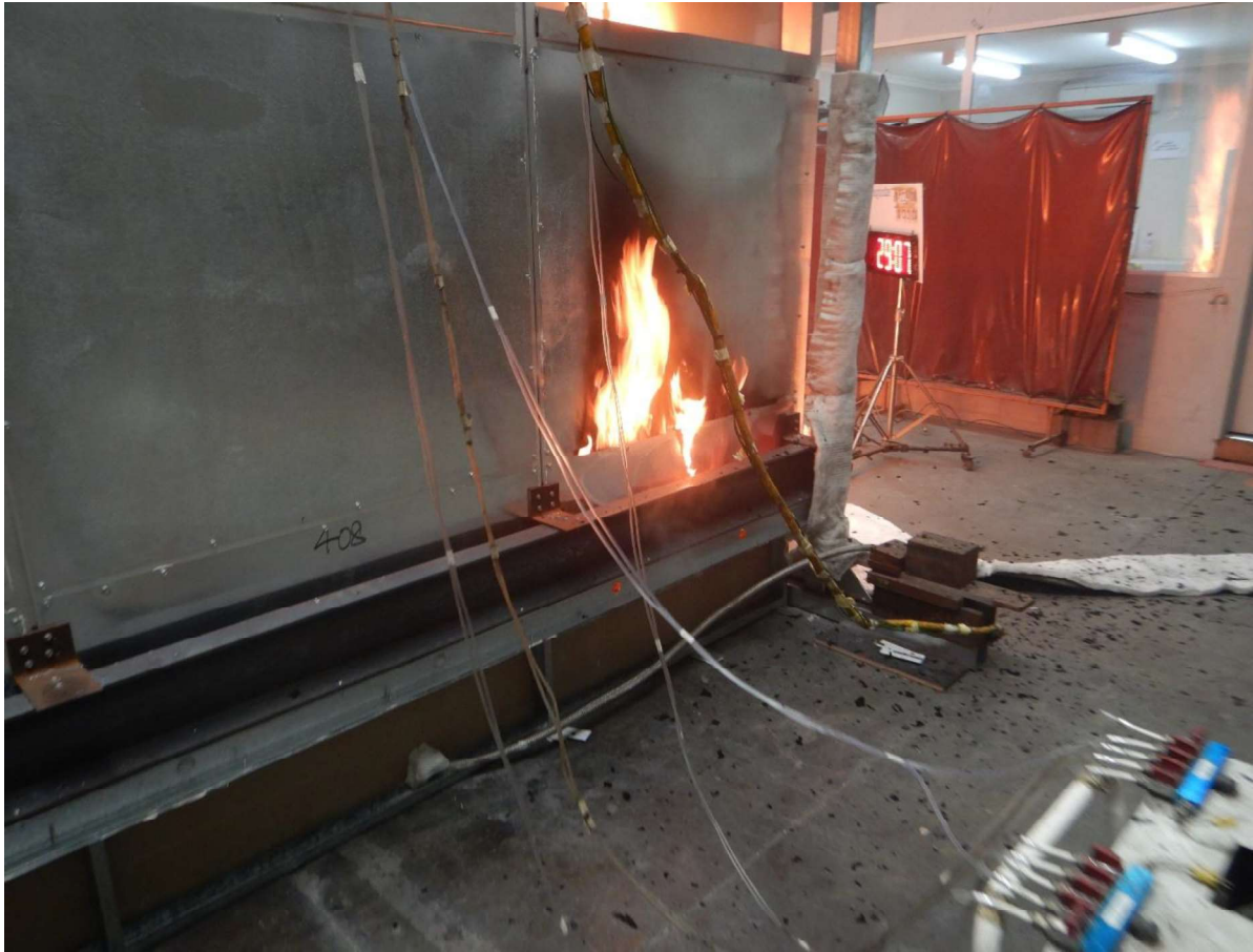
Figure 49 The specimen 29 minutes 7 seconds into the test (burner output at 300 kW) – unexposed side.
