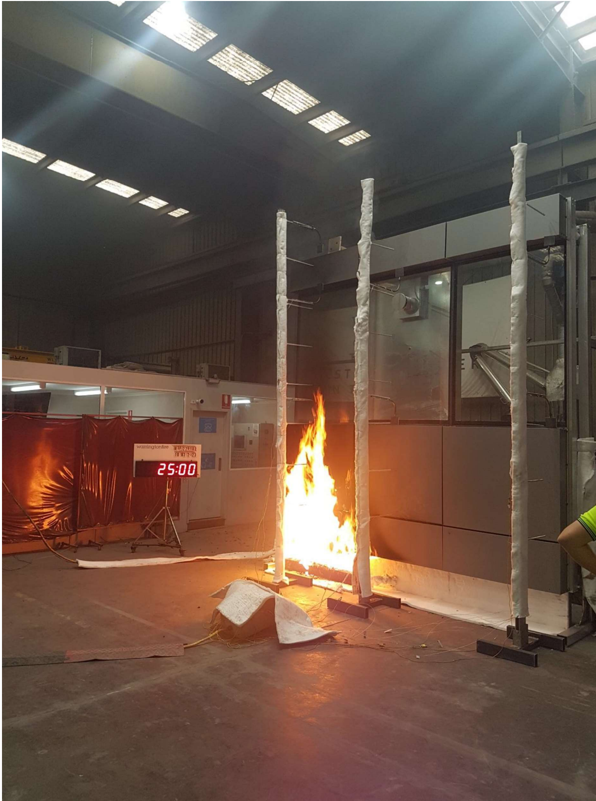
Figure 44 The specimen 25 minutes into the test (burner output at 300 kW)
