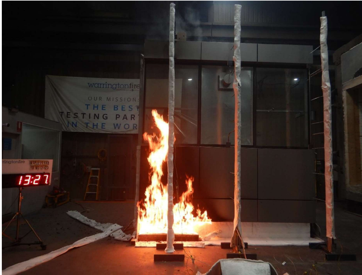
Figure 32 The specimen 13 minutes 27 seconds into the test (burner output at 300 kW)
