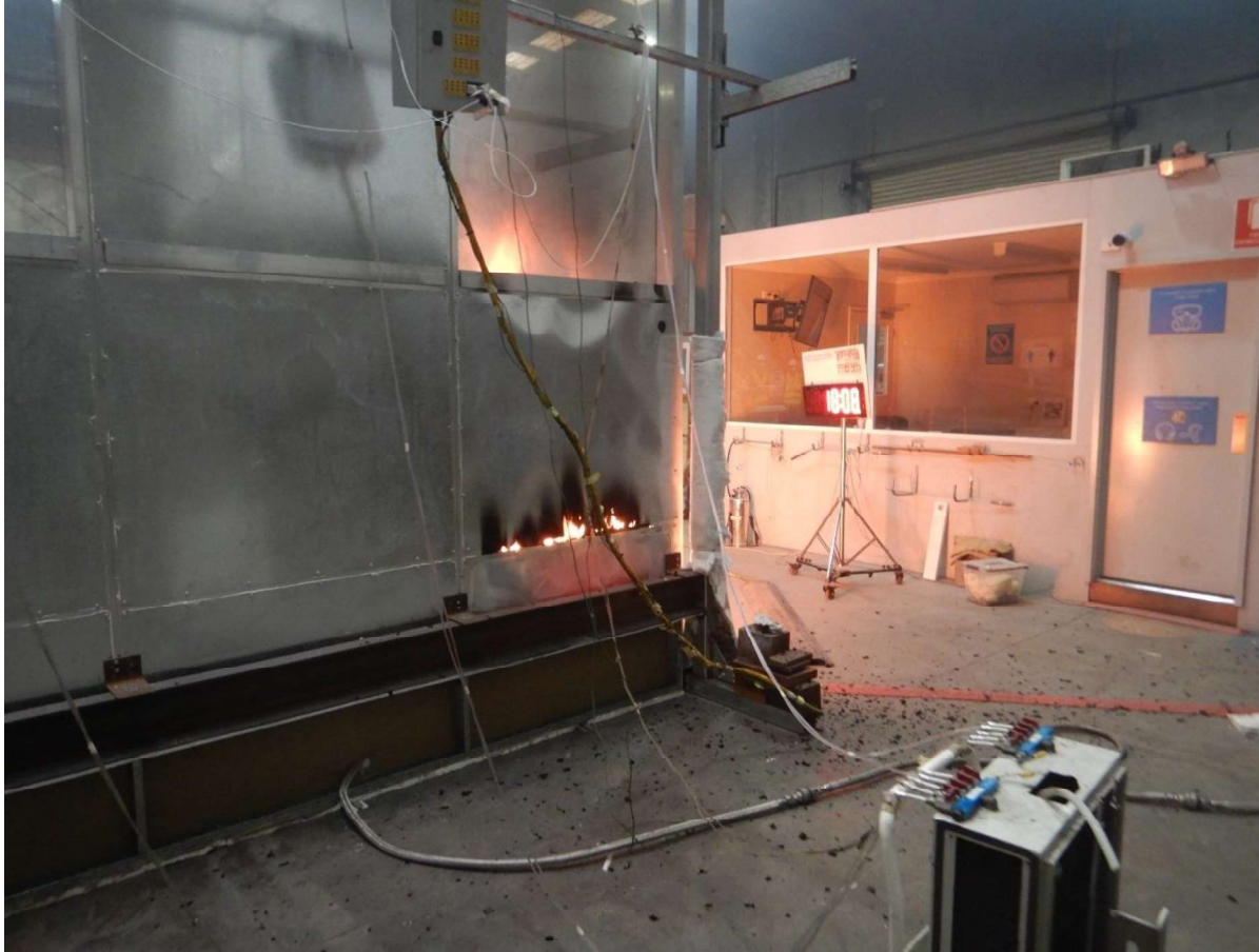
Figure 26 The specimen 18 minutes 8 seconds into the test (burner output at 300 kW) - unexposed side.
