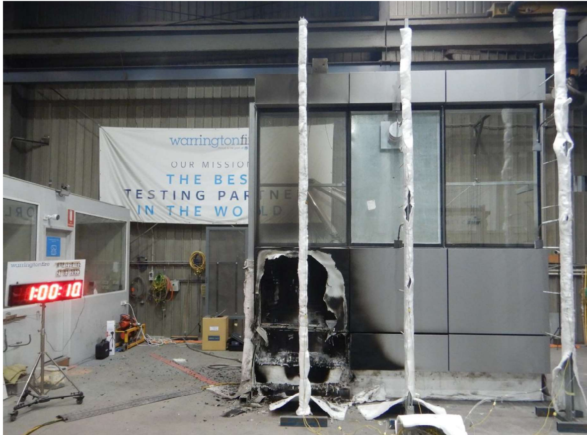
Figure 39 The specimen at end of test – exposed side.
