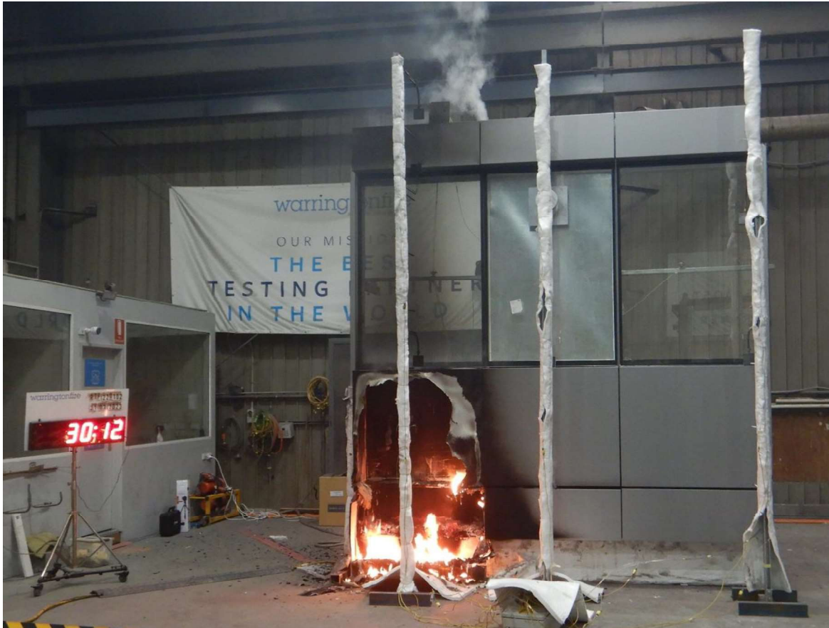
Figure 34 The specimen 30 minutes 12 seconds into the test – just after burner is turned off.
