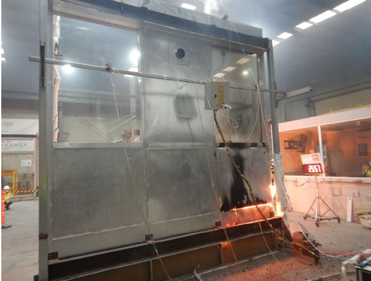
Figure 32 The specimen 25 minutes 57 seconds into the test (burner output at 300 kW) – unexposed side.
