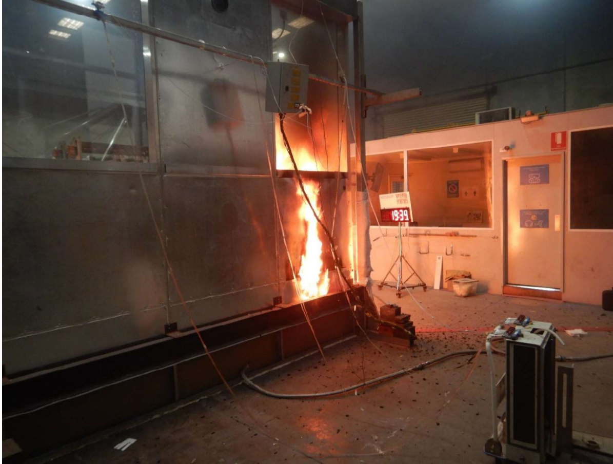
Figure 28 The specimen (unexposed side view) 19 minutes 39 seconds into the test (burner output at 300 kW).
