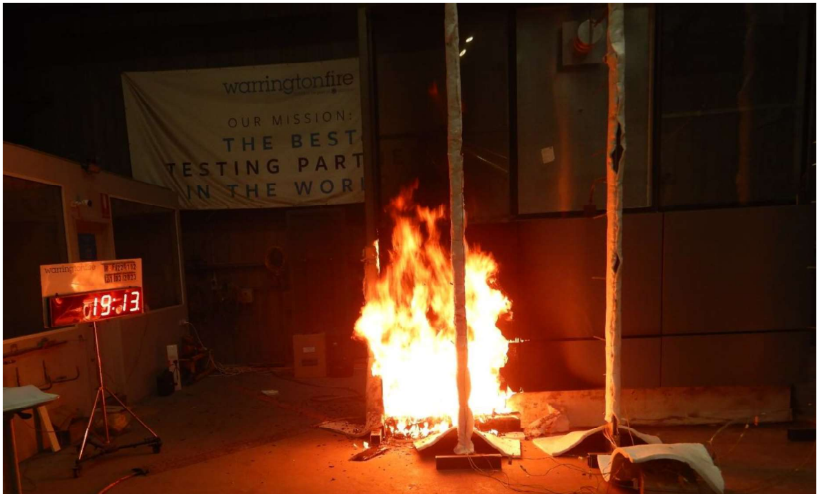
Figure 27 The specimen 20 minutes into the test (burner output at 300 kW).
