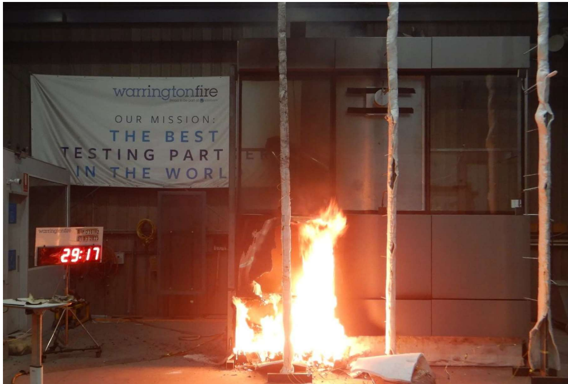
Figure 35 The specimen 29 minutes 17 seconds into the test (burner output at 300 kW).
