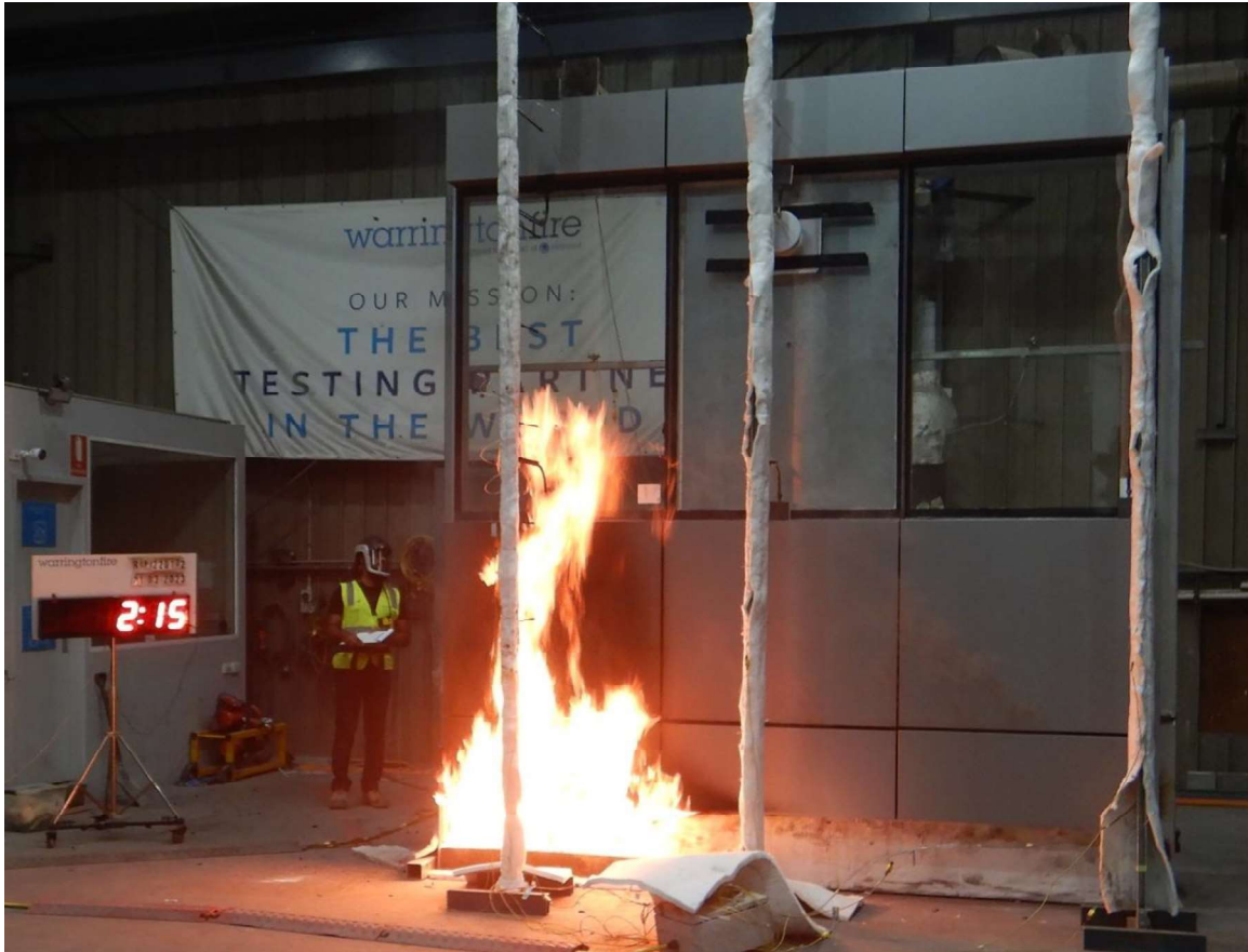
Figure 24 The specimen 2 minutes 14 seconds into the test (burner output at 300 kW)
