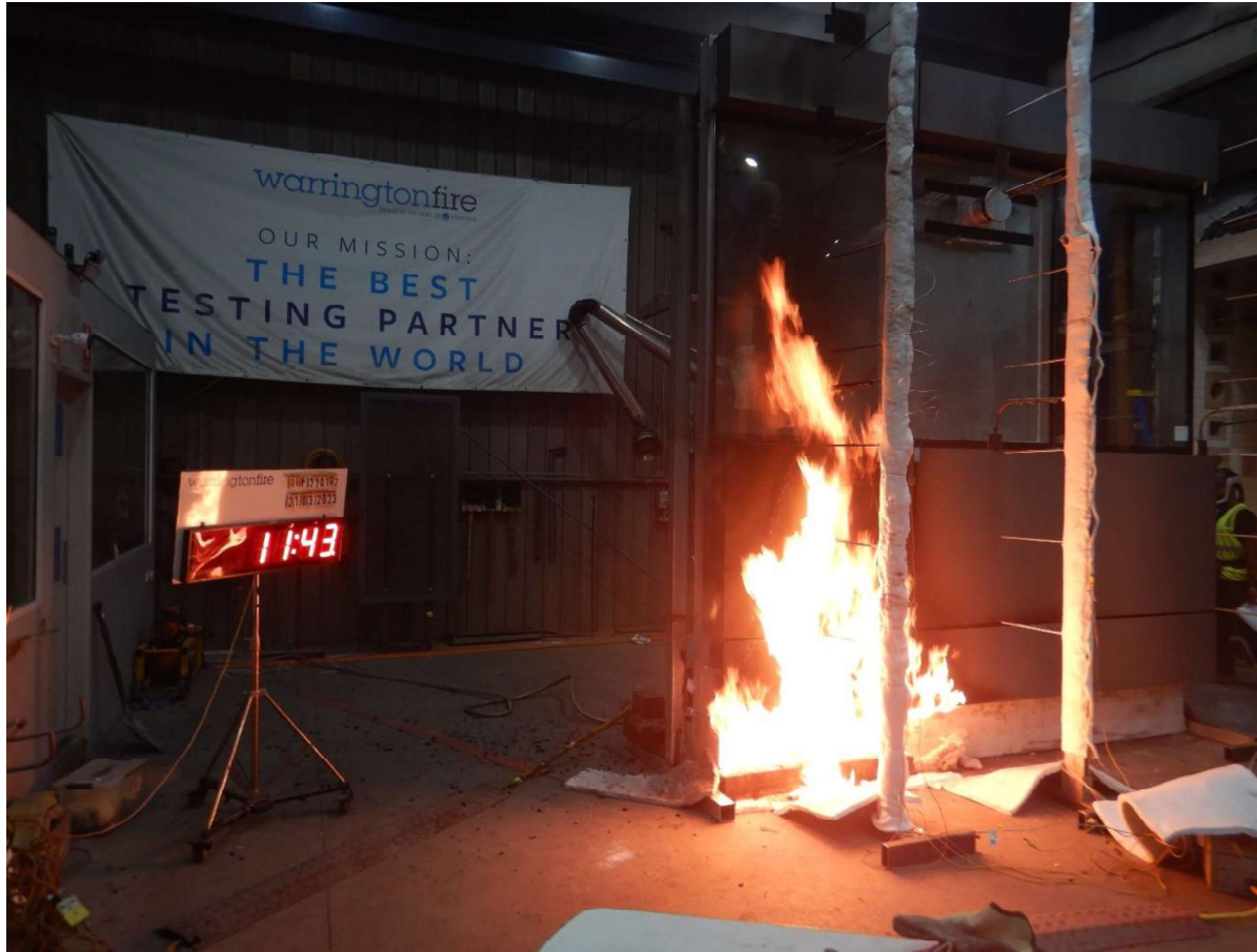
Figure 25 The specimen 11 minutes 43 seconds into the test (burner output at 300 kW)
