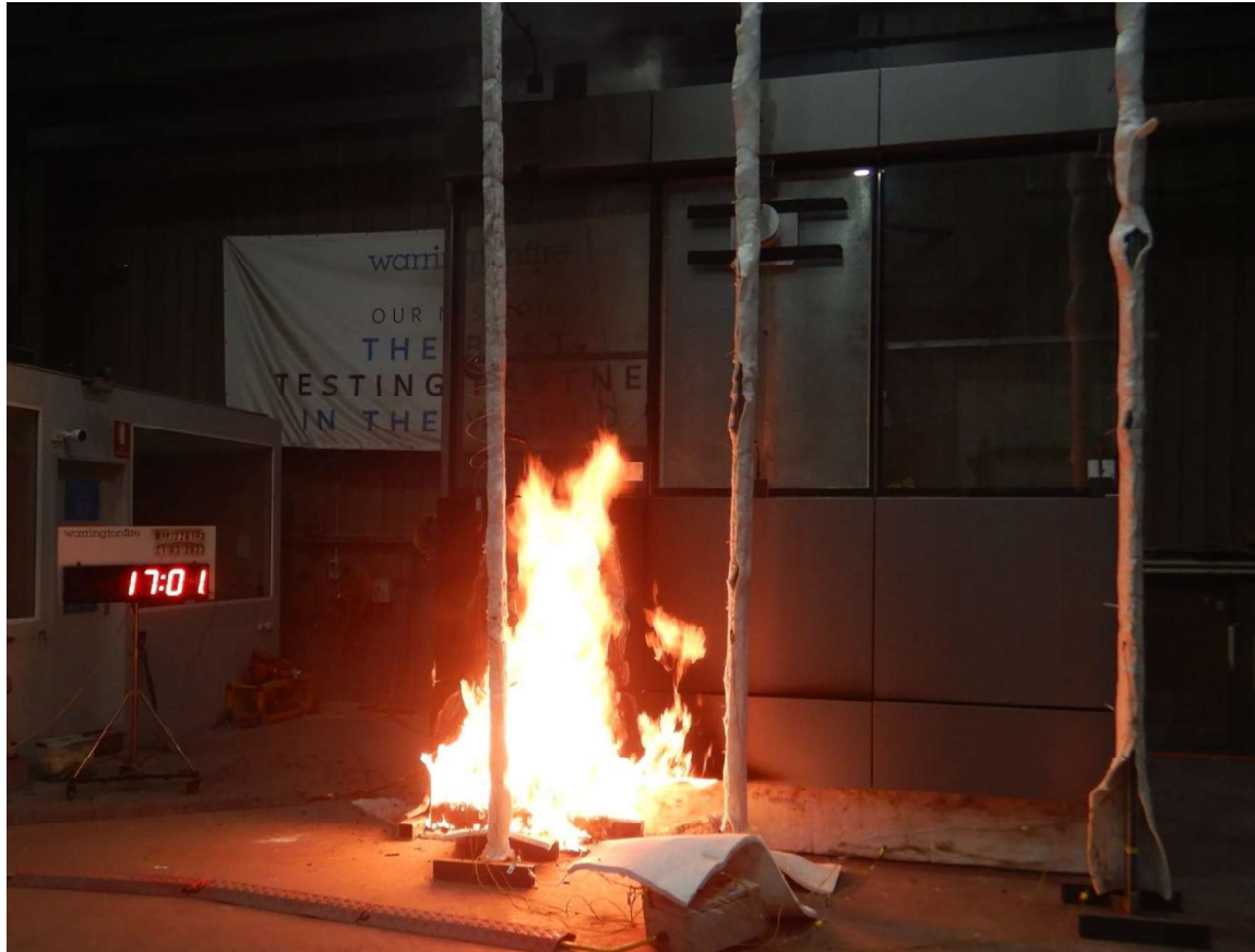
Figure 27 The specimen 17 minutes 1 second into the test (burner output at 300 kW)
