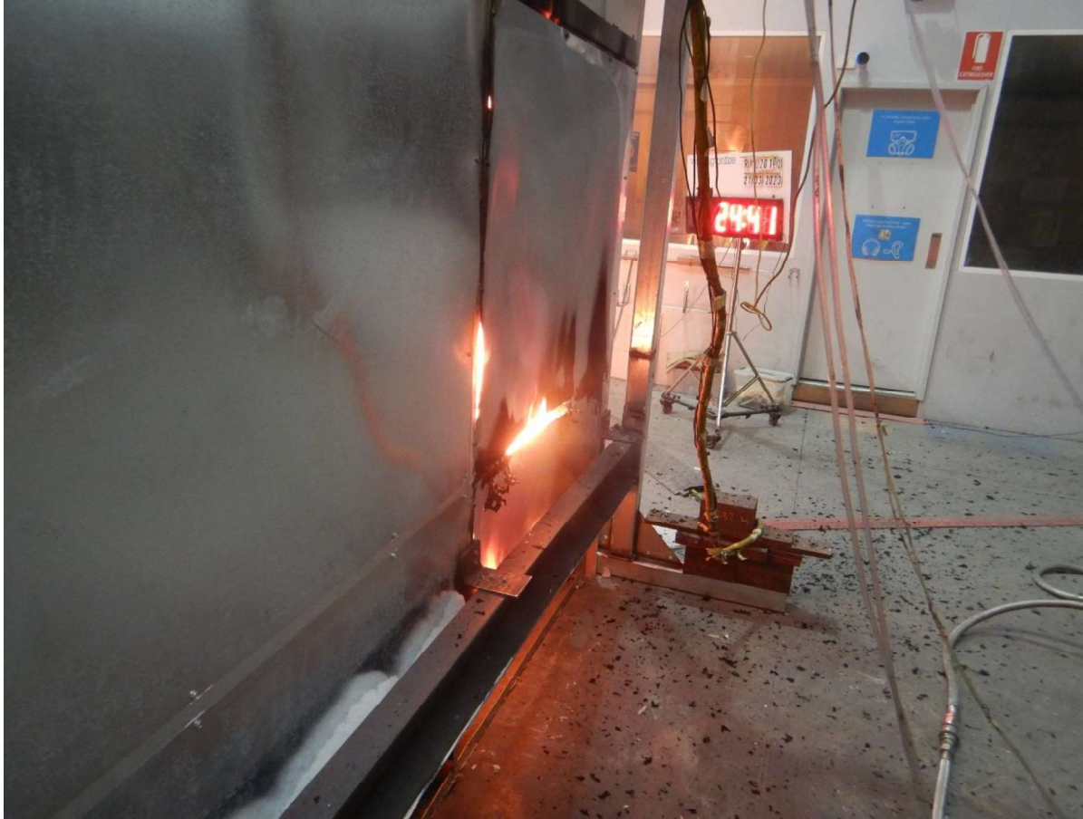
Figure 33 The specimen 24 minutes 41 seconds into the test (burner output at 300 kW) – unexposed side.
