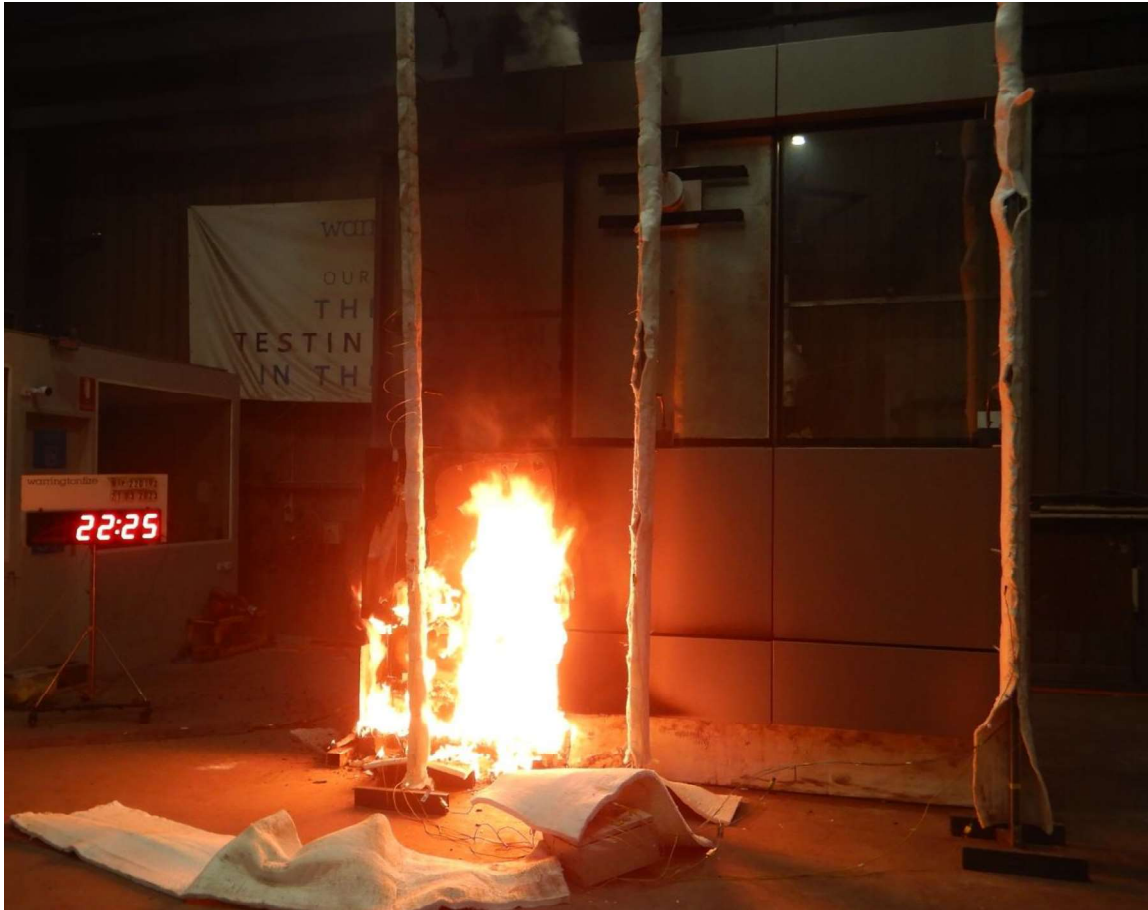
Figure 32 The specimen 22 minutes 25 seconds into the test (burner output at 300 kW).
