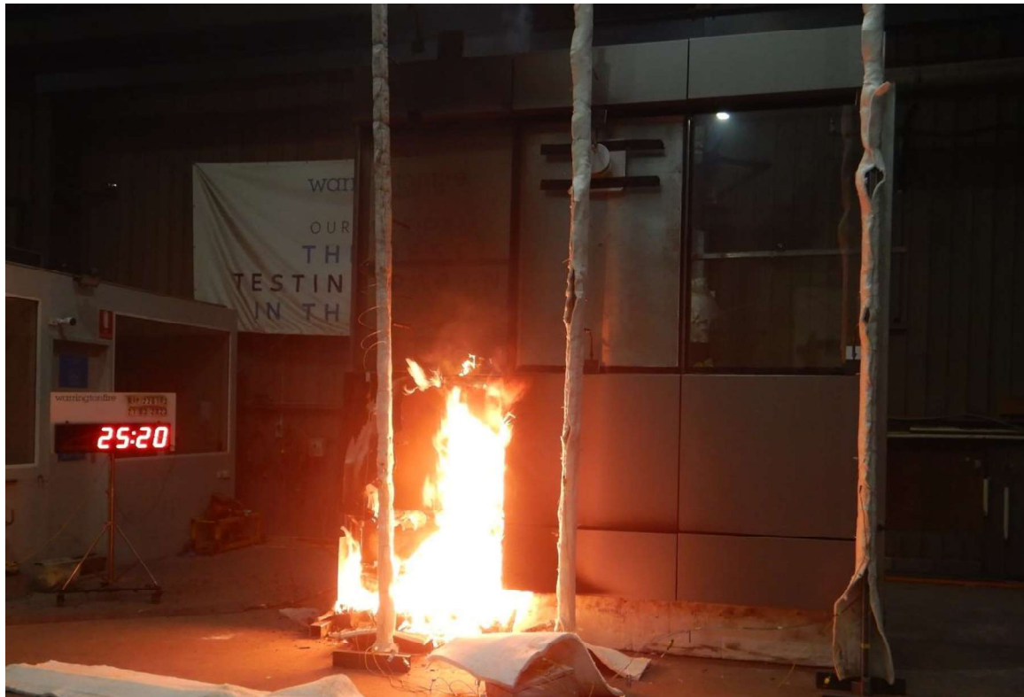
Figure 34 The specimen 25 minutes 20 seconds into the test (burner output at 300 kW) – unexposed side.
