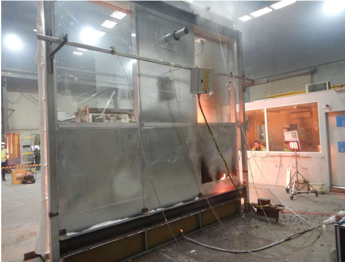
Figure 28 The specimen 17 minutes 17 seconds into the test (burner output at 300 kW) – unexposed side.
