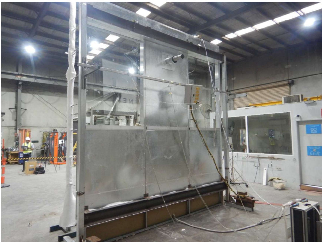
Figure 21 The specimen (unexposed side) before the reaction to fire test
