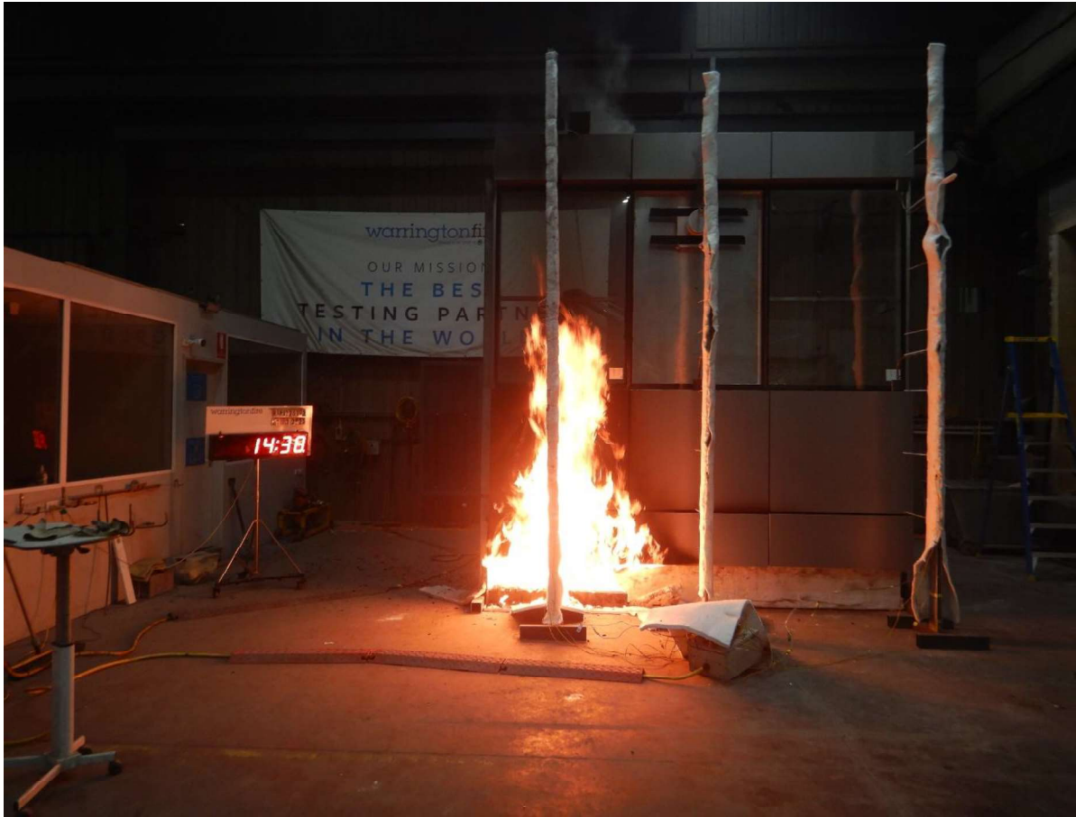
Figure 26 The specimen 14 minutes 38 seconds into the test (burner output at 300 kW)
