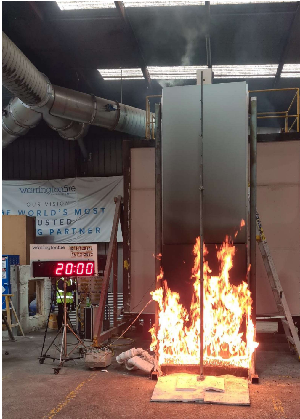
Figure 13 The specimen 20 minutes into the test (5 minutes after burner output was increased to 300 kW)
