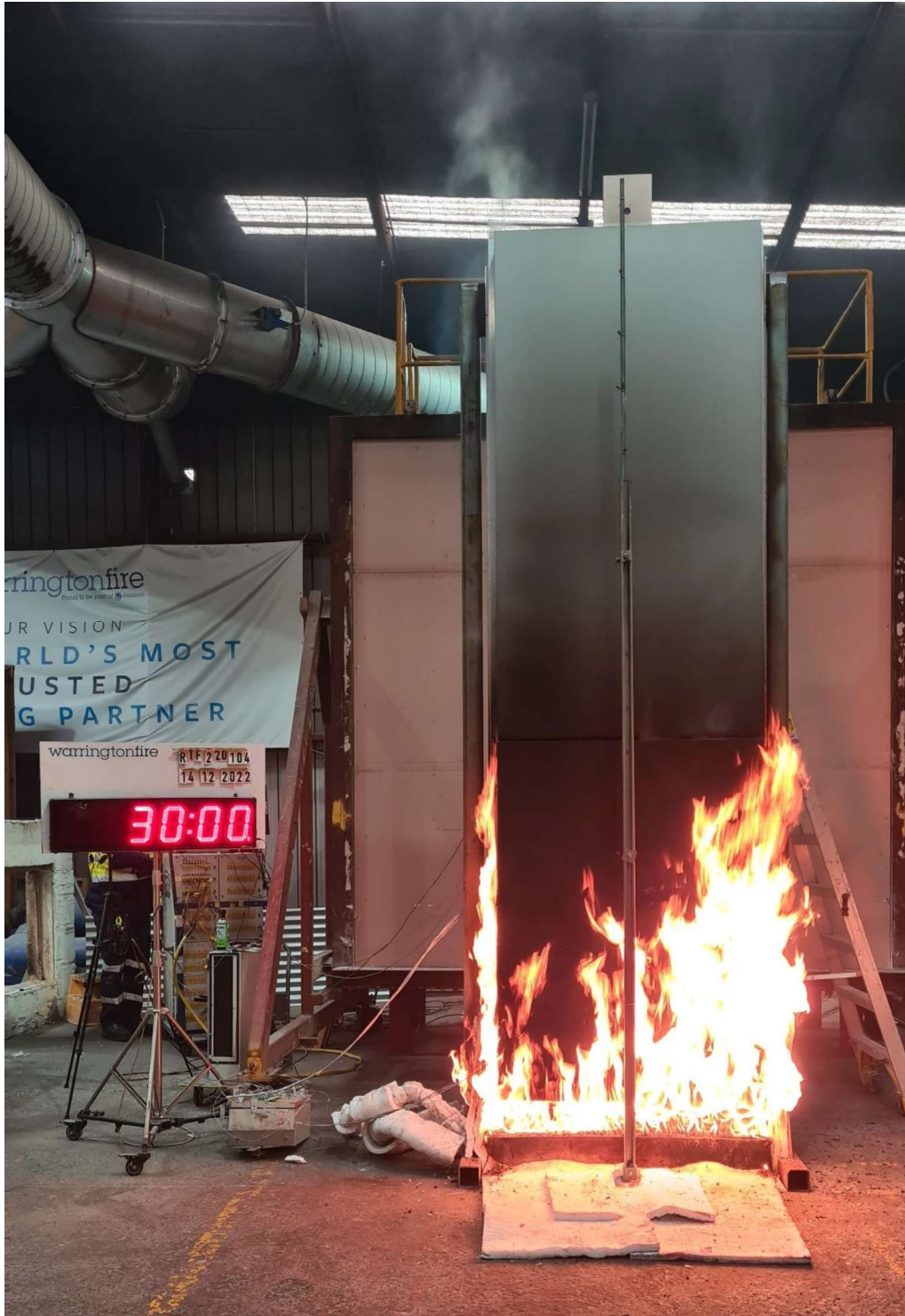
Figure 14 The specimen 30 minutes into the test (15 minutes after burner output was increased to 300 kW)
