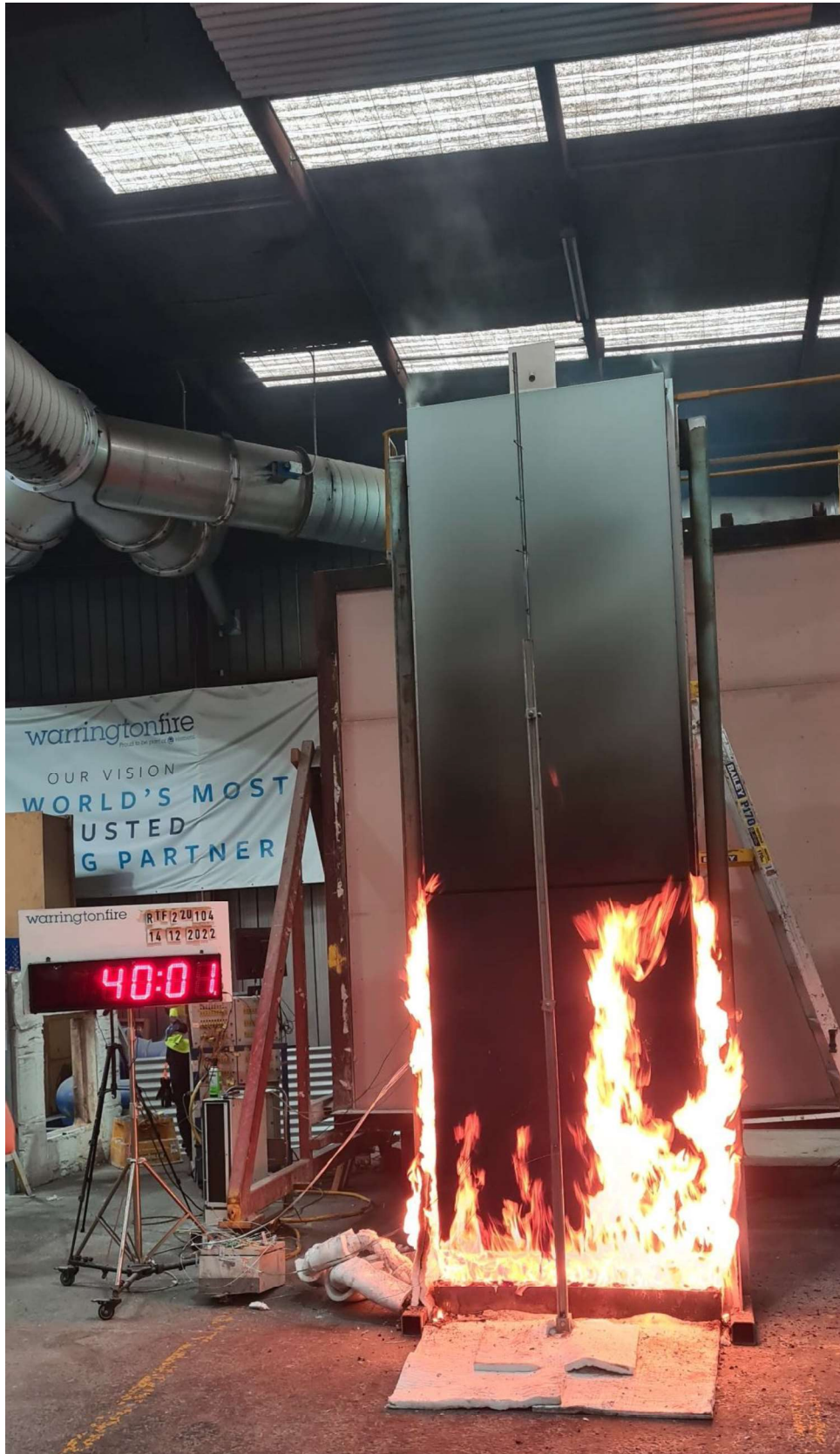
Figure 15 The specimen 40 minutes 1 second into the test (25 minutes 1 second after burner output was increased to 300 kW) – burner turned off.
