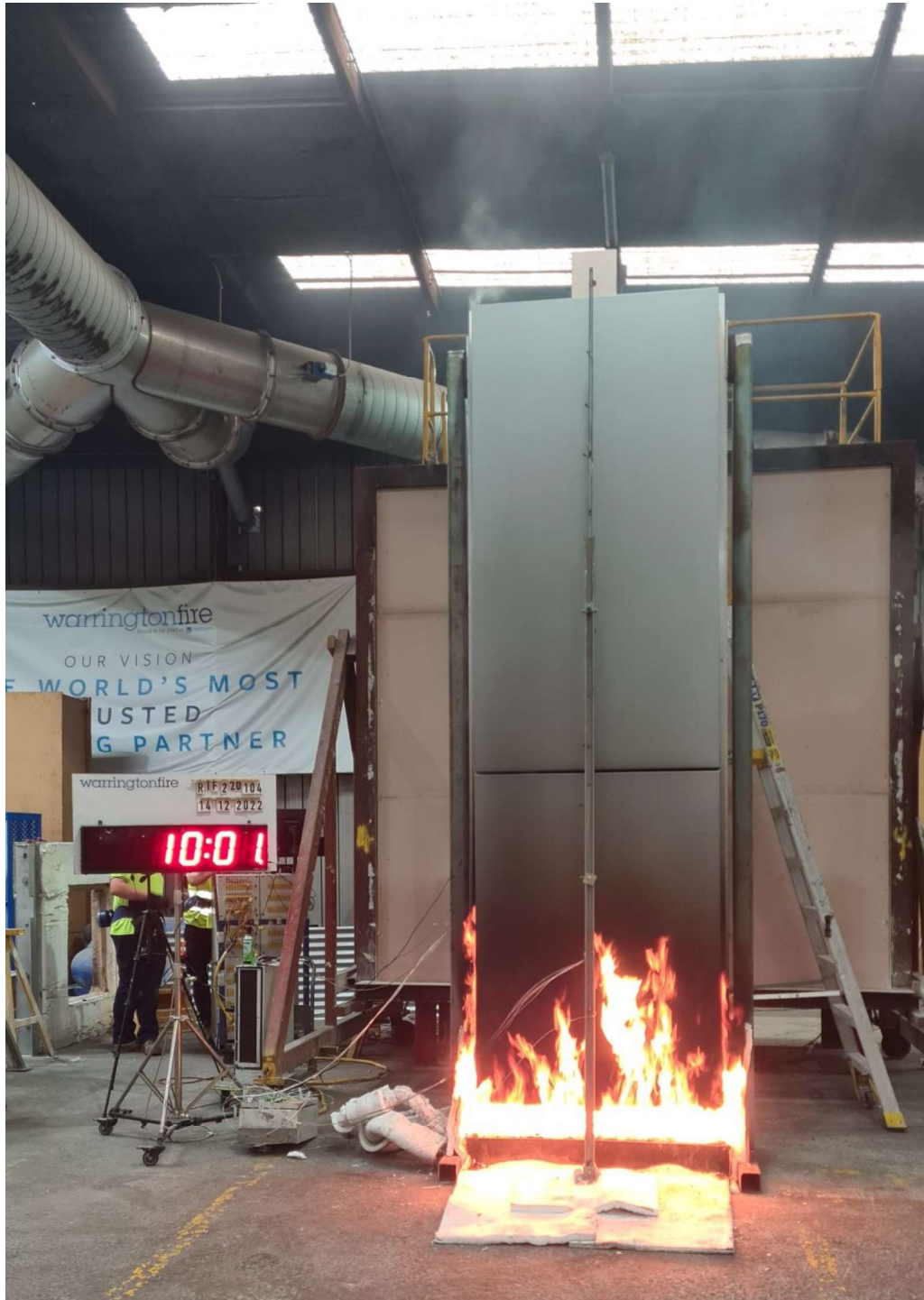
Figure 11 The specimen 10 minutes 1 second into the test (burner output at 100 kW)
