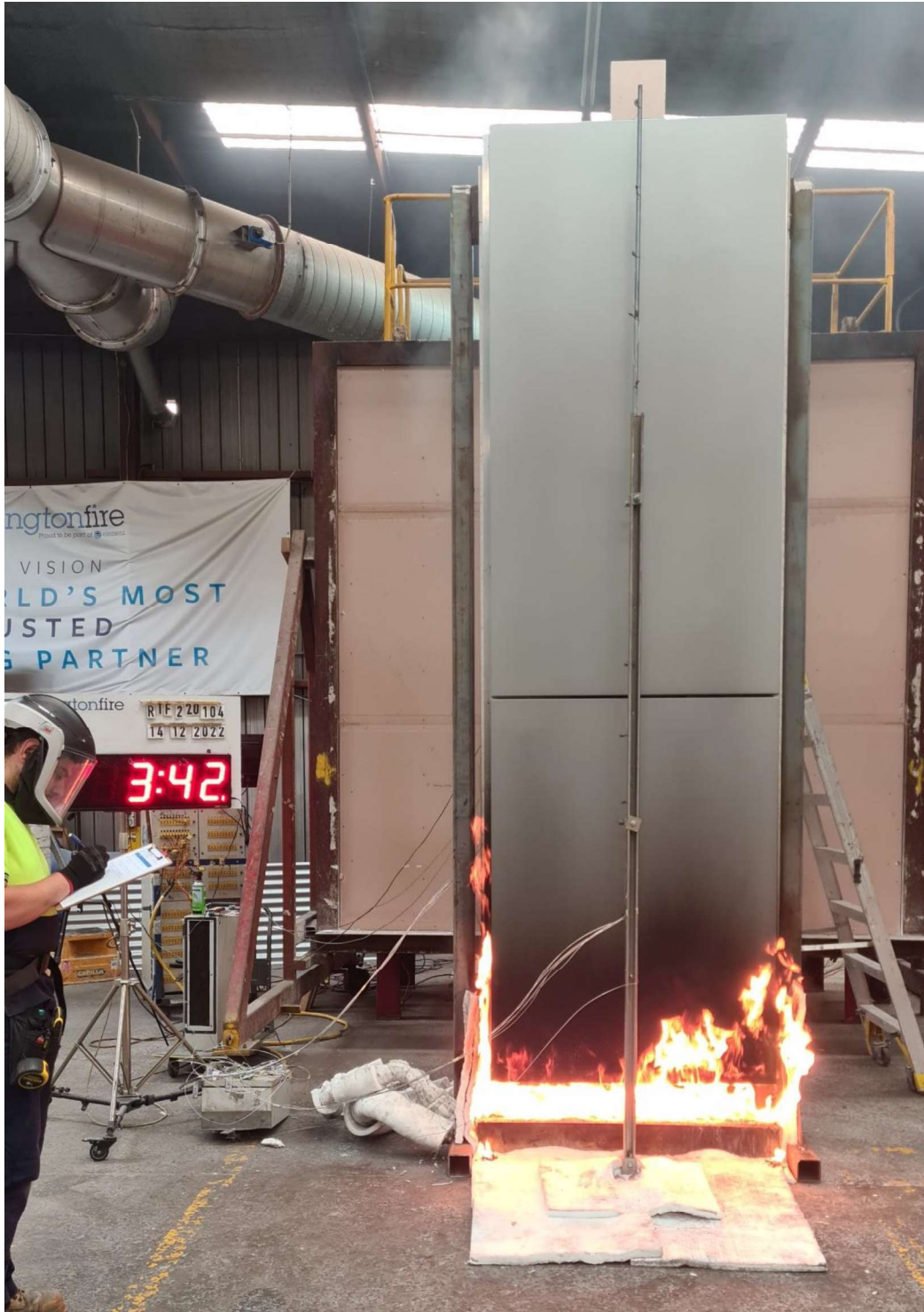
Figure 10 The specimen 3 minutes 42 seconds into the test (burner output at 100 kW)
