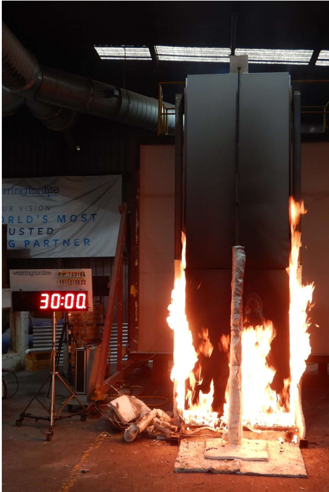
Figure 13 The specimen 30 minutes into the test (15 minutes after burner output was increased to 300 kW)
