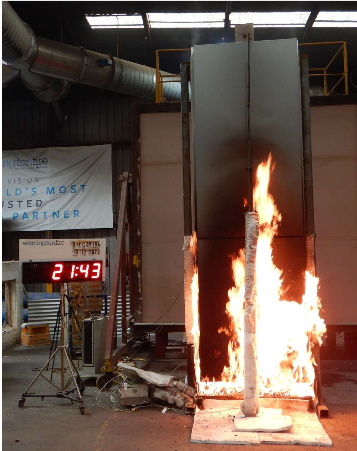
Figure 13 The specimen 21 minutes 43 seconds into the test (6 minutes 43 seconds after burner output was increased to 300 kW)
