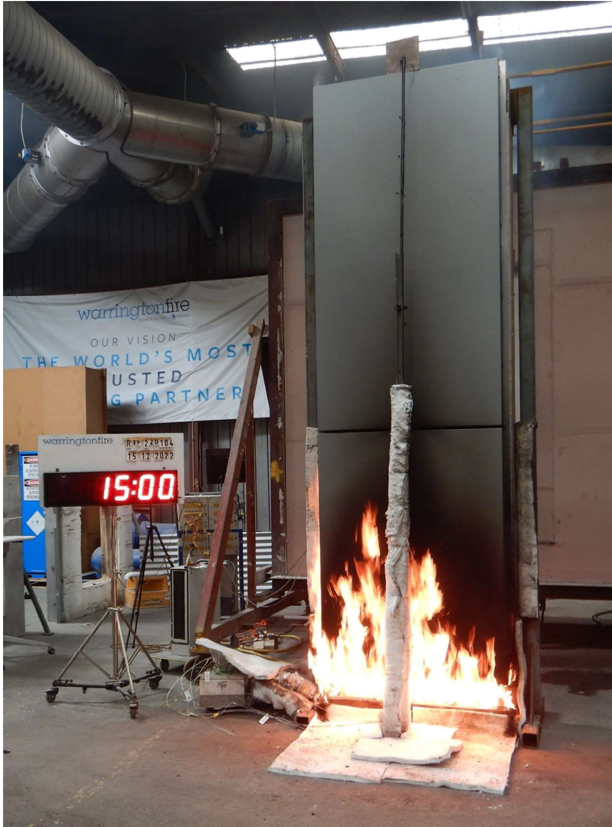
Figure 12 The specimen 15 minutes into the test (burner output at 100 kW changed to 300 kW)
