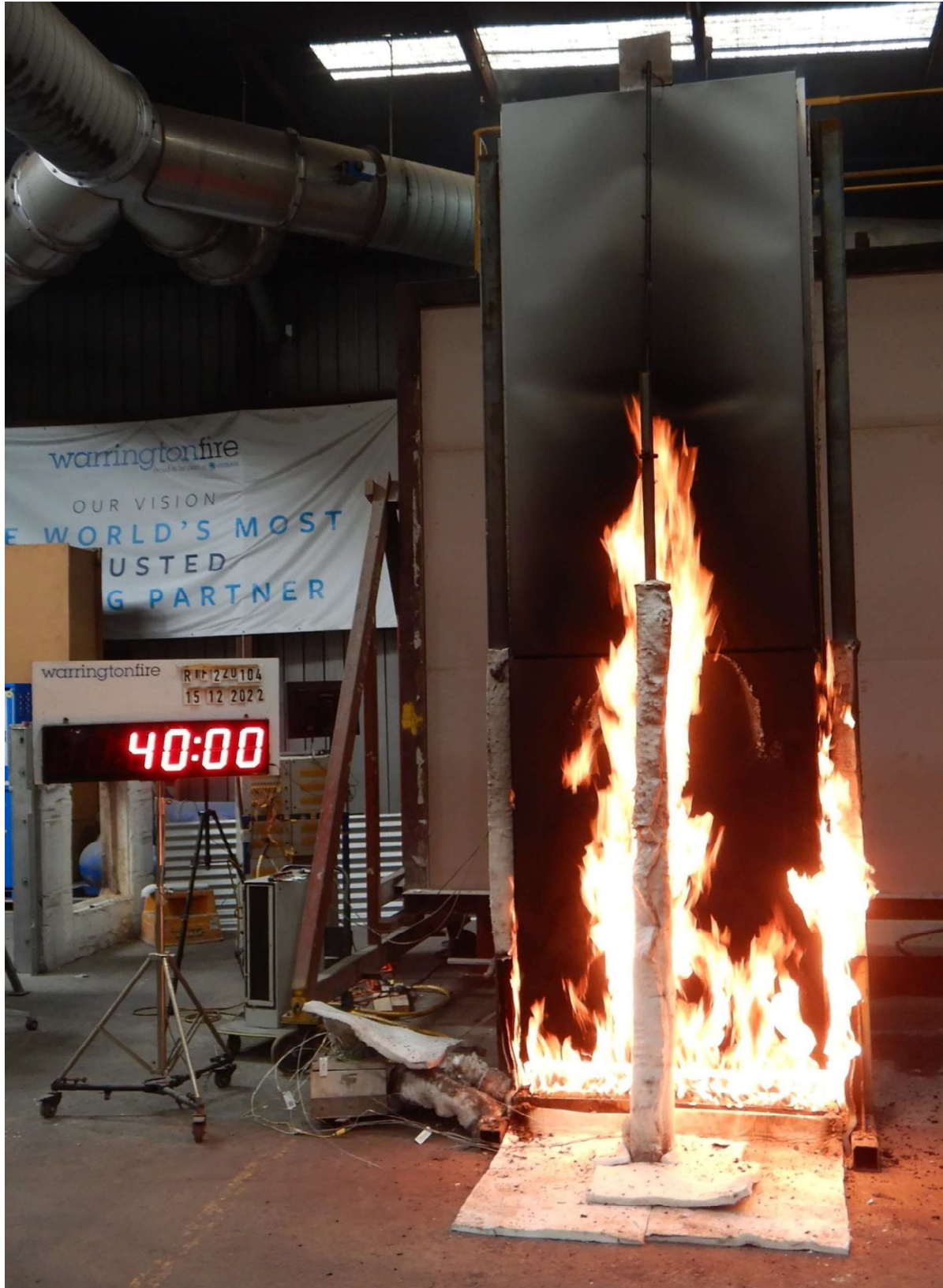
Figure 15 The specimen 40 minutes into the test (25 minutes after burner output was increased to 300 kW) – burner turned off.
