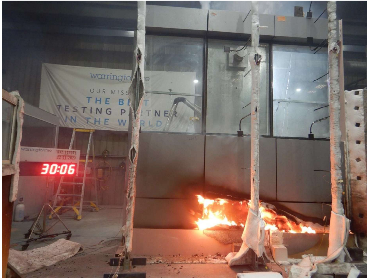
Figure 50 The specimen 30 minutes 6 seconds into the test – just after burner is turned off.
