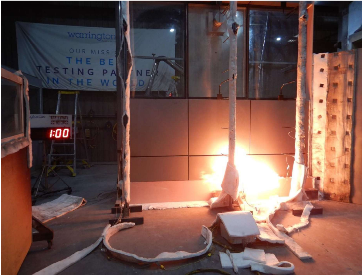
Figure 32 The specimen 1 minute into the test (burner output at 300 kW and wind on)
