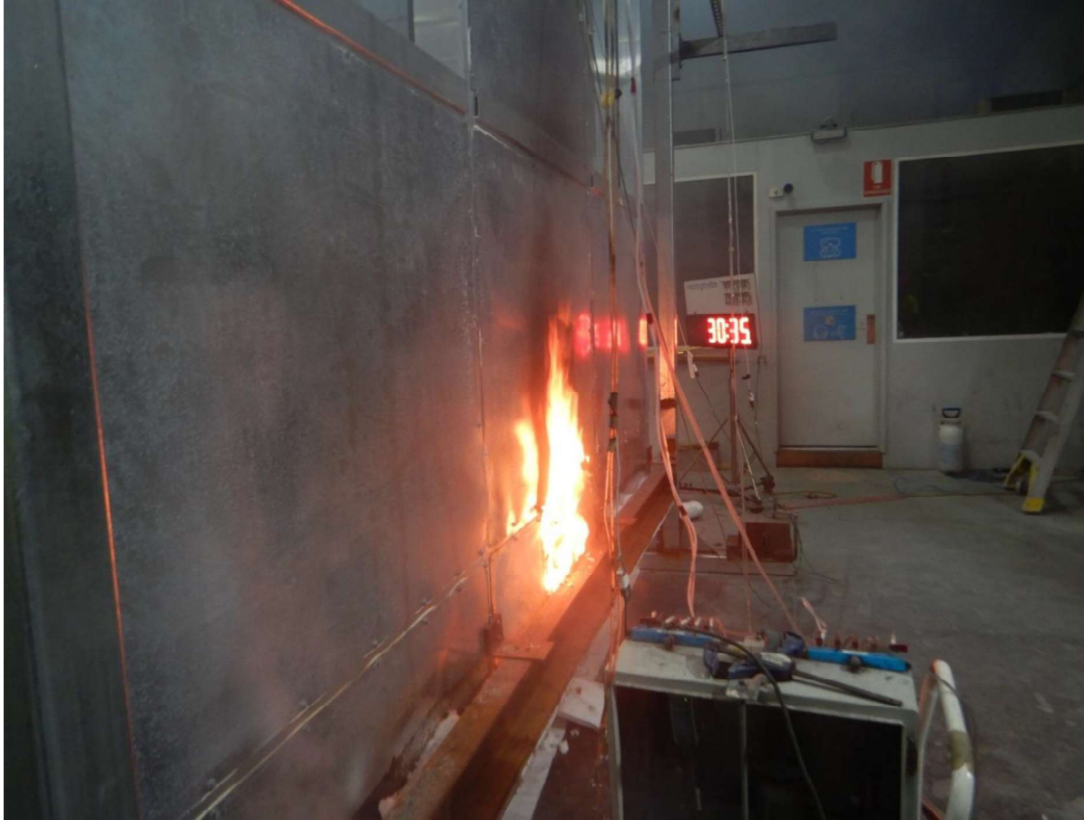
Figure 52 The specimen 30 minutes 35 seconds into the test –burner off – unexposed side.
