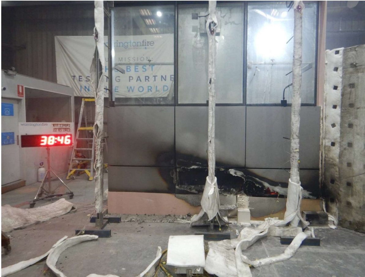
Figure 54 The specimen 38 minutes 46 seconds into the test (burner off).
