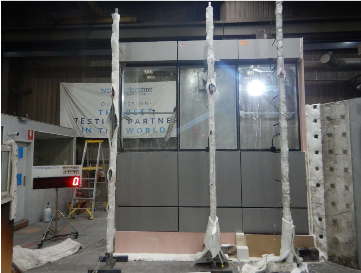
Figure 30 The specimen before the reaction to fire test - exposed side.
