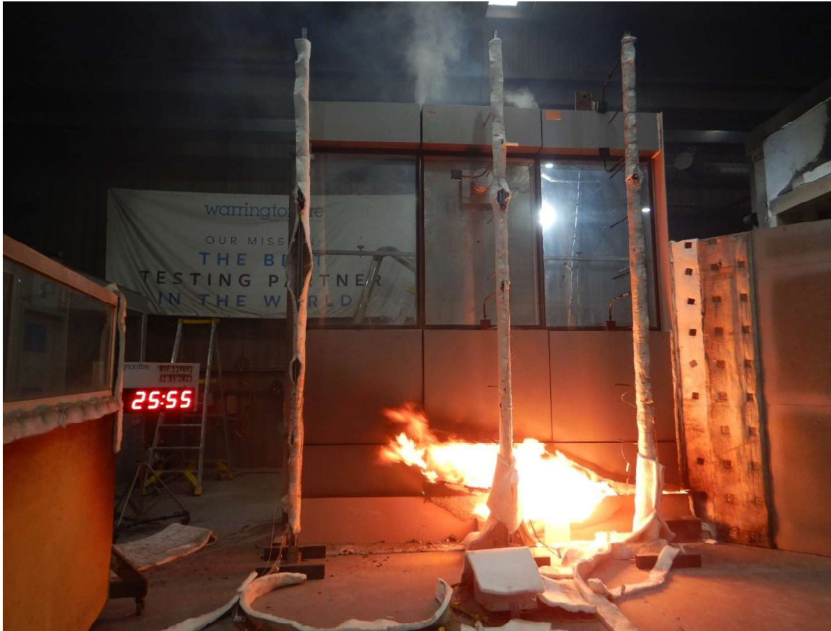
Figure 41 The specimen 25 minutes 55 seconds into the test (burner output at 300 kW and wind on).
