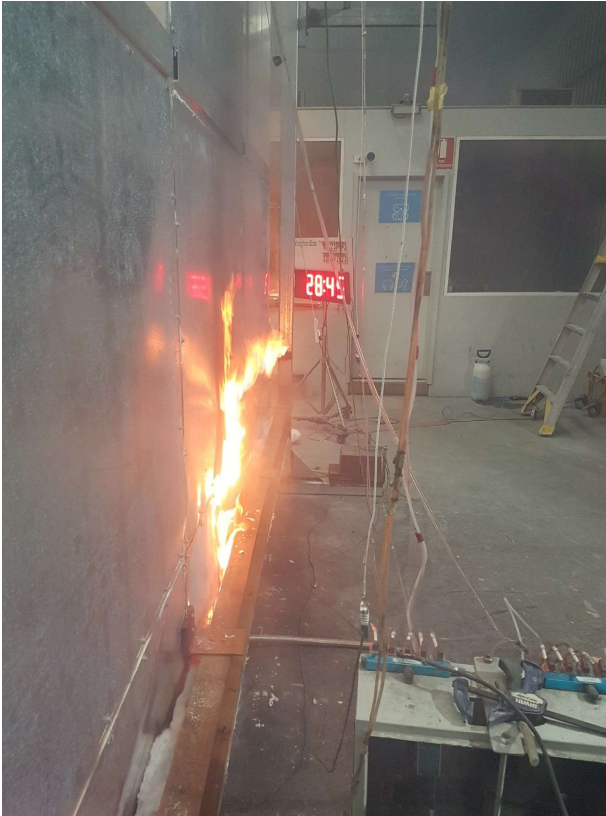
Figure 47 The specimen 28 minutes 45 seconds into the test (burner output at 300 kW and wind on) – unexposed side.
