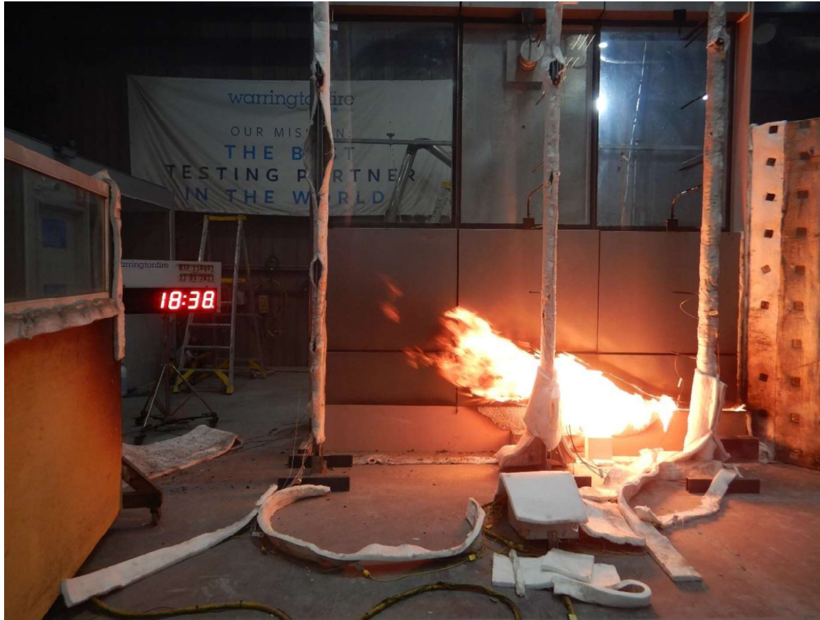
Figure 38 The specimen 18 minutes 38 seconds into the test (burner output at 300 kW and wind on).
