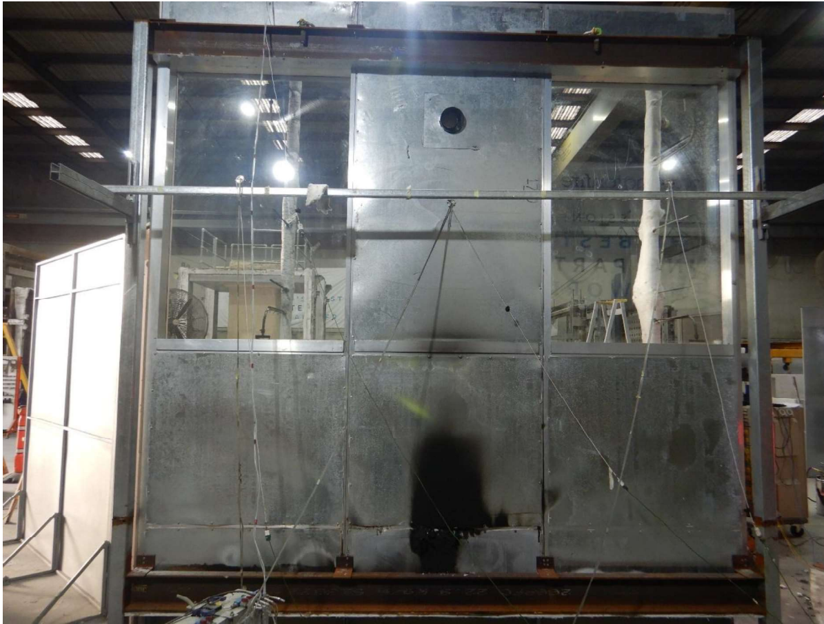
Figure 57 The specimen at the end of test – unexposed side.
