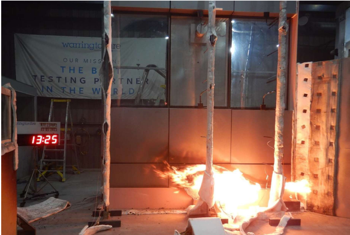
Figure 36 The specimen 13 minutes 25 seconds into the test (burner output at 300 kW and wind on).
