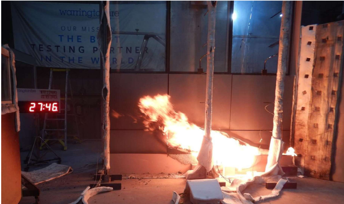
Figure 45 The specimen 27 minutes 46 seconds into the test (burner output at 300 kW and wind on).
