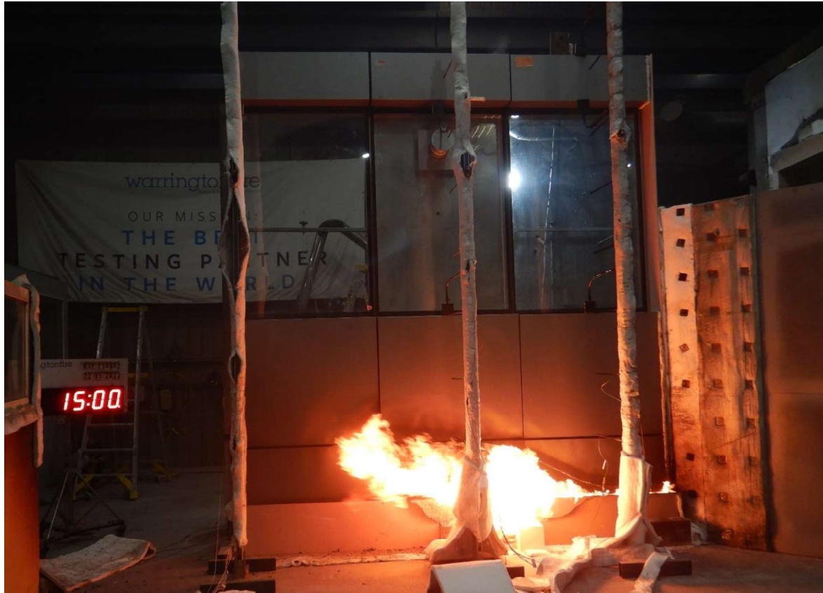
Figure 37 The specimen 15 minutes into the test (burner output at 300 kW and wind on).
