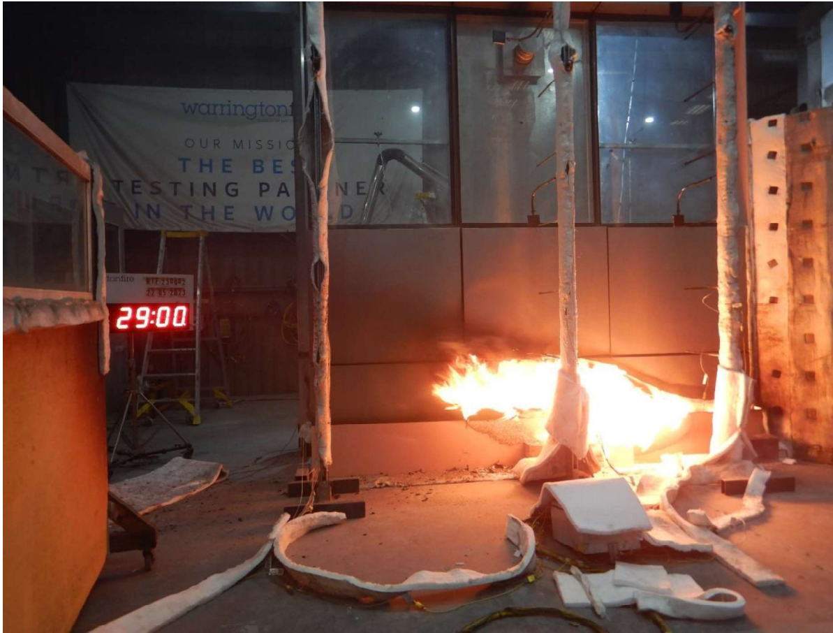
Figure 48 The specimen 29 minutes into the test (burner output at 300 kW and wind on).
