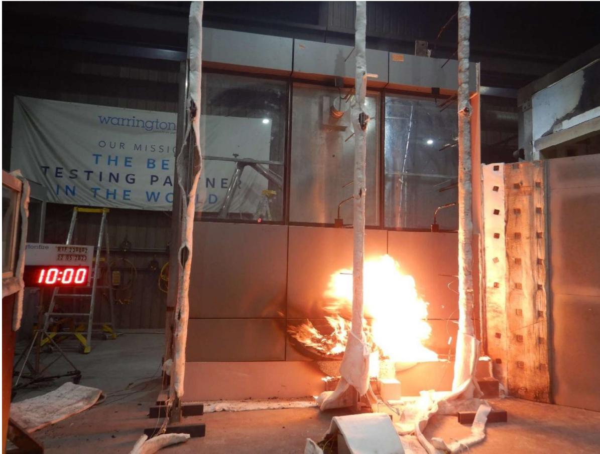
Figure 35 The specimen 10 minutes into the test (burner output at 300 kW and wind on)
