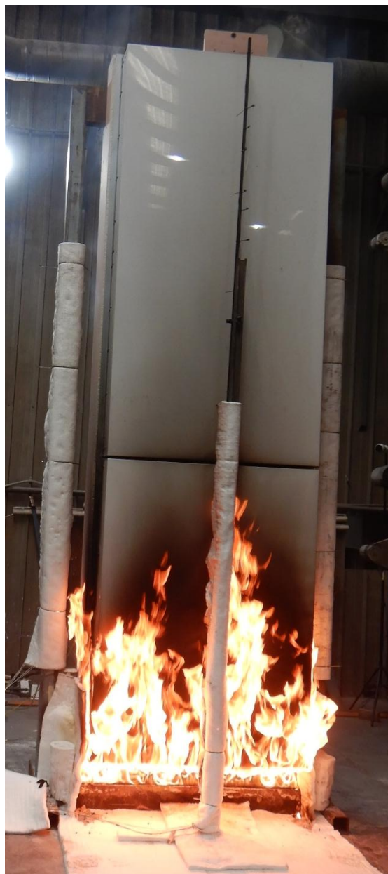
Figure 18 The specimen 15 minutes 2 seconds into the test (2 seconds after burner output was changed to 300 kW)
