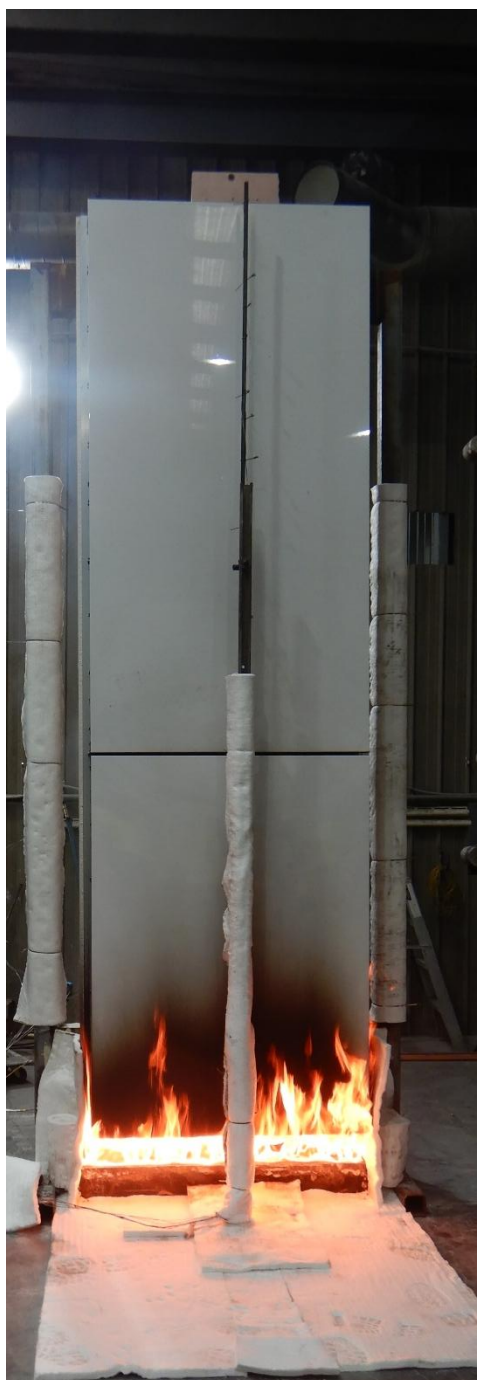
Figure 12 The specimen 1 minute 42 seconds into the test (burner output at 100 kW)
