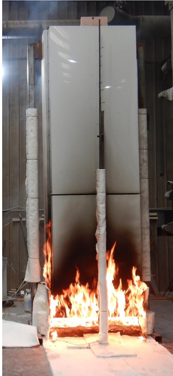
Figure 15 The specimen 9 minutes 53 seconds into the test (burner output at 100 kW)
