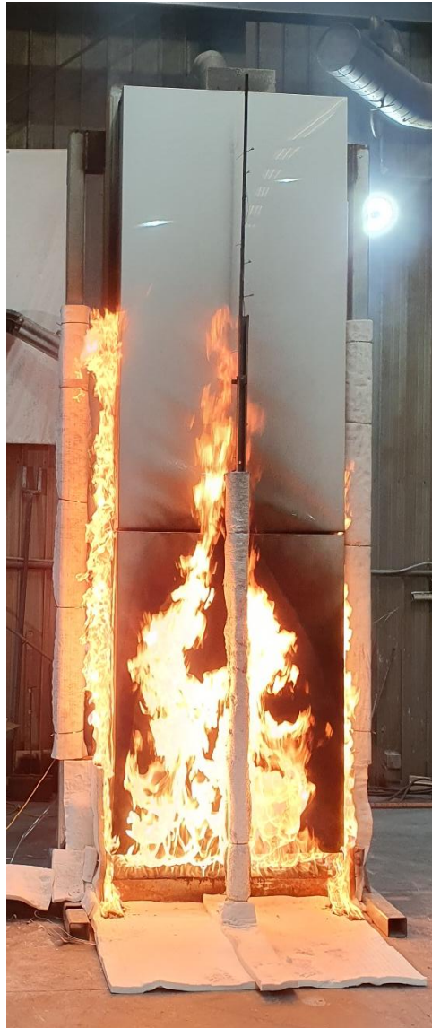
Figure 14 The specimen 9 minutes 20 seconds into the test (burner output at 200 kW)
