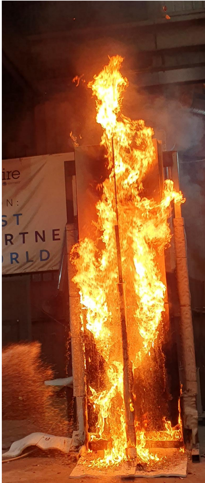
Figure 23 The specimen 20 minutes 51 seconds into the test (burner output at 200 kW) – at test termination.
