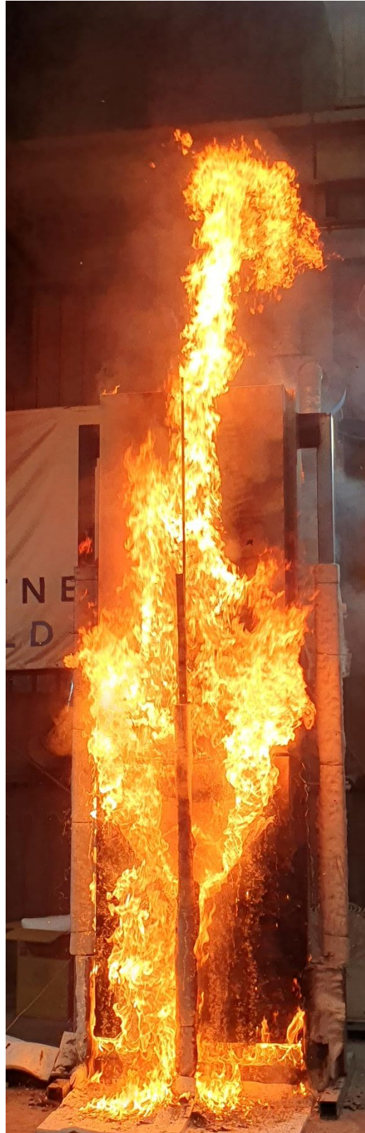
Figure 22 The specimen 20 minutes 47 seconds into the test (burner output at 200 kW)
