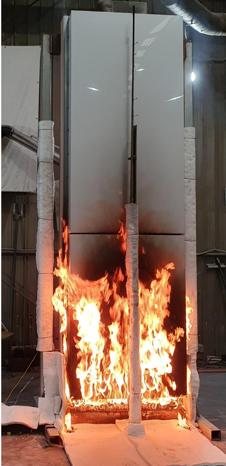
Figure 13 The specimen 6 minutes 7 seconds into the test (burner output at 200 kW)
