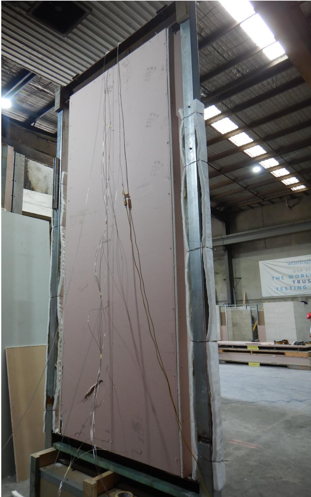
Figure 11 The specimen before the reaction to fire test – unexposed side
