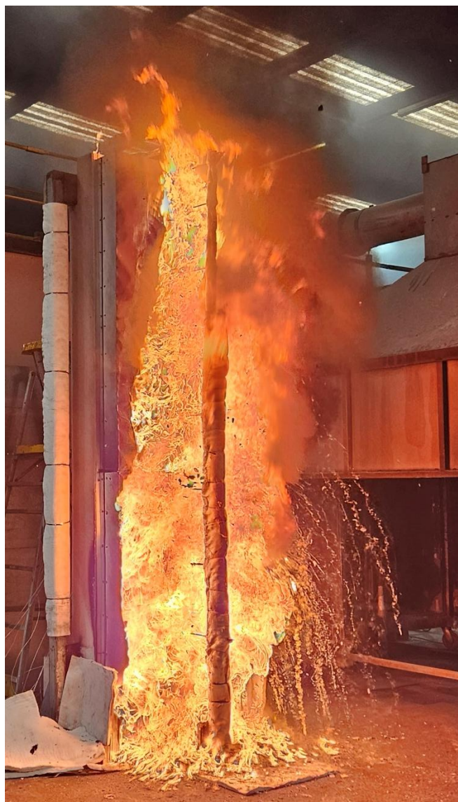
Figure 21 The specimen 6 minutes 46 seconds into the test (burner output at 200 kW) – 2 seconds before end of test.
