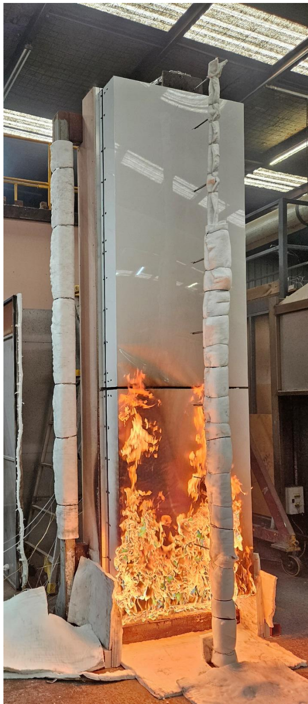
Figure 16 The specimen 5 minutes into the test (burner output at 200 kW)
