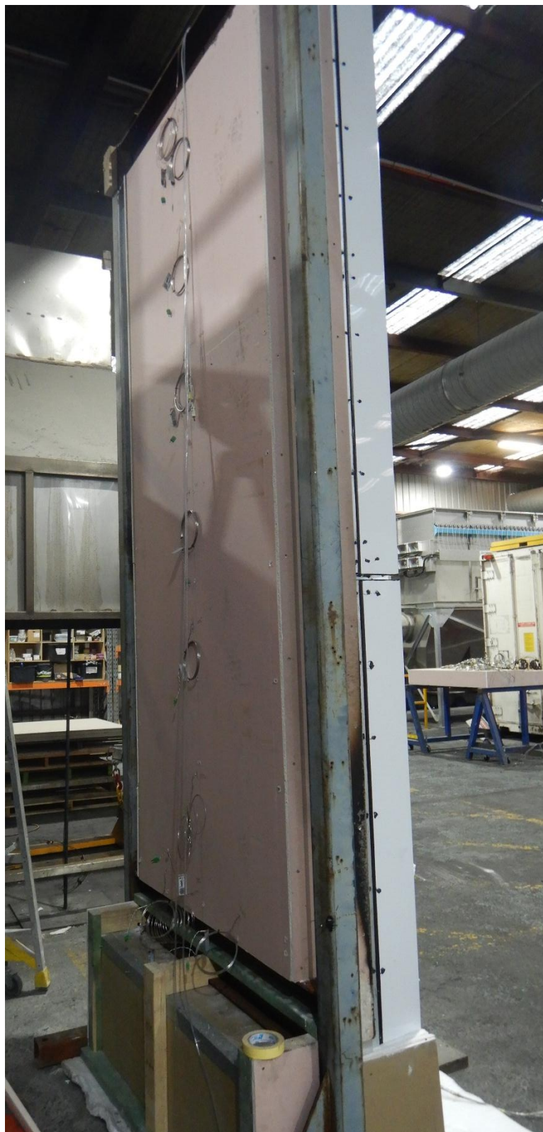
Figure 11 The specimen before the reaction to fire test – unexposed side
