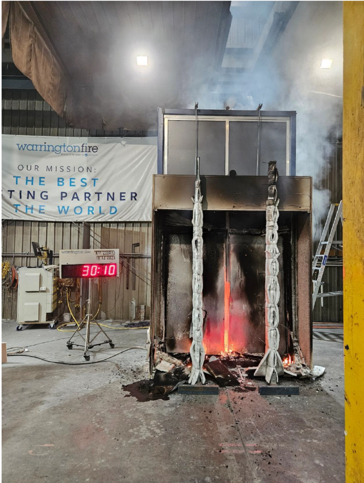
Figure 26 The specimen 10 seconds after the burner was turned off (30 minutes 10 seconds into the test)
