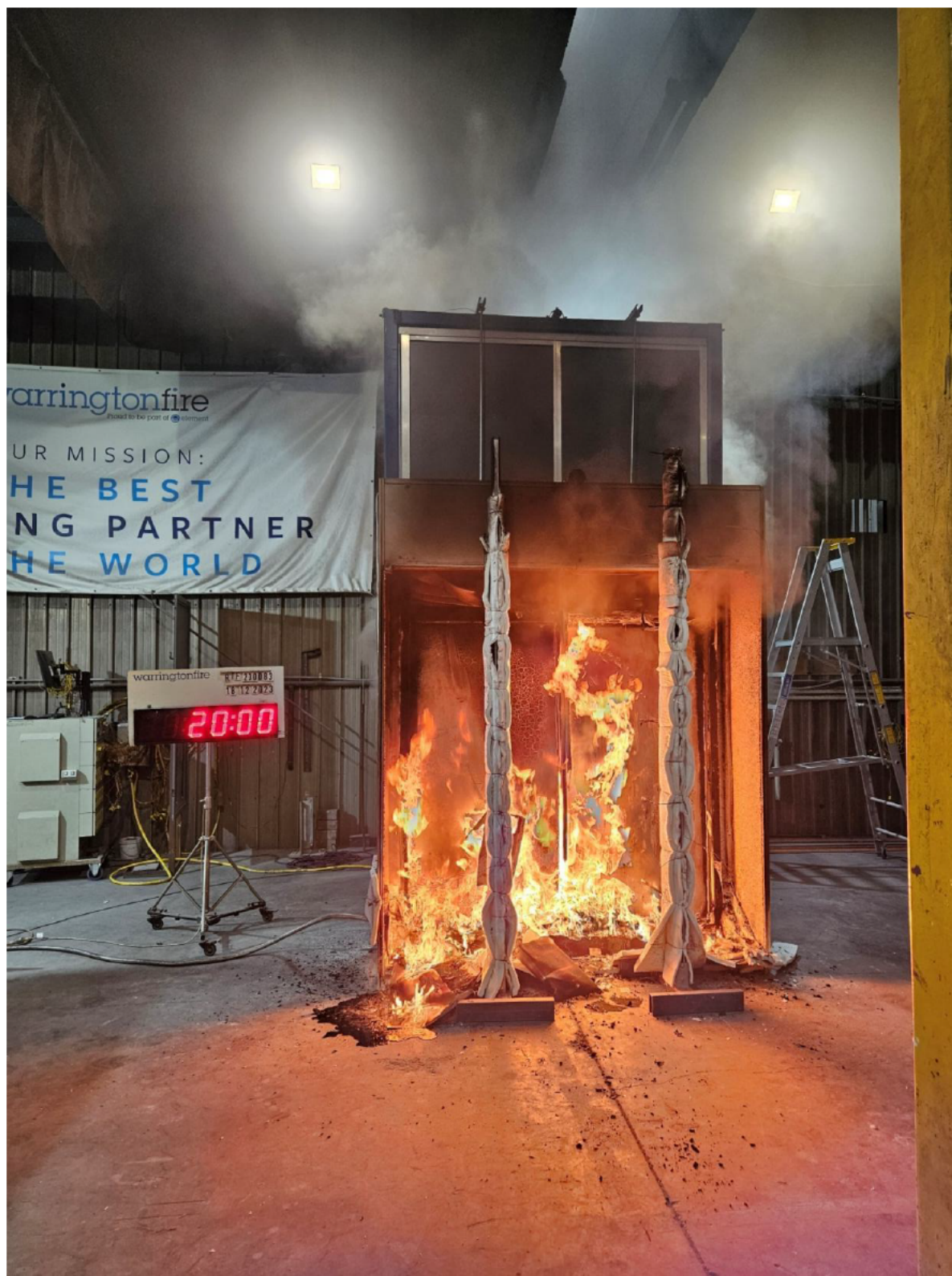
Figure 24 The specimen 20 minutes into the test
