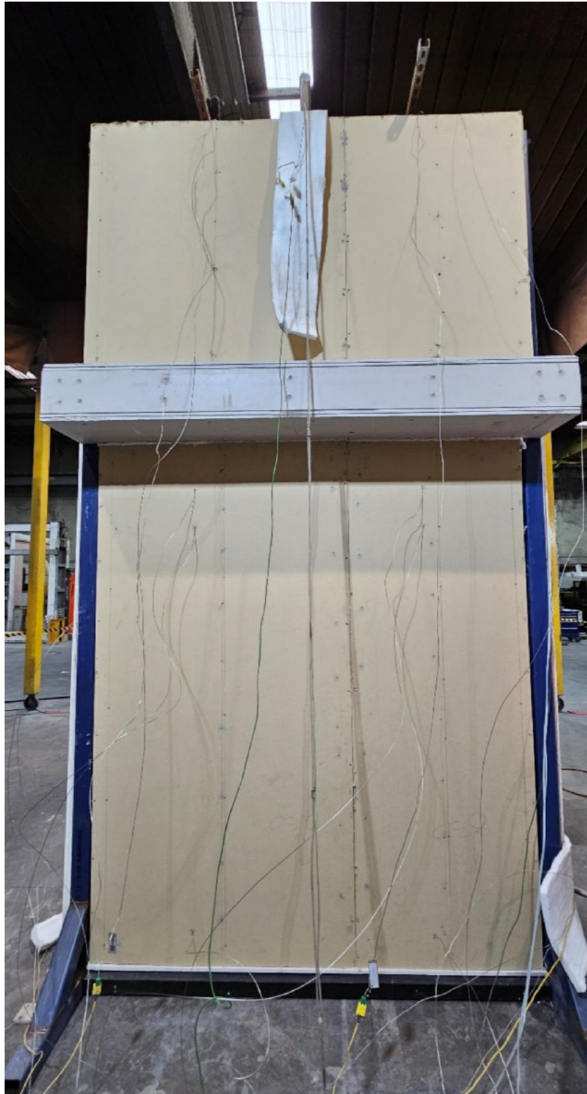
Figure 19 The specimen before the reaction to fire test – unexposed side
