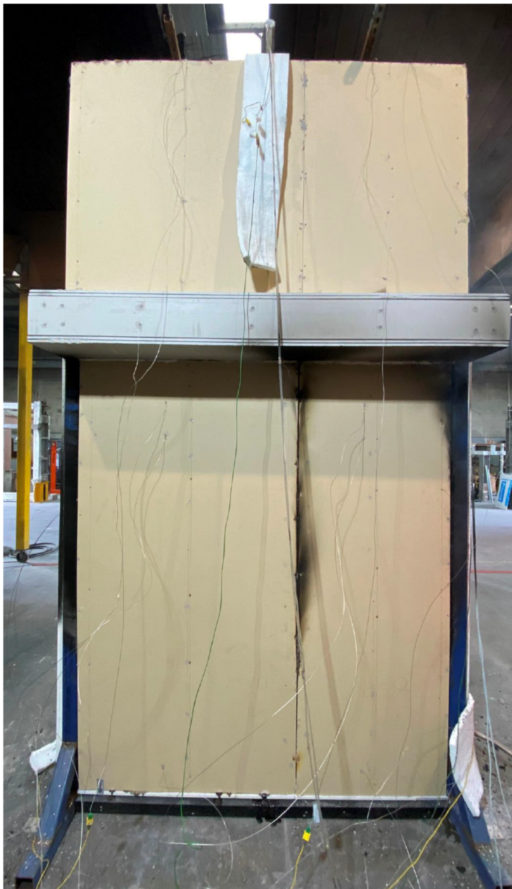
Figure 28 The specimen after the test – unexposed side.
