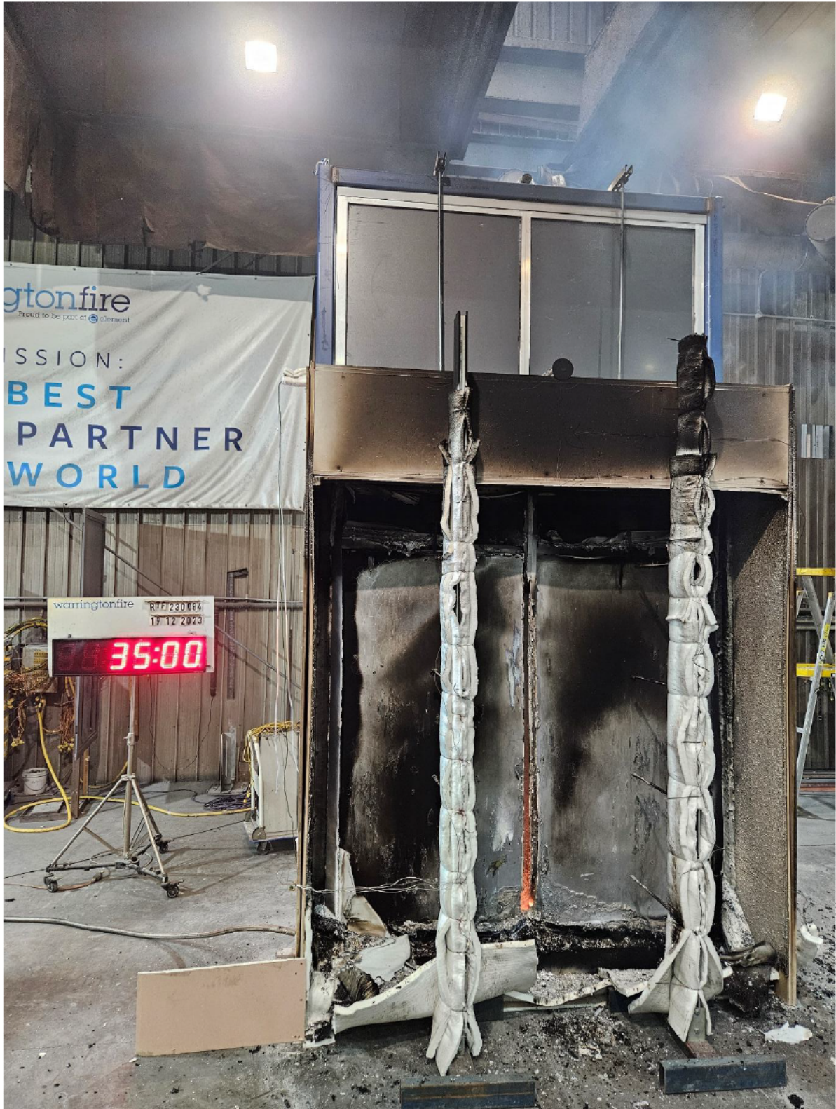
Figure 28 The specimen 5 minutes after the burner was turned off (35 minutes into the test)
