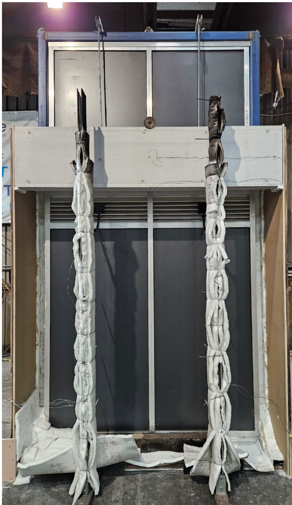
Figure 18 The specimen before the reaction to fire test
