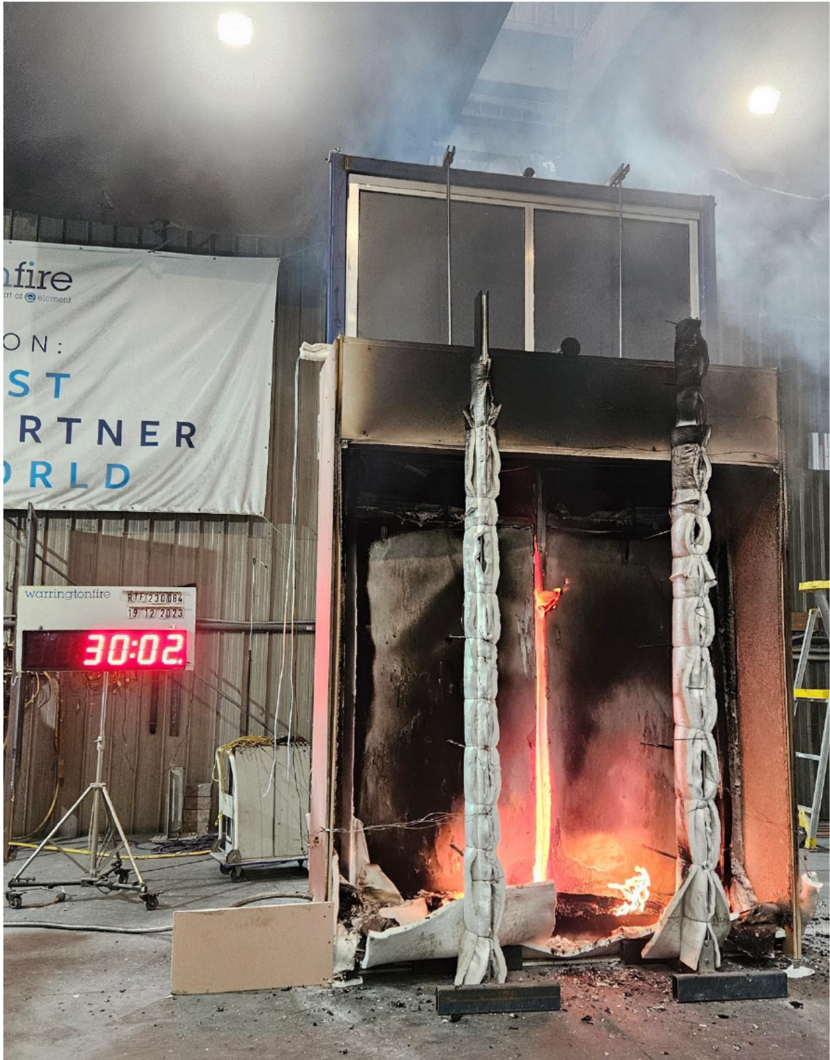
Figure 27 The specimen 2 seconds after the burner was turned off (30 minutes 2 seconds into the test)
