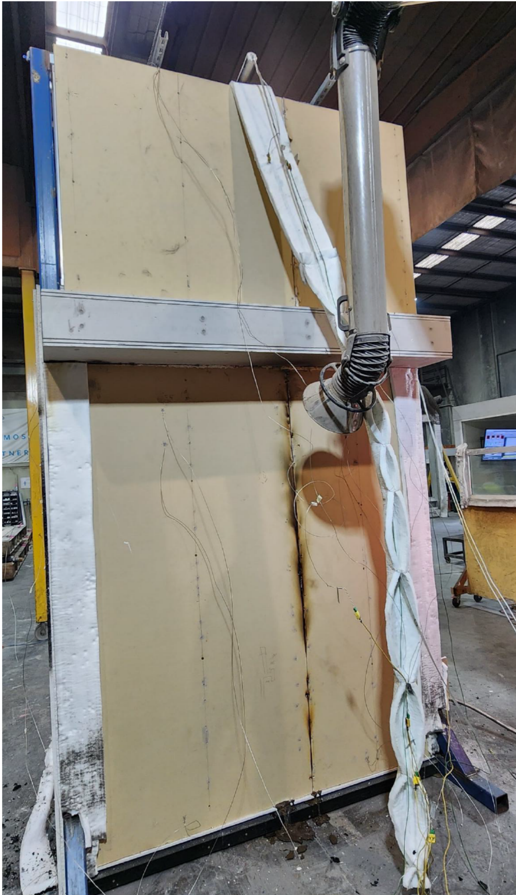
Figure 31 The specimen after the test – unexposed side.
