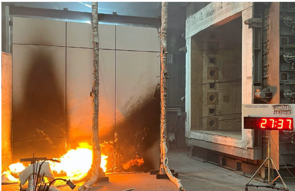
Figure 27 The specimen 27 minutes 37 seconds into the test (burner output at 300 kW)
