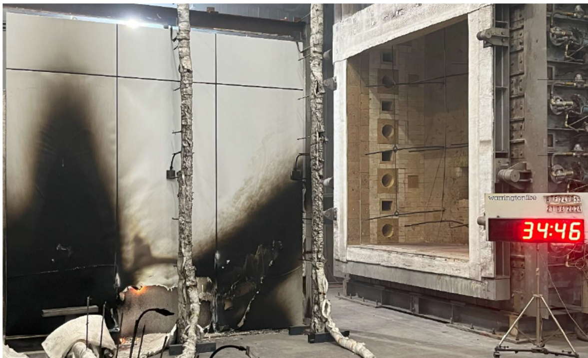
Figure 29 The specimen 34 minutes 46 seconds into the test (4 minutes 46 seconds after burner off)
