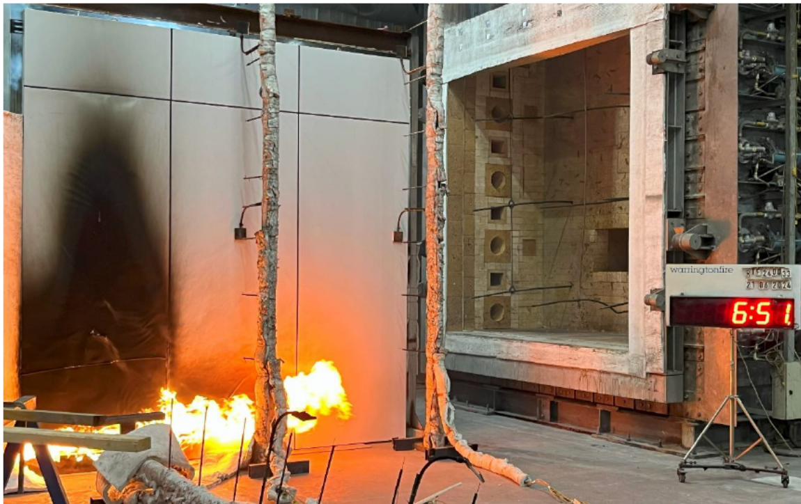
Figure 24 The specimen 6 minutes 51 seconds into the test (burner output at 300 kW)
