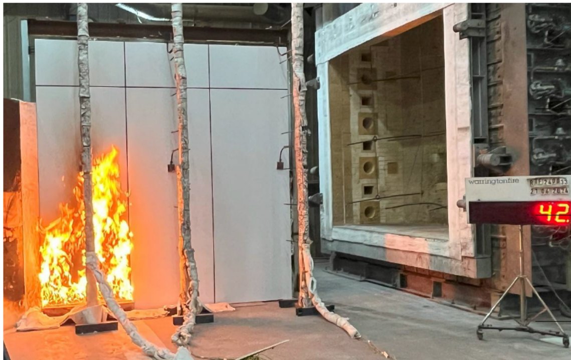
Figure 21 The specimen 42 seconds into the test (burner output at 300 kW)
