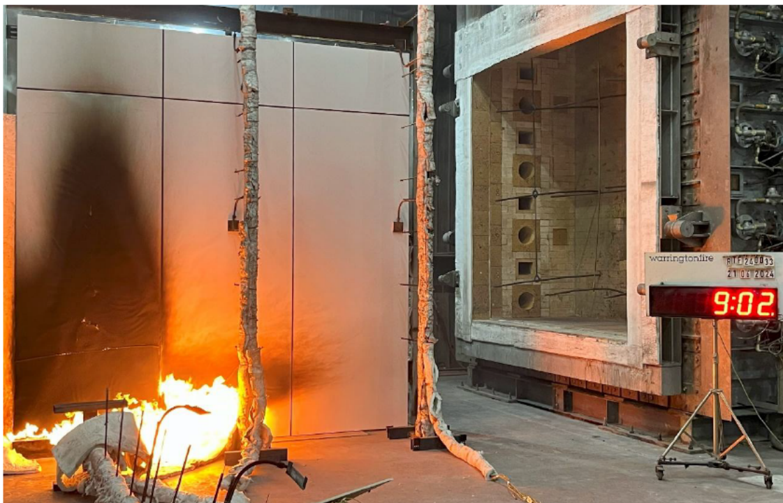
Figure 25 The specimen 9 minutes 2 seconds into the test (burner output at 300 kW)
