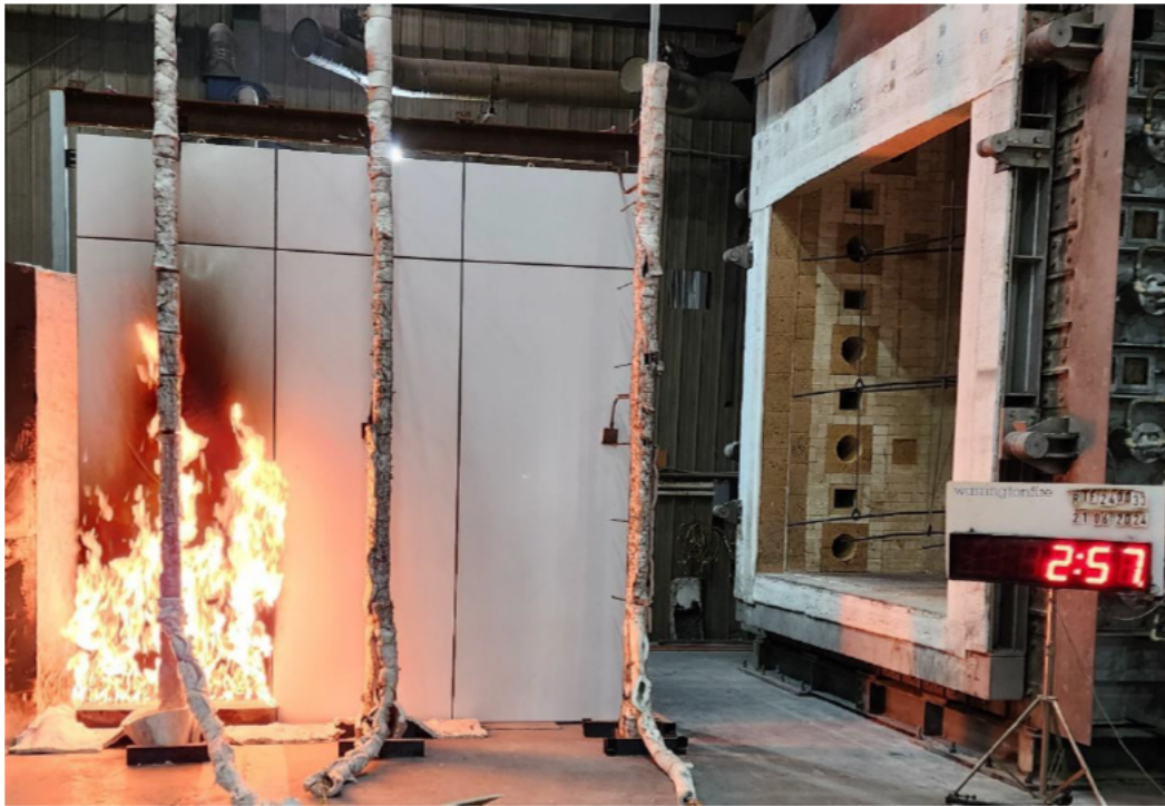
Figure 22 The specimen 2 minutes 57 seconds into the test (burner output at 300 kW)
