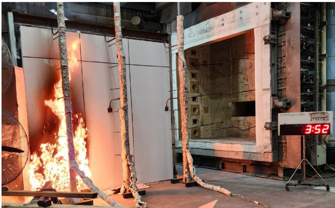
Figure 23 The specimen 3 minutes 52 seconds in the test (burner output at 300 kW)
