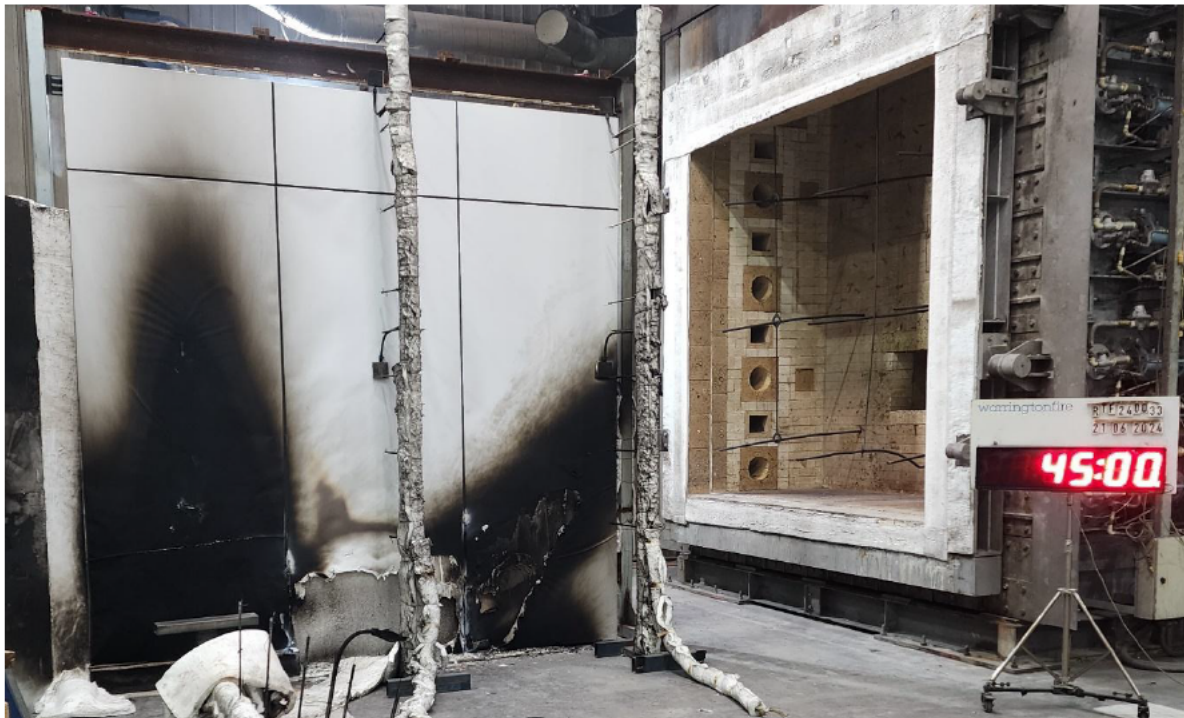
Figure 30 The specimen 45 minutes into the test (5 minutes after burner off)
