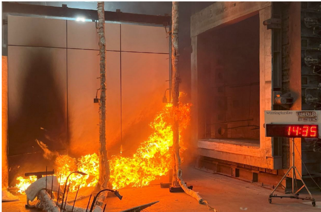
Figure 26 The specimen 14 minutes 35 seconds into the test (burner output at 300 kW)
