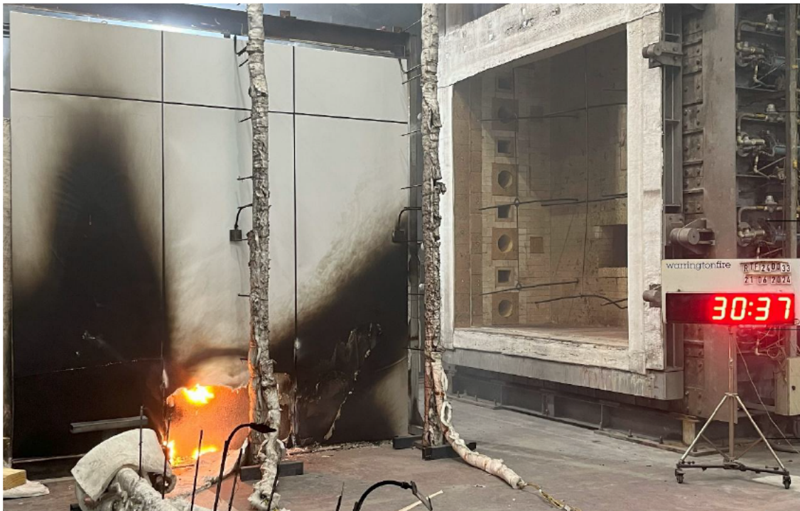
Figure 28 The specimen 30 minutes 37 seconds into the test (37 seconds after burner off)
