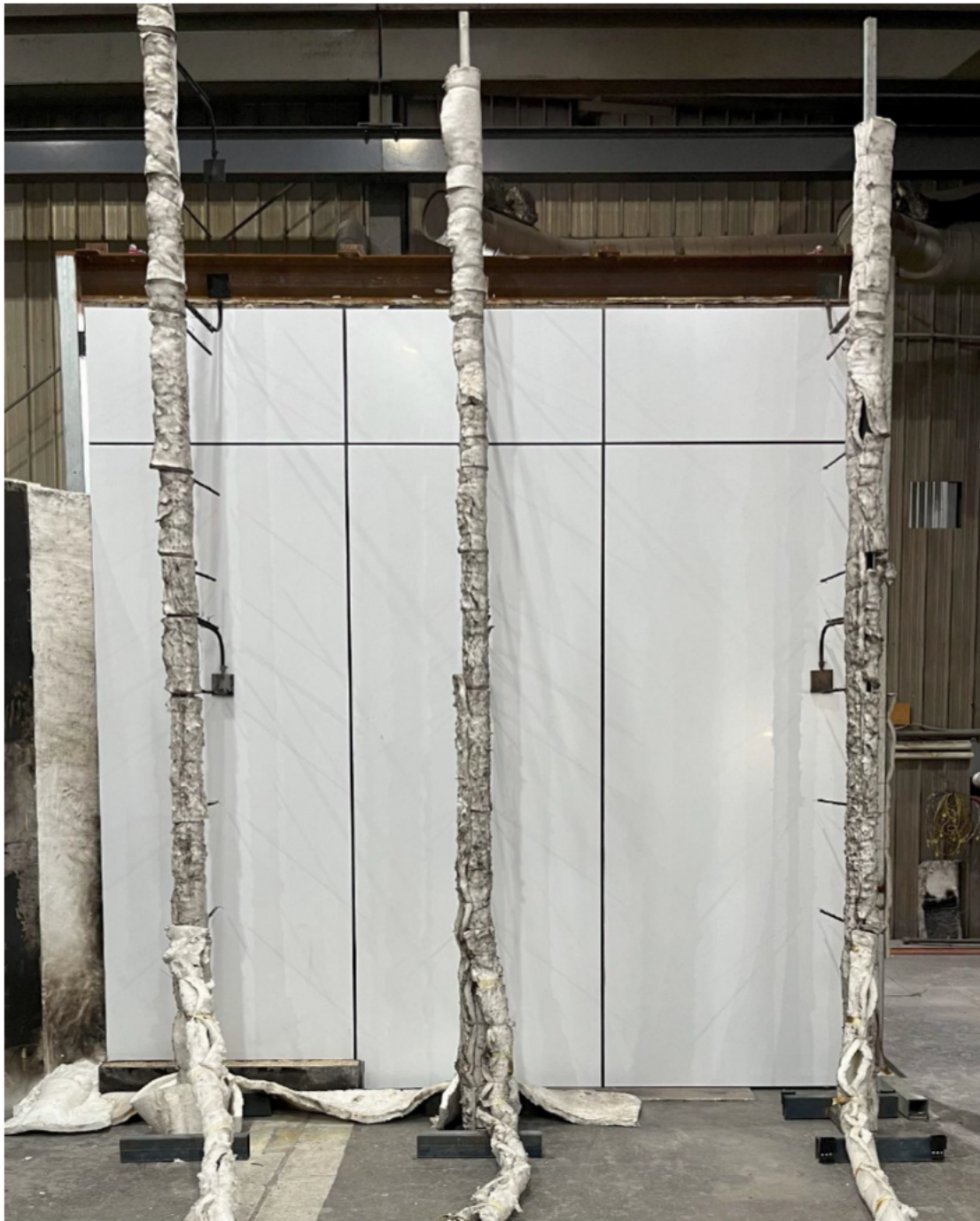
Figure 19 The specimen before the reaction to fire test – exposed side
