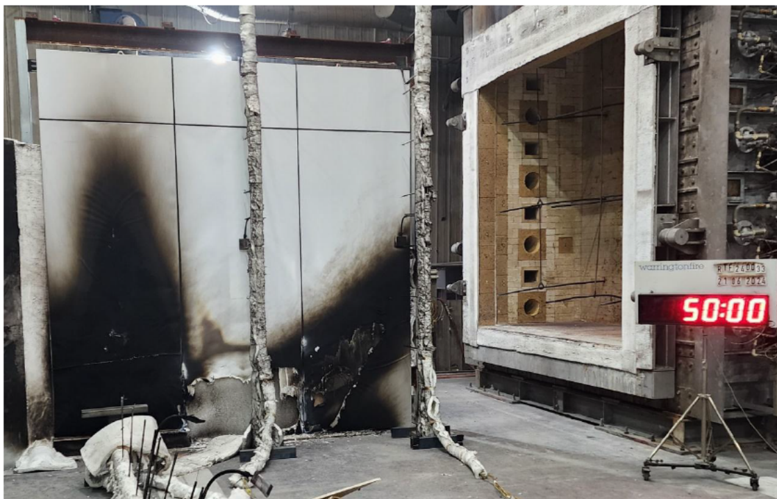
Figure 31 The specimen 50 minutes into the test (10 minutes after burner off)
