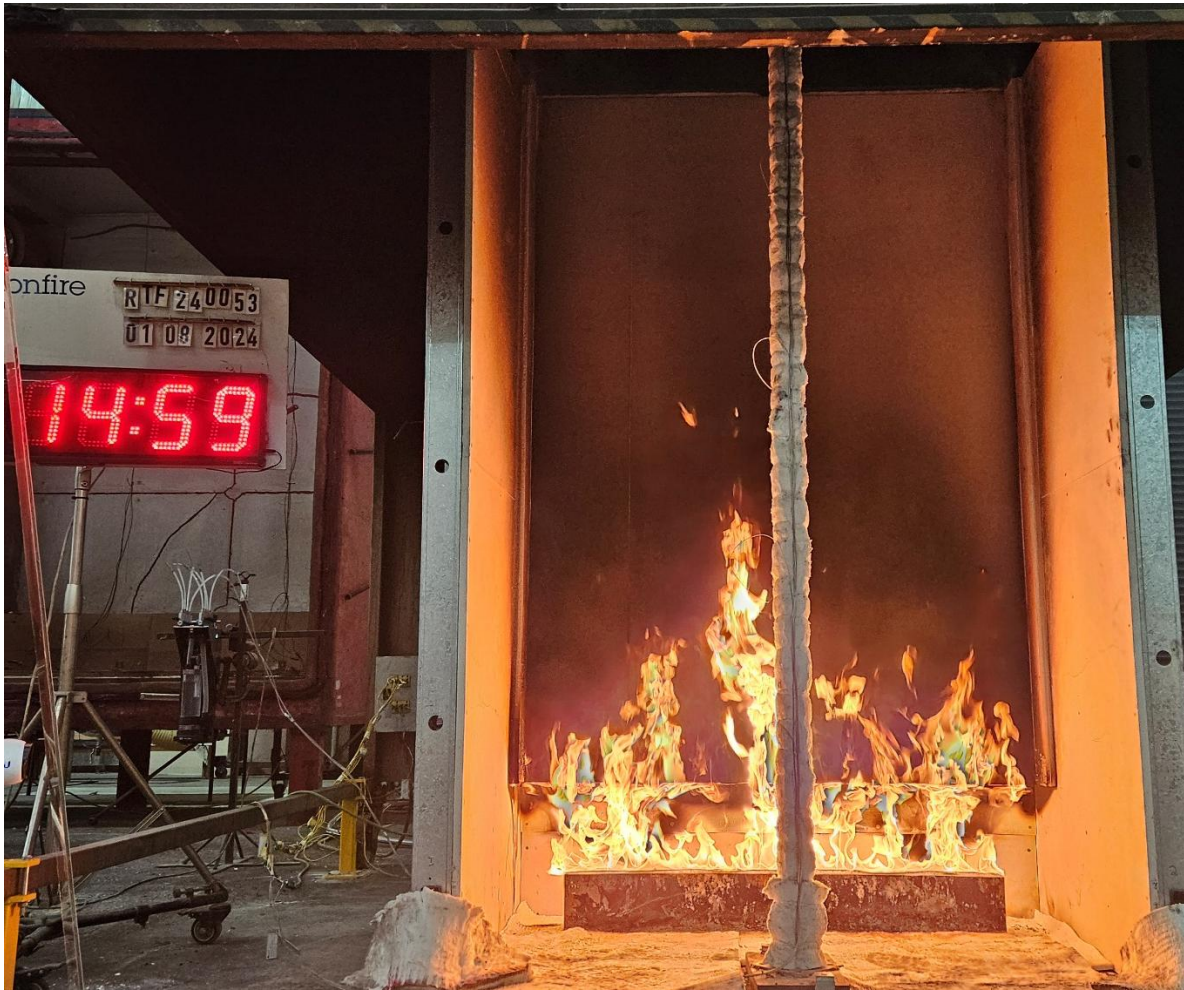
Figure 19 The specimen 14 minutes 59 seconds into the test (burner output at 100 kW)
