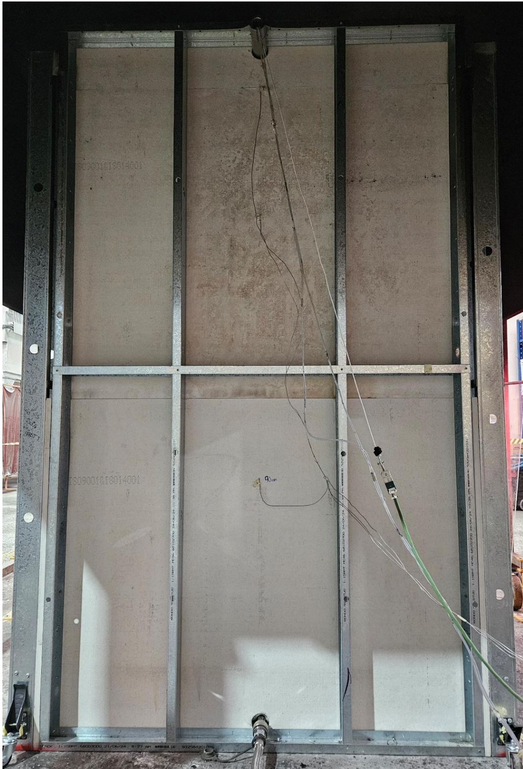
Figure 24 The specimen after the reaction to fire test – unexposed side
