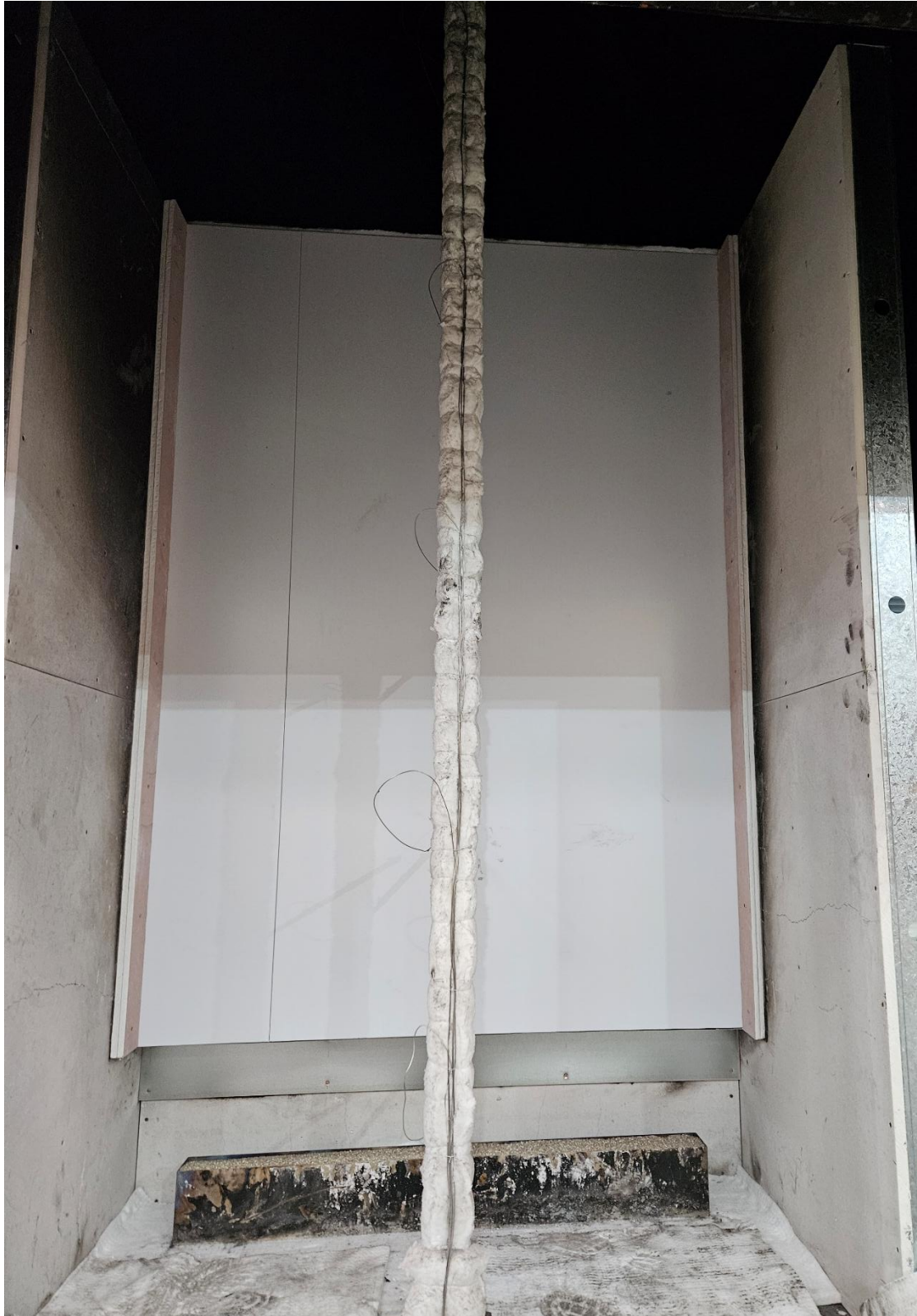
Figure 15 The specimen before the reaction to fire test – exposed side
