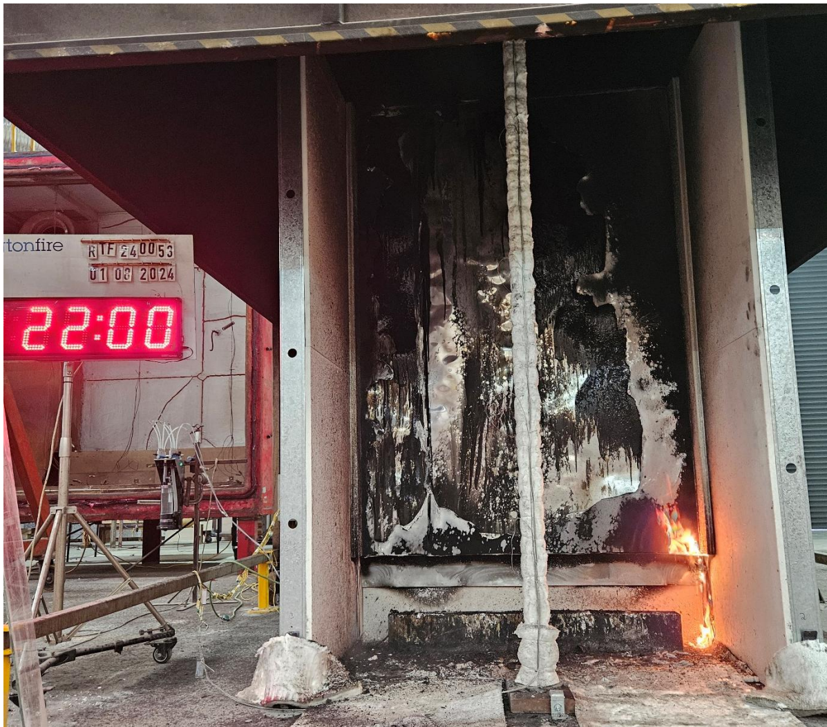
Figure 23 The specimen at end of the reaction to fire test – exposed side
