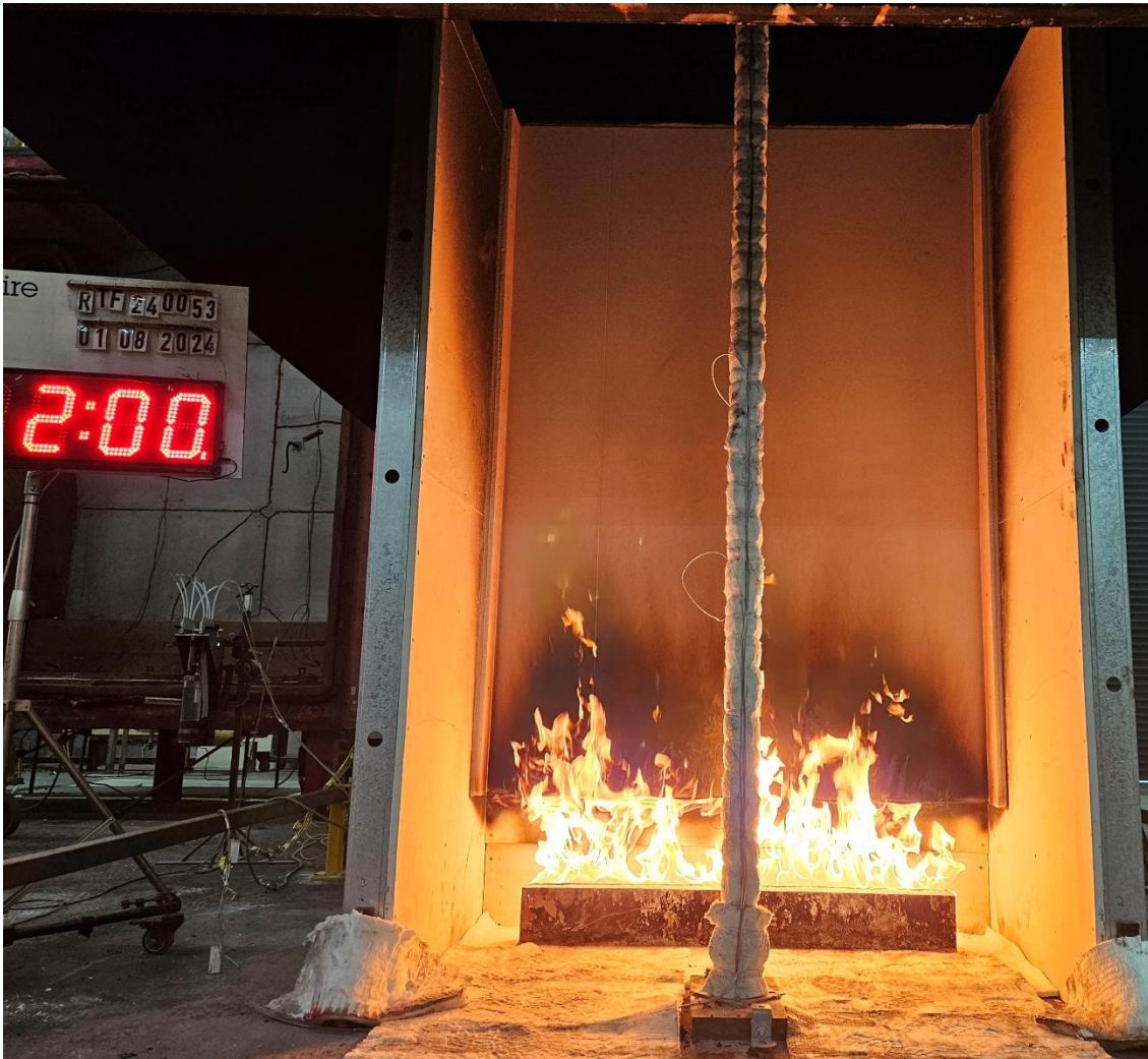
Figure 17 The specimen 2 minutes into the test (burner output at 100 kW)
