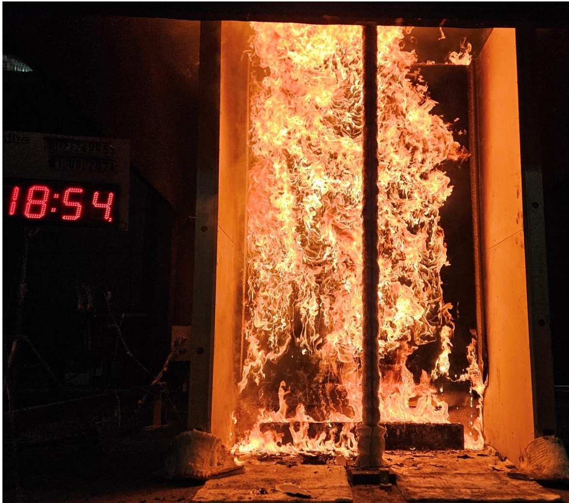
Figure 22 The specimen 18 minutes 54 seconds into the test (burner output at 300 kW)
