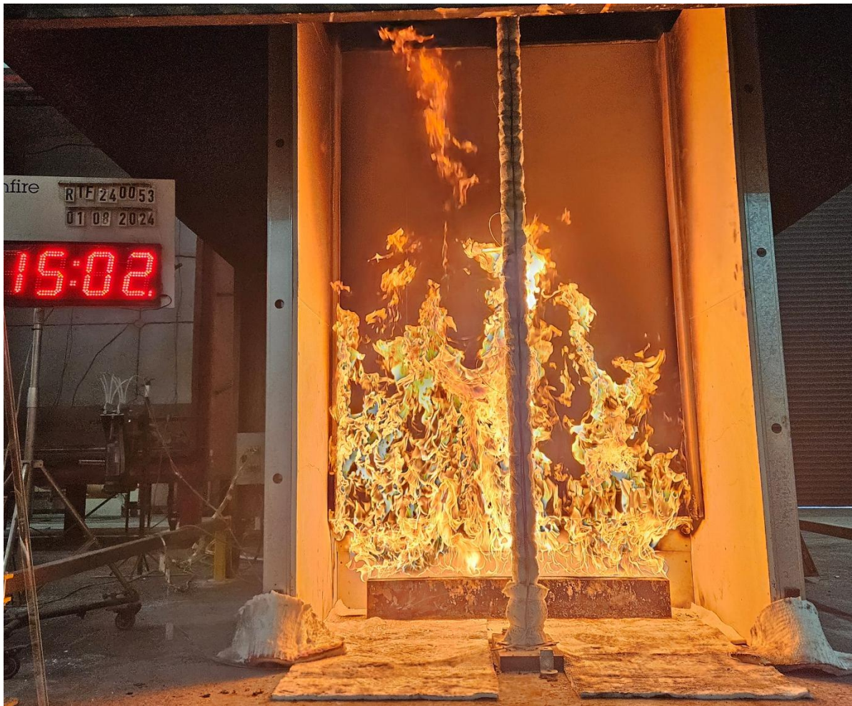
Figure 20 The specimen 15 minutes 02 seconds into the test (burner output at 300 kW)
