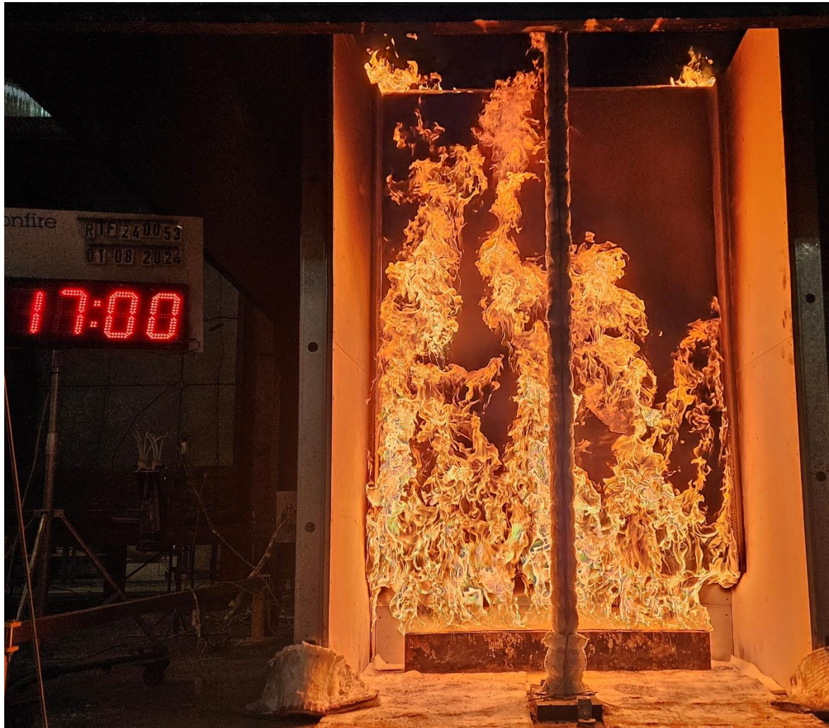
Figure 21 The specimen 17 minutes into the test (burner output at 300 kW)
