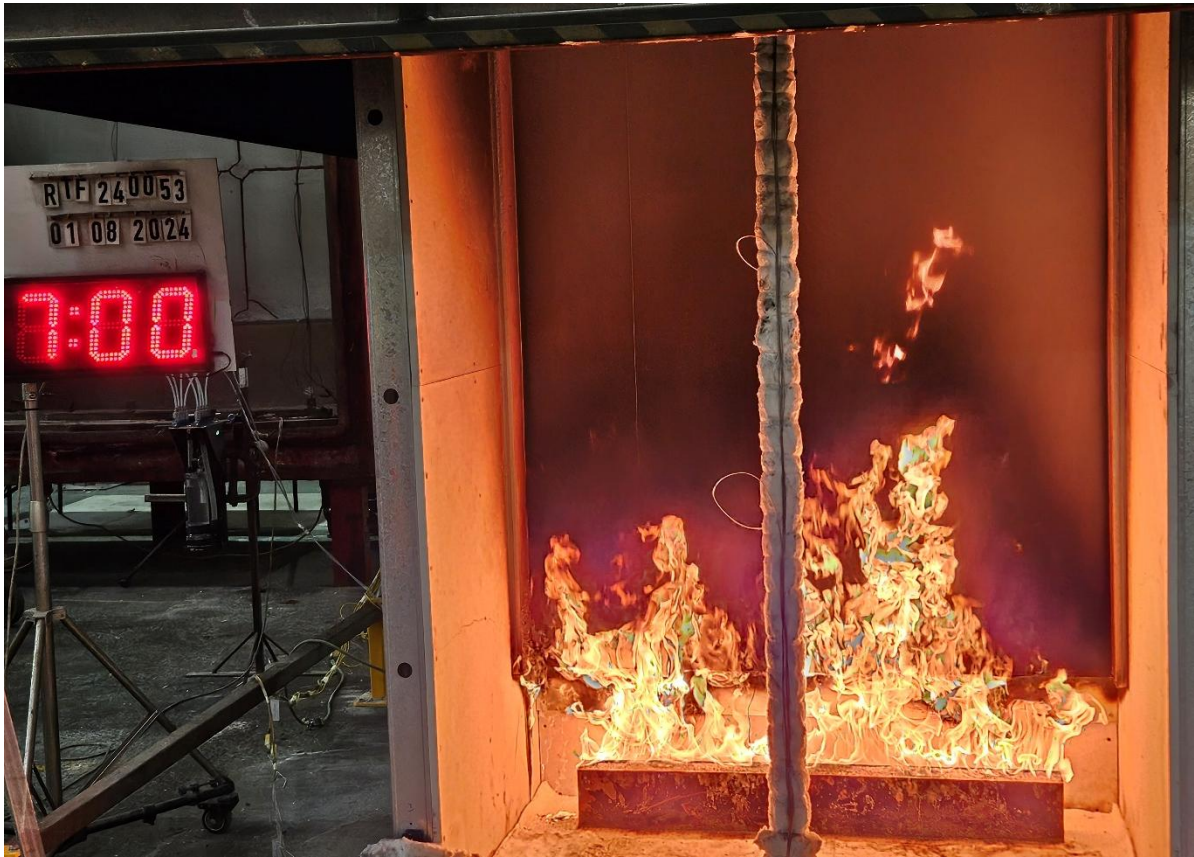
Figure 18 The specimen 7 minutes into the test (burner output at 100 kW)
