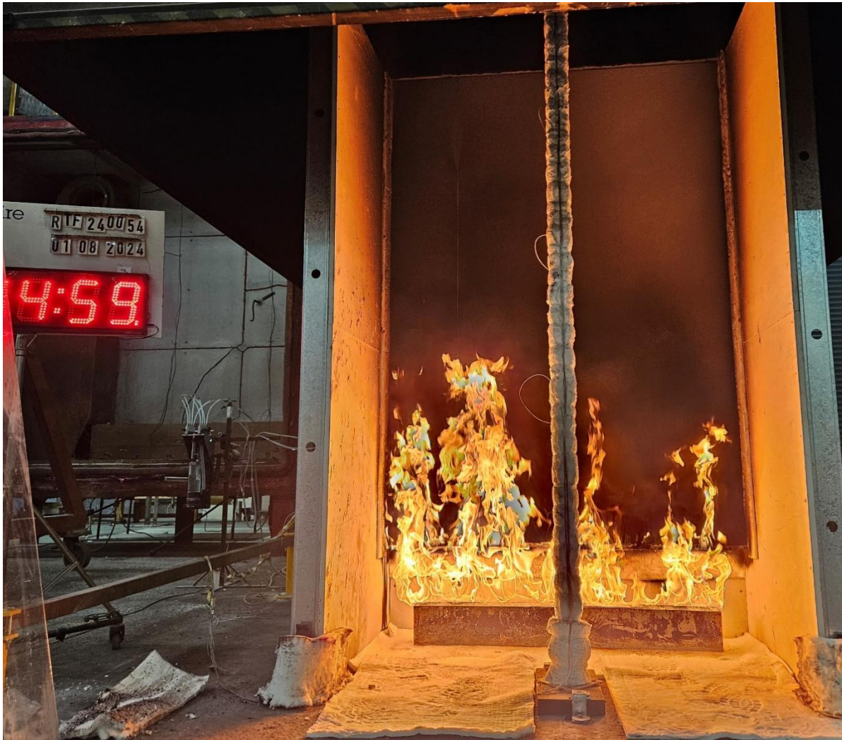
Figure 19 The specimen 14 minutes 59 seconds into the test (burner output at 100 kW)
