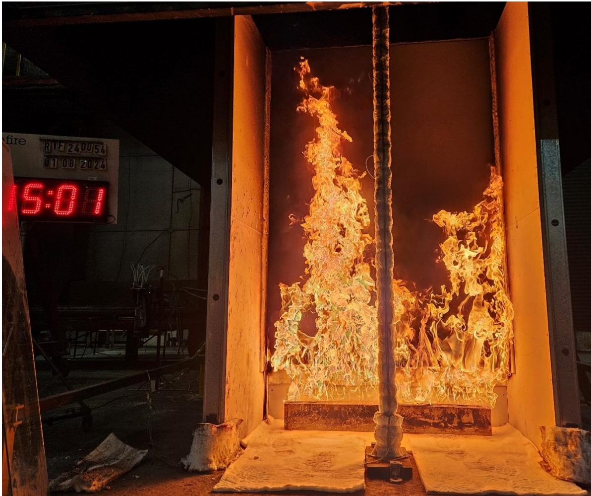
Figure 20 The specimen 15 minutes 01 seconds into the test (burner output at 300 kW)
