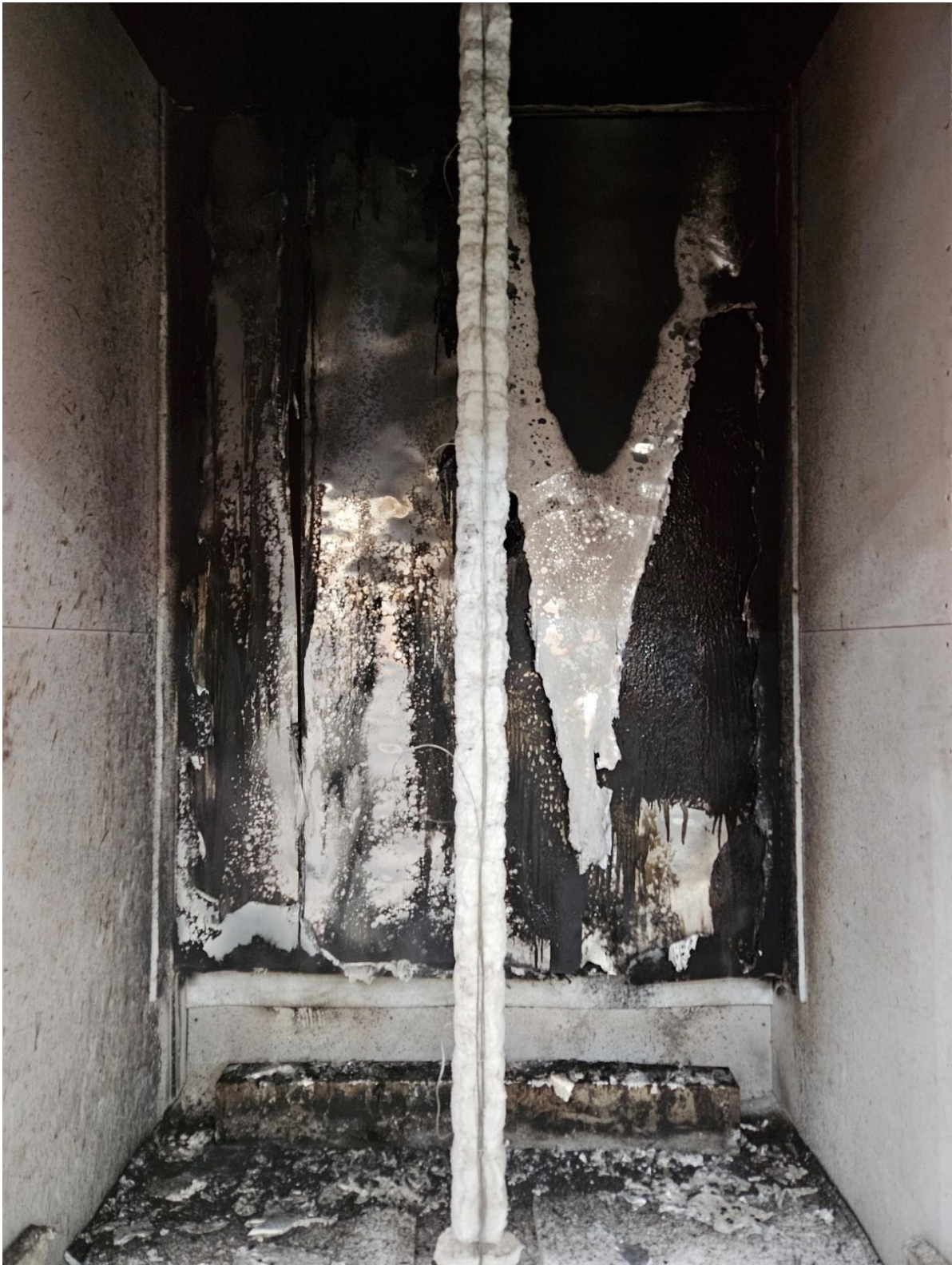
Figure 23 The specimen at end of the reaction to fire test – exposed side
