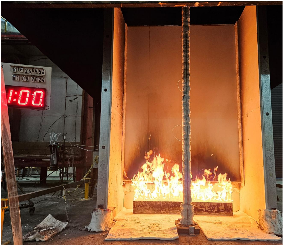
Figure 17 The specimen 1 minute into the test (burner output at 100 kW)
