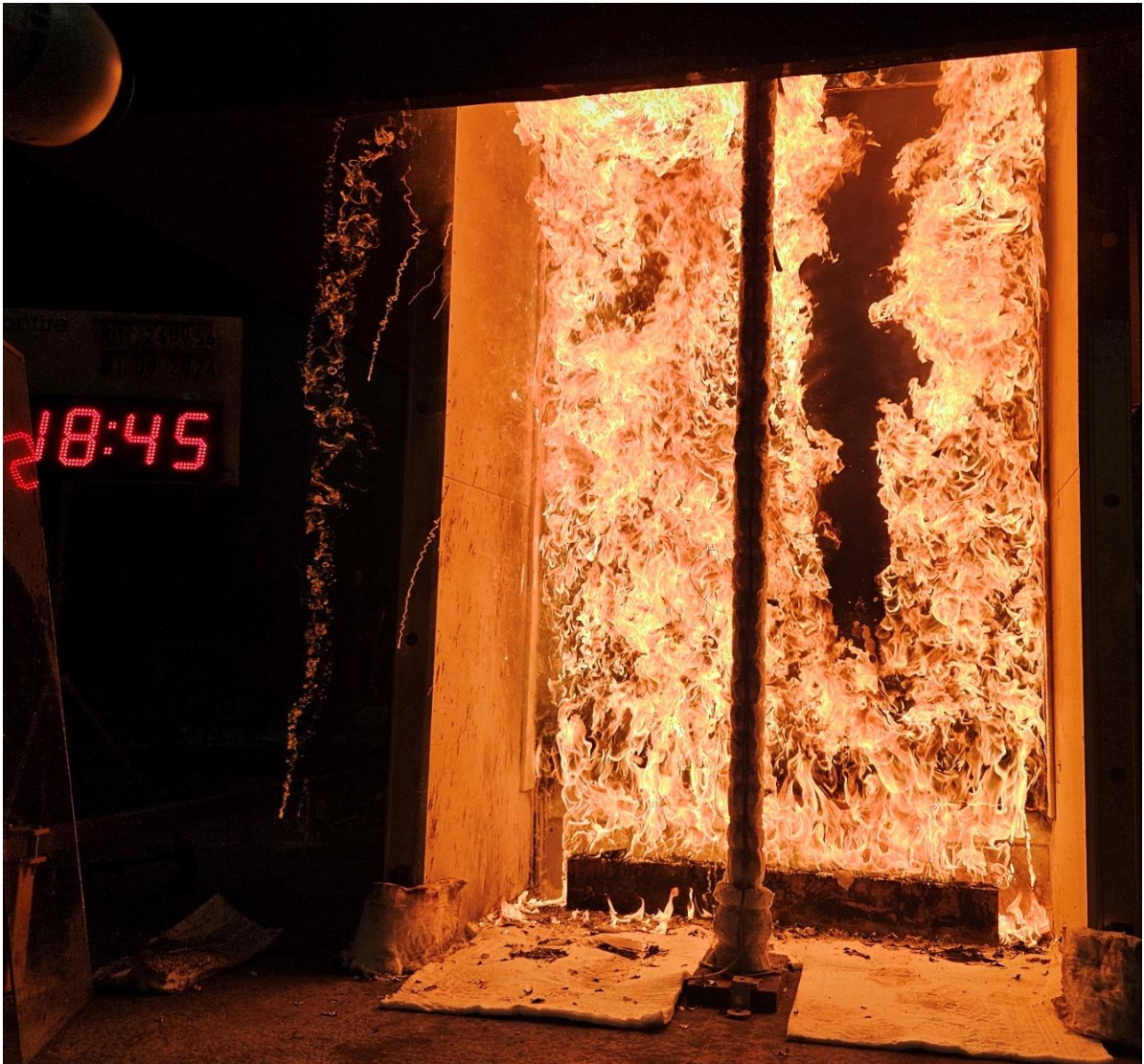
Figure 22 The specimen 18 minutes 45 seconds into the test (burner output at 300 kW)
