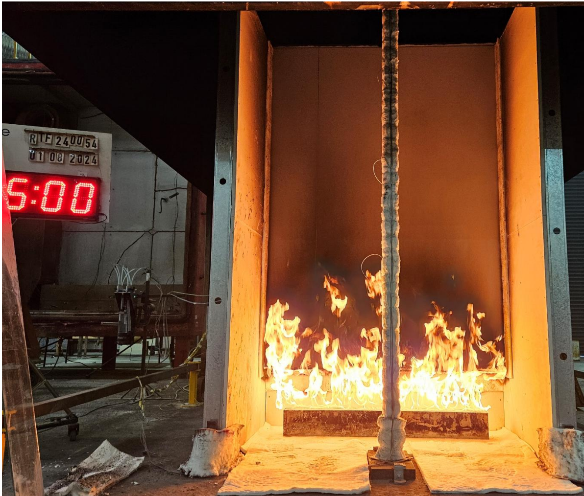
Figure 18 The specimen 5 minutes into the test (burner output at 100 kW)
