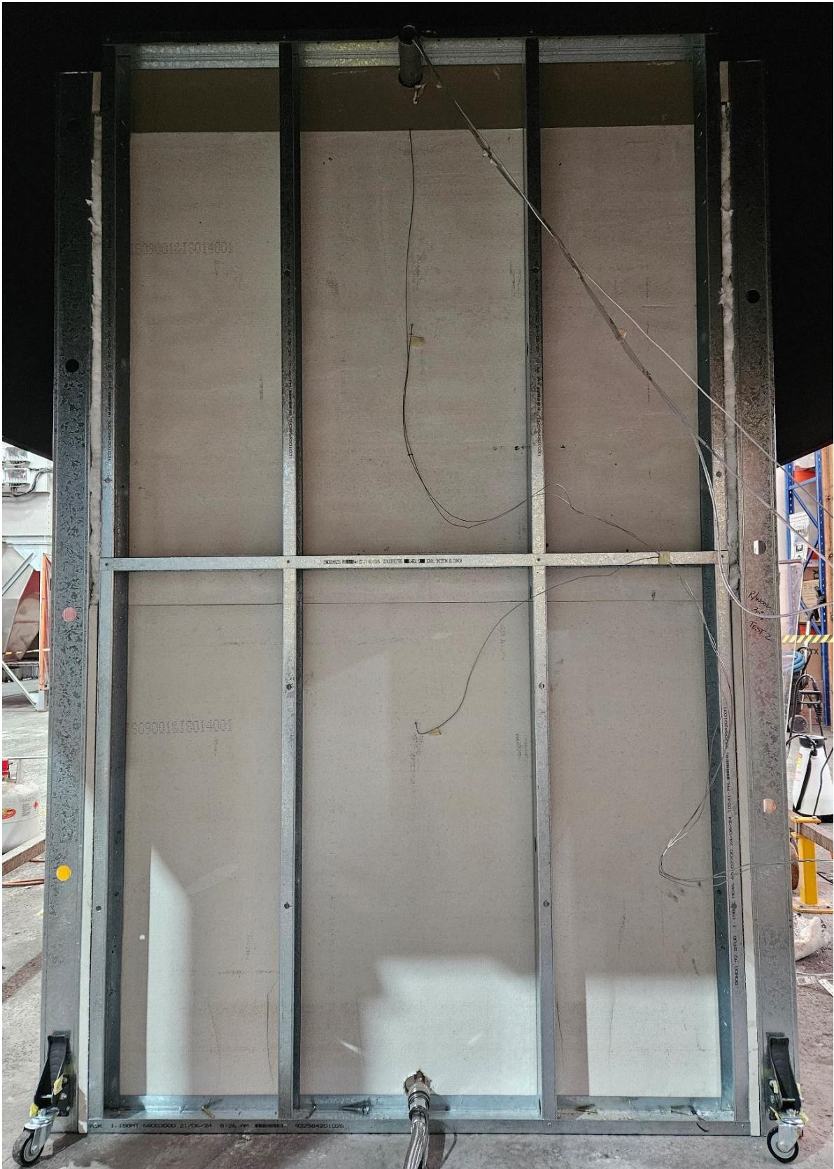
Figure 16 The specimen before the reaction to fire test – unexposed side
