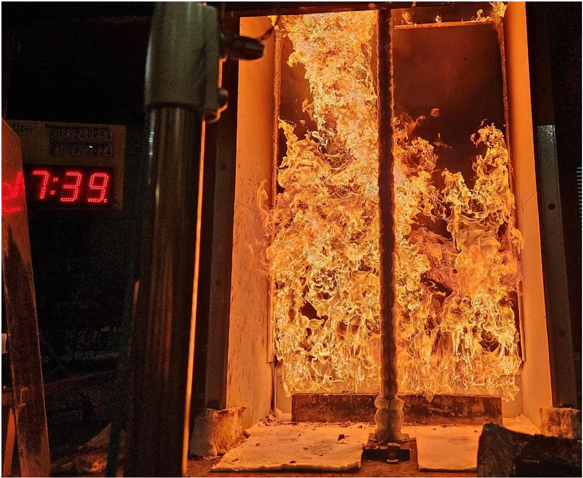
Figure 21 The specimen 17 minutes 39 seconds into the test (burner output at 300 kW)
