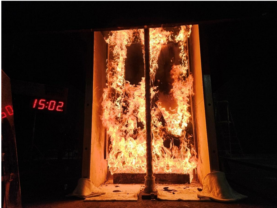
Figure 21 The specimen 15 minutes 02 seconds into the test (burner output at 300 kW)
