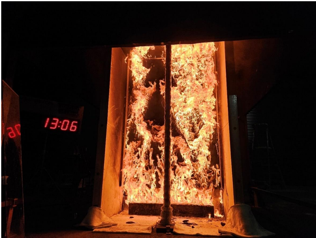
Figure 20 The specimen 13 minutes 06 seconds into the test (burner output at 100 kW)
