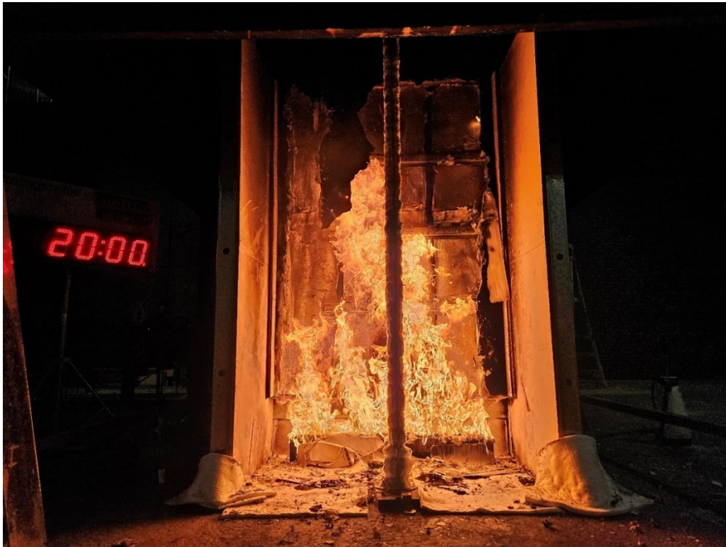
Figure 23 The specimen 20 minutes into the test (burner output at 300 kW)
