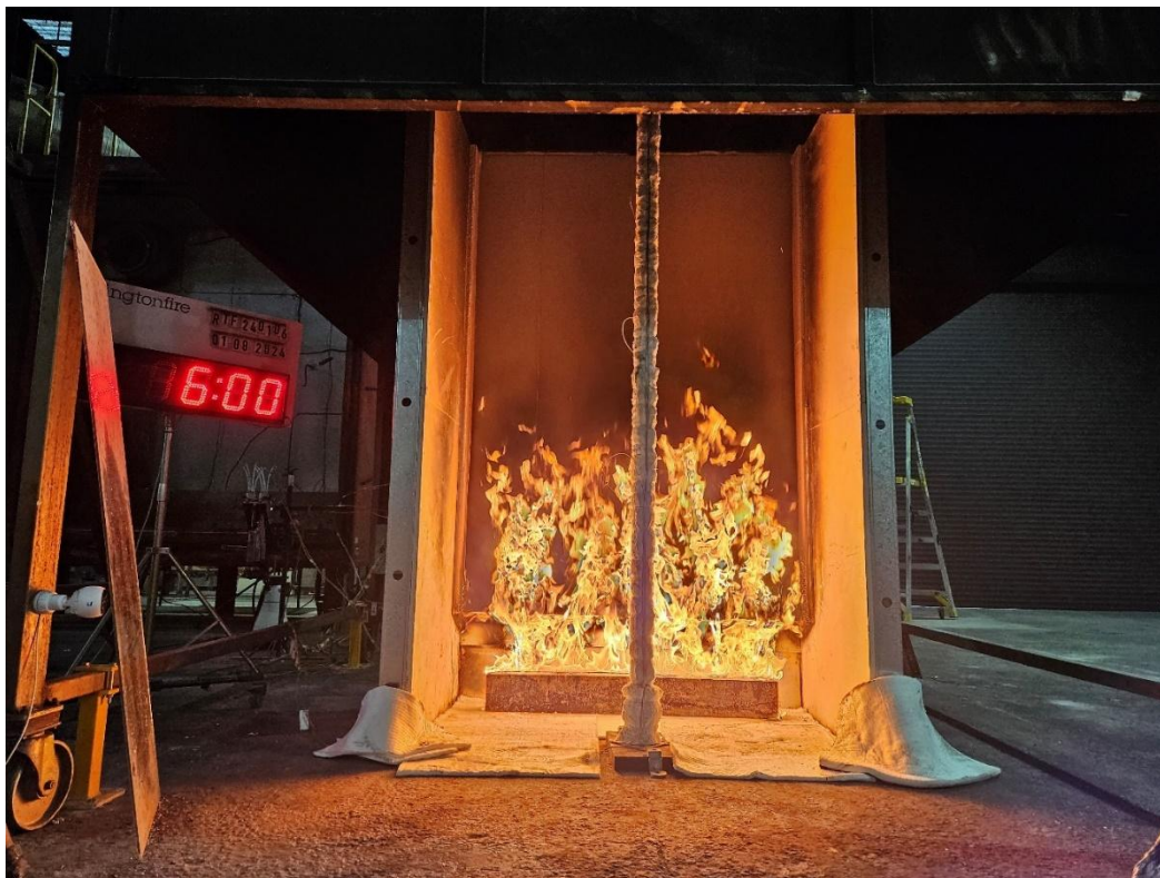
Figure 18 The specimen 6 minutes into the test (burner output at 100 kW)
