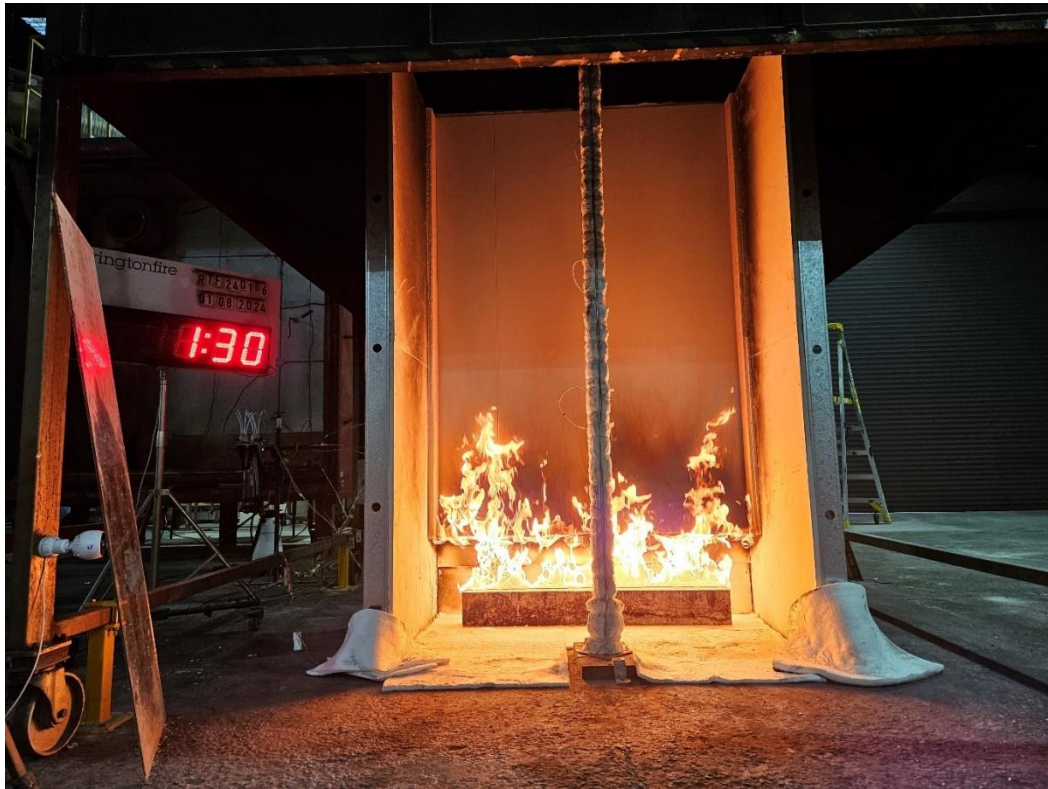
Figure 17 The specimen 1 minute 30 seconds into the test (burner output at 100 kW)
