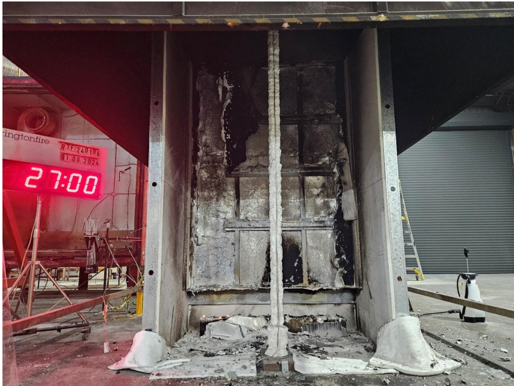
Figure 25 The specimen at end of the reaction to fire test – exposed side
