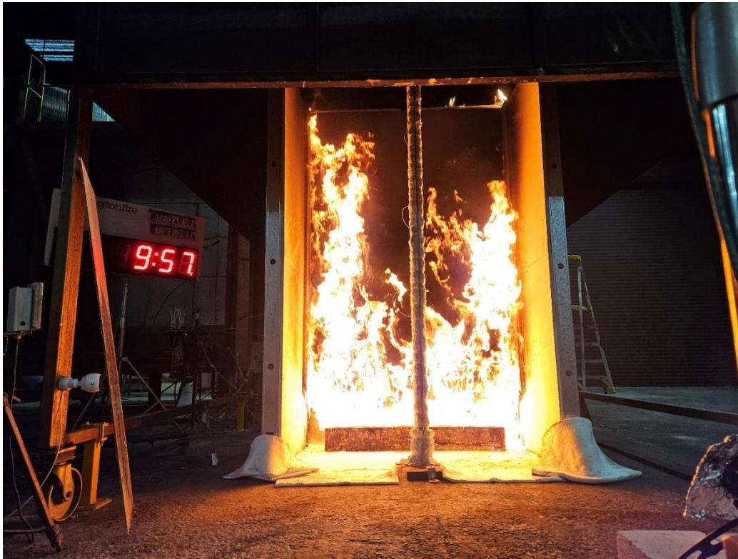
Figure 19 The specimen 9 minutes 57 seconds into the test (burner output at 100 kW)
