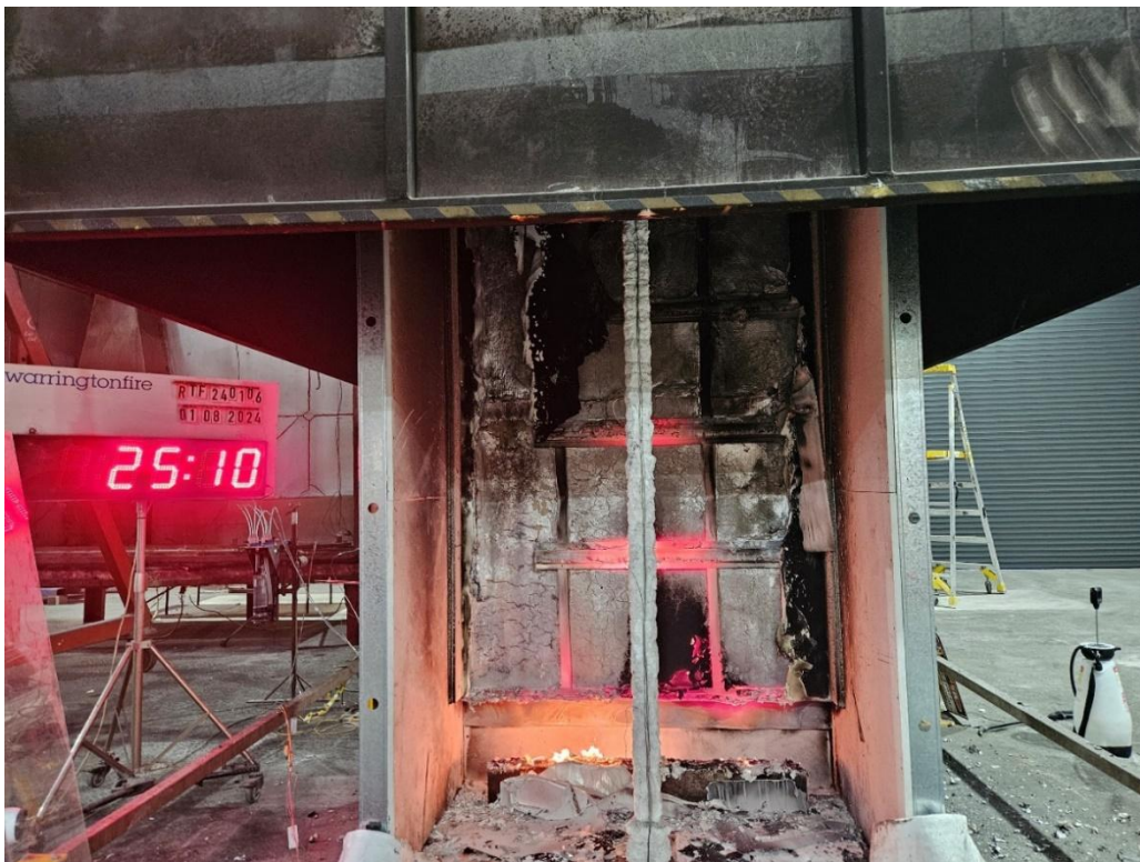
Figure 24 The specimen 25 minutes 10 seconds into the test (10 seconds after the burner was turned off)
