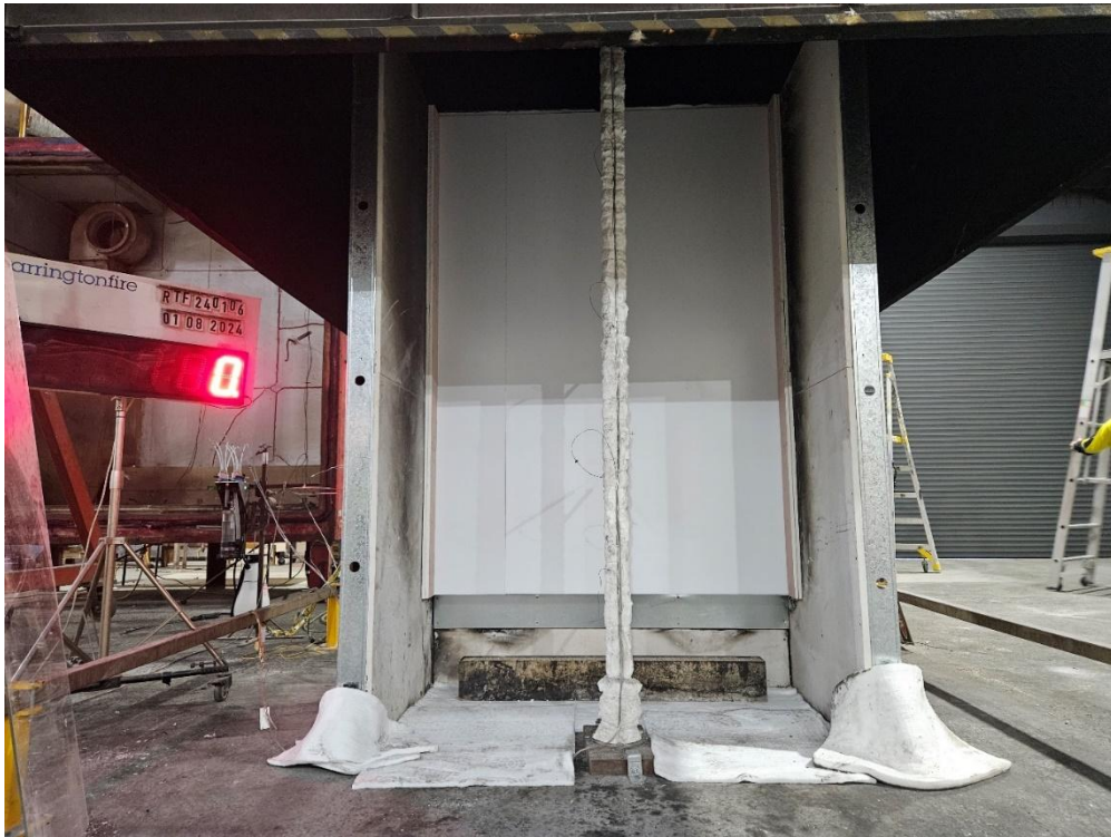
Figure 15 The specimen before the reaction to fire test – exposed side
