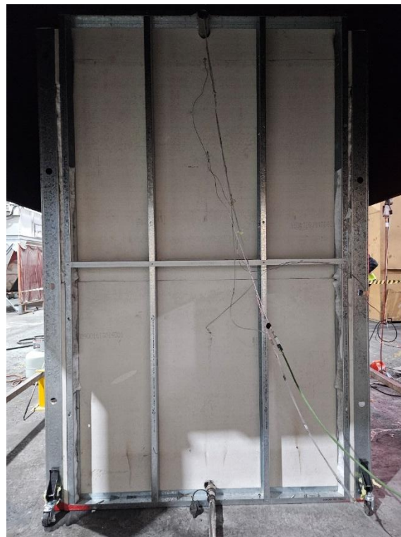
Figure 16 The specimen before the reaction to fire test – unexposed side
