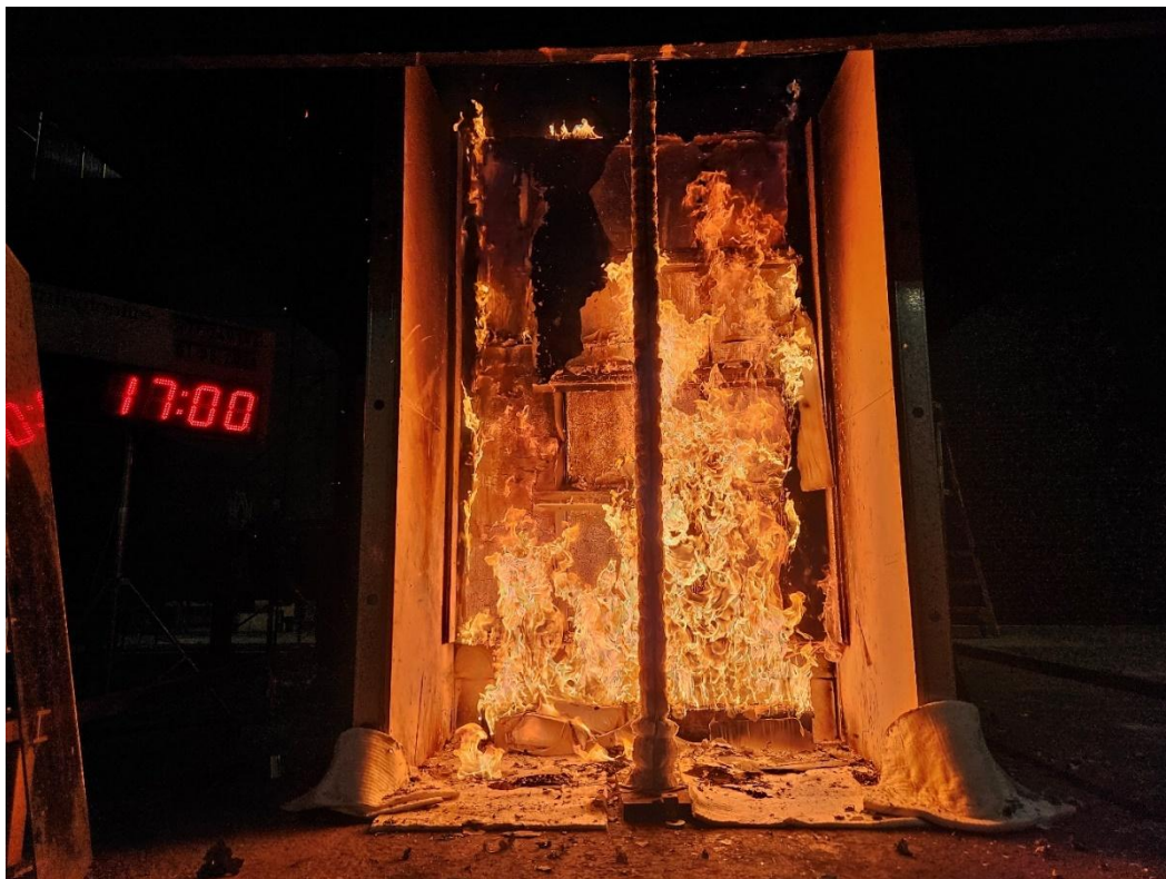
Figure 22 The specimen 17 minutes into the test (burner output at 300 kW)
