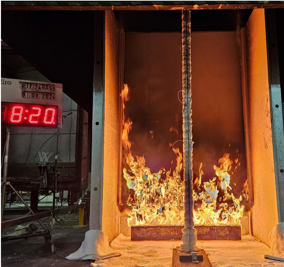
Figure 18 The specimen 8 minutes 20 seconds into the test (burner output at 100 kW)
