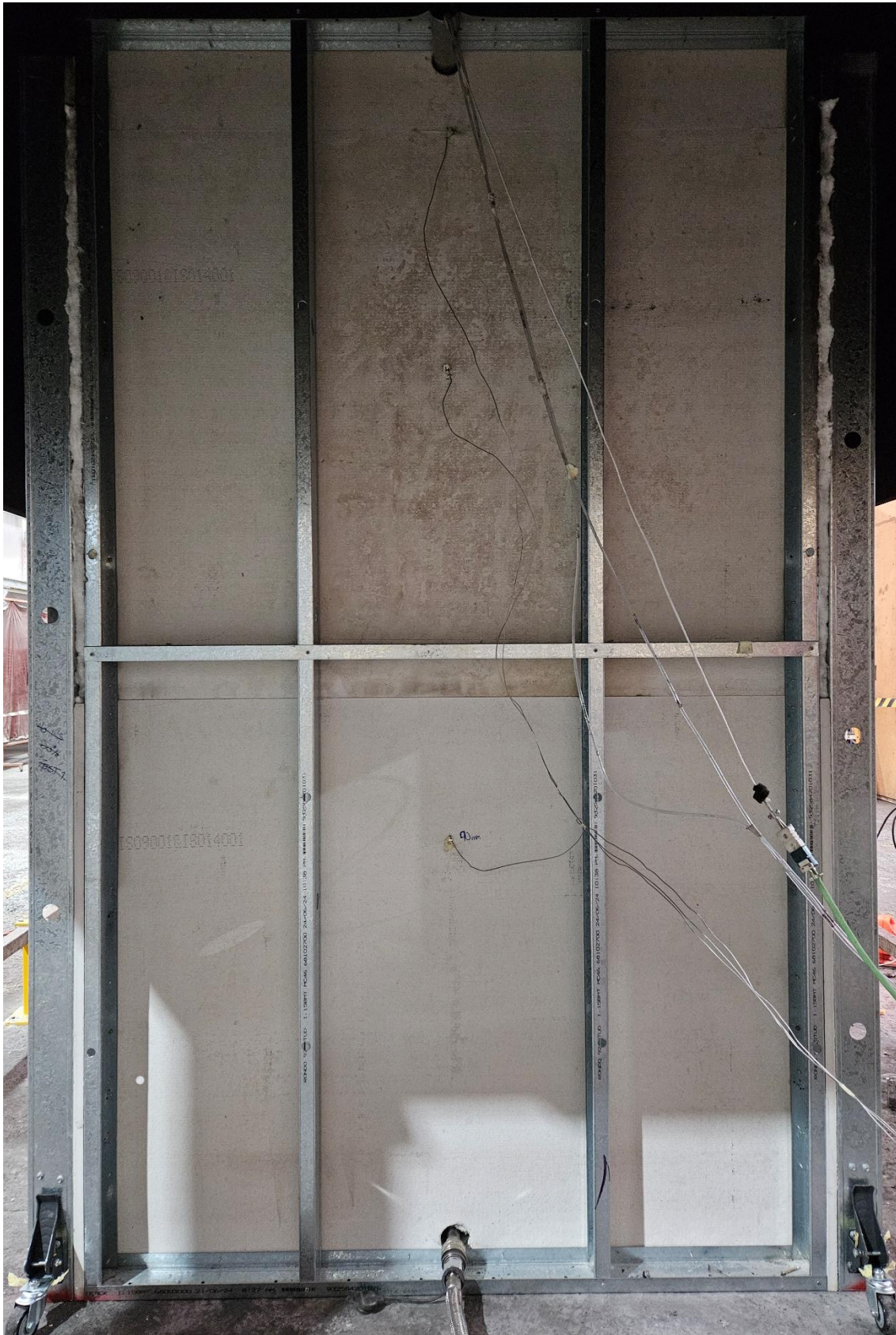
Figure 16 The specimen before the reaction to fire test – unexposed side
