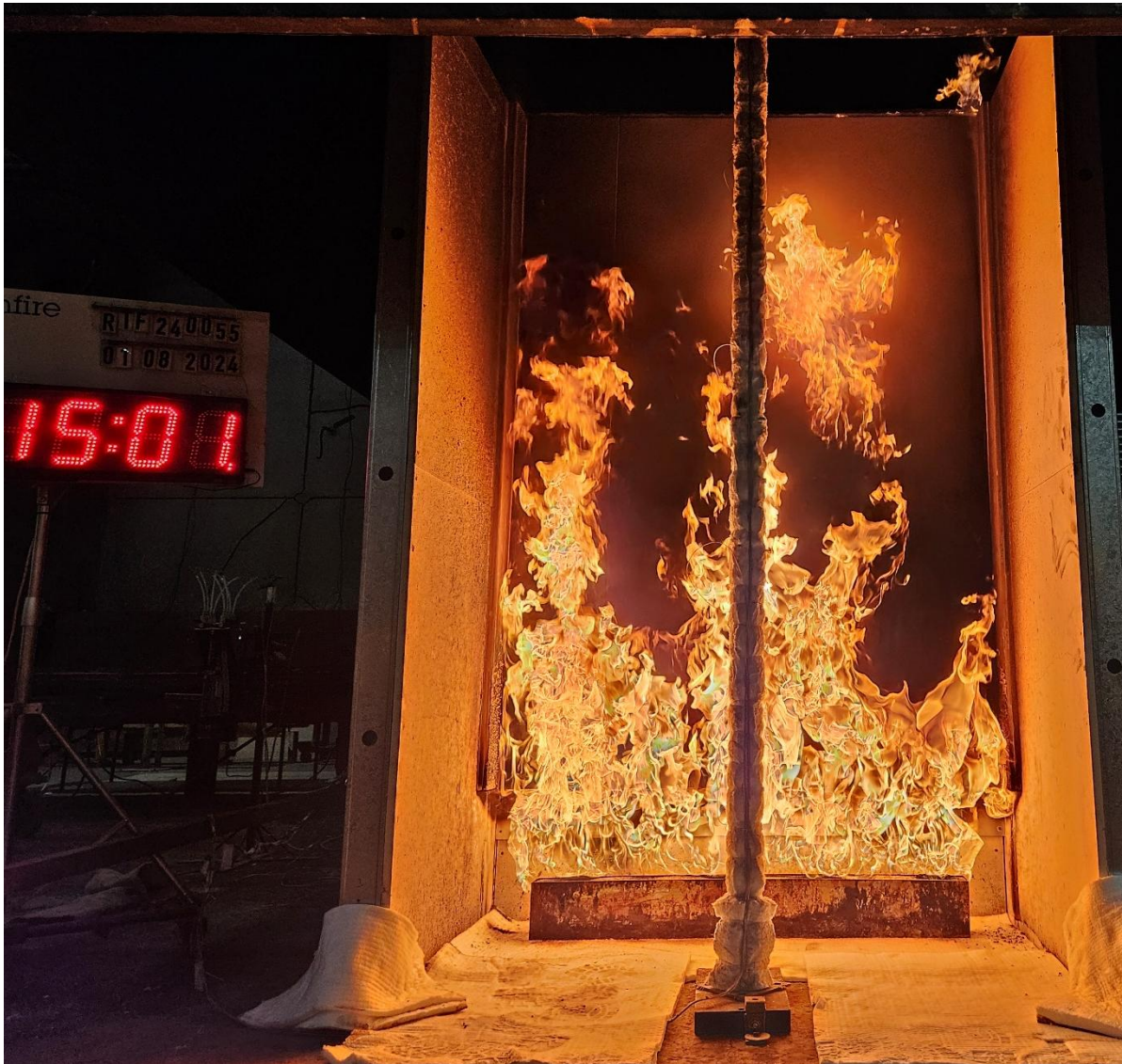
Figure 20 The specimen 15 minutes 01 seconds into the test (burner output at 300 kW)
