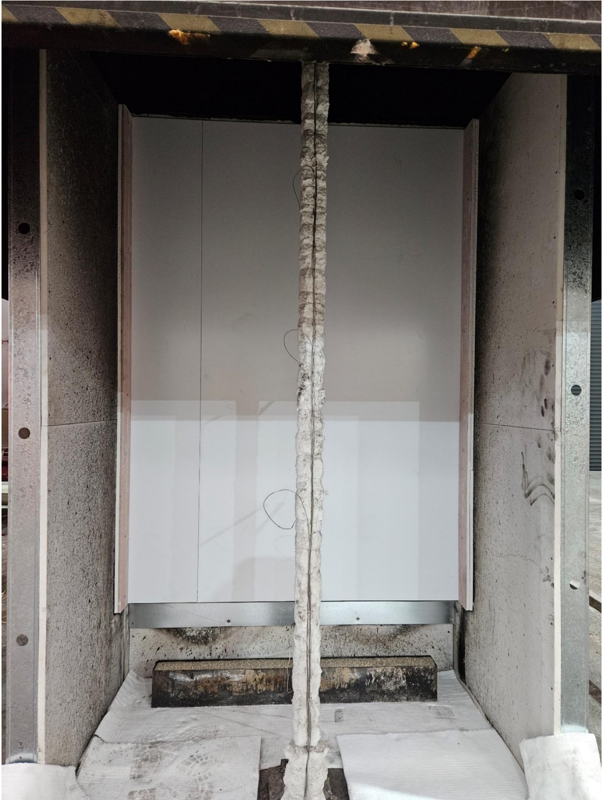
Figure 15 The specimen before the reaction to fire test – exposed side
