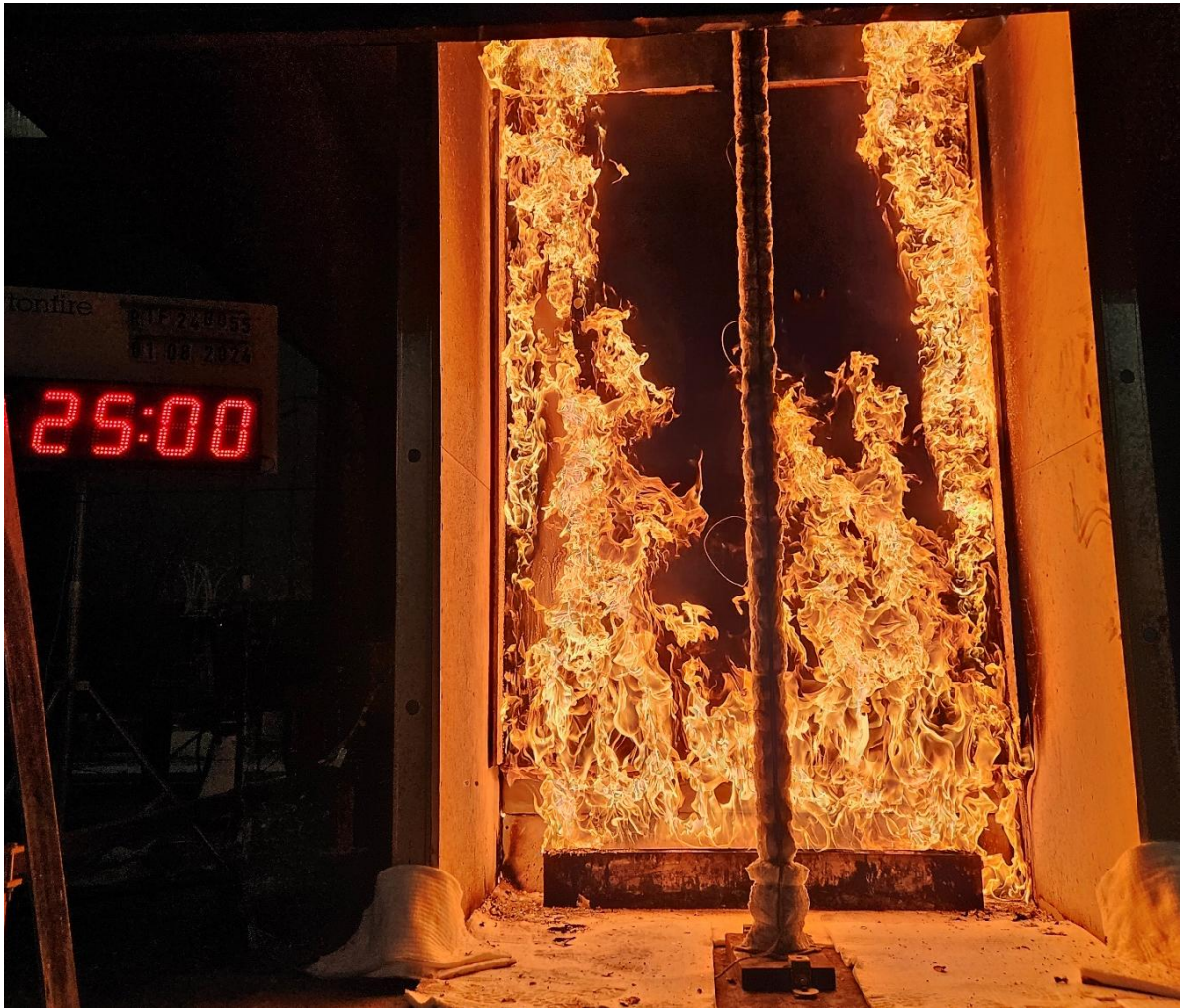
Figure 21 The specimen 25 minutes into the test (burner output at 300 kW)
