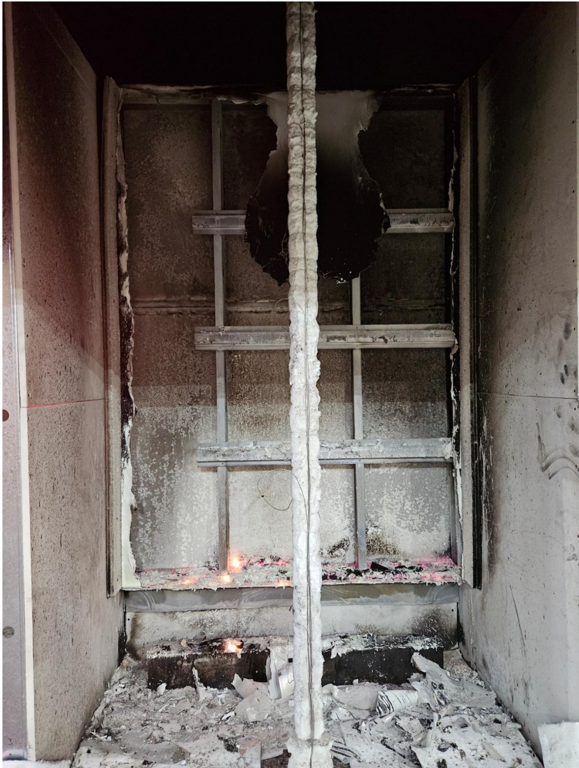
Figure 24 The specimen at end of the reaction to fire test – exposed side
