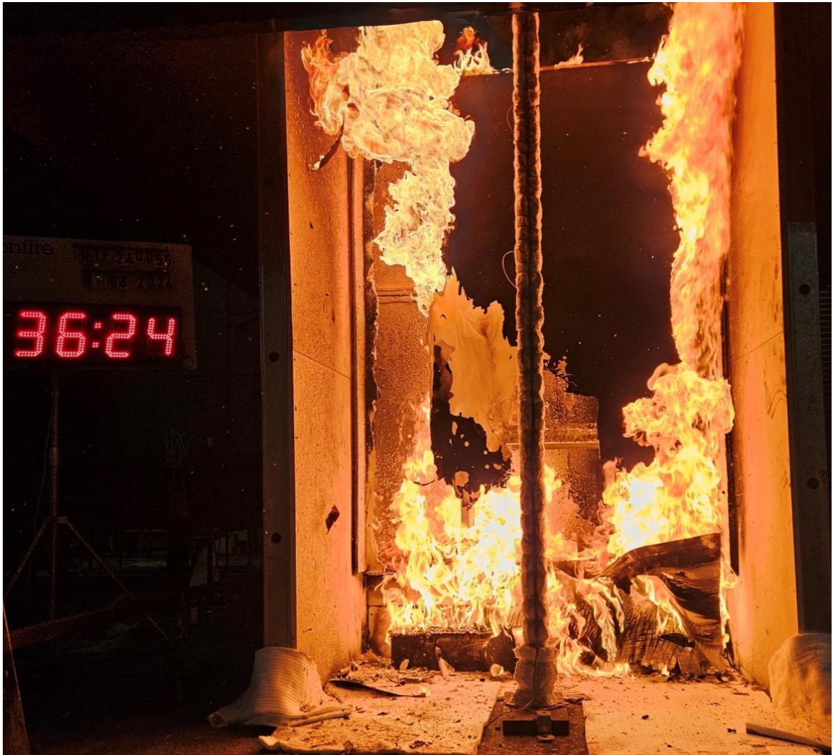
Figure 22 The specimen 36 minutes 24 seconds into the test (burner output at 300 kW)
