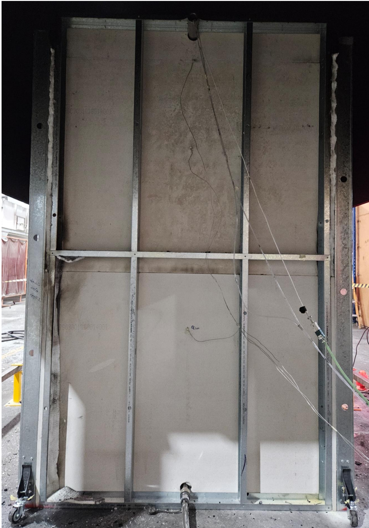
Figure 25 The specimen after the reaction to fire test – unexposed side
