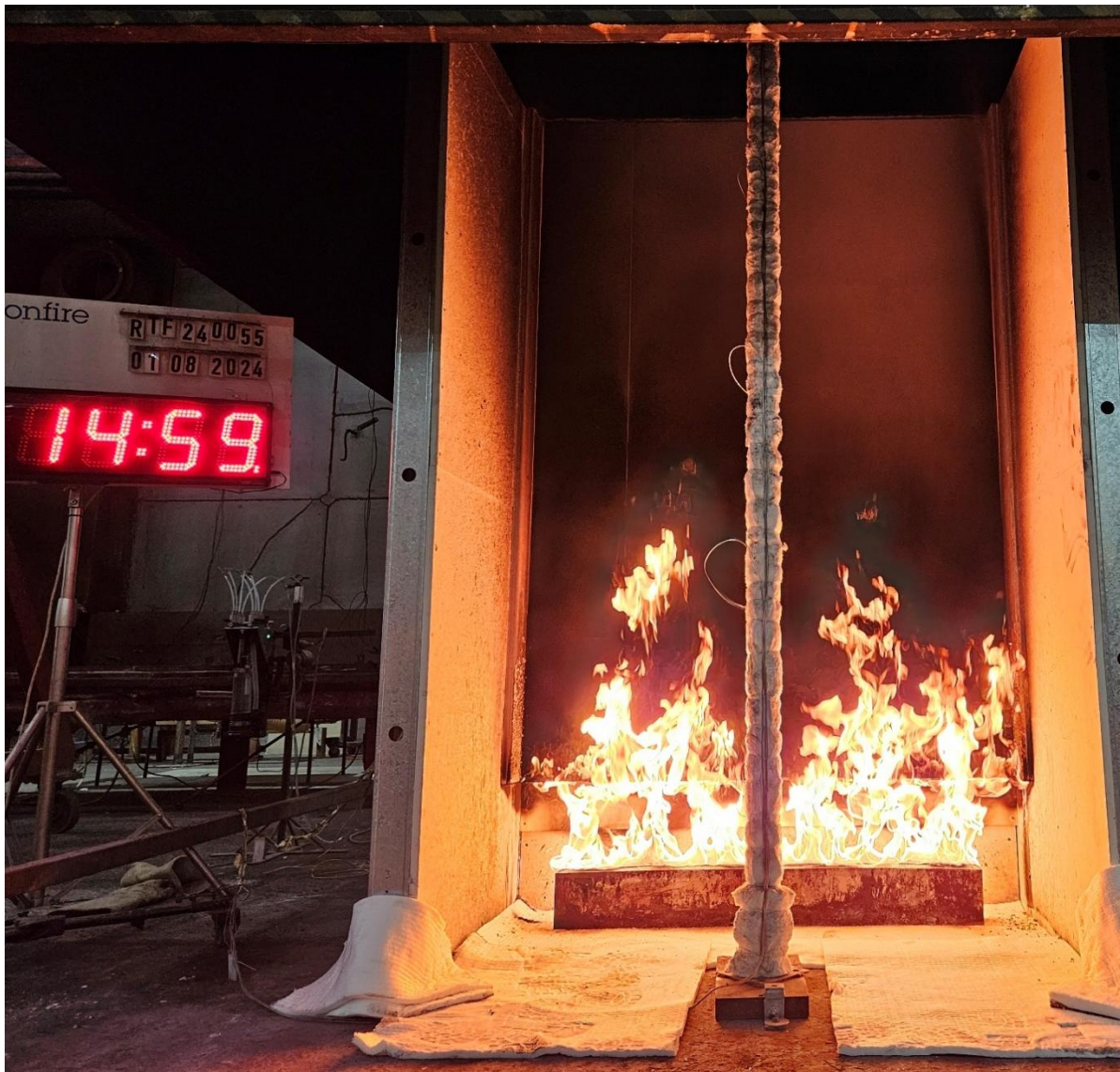
Figure 19 The specimen 14 minutes 59 seconds into the test (burner output at 100 kW)
