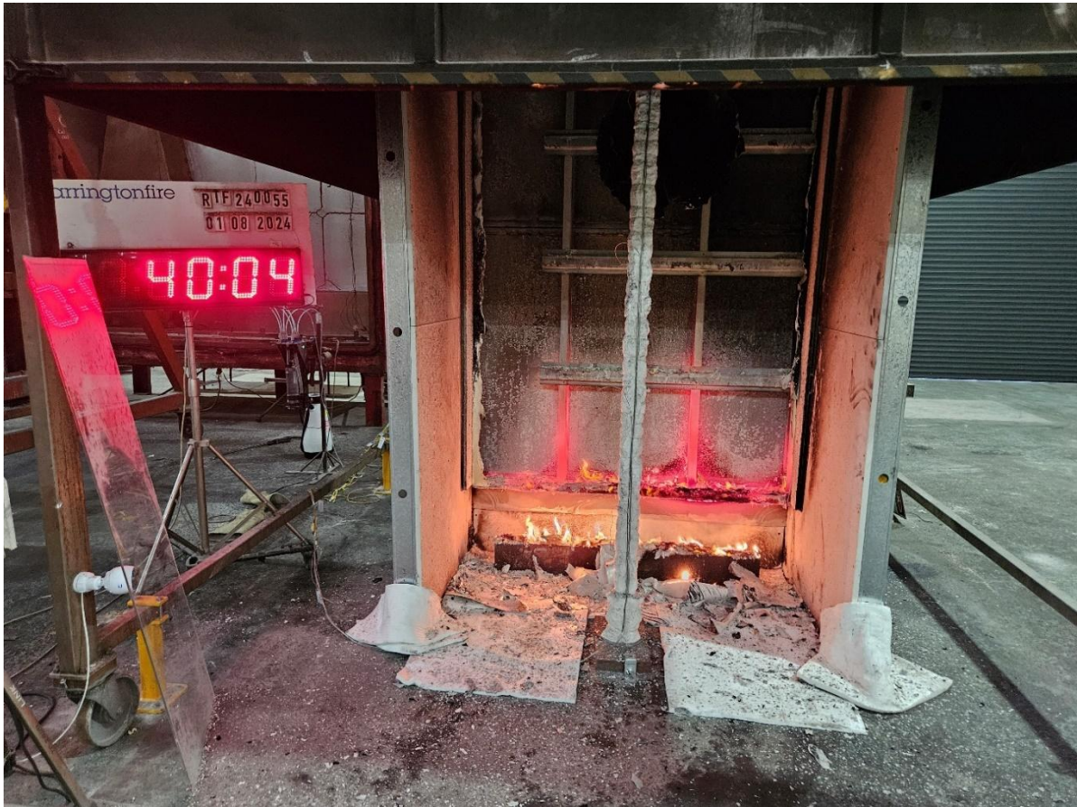
Figure 23 The specimen 40 minutes 04 seconds into the test (burner off)
