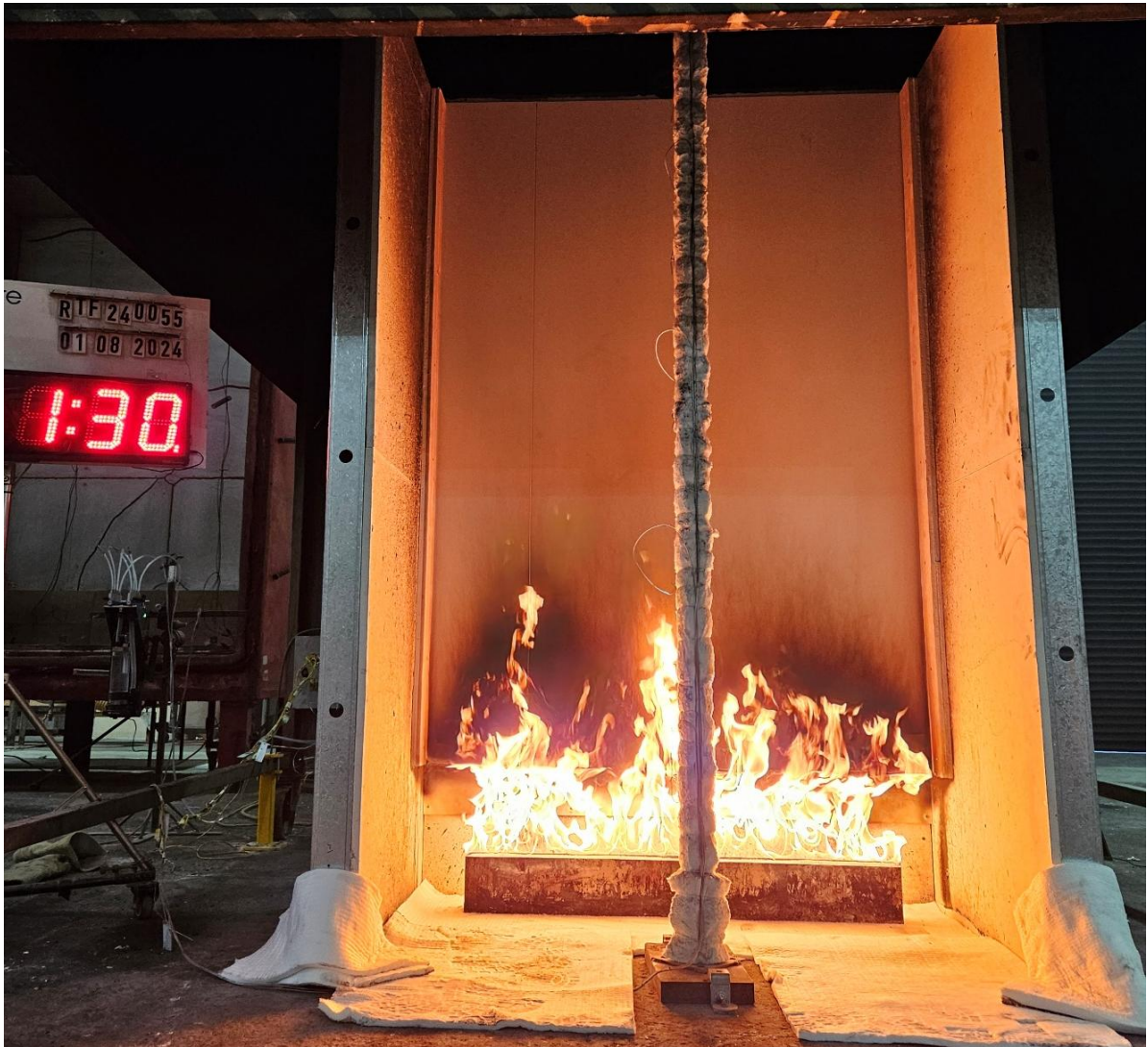
Figure 17 The specimen 1 minutes 30 seconds into the test (burner output at 100 kW)
