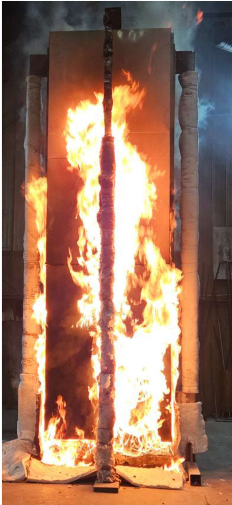
Figure 21 The specimen 5 minutes after the burner output was increased to 300 kW (20 minutes into the test)
