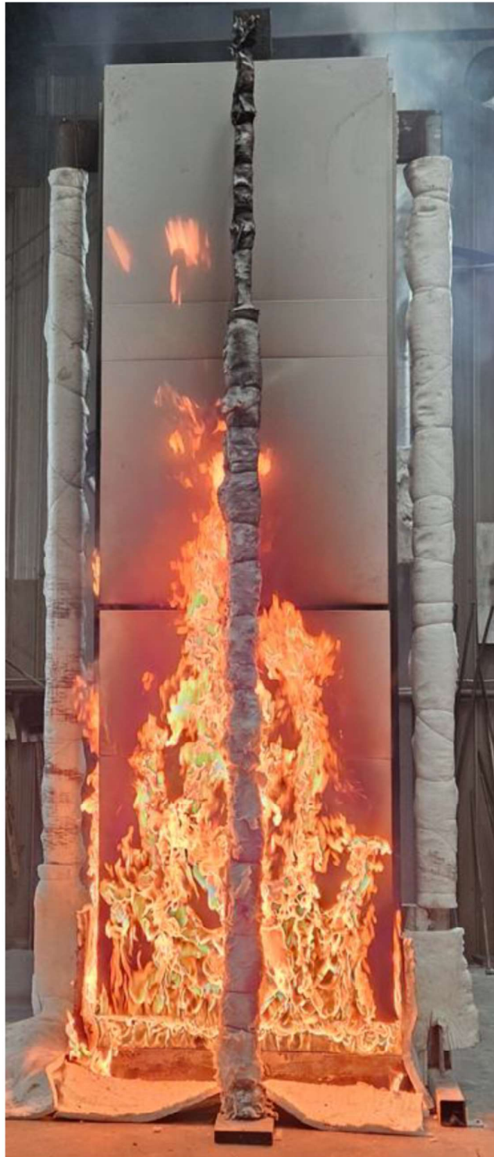
Figure 19 The specimen 1 minute after the burner output was increased to 300 kW (16 minutes into the test)
