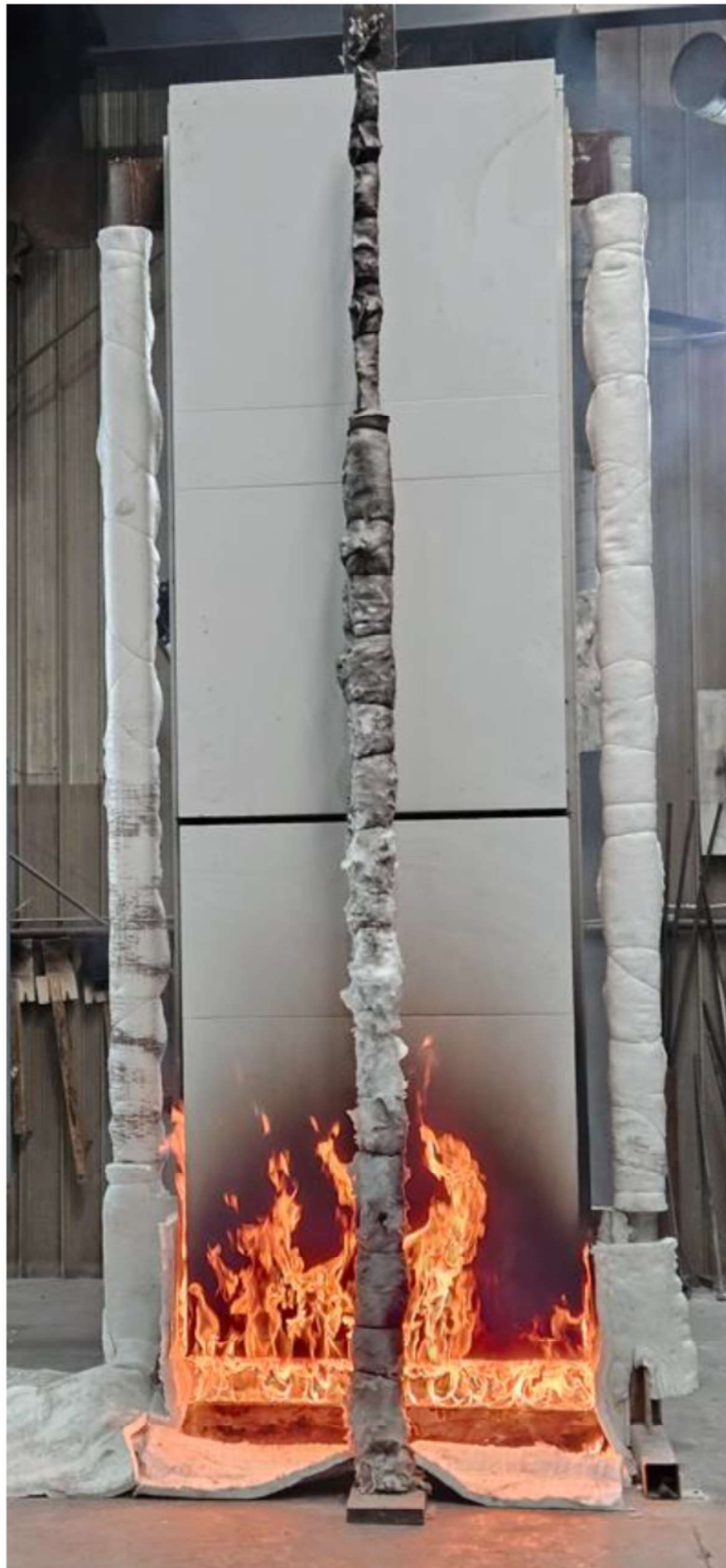
Figure 15 The specimen 4 minutes into the test at 100 kW
