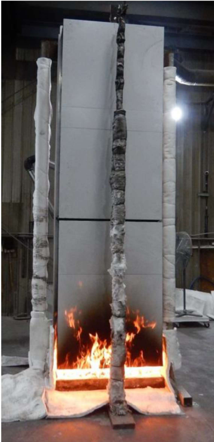
Figure 14 The specimen 1 minute into the test at 100 kW
