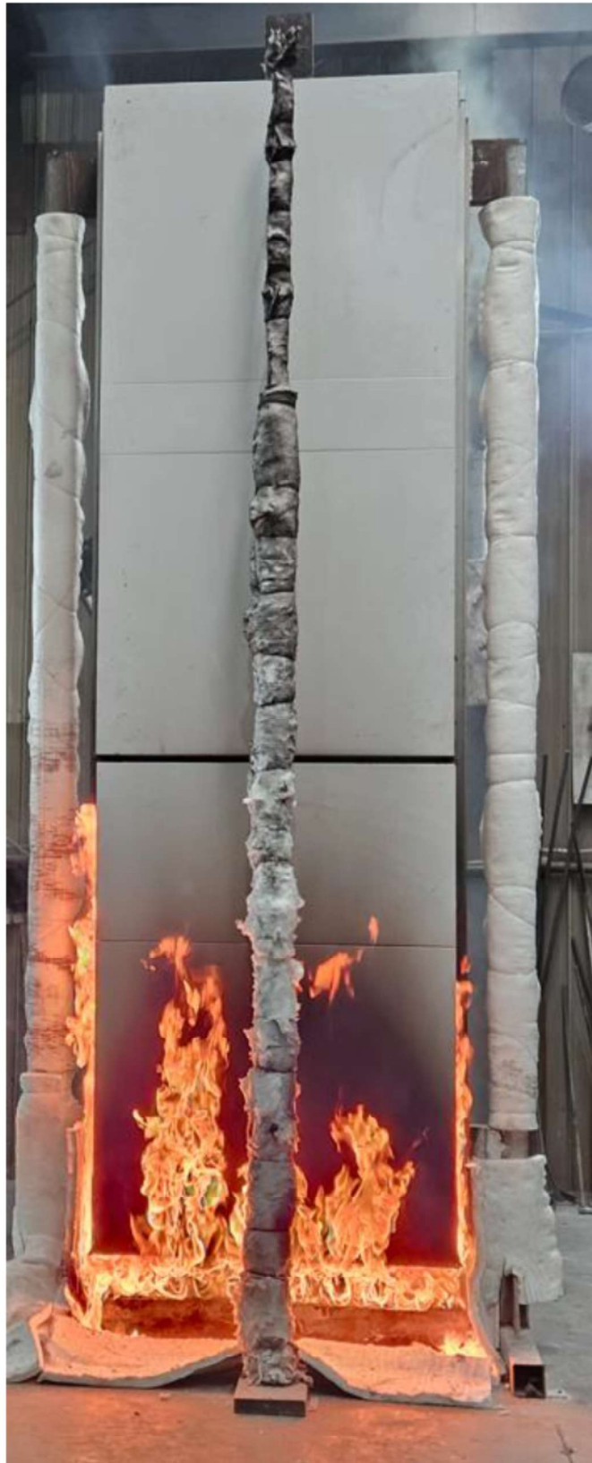
Figure 16 The specimen 7 minutes into the test at 100 kW
