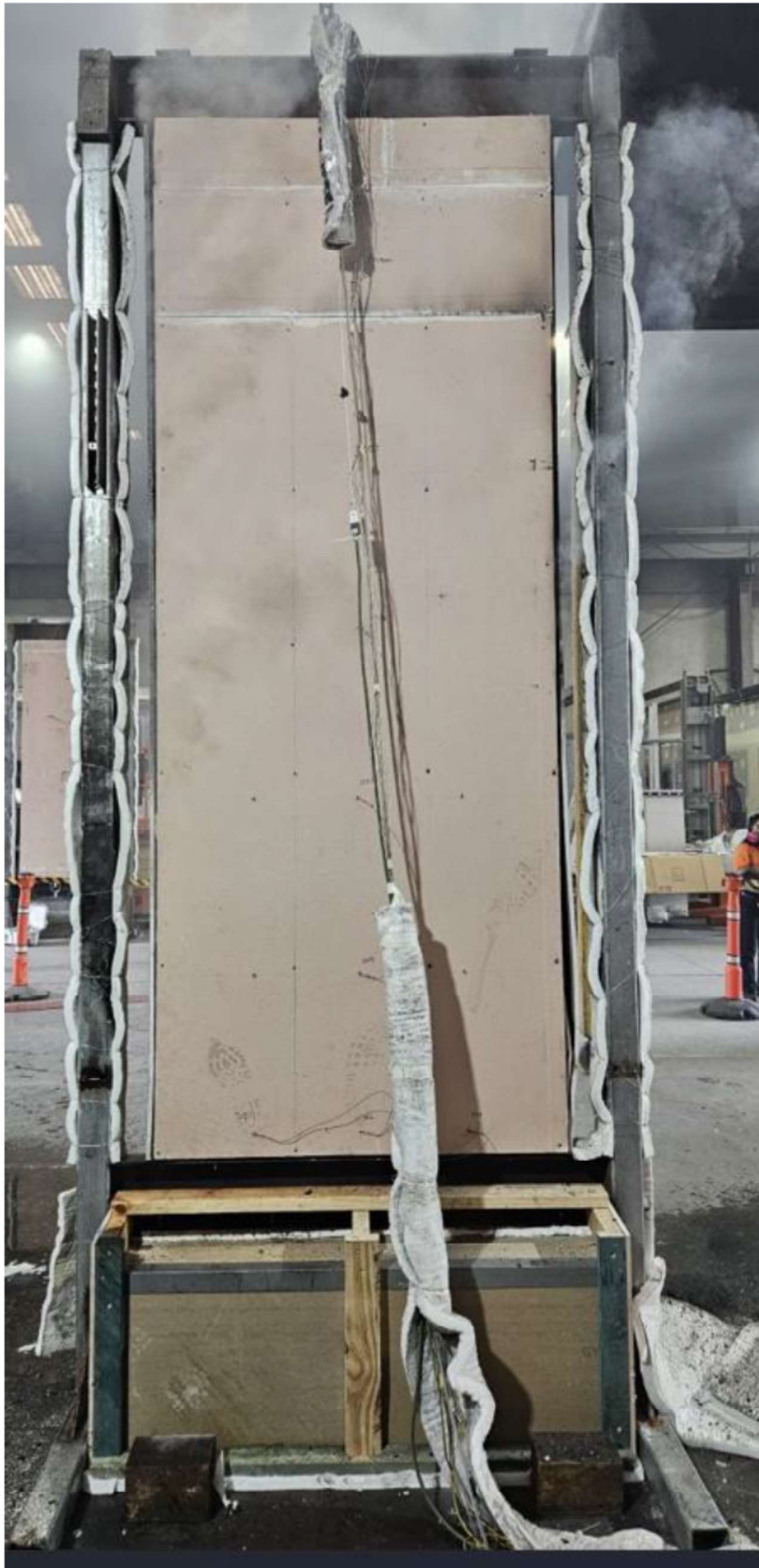
Figure 24 The unexposed face of the specimen after the end of the test
