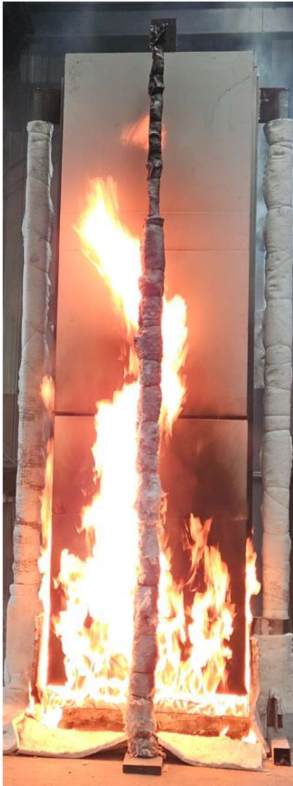
Figure 20 The specimen 2 minutes after the burner output was increased to 300 kW (17 minutes into the test)
