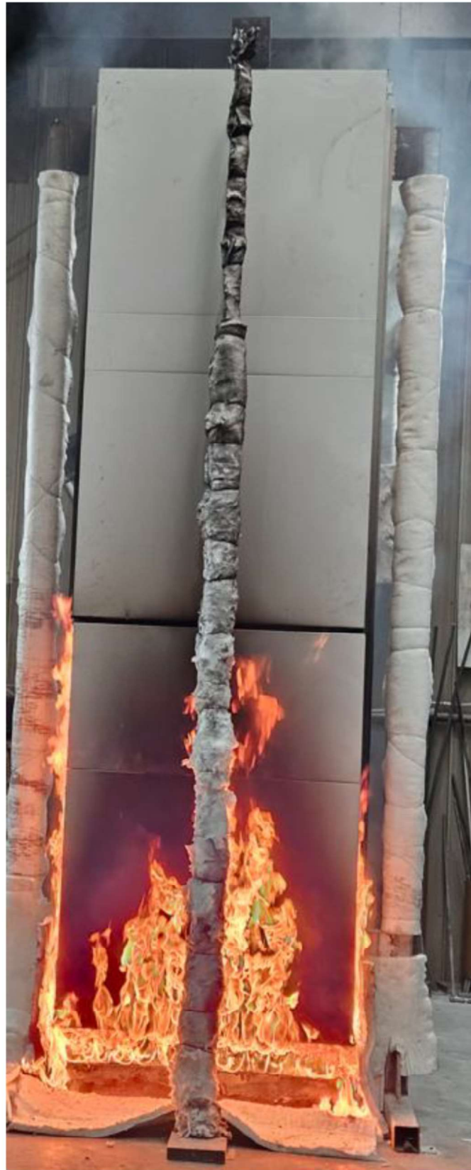
Figure 17 The specimen 10 minutes into the test at 100 kW
