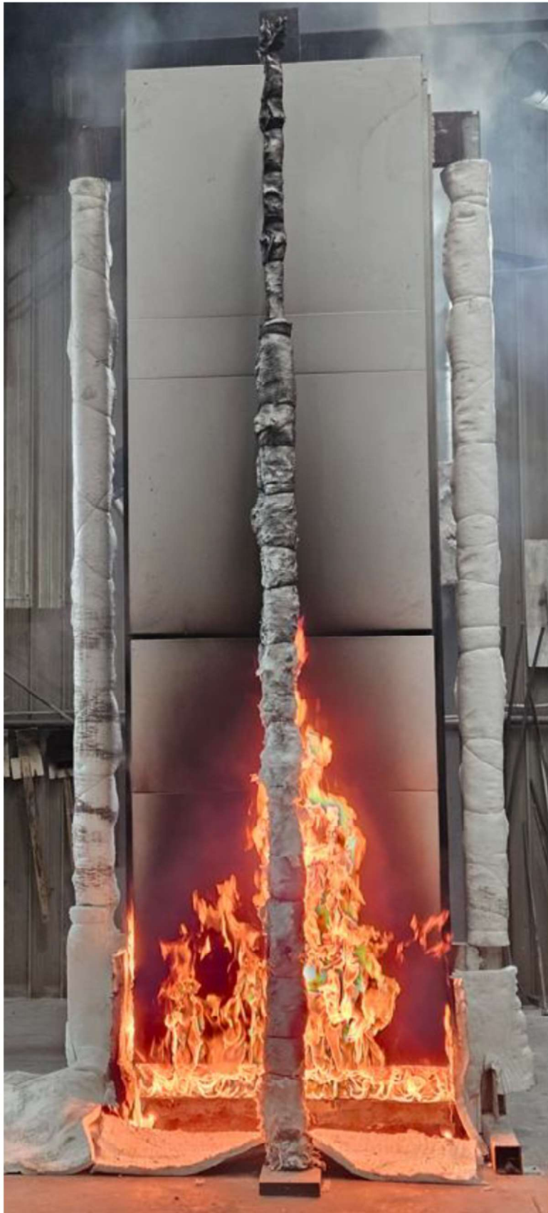
Figure 18 The specimen 14 minutes and 59 seconds into the test at 100 kW
