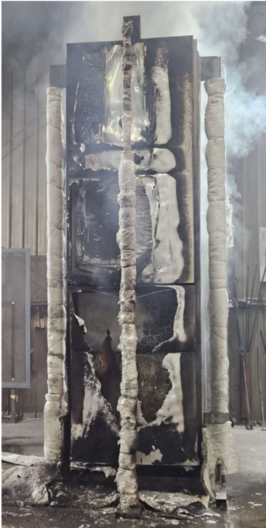
Figure 25 The exposed face of the specimen after the end of the test
