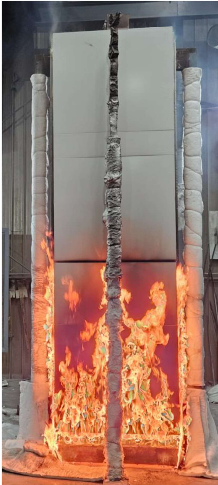
Figure 17 The specimen 10 minutes into the test at 200 kW
