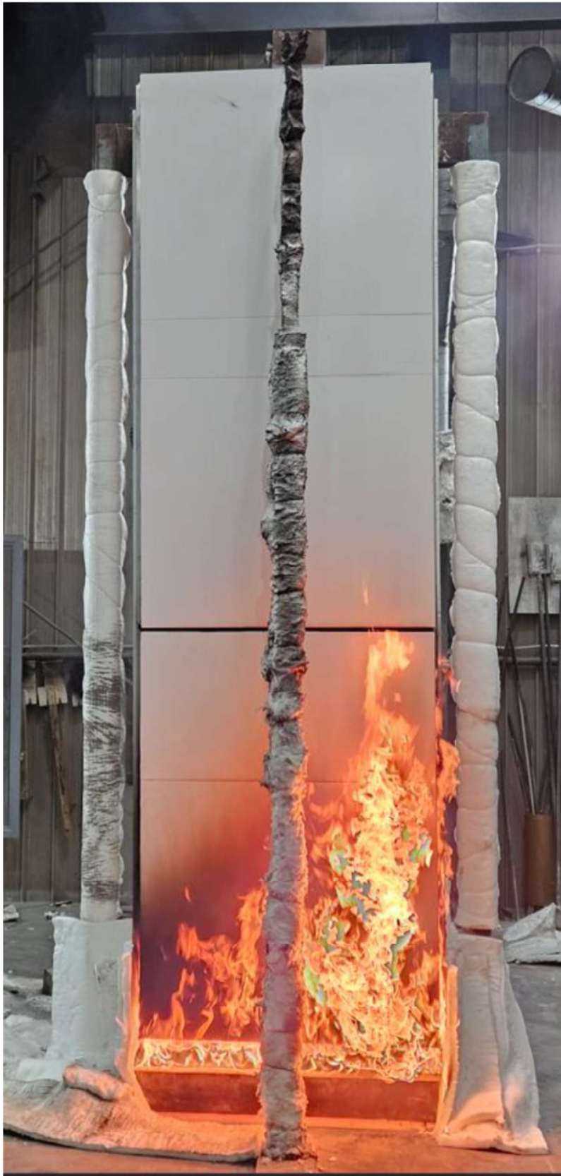
Figure 15 The specimen 3 minutes into the test at 200 kW
