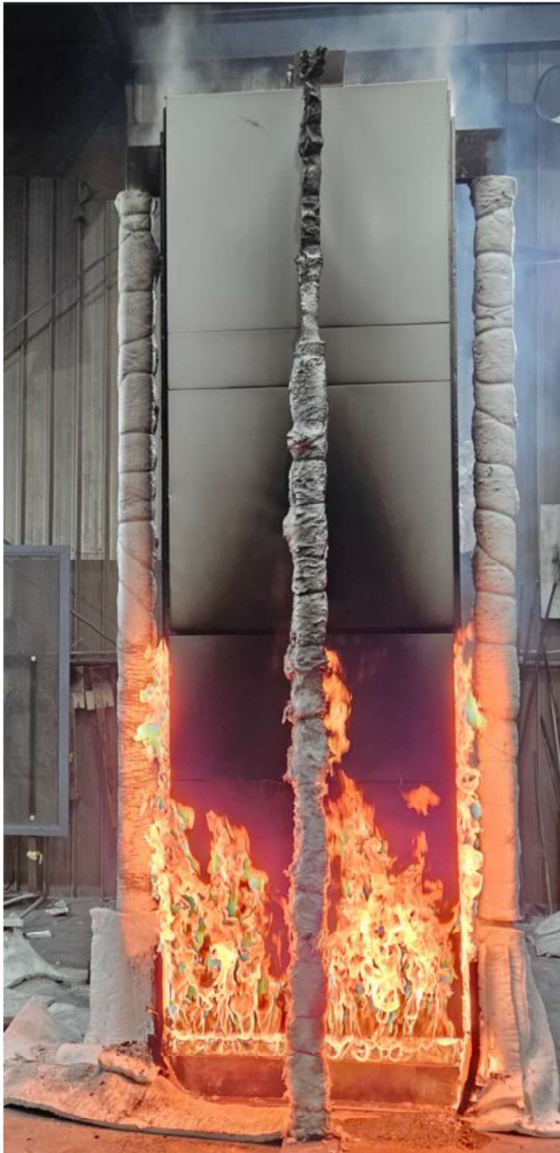
Figure 22 The specimen 35 minutes into the test at 200 kW
