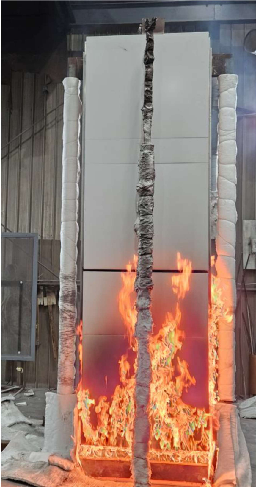
Figure 16 The specimen 5 minutes into the test at 200 kW
