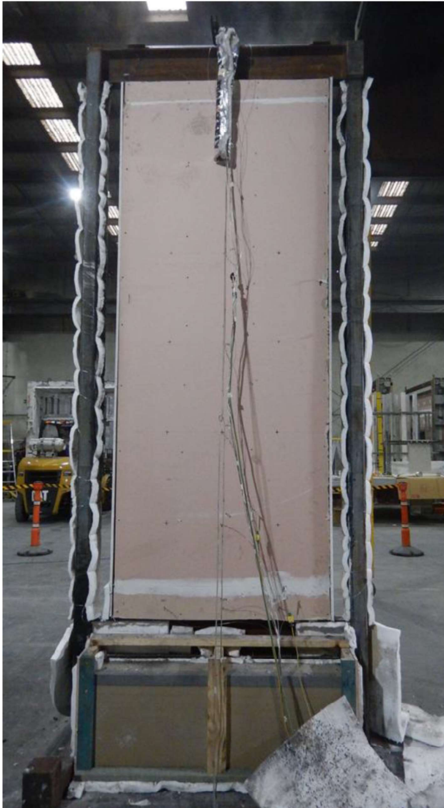
Figure 26 The unexposed face of the specimen after the end of the test
