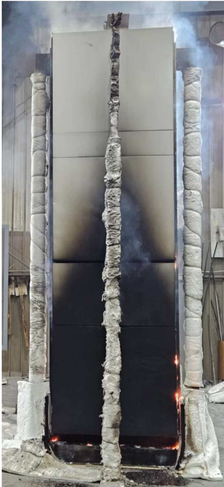
Figure 24 The specimen 42 minutes into the test
