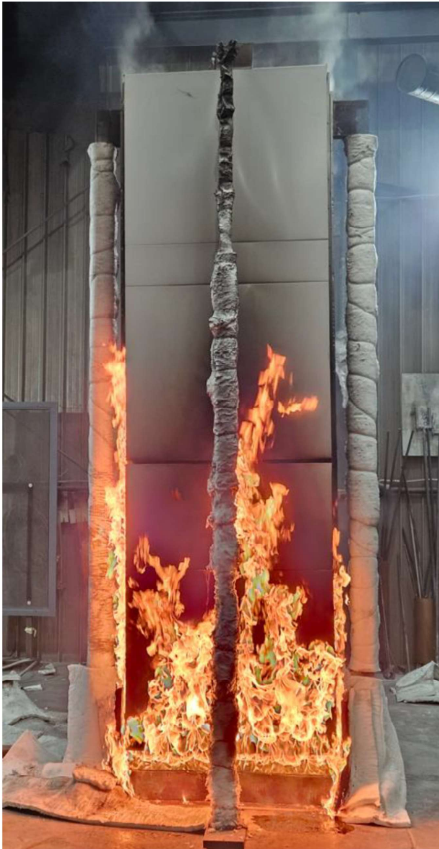
Figure 19 The specimen 20 minutes into the test at 200 kW
