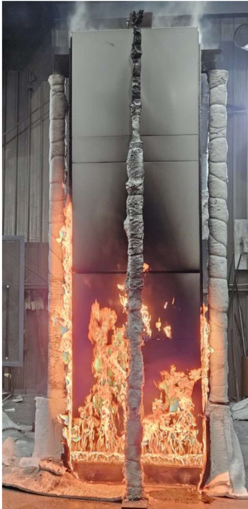
Figure 20 The specimen 26 minutes into the test at 200 kW
