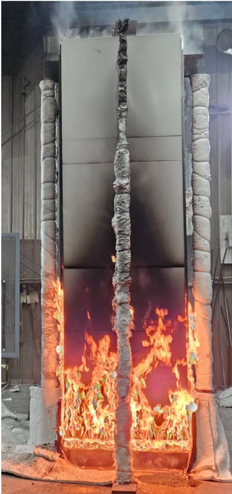
Figure 21 The specimen 30 minutes into the test at 200 kW
