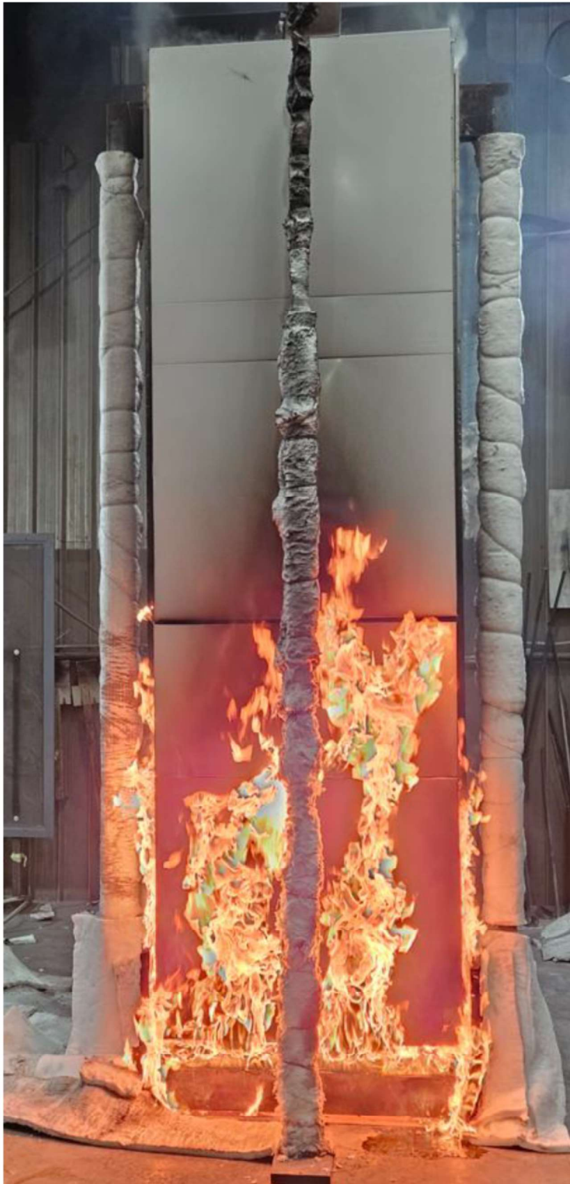
Figure 18 The specimen 15 minutes into the test at 200 kW
