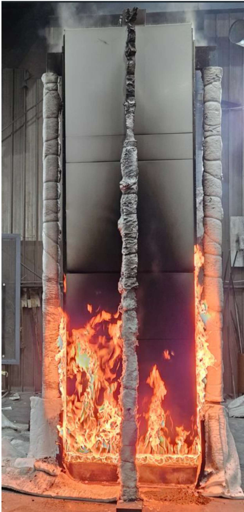
Figure 23 The specimen at the end of the 40 minute exposure period at 200 kW
