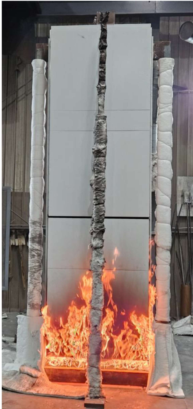
Figure 14 The specimen 1 minute into the test at 200 kW
