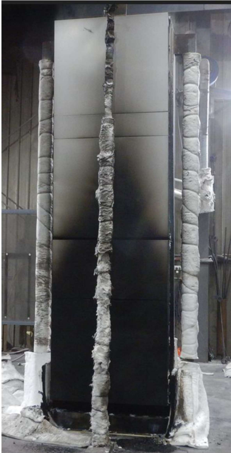
Figure 25 The exposed face of the specimen after the end of the test
