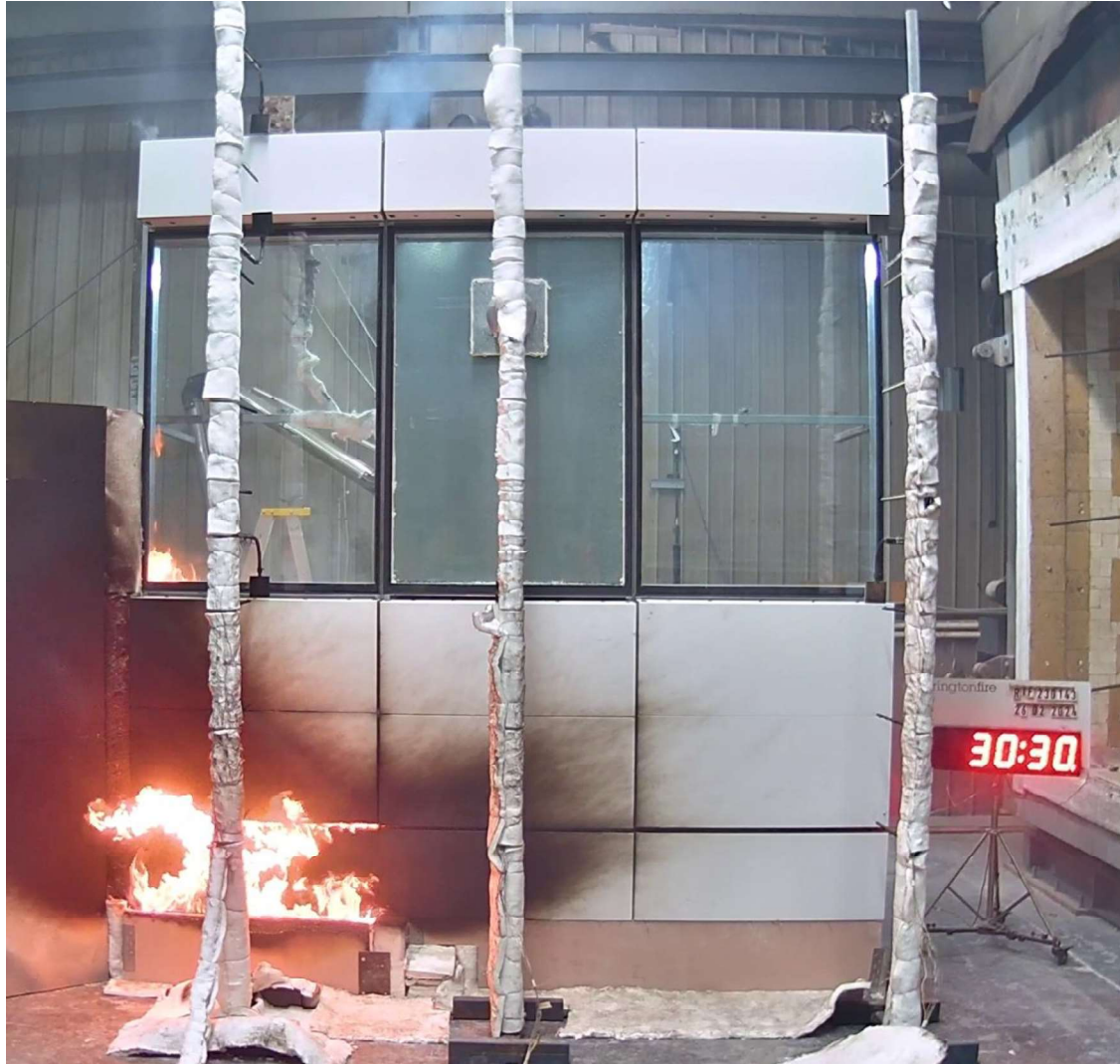
Figure 38 The specimen 30 minutes 30 seconds into the test (30 seconds after burner off and wind on).
