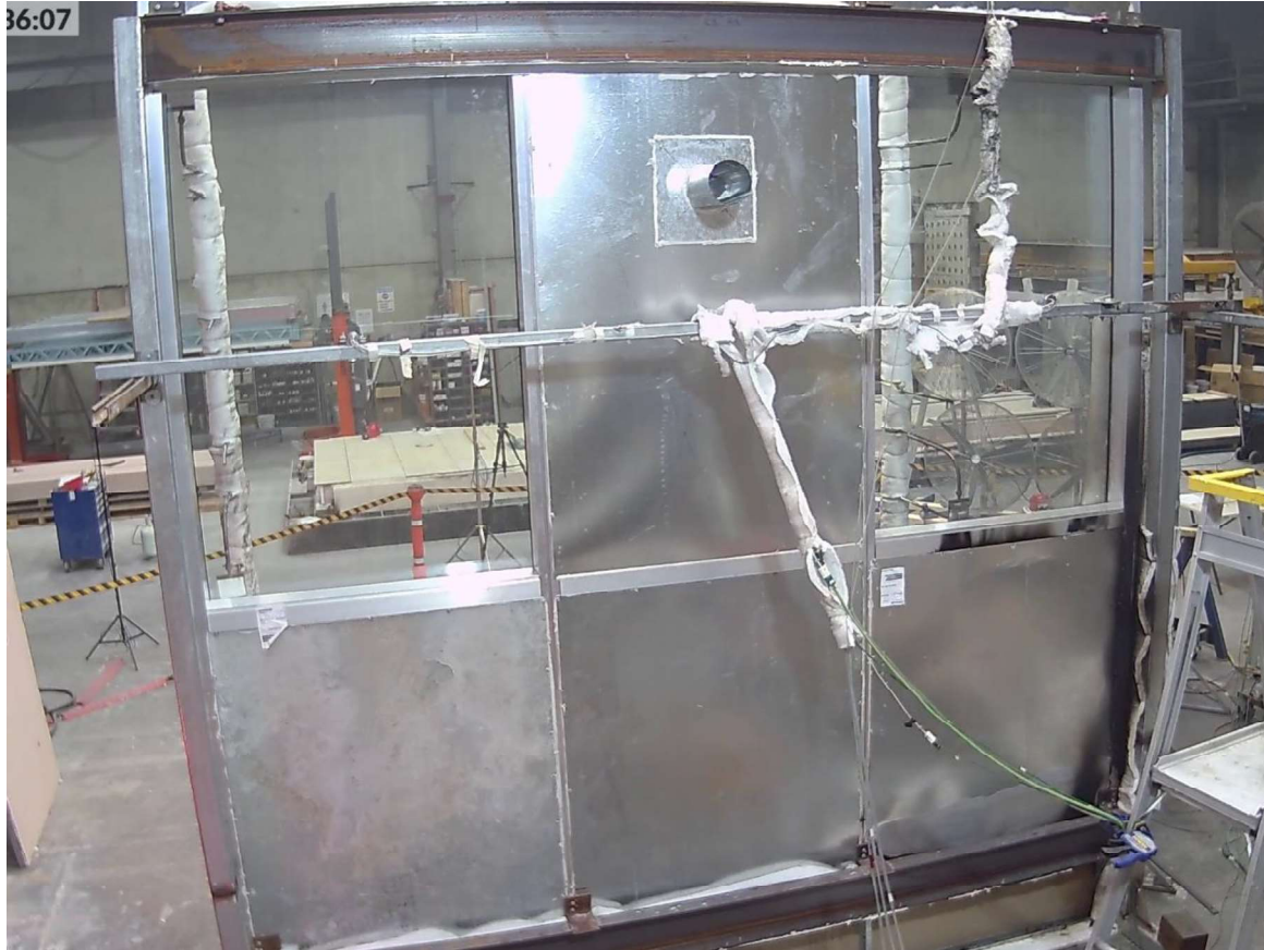
Figure 49 The unexposed side of the specimen at the end of test.
