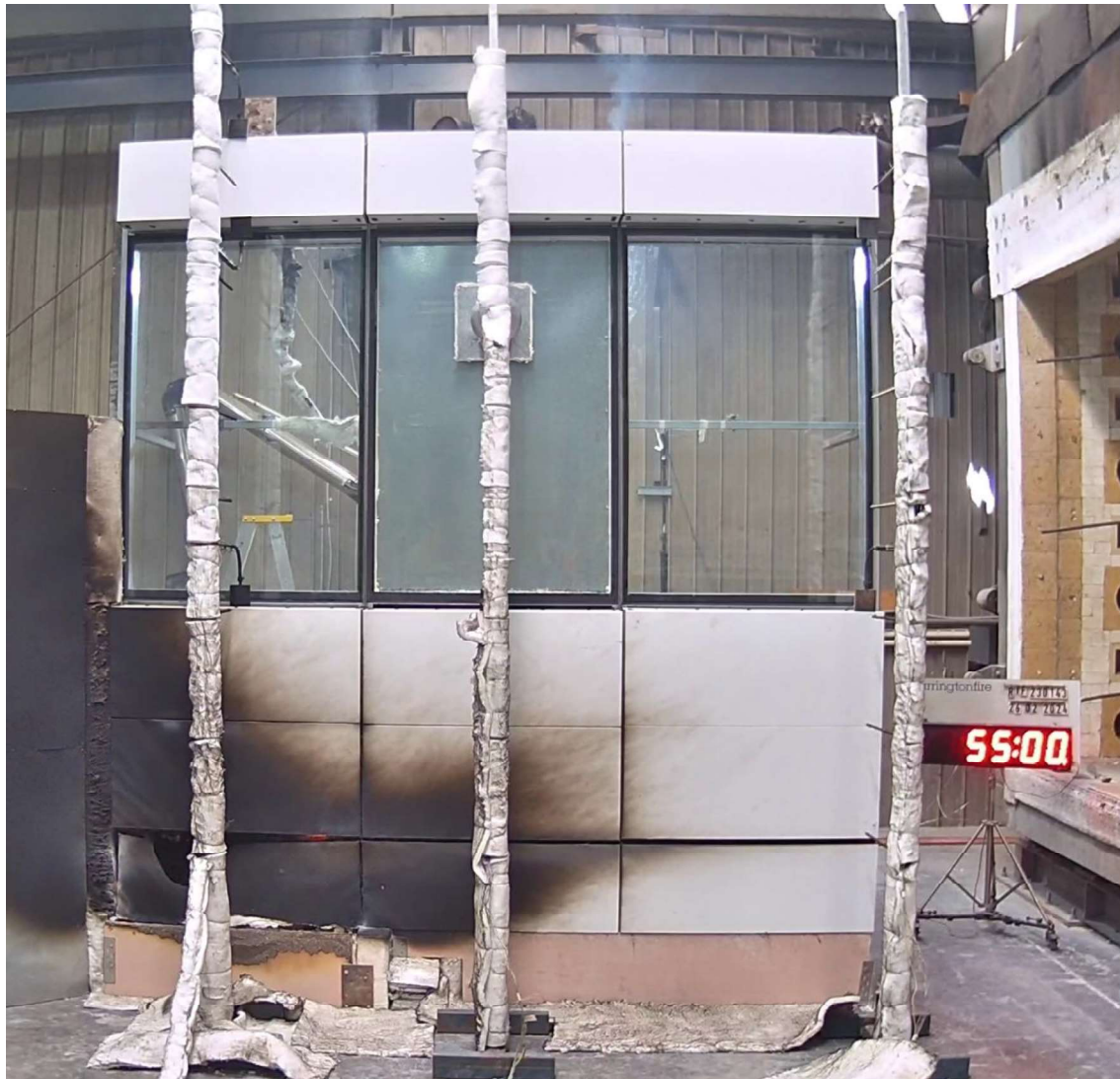
Figure 47 The specimen 55 minutes into the test (25 minutes after burner off and 2 minutes 20 seconds after wind off).
