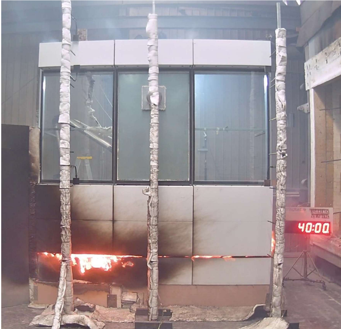
Figure 43 The specimen 40 minutes into the test (10 minutes after burner off and wind on).
