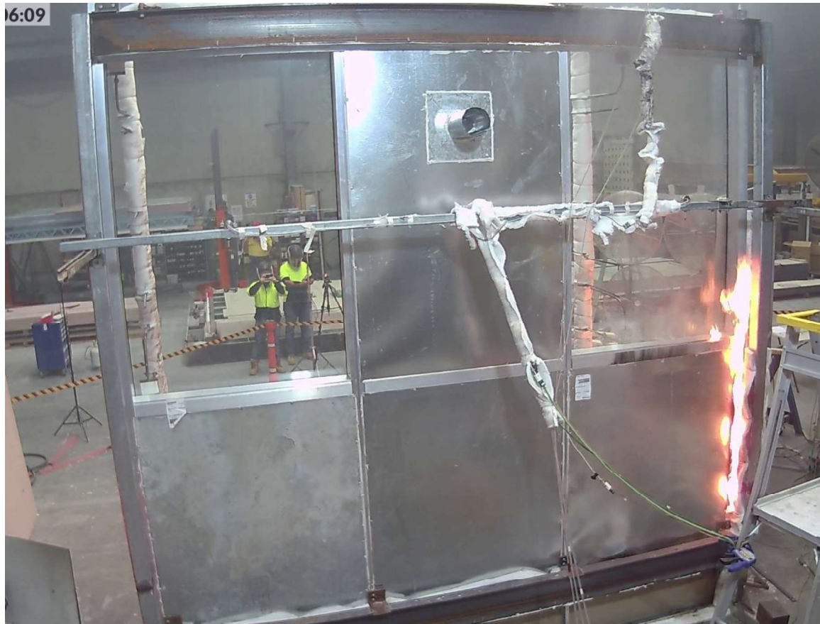
Figure 35 Unexposed side of the specimen 30 minutes into the test (burner off and wind on).
