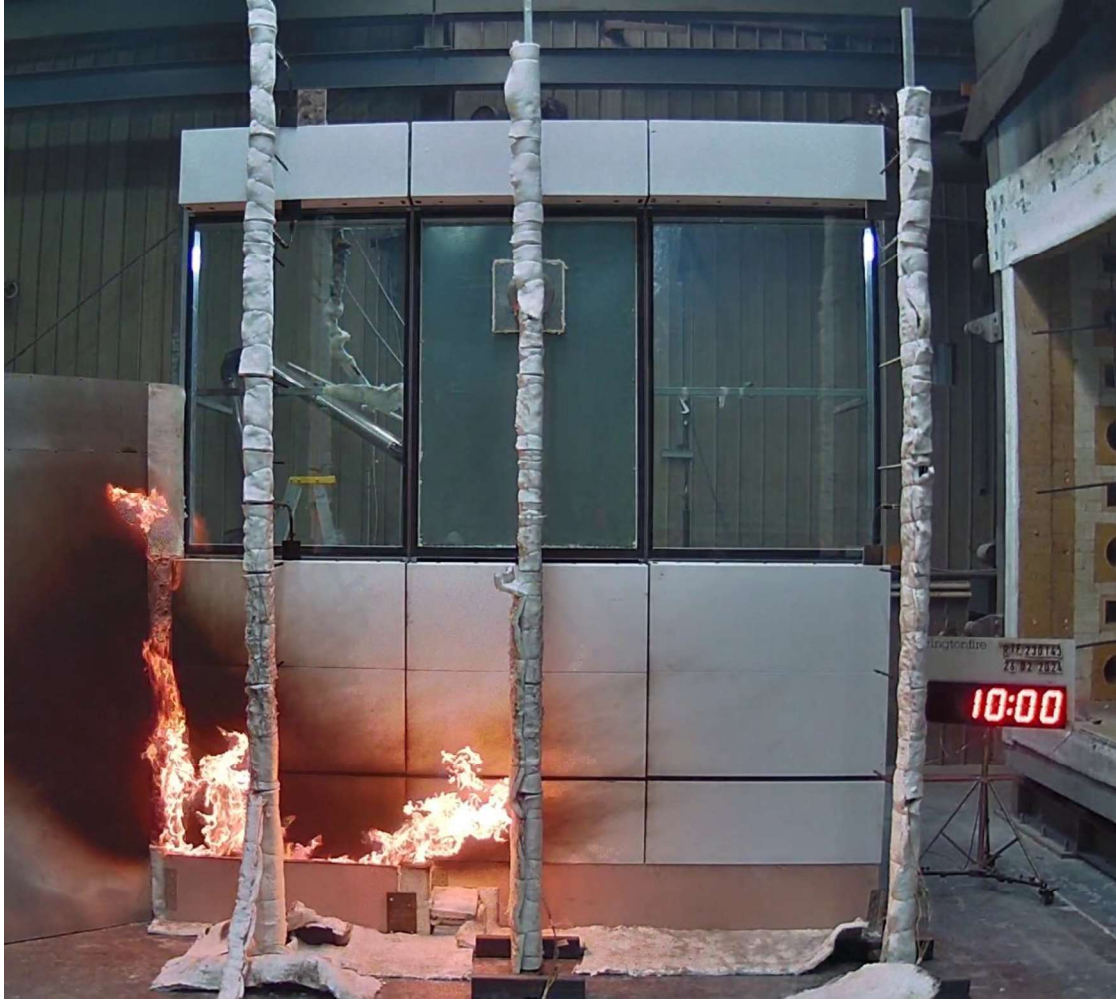
Figure 30 The specimen 10 minutes into the test (burner output at 300 kW and wind on).
