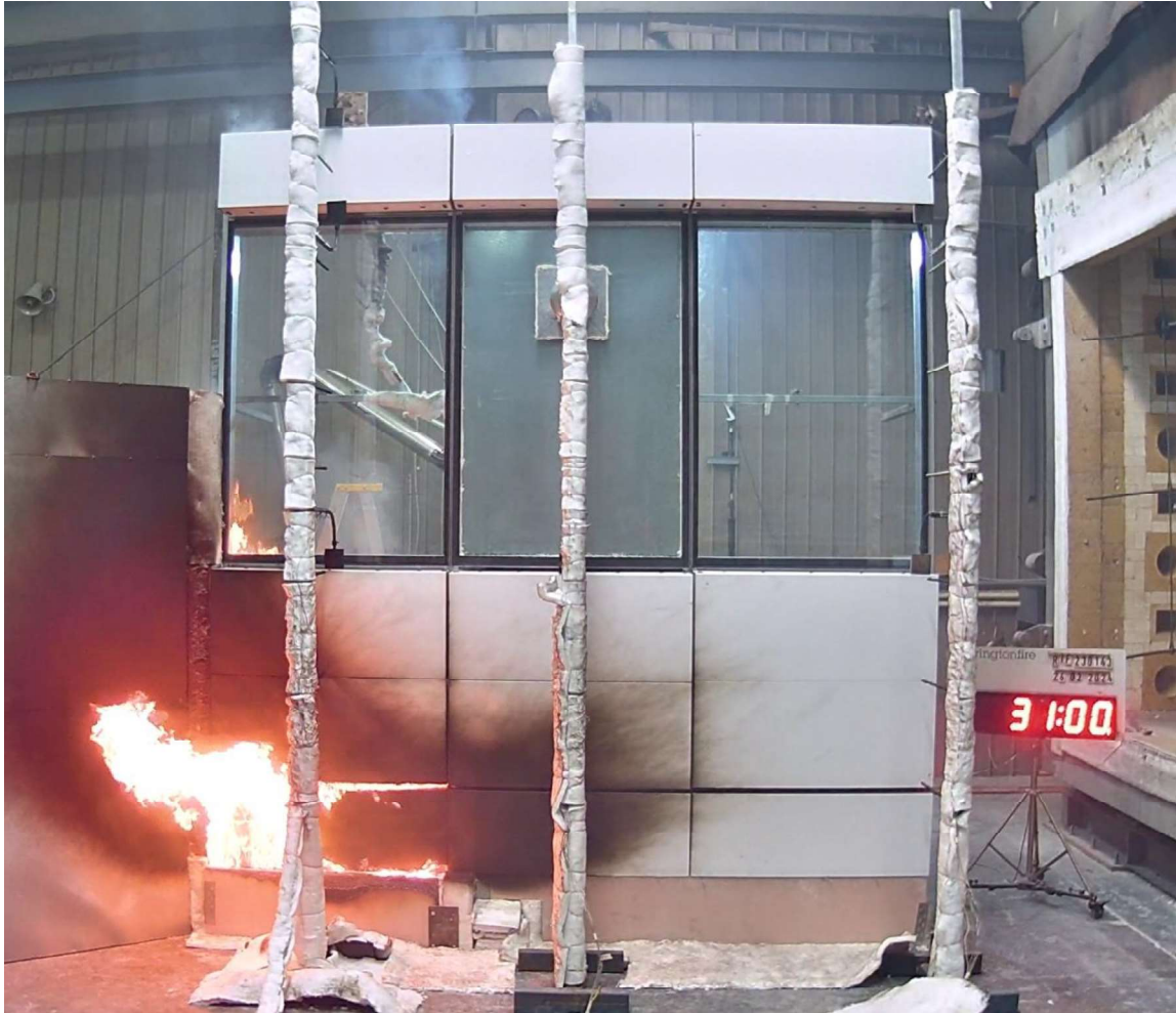
Figure 39 The specimen 31 minutes into the test (1 minute after burner off and wind on).
