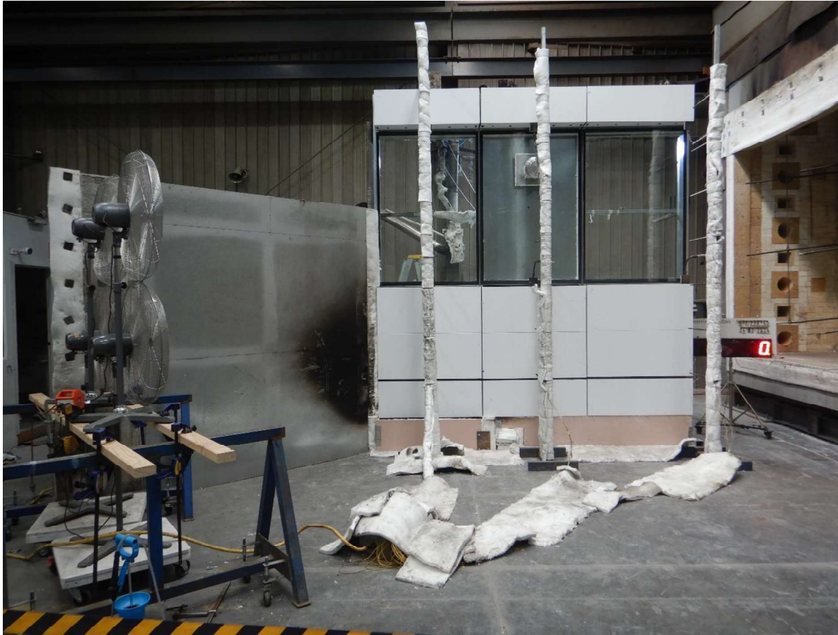
Figure 23 The specimen and test setup (angled - exposed side) before the reaction to fire test
