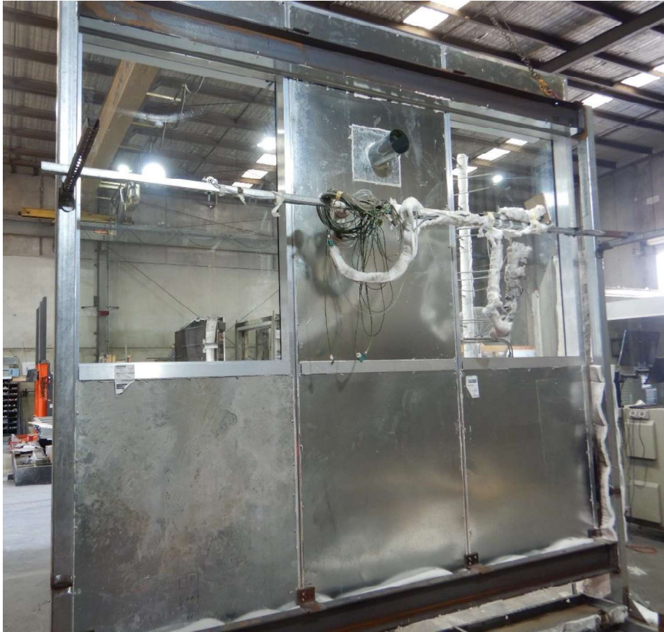
Figure 25 The specimen before the reaction to fire test - unexposed side.
