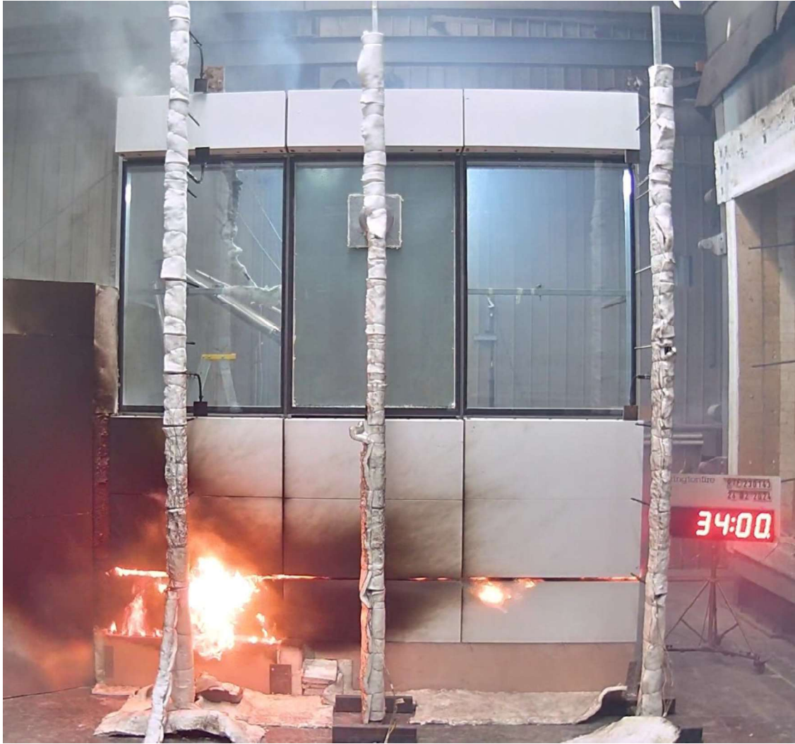
Figure 41 The specimen 34 minutes into the test (4 minutes after burner off and wind on).
