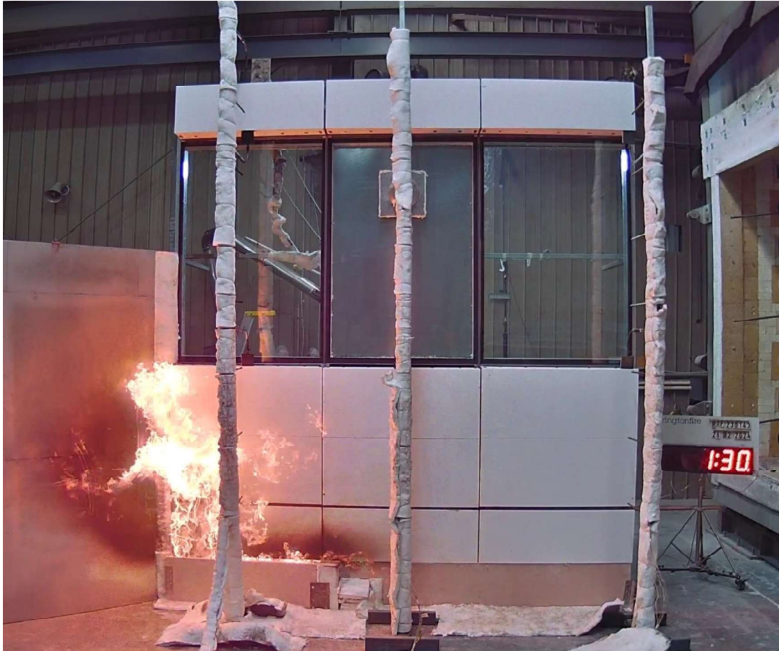
Figure 26 The specimen 1 minute 30 seconds into the test (burner output at 300 kW and wind on)
