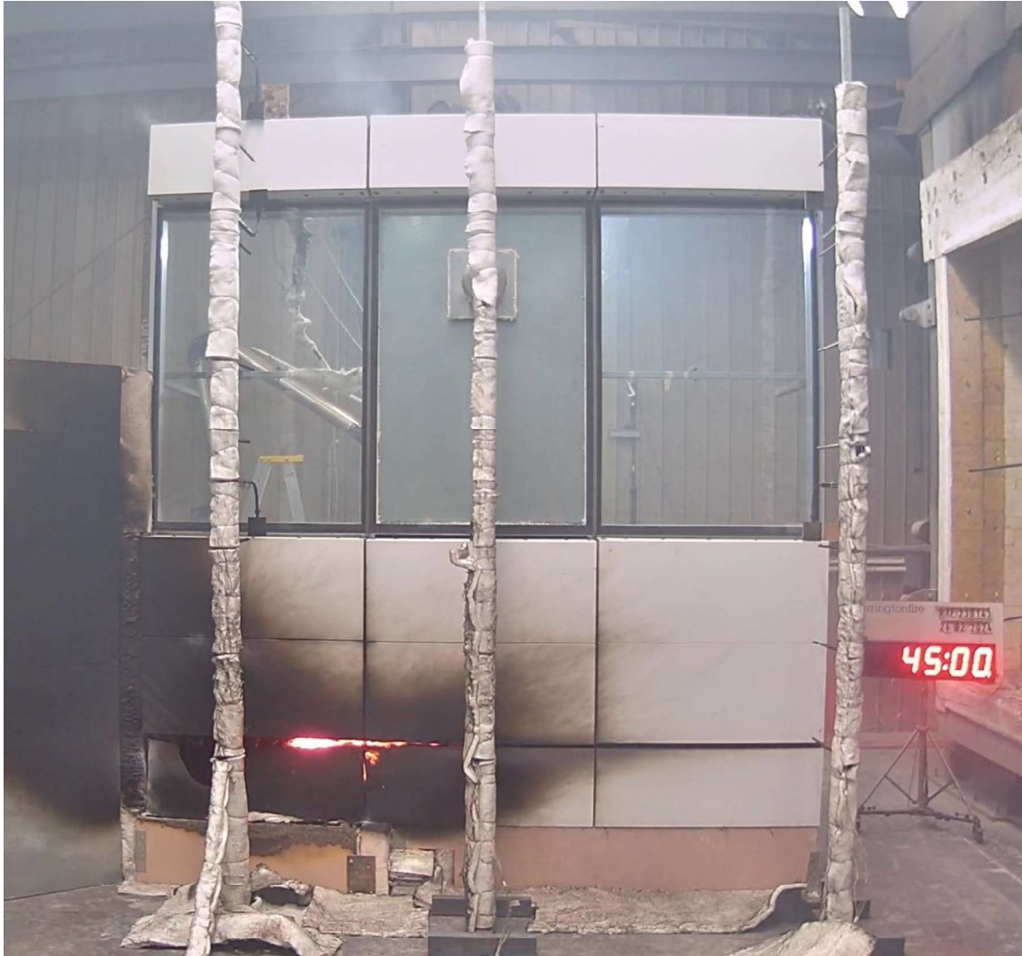
Figure 44 The specimen 45 minutes into the test (15 minutes after burner off and wind on).
