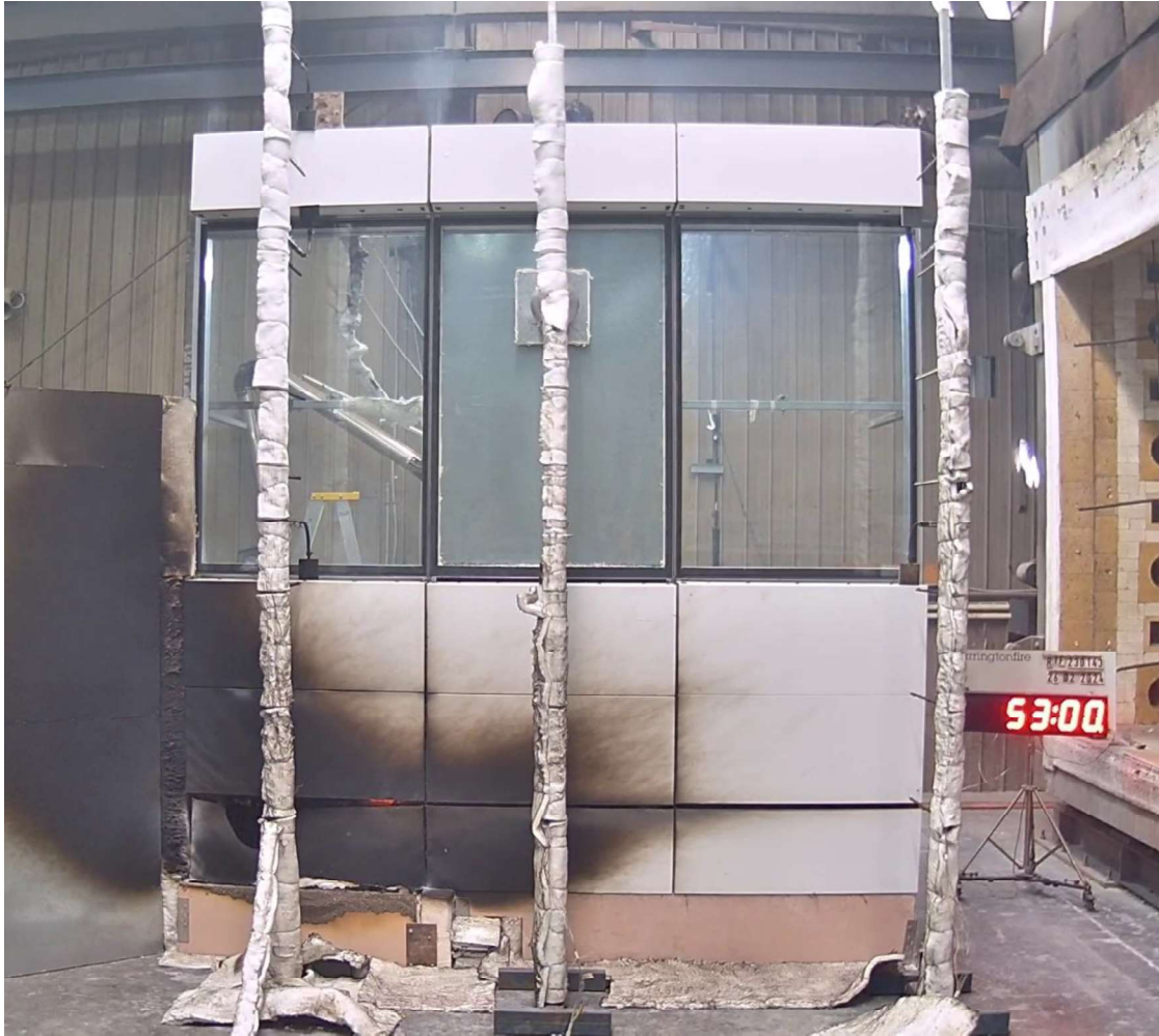
Figure 46 The specimen 53 minutes into the test (23 minutes after burner off and 20 seconds after wind off).
