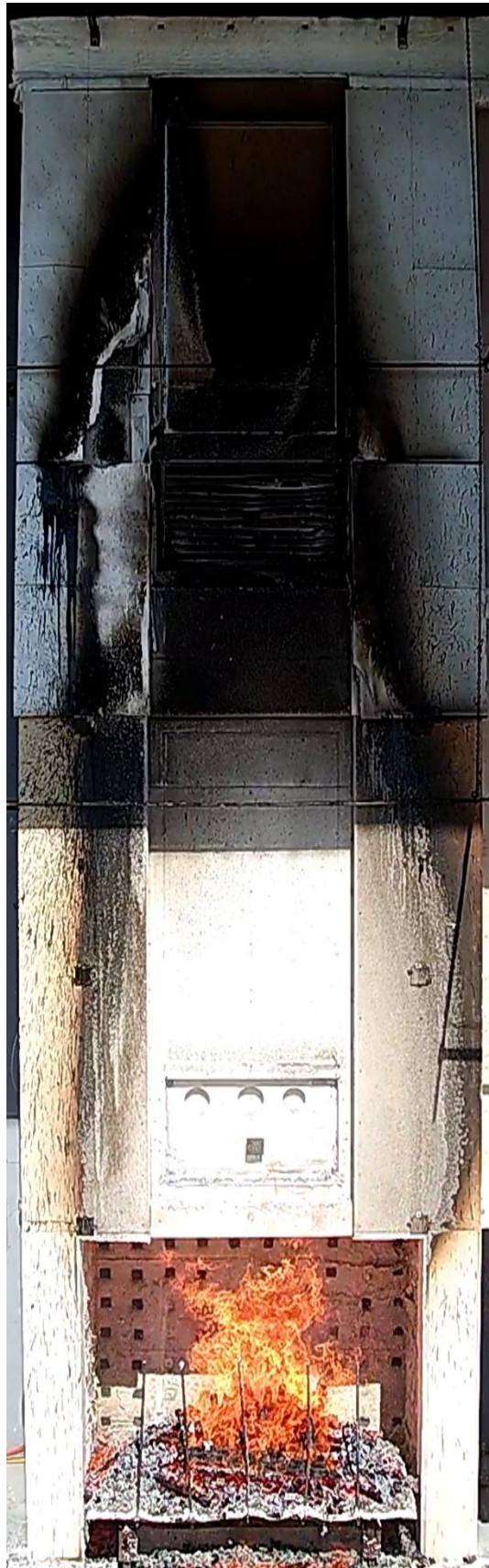
Figure 41 The external wall system during the test – 30 minutes after crib ignition
