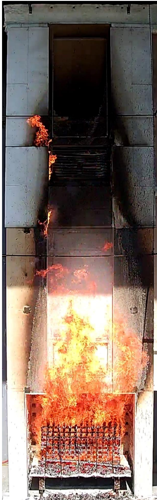
Figure 39 The external wall system during the test – 20 minutes after crib ignition
