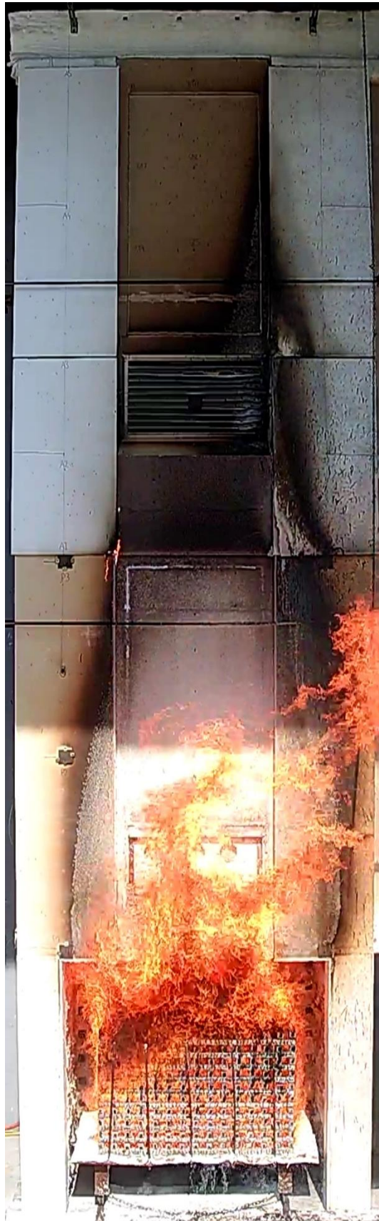
Figure 38 The external wall system during the test – 15 minutes after crib ignition
