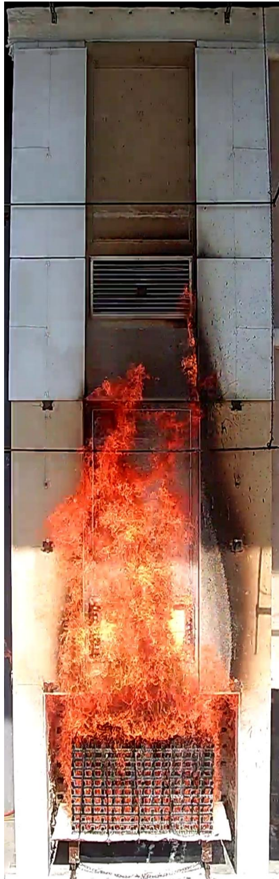
Figure 37 The external wall system during the test – 10 minutes after crib ignition
