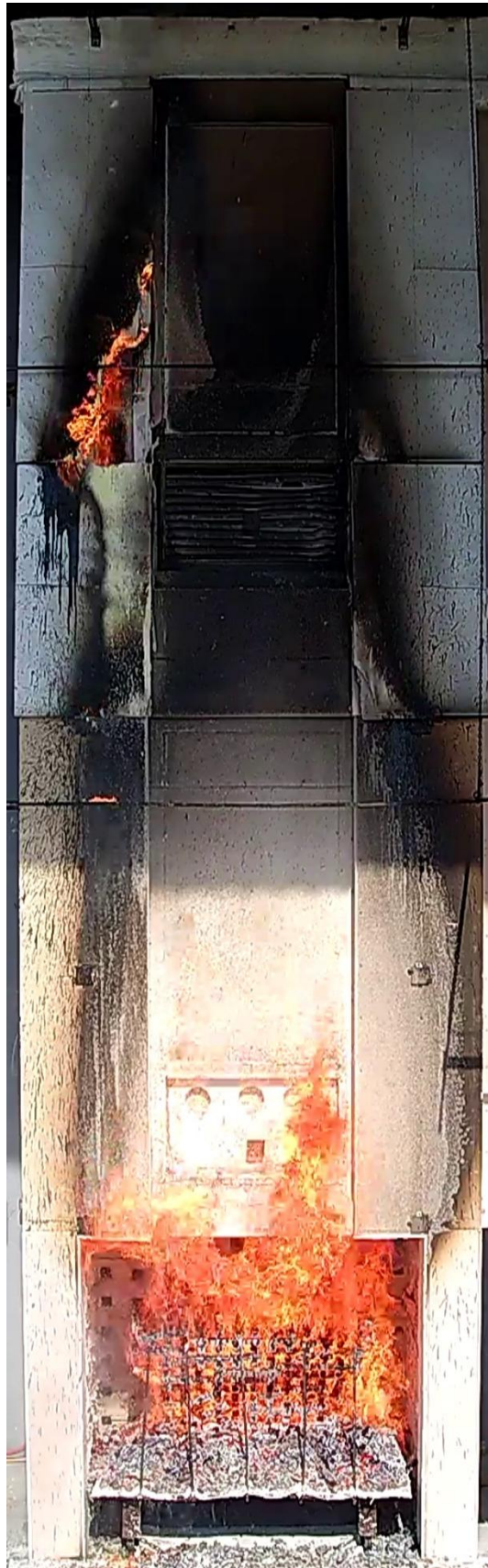
Figure 40 The external wall system during the test – 25 minutes after crib ignition
