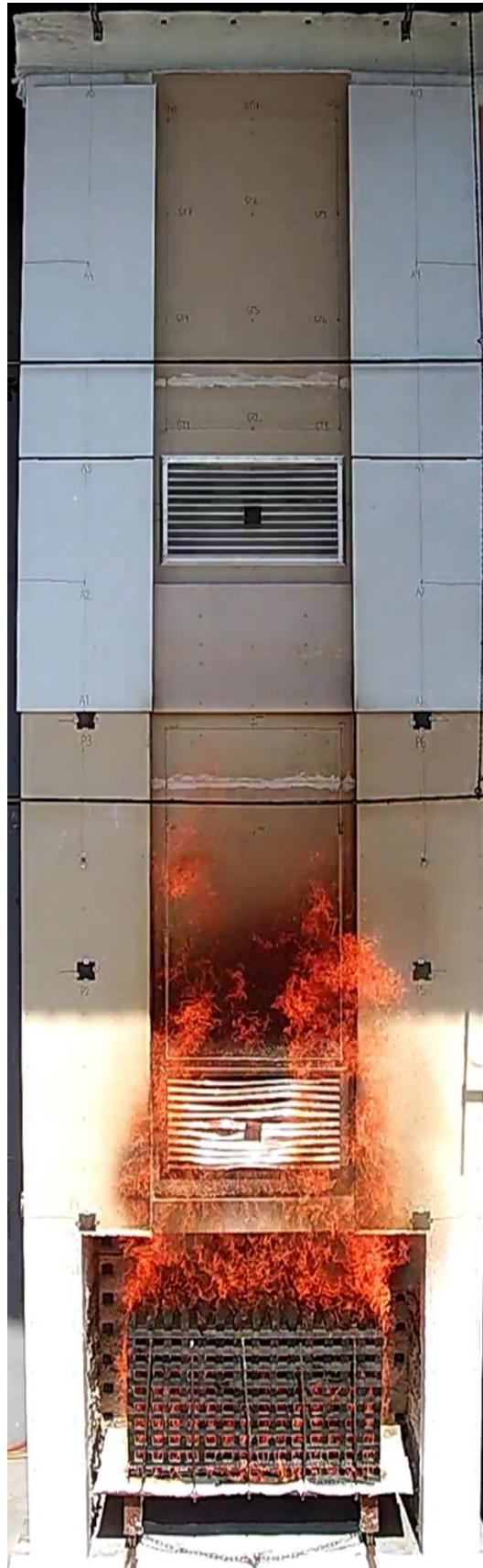
Figure 36 The external wall system during the test – 5 minutes after crib ignition
