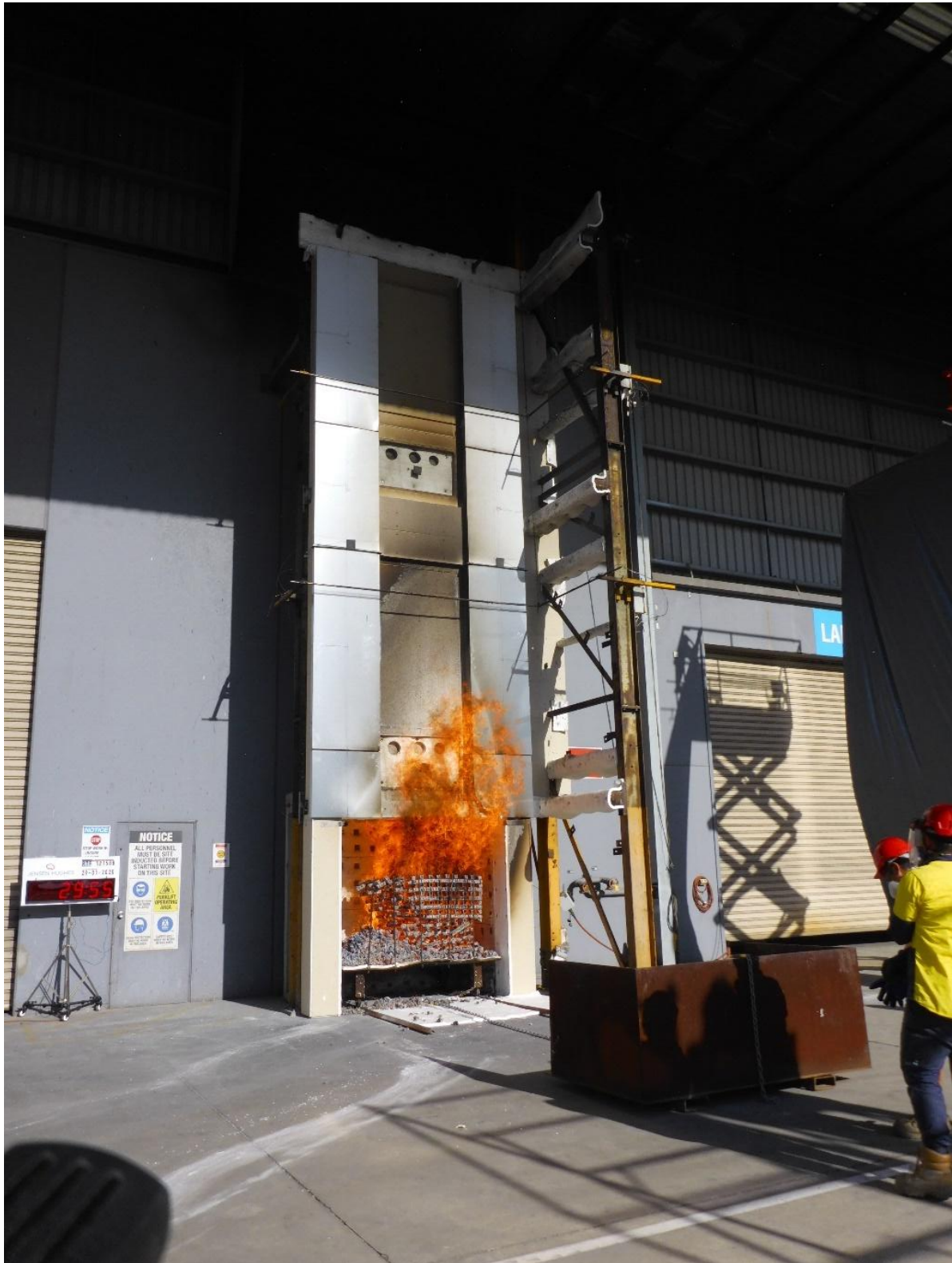
Figure 46 The external wall system during the test – 29 minutes 55 seconds after crib ignition
