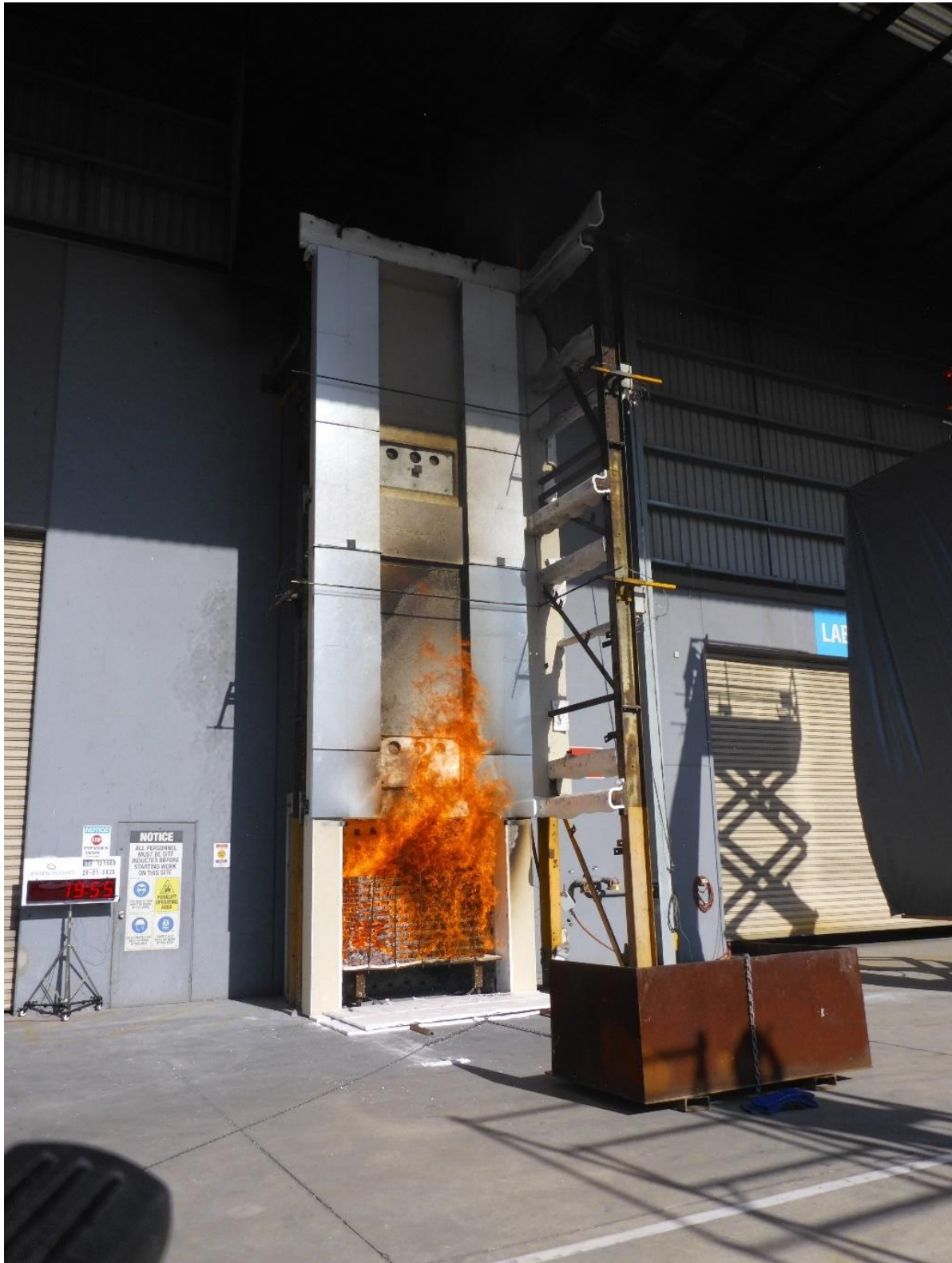
Figure 44 The external wall system during the test – 19 minutes 55 seconds after crib ignition
