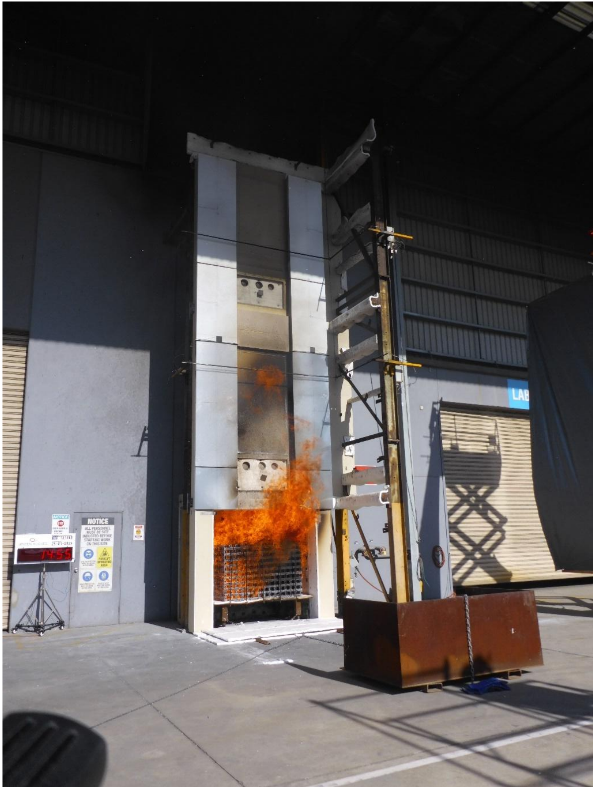
Figure 43 The external wall system during the test – 14 minutes 55 seconds after crib ignition
