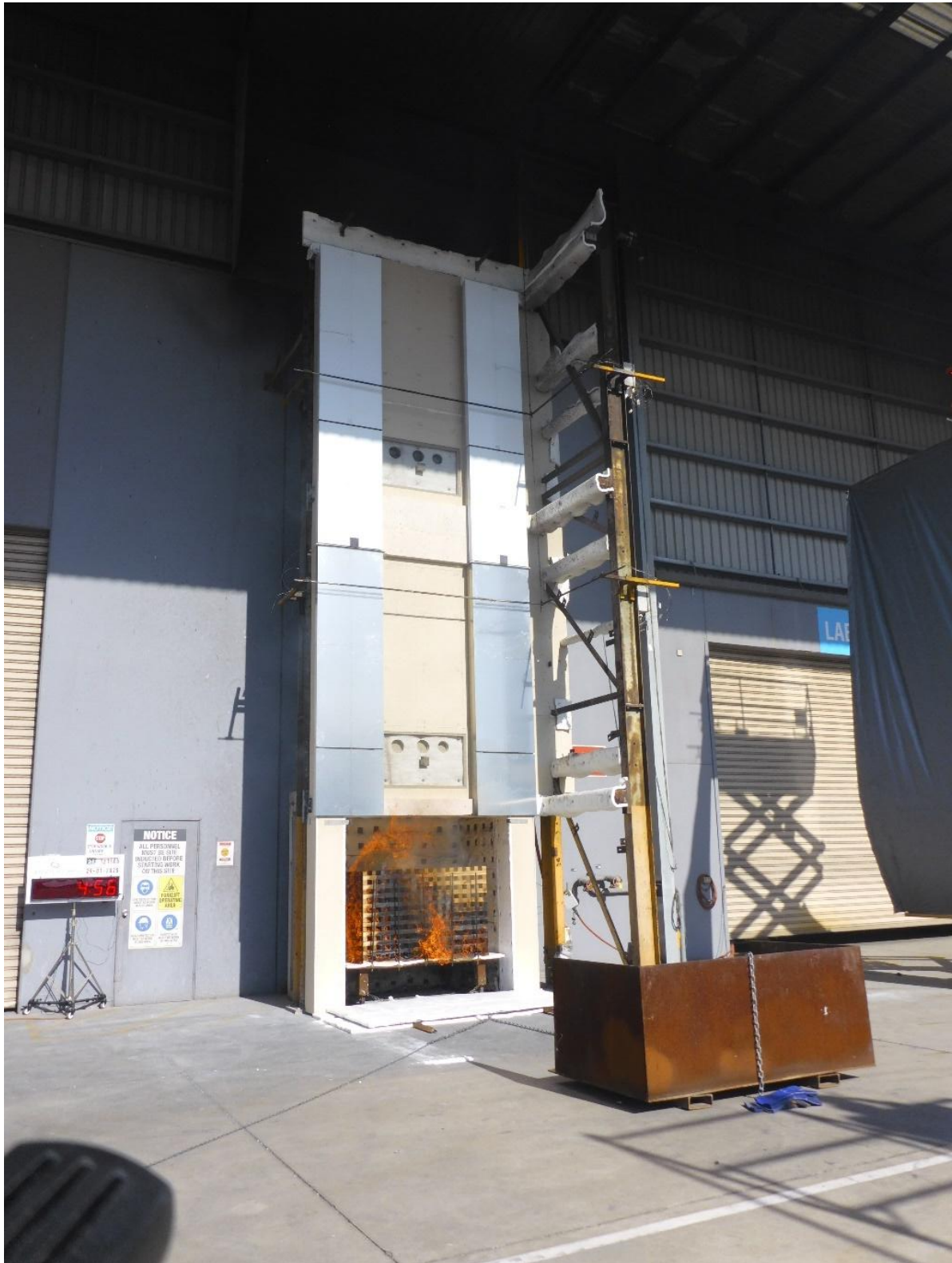
Figure 41 The external wall system during the test – 4 minutes 56 seconds after crib ignition
