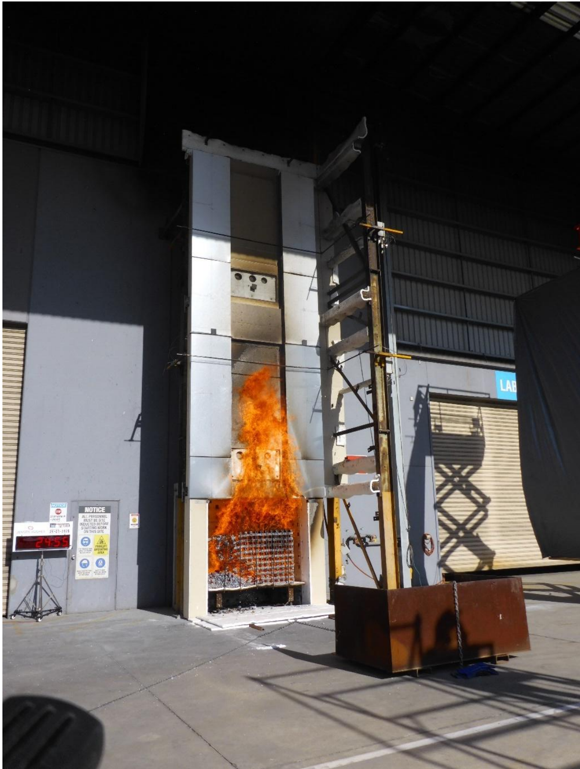
Figure 45 The external wall system during the test – 24 minutes 55 seconds after crib ignition
