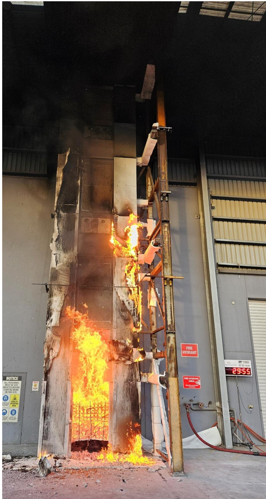
Figure 51 The external wall system during the test – 29 minutes 55 seconds after crib ignition
