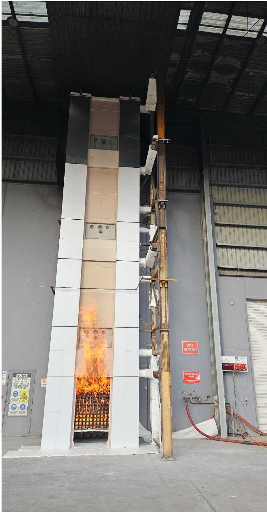
Figure 46 The external wall system during the test – 6 minutes after crib ignition
