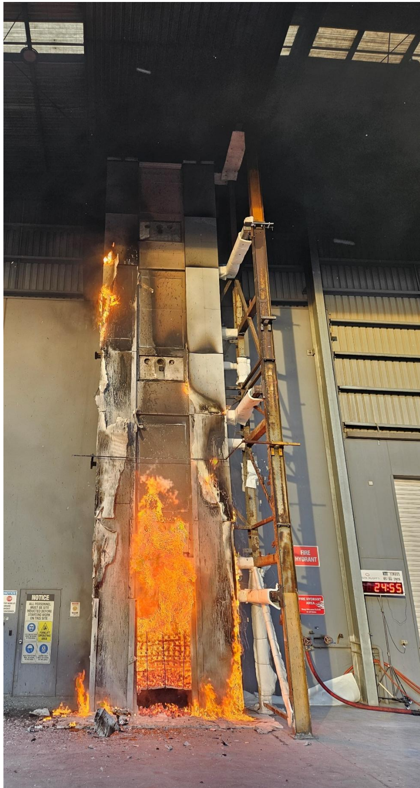
Figure 50 The external wall system during the test – 24 minutes 55 seconds after crib ignition
