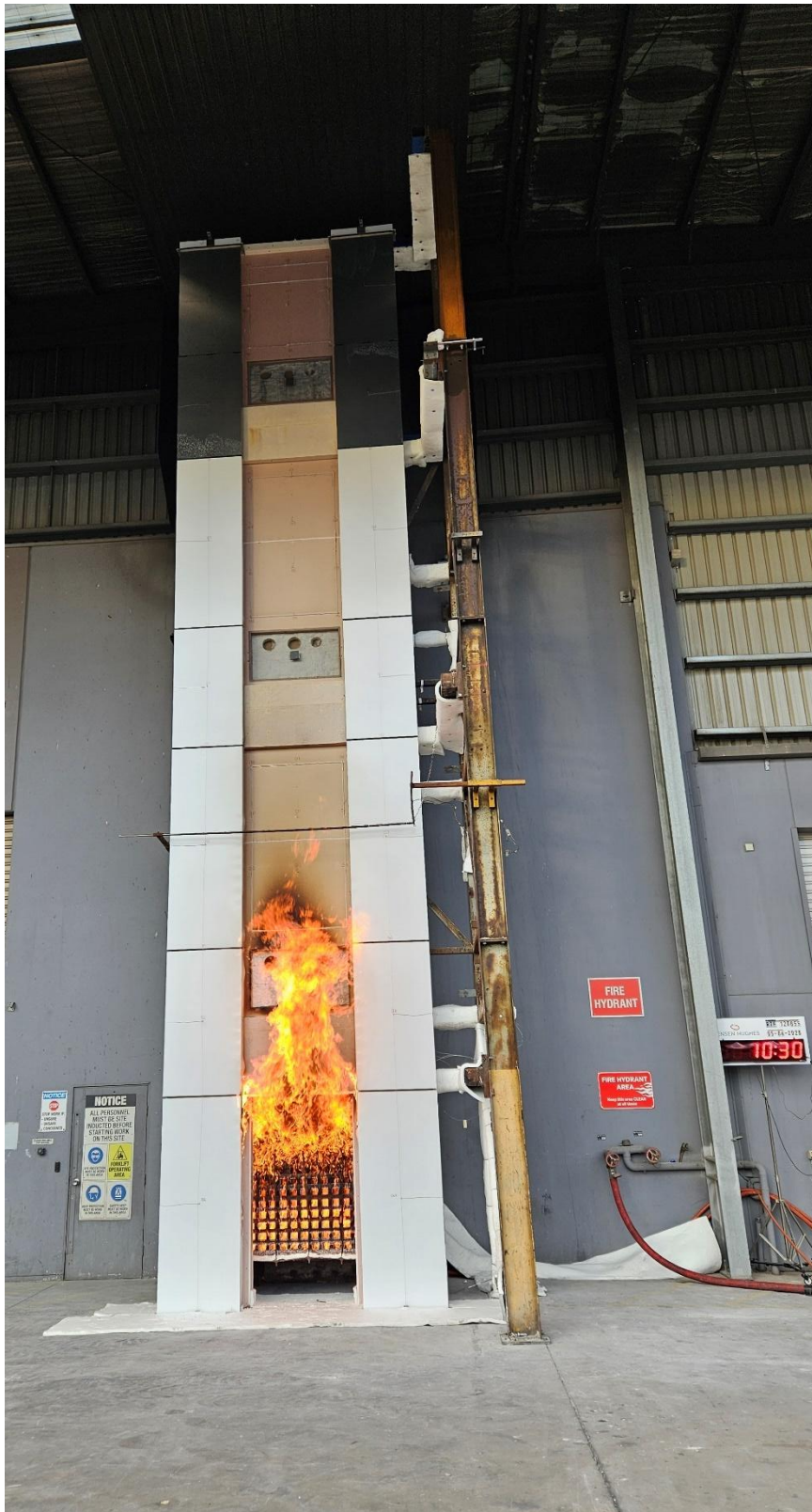
Figure 47 The external wall system during the test – 10 minutes 30 seconds after crib ignition
