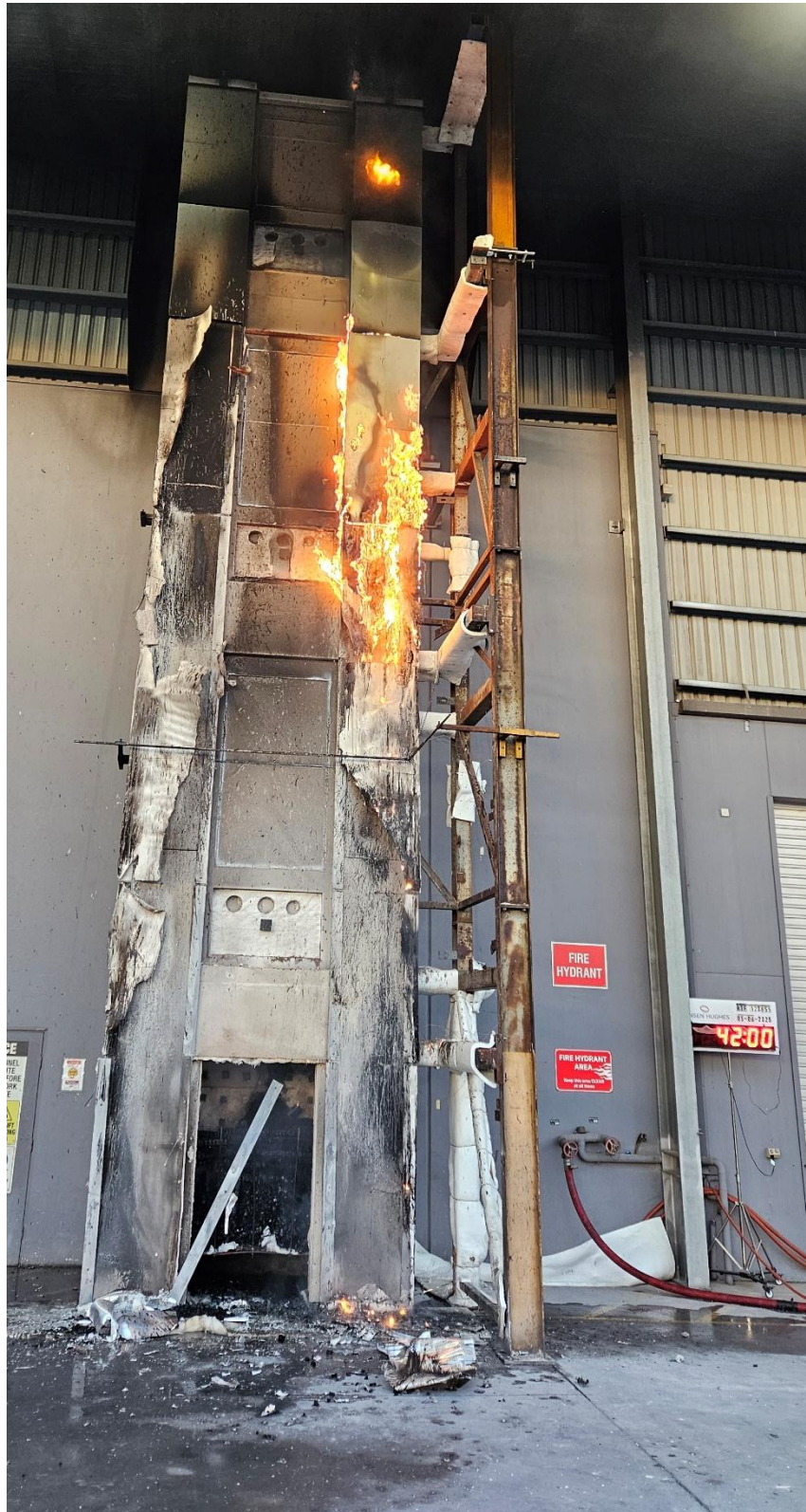
Figure 55 The external wall system – 12 minutes after crib was extinguished,
