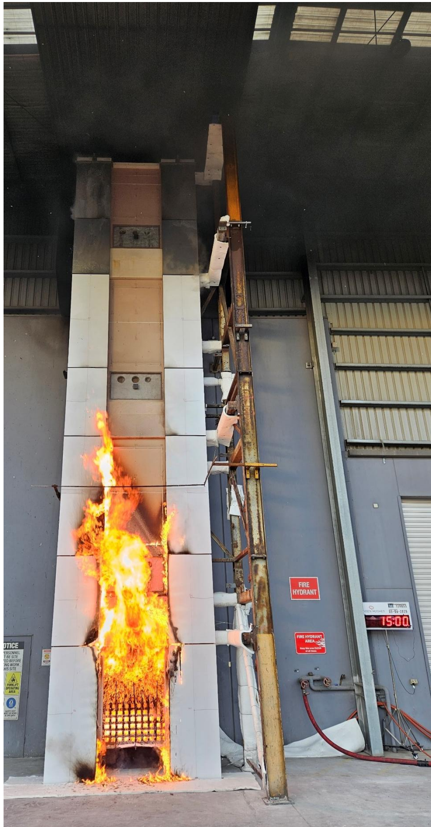
Figure 48 The external wall system during the test – 15 minutes after crib ignition
