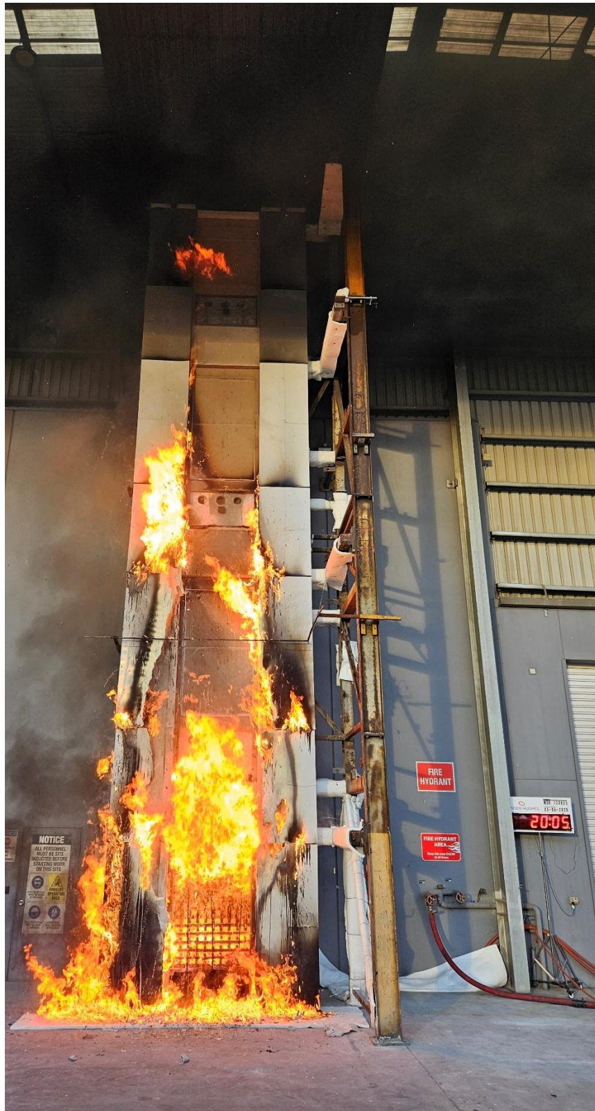
Figure 49 The external wall system during the test – 20 minutes 5 seconds after crib ignition
