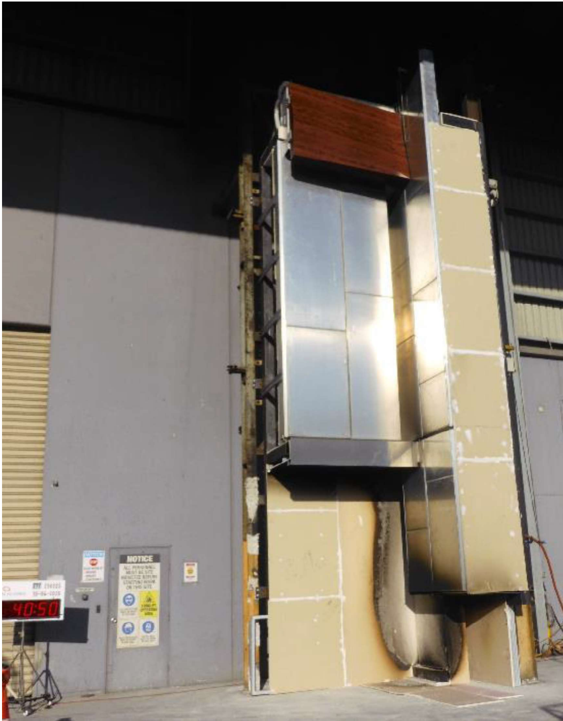
Figure 44 The specimen 40 minutes and 50 seconds into the test – 50 seconds after the burner was turned off.
