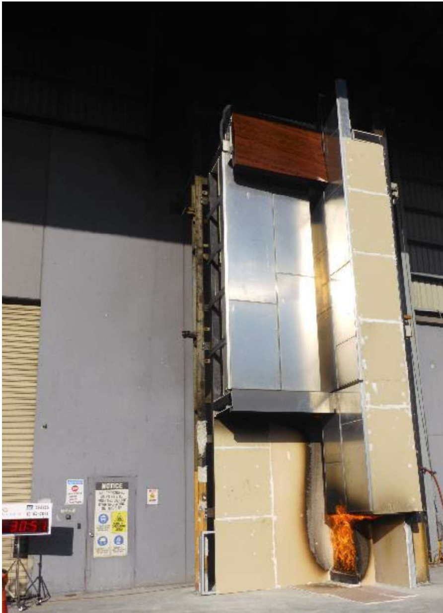
Figure 42 The specimen 30 minutes and 51 seconds into the test – 15 minutes 51 seconds after the burner output was increased to 300 kW.
