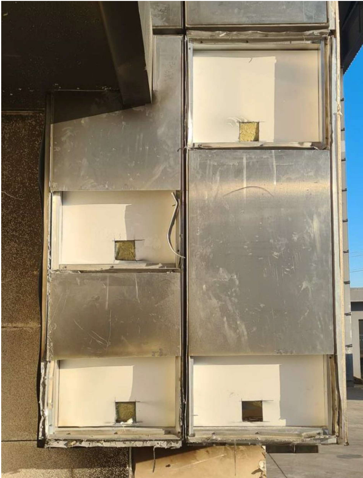
Figure 46 The exposed face of backpan of modules 6 and 7, respectively, after sampling at the end of the test.
