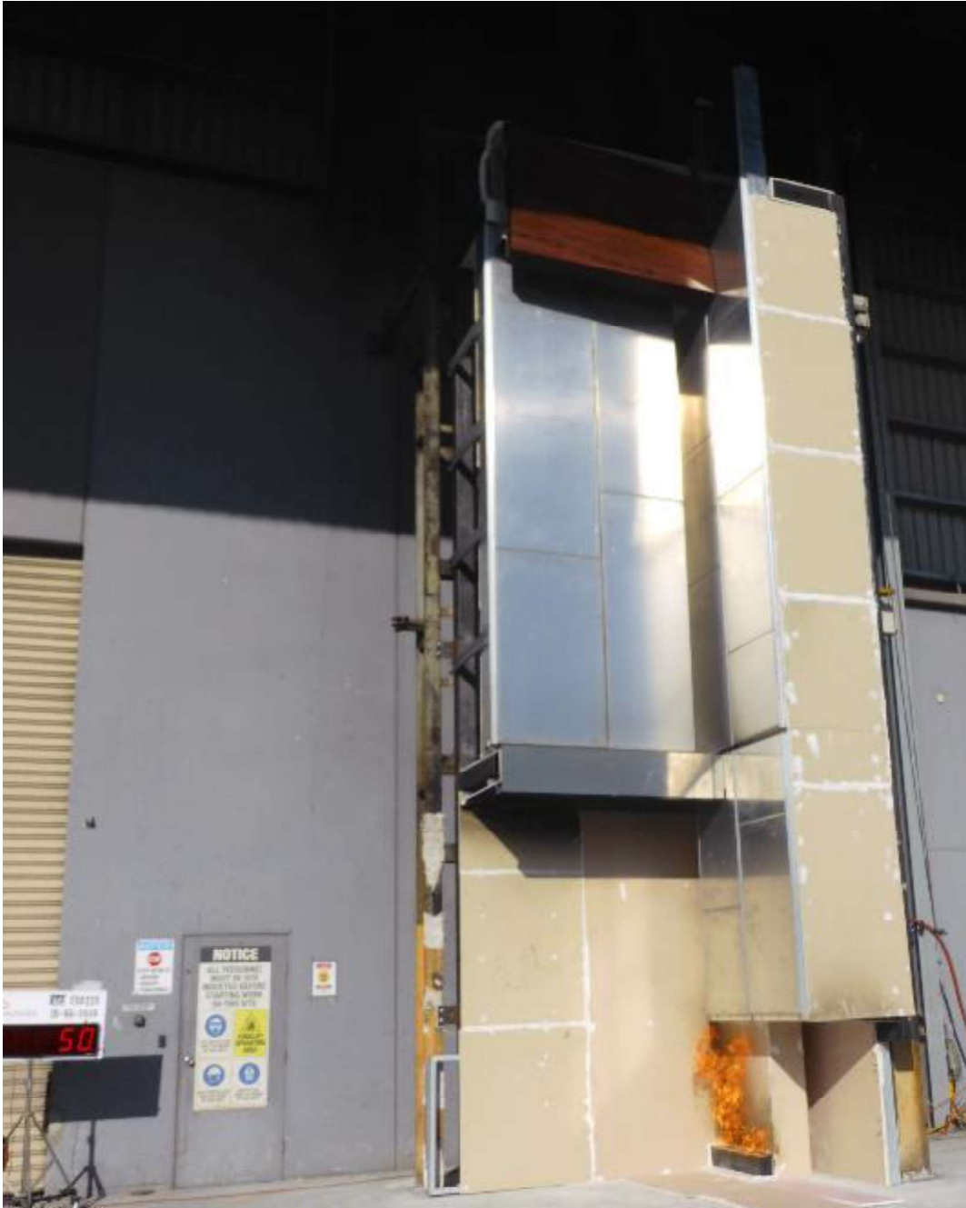
Figure 39 The specimen 50 seconds into the test with the burner at 500 kW
