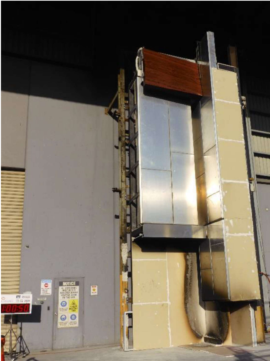
Figure 45 The exposed face of the specimen after the test
