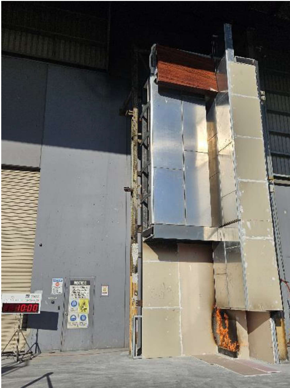
Figure 40 The specimen 10 minutes into the test with the burner at 100 kW
