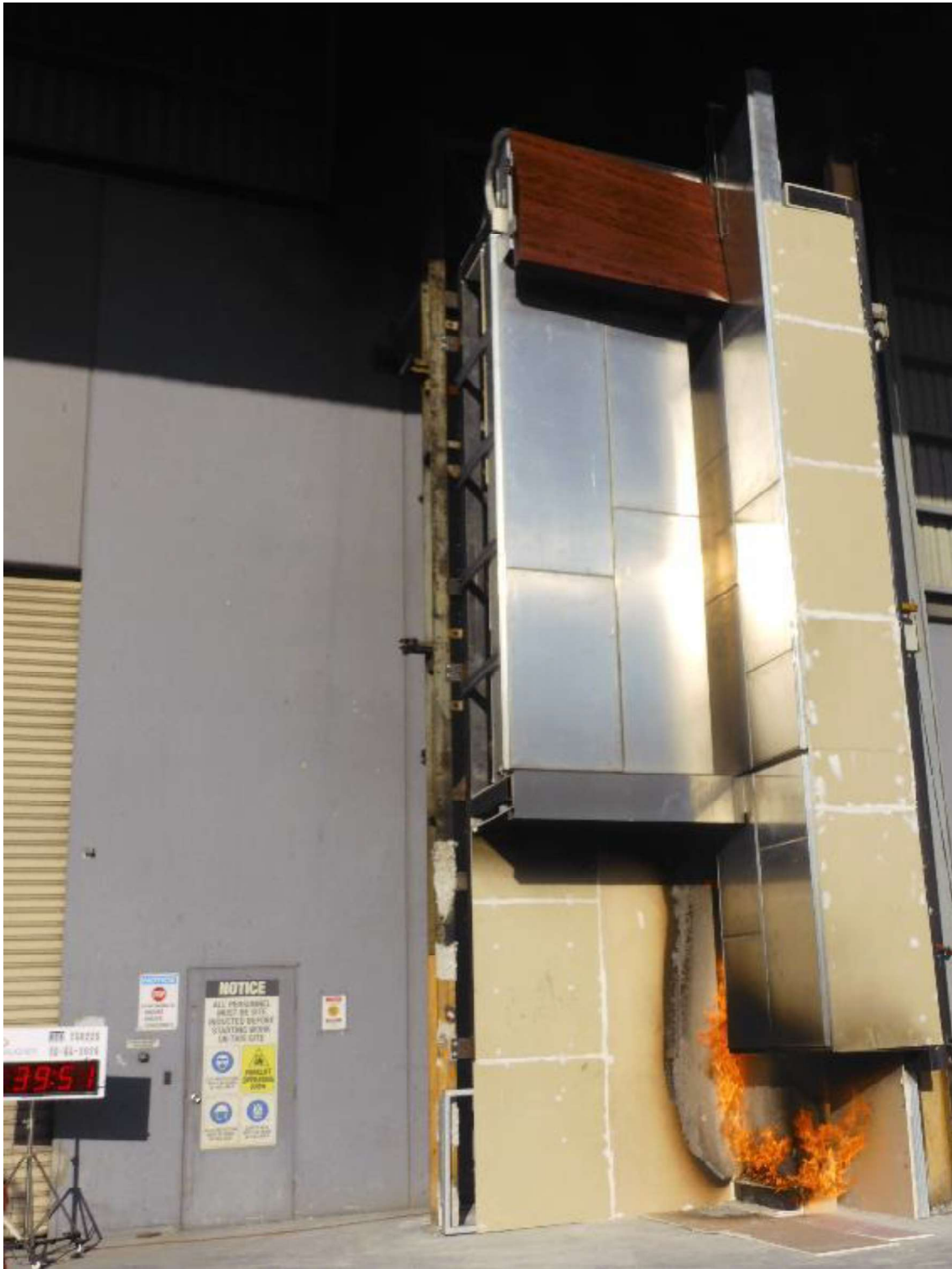
Figure 43 The specimen 39 minutes 51 seconds into the test – 24 minutes 51 seconds after the burner output was increased to 300 kW.
