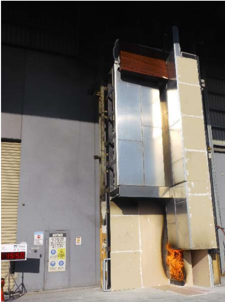
Figure 41 The specimen 15 minutes and 50 seconds into the test - 50 seconds after the burner output was increased to 300 kW.
