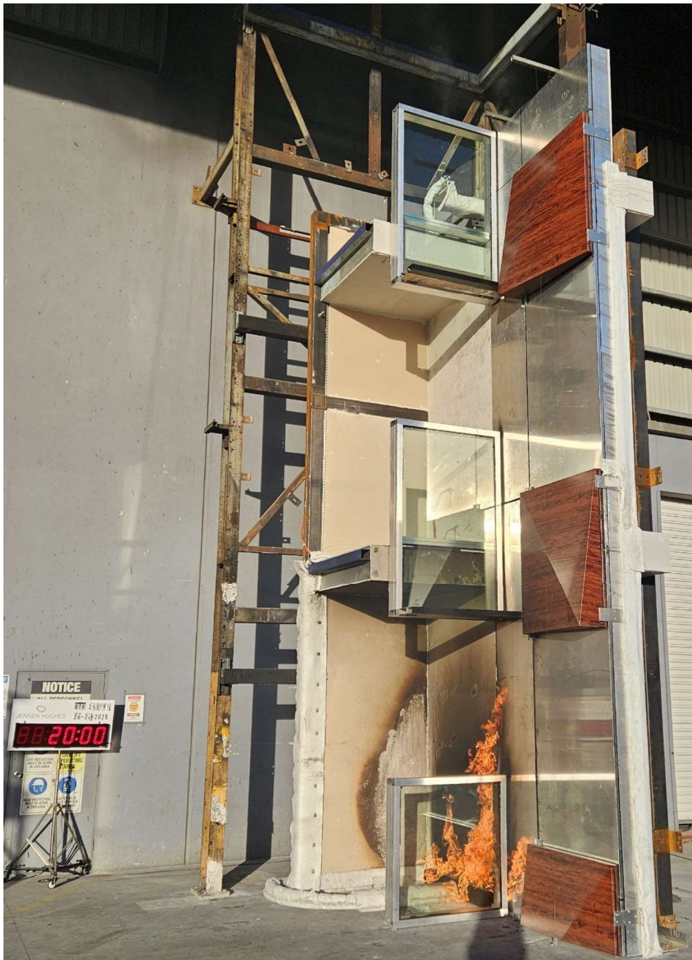
Figure 35 The specimen 20 minutes into the test – 5 minutes after the burner output was increased to 300 kW.
