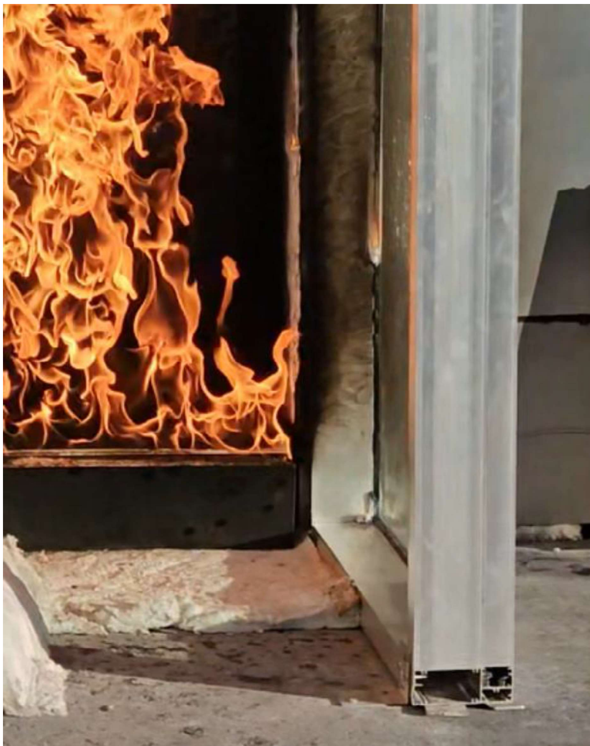
Figure 37 The specimen after 20 minutes into the test – sealant around the ground level balustrade on fire.
