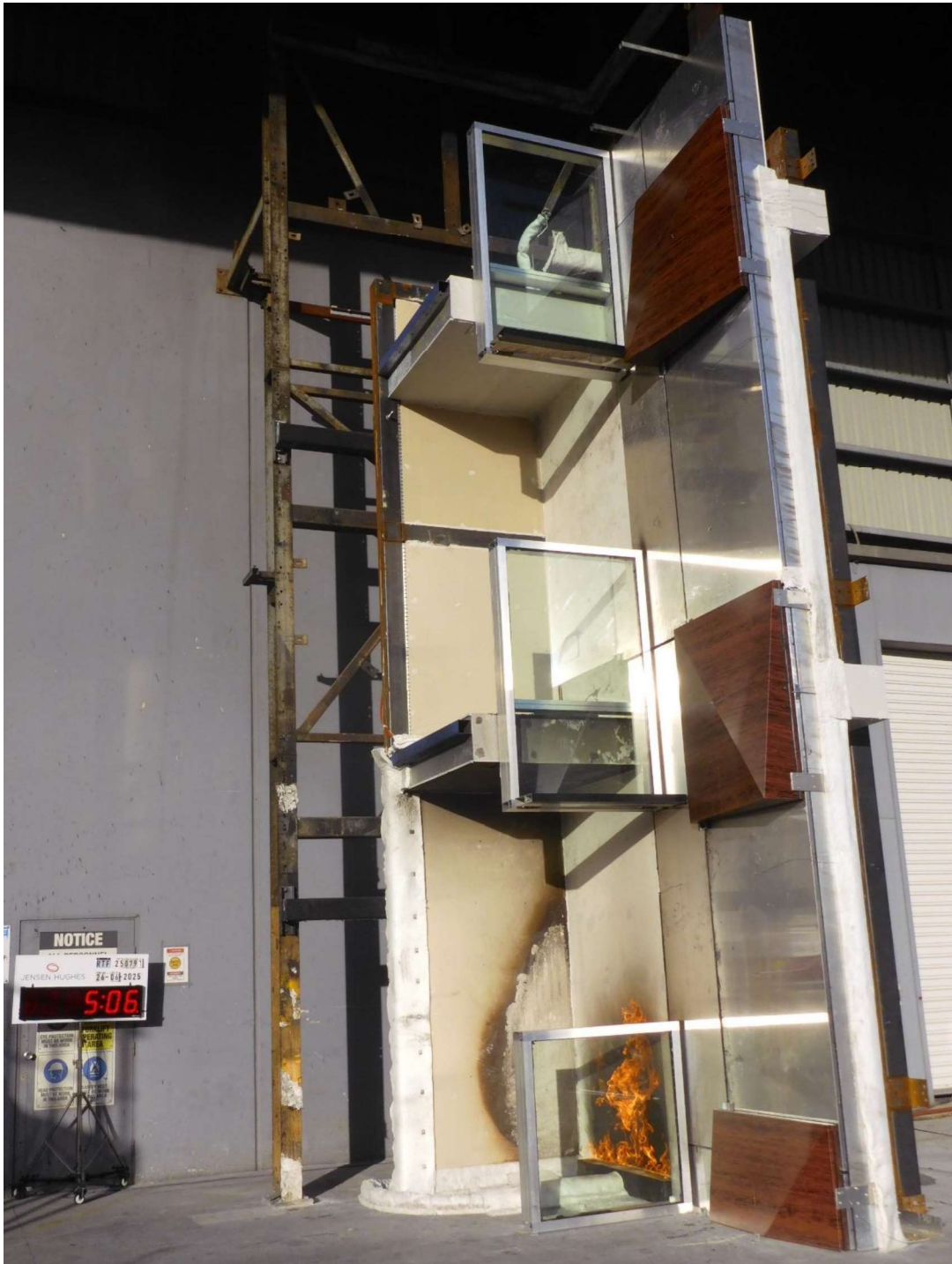
Figure 32 The specimen 5 minutes 6 seconds into the test with the burner at 100 kW.
