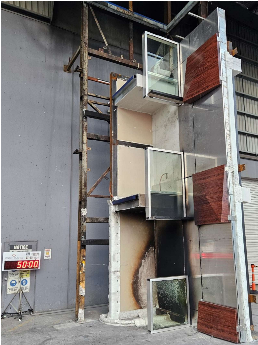
Figure 40 The specimen 50 minutes into the test – 35 minutes after the burner output was increased to 300 kW.
