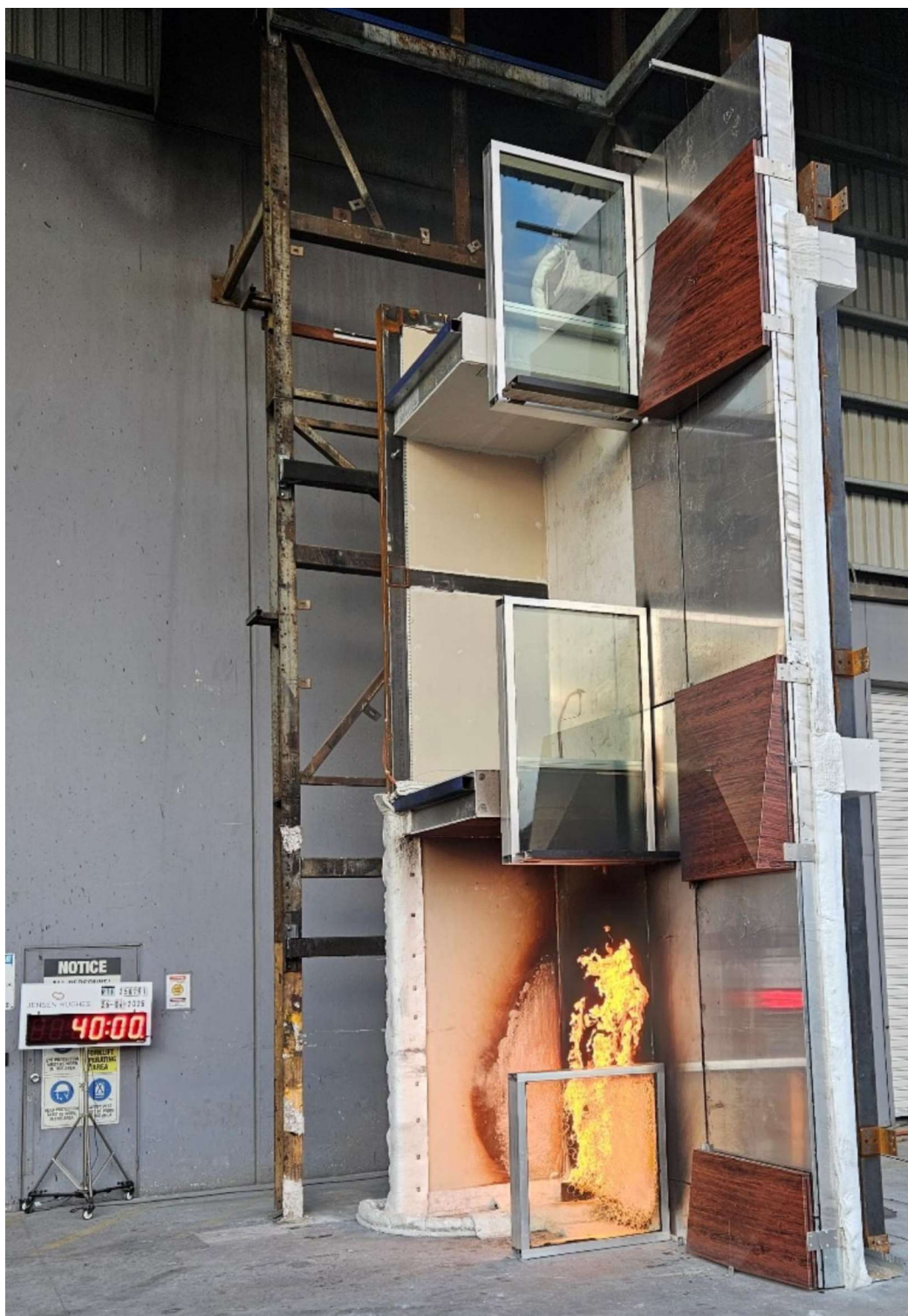
Figure 39 The specimen 40 minutes into the test – 25 minutes after the burner output was increased to 300 kW - burner was turned off
