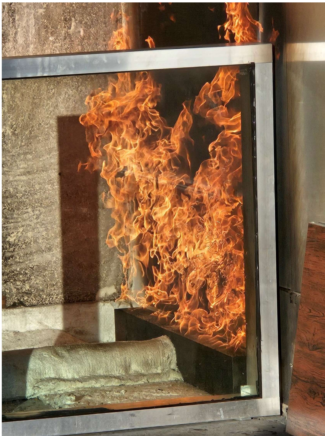
Figure 36 The specimen after 20 minutes into the test – formation of bubbles in the PVB interlayer of glazing.
