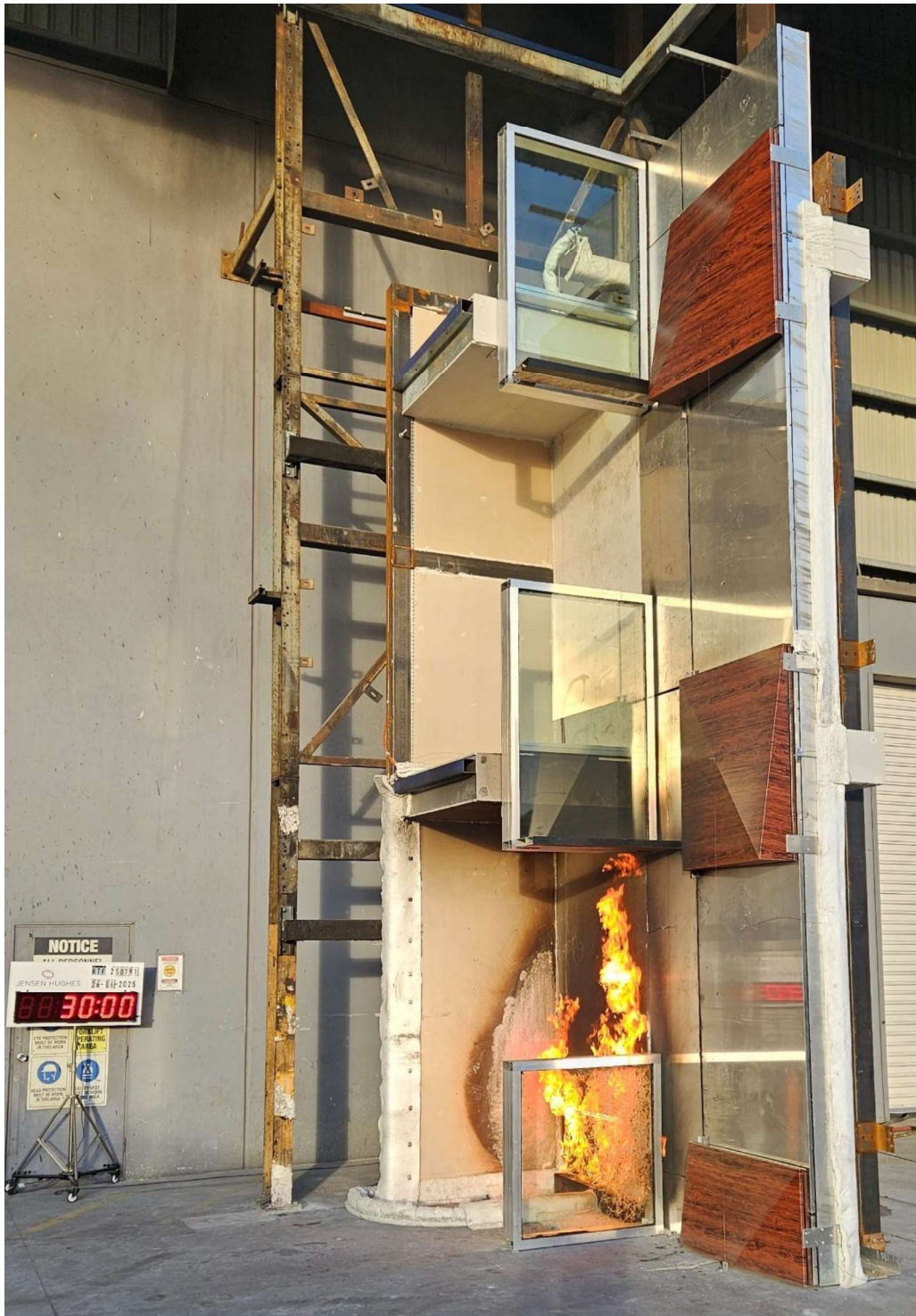
Figure 38 The specimen 30 minutes into the test – 15 minutes after the burner output was increased to 300 kW.
