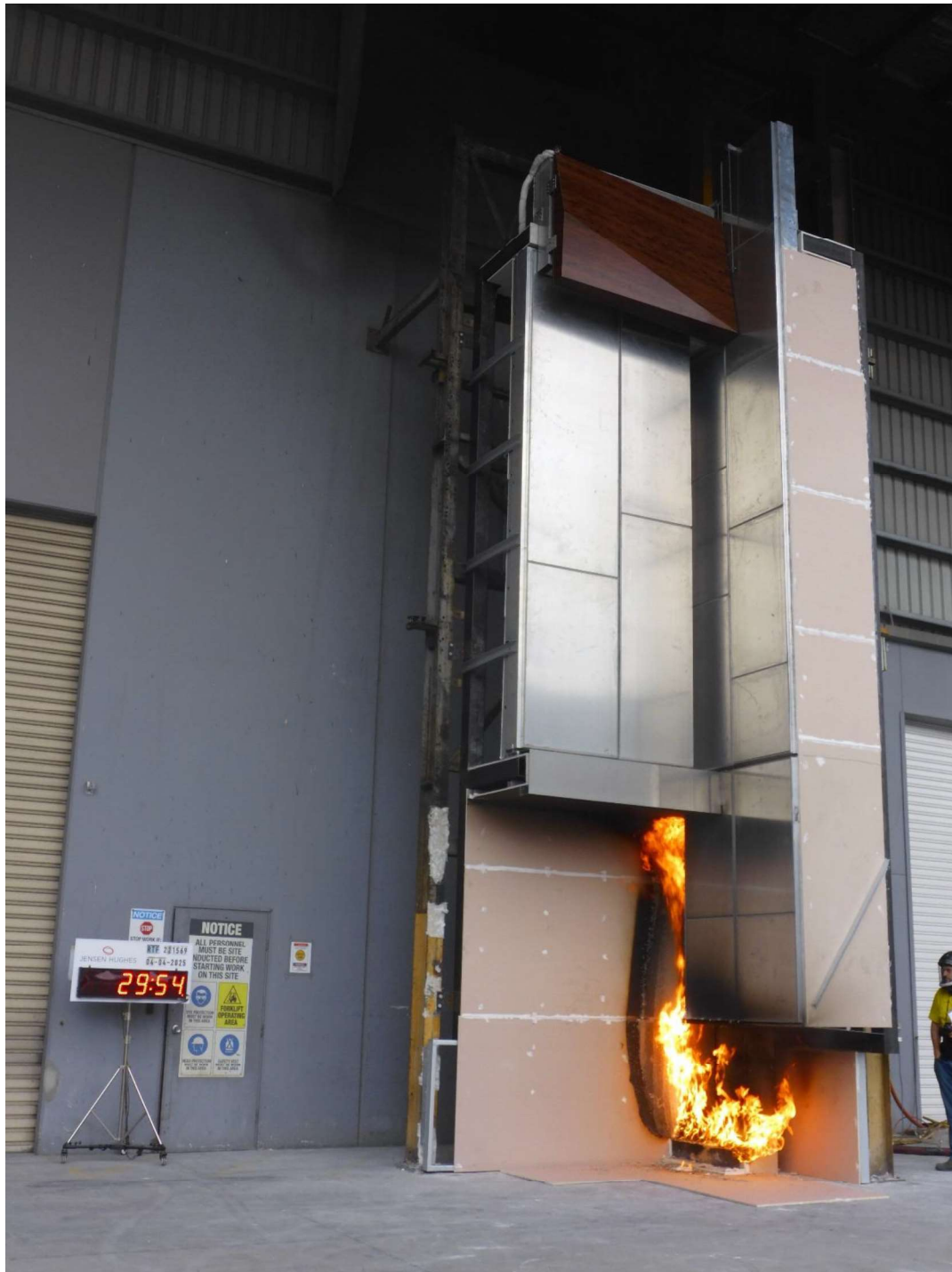
Figure 43 The specimen 29 minutes 54 seconds into the test – 14 minutes 55 seconds after the burner output was increased to 300 kW.
