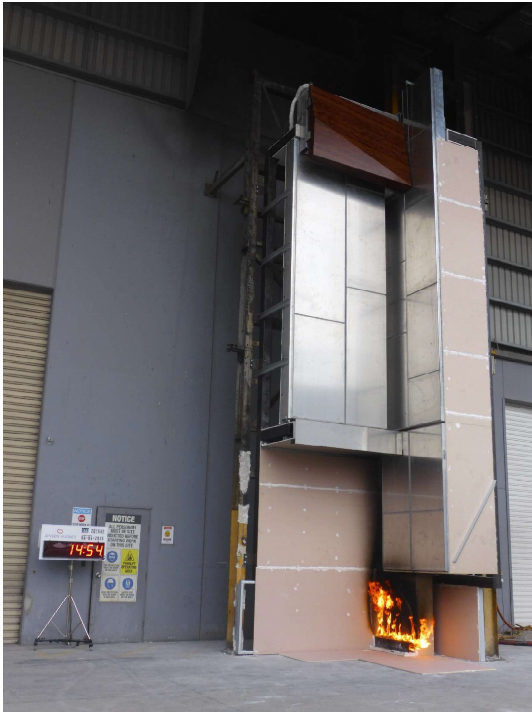
Figure 41 The specimen 14 minutes 54 seconds into the test with the burner at 100 kW
