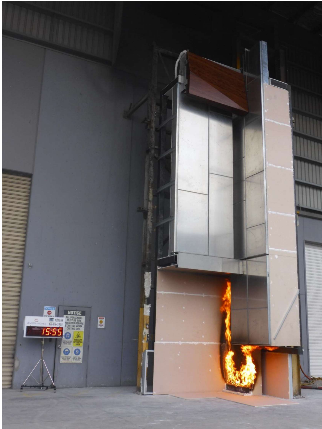
Figure 42 The specimen 15 minutes 55 seconds into the test - 55 seconds after the burner output was increased to 300 kW.
