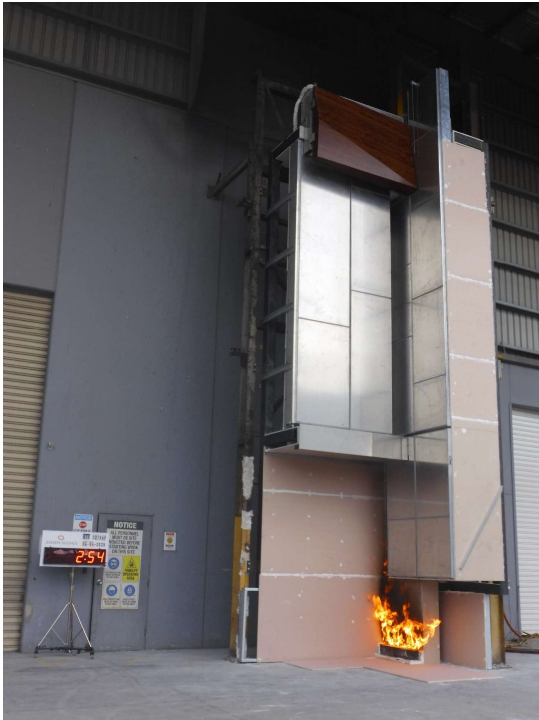
Figure 39 The specimen 2 minutes 54 seconds into the test with the burner at 100 kW.
