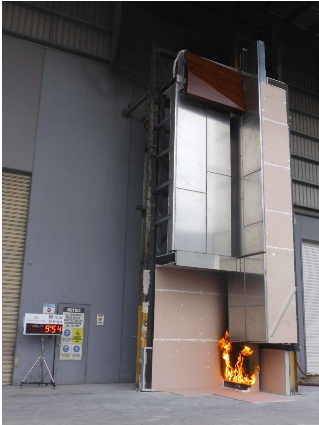
Figure 40 The specimen 9 minutes 54 seconds into the test with the burner at 100 kW
