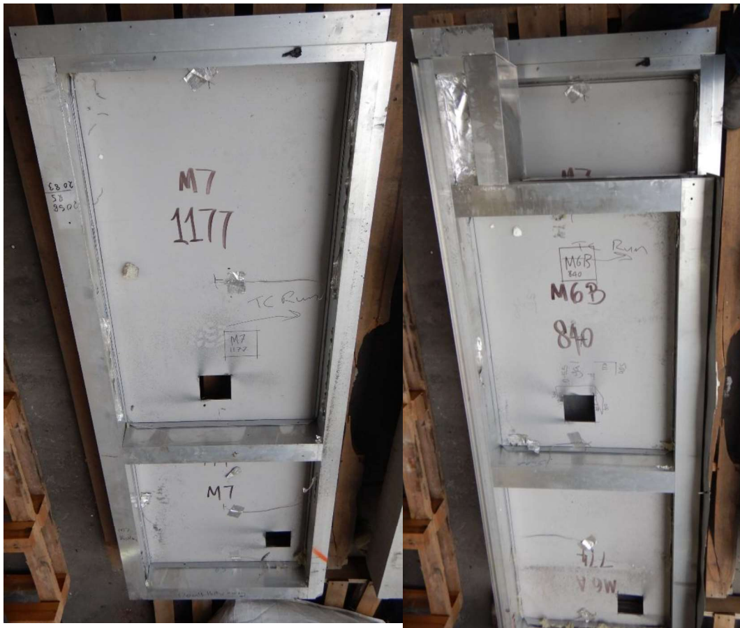
Figure 46 The unexposed face of backpan of modules 7 and 6, respectively, after sampling at the end of the test.
