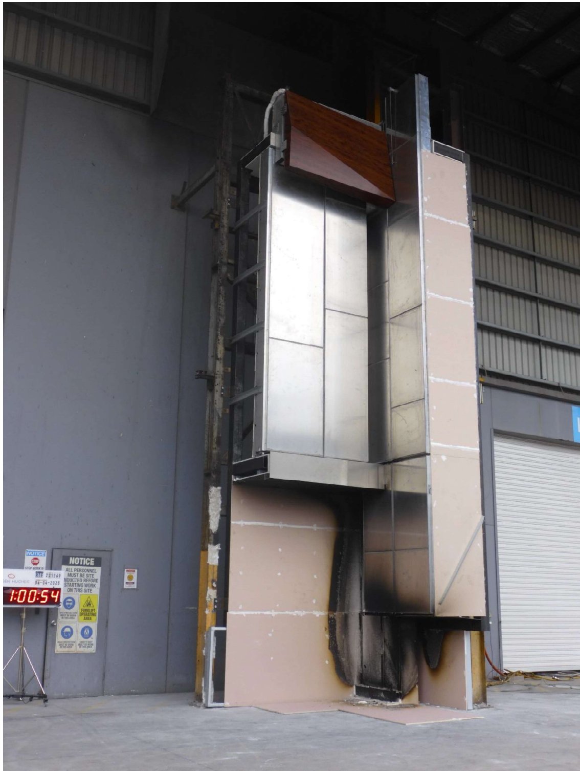
Figure 45 The specimen at the end of the test.
