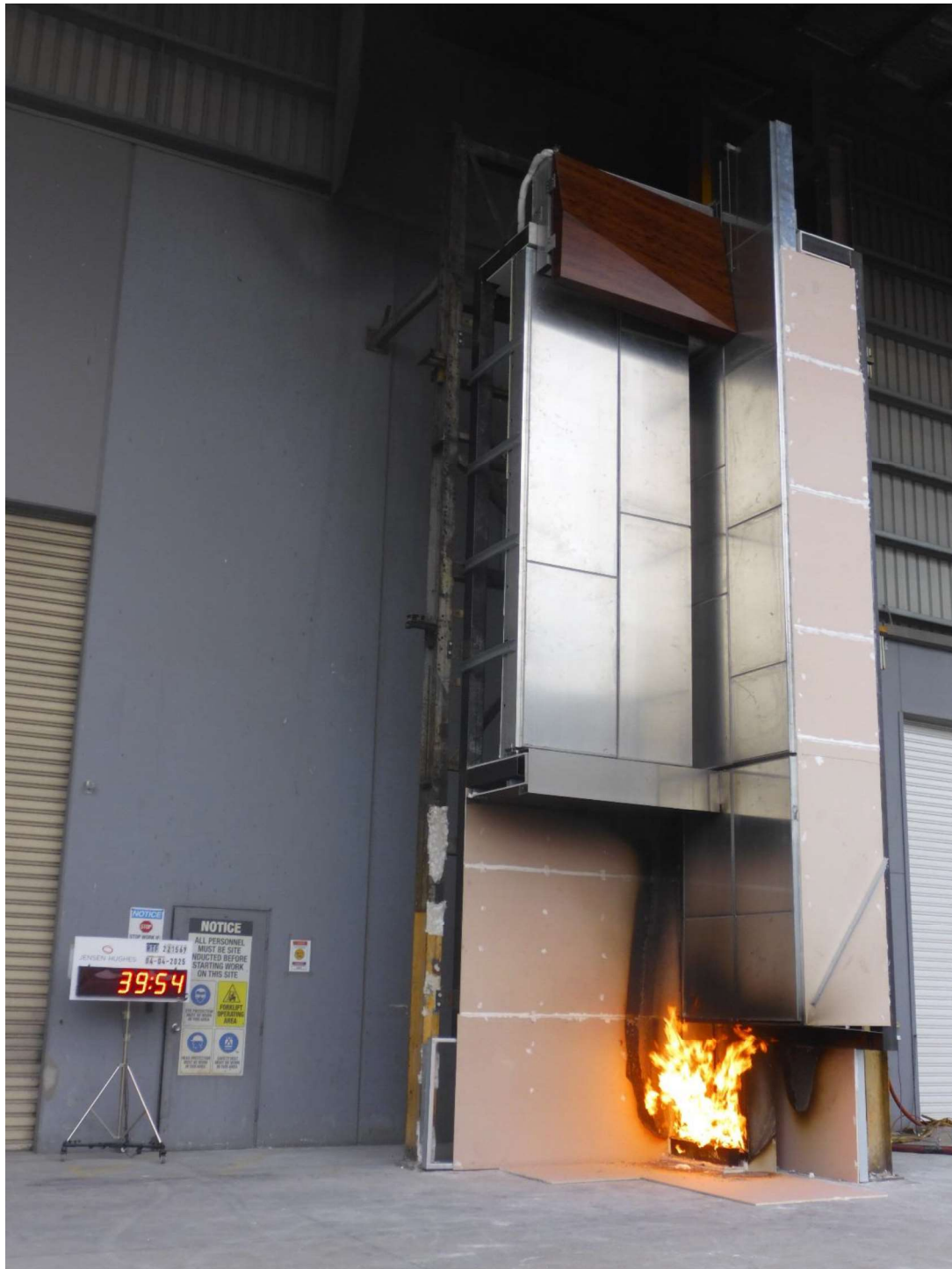
Figure 44 The specimen 39 minutes 54 seconds into the test – 24 minutes 55 seconds after the burner output was increased to 300 kW.
