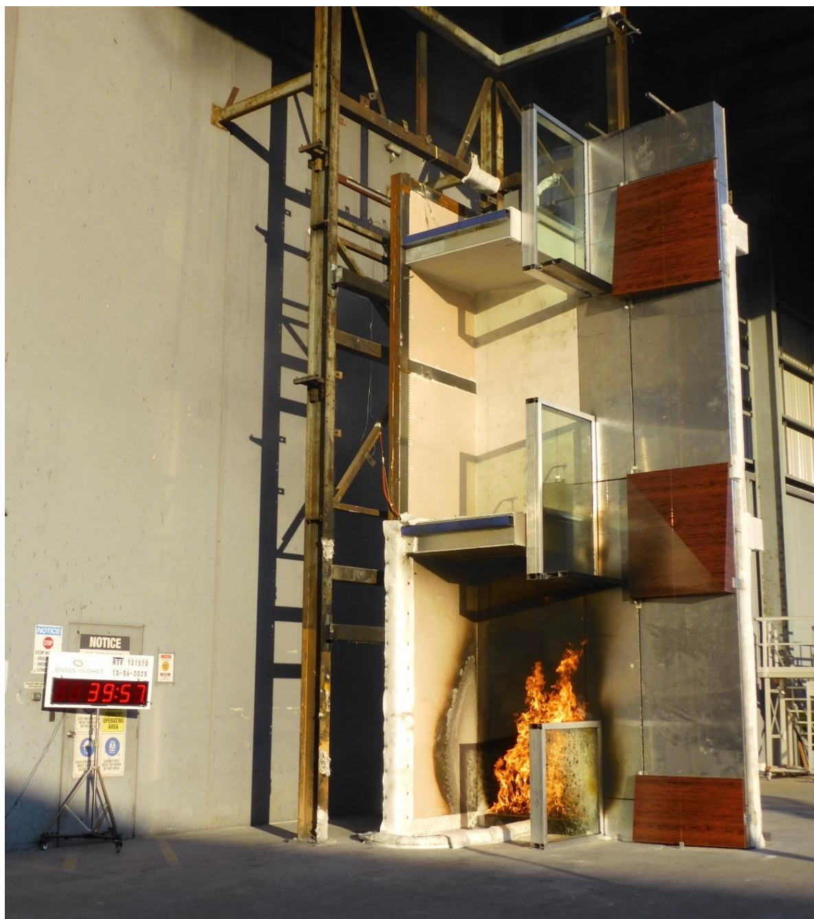
Figure 39 The specimen 39 minutes 57 seconds into the test – 24 minutes 57 seconds after the burner output was increased to 300 kW.
