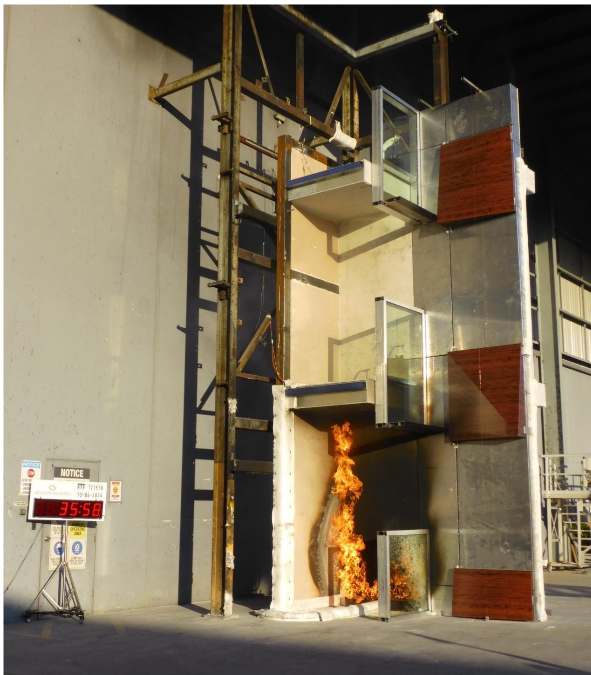
Figure 38 The specimen 35 minutes 58 seconds into the test – 20 minutes 58 seconds after the burner output was increased to 300 kW.
