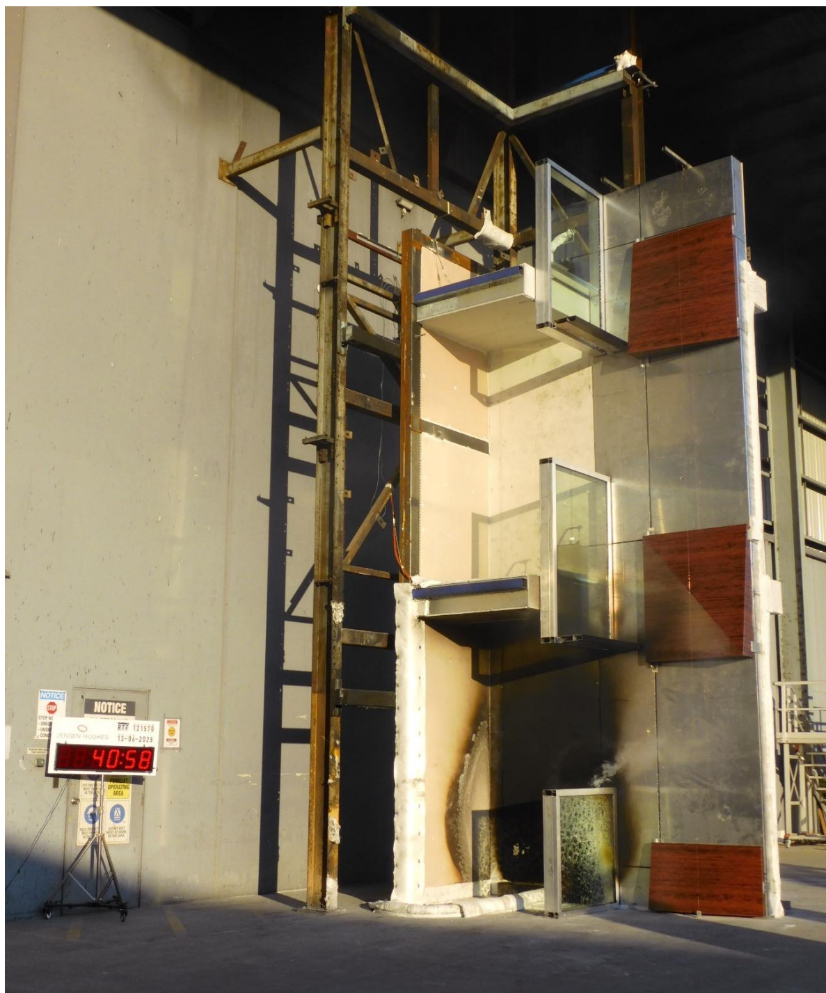
Figure 40 The specimen 40 minutes 58 seconds into the test – 58 seconds after the burner was turned off.
