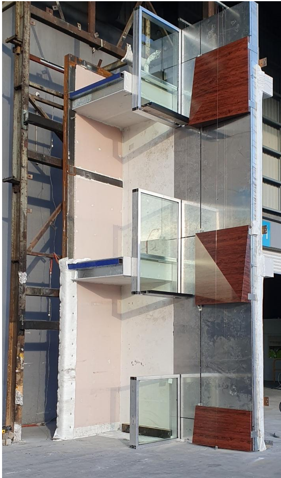
Figure 30 The specimen before the start of the test – exposed side.
