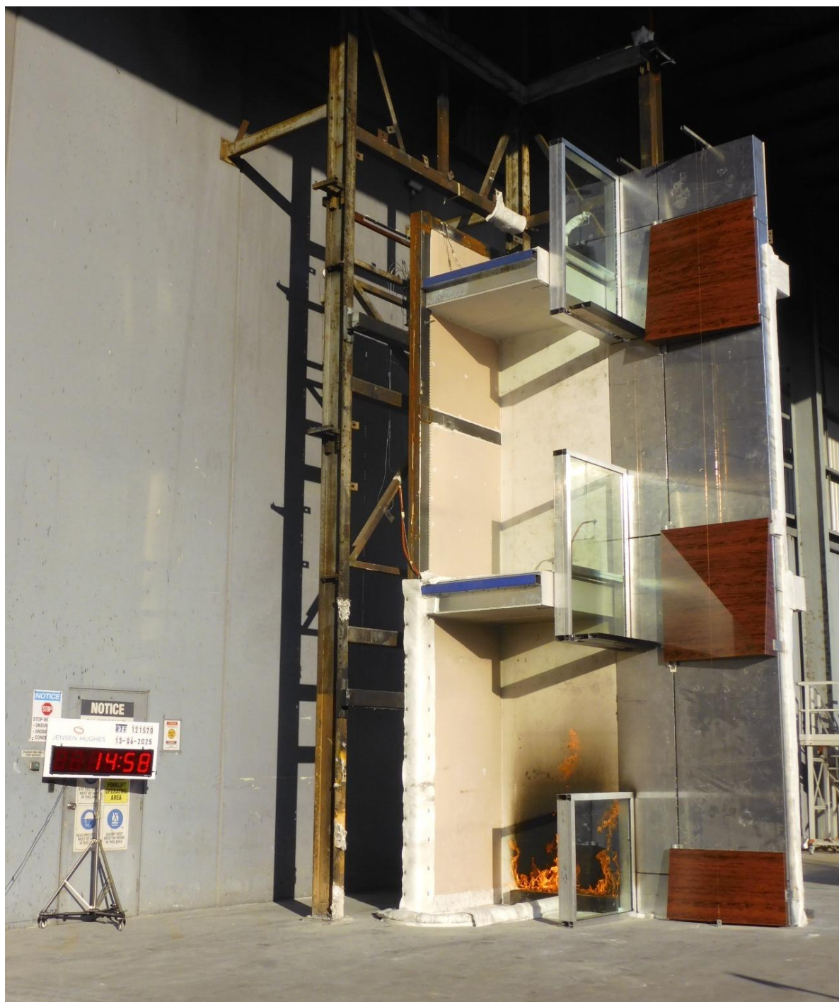
Figure 33 The specimen 14 minutes 58 seconds into the test with the burner at 100 kW.
