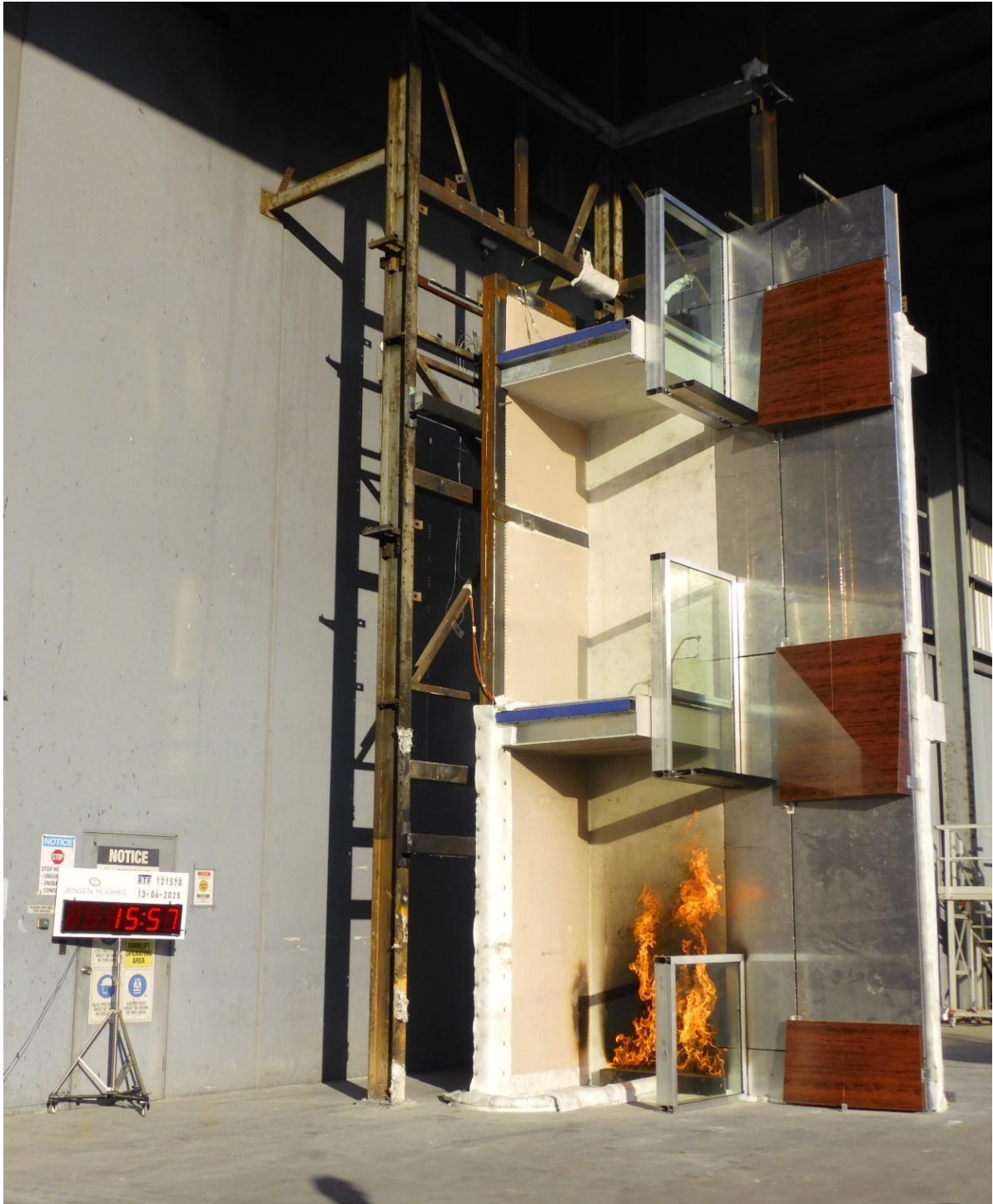
Figure 34 The specimen 15 minutes 57 seconds into the test – 57 seconds after the burner output was increased to 300 kW.
