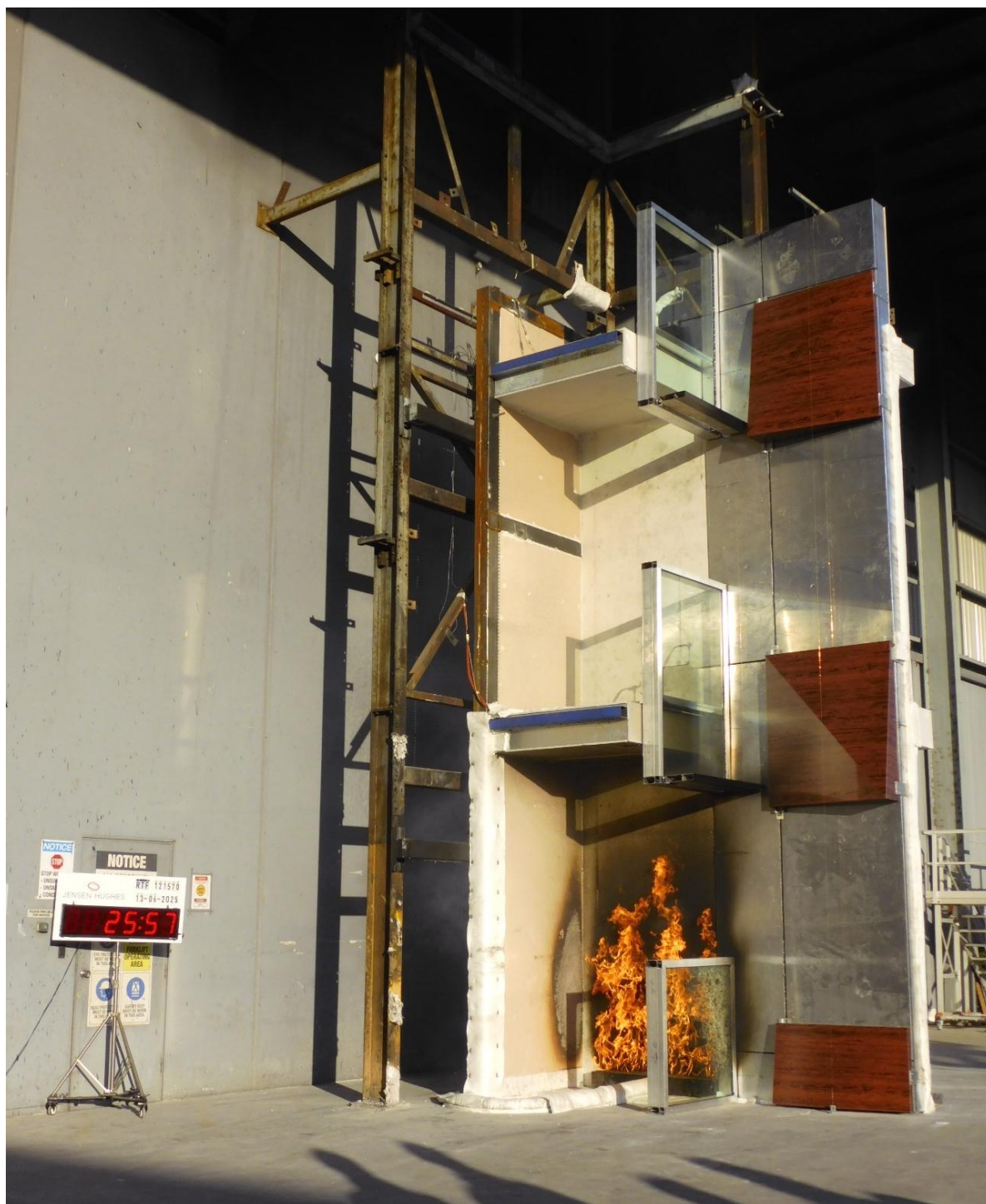
Figure 37 The specimen 25 minutes 57 seconds into the test – 10 minutes 57 seconds after the burner output was increased to 300 kW.
