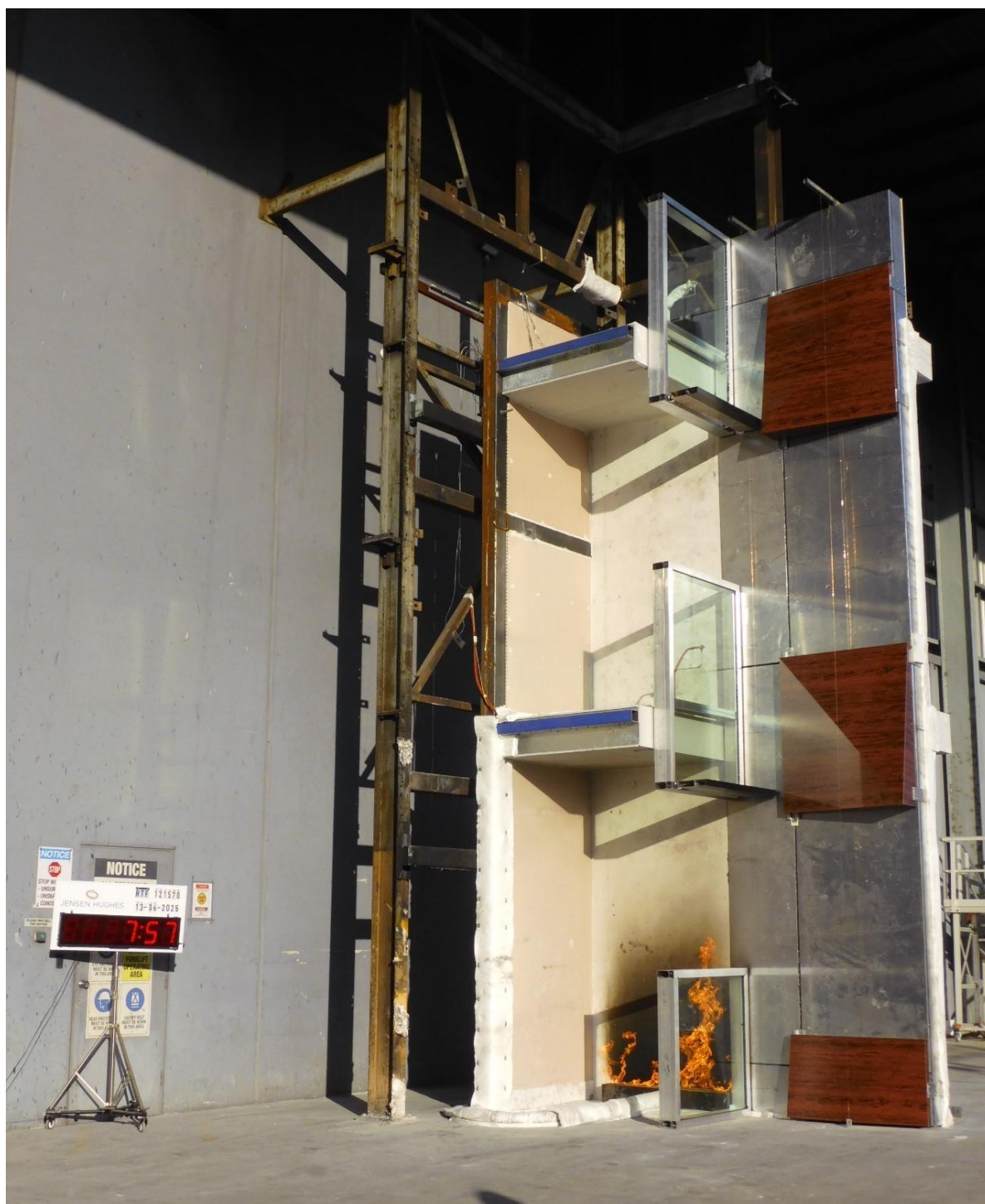
Figure 32 The specimen 7 minutes 57 seconds into the test with the burner at 100 kW.
