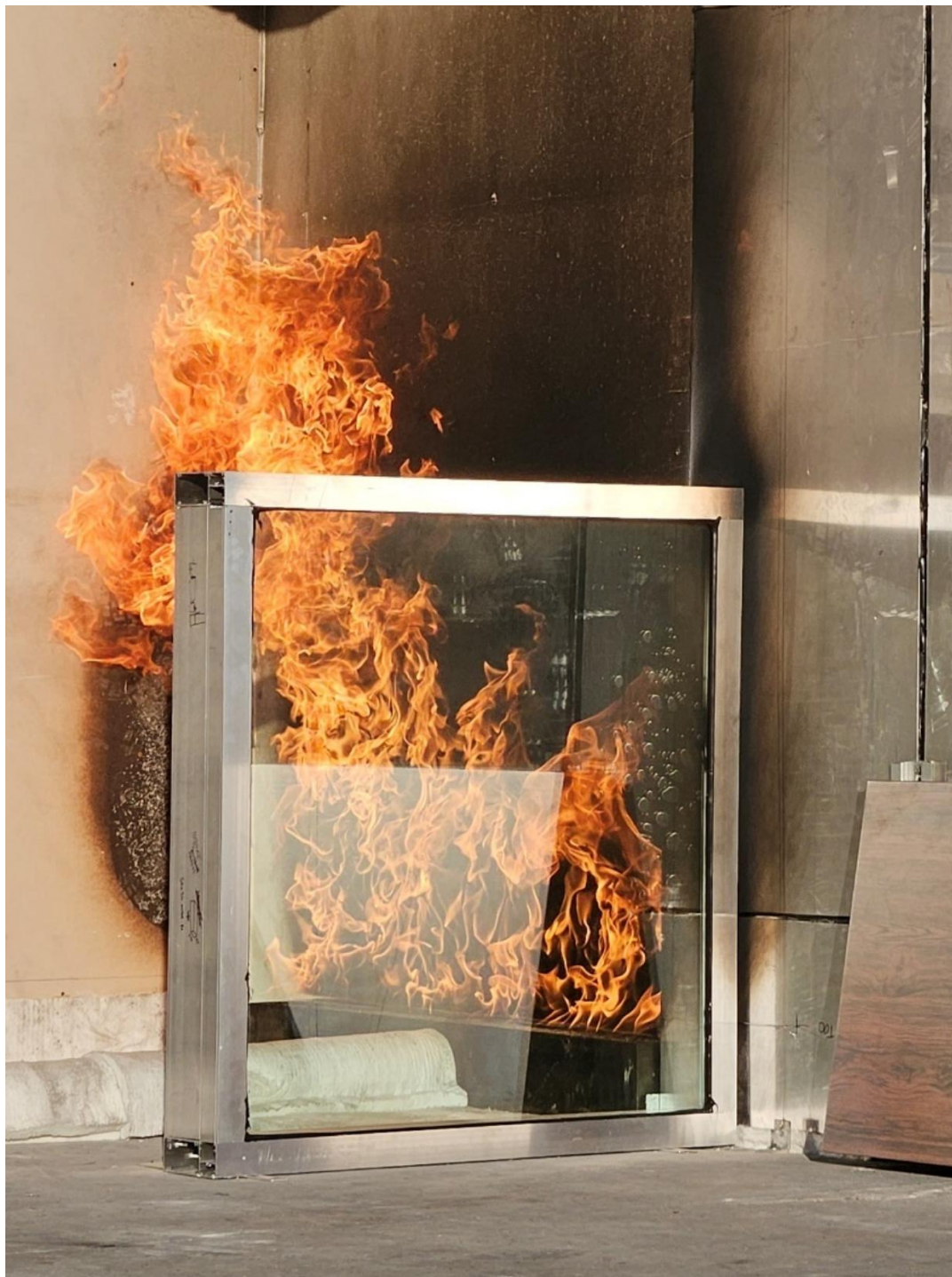
Figure 36 The specimen 18 minutes 40 seconds into the test – formation of bubbles in the PVB interlayer of glazing.
