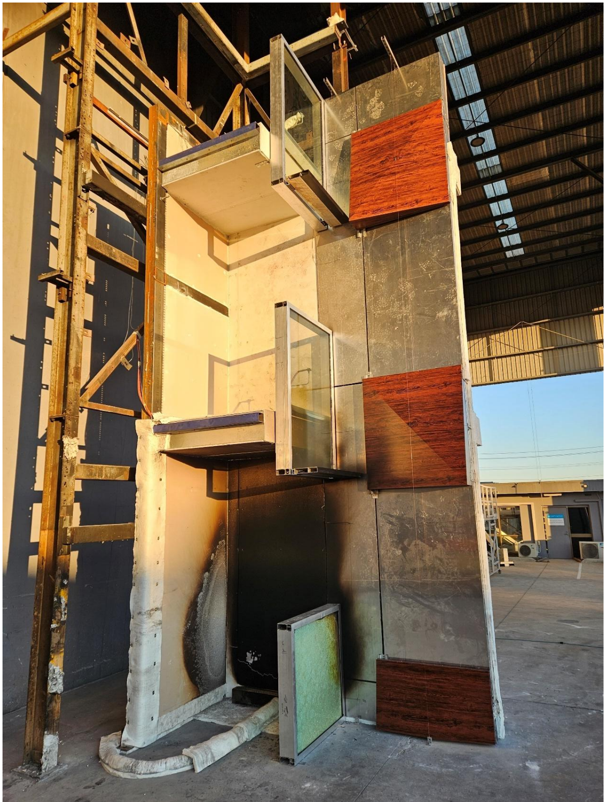
Figure 42 Specimen at the end of the test.
