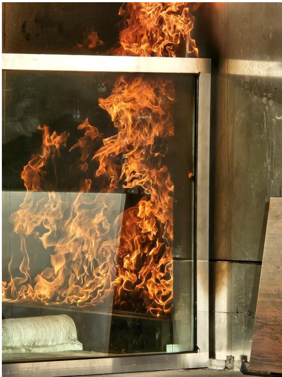
Figure 35 The specimen 17 minutes 30 seconds into the test – sealant around the ground level balustrade on fire.
