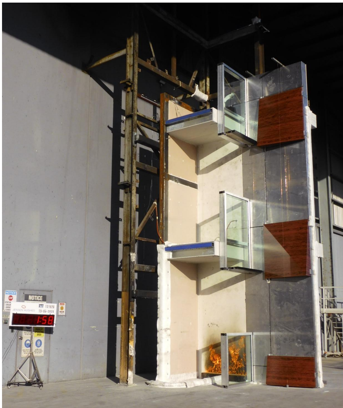
Figure 31 The specimen 1 minute 58 seconds into the test with the burner at 100 kW.
